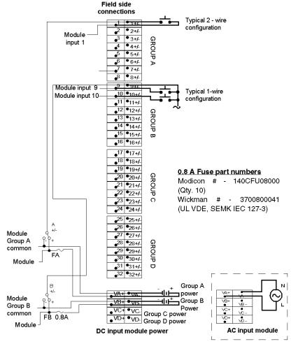
**NOTE:** The terminal block commoning strip, Modicon # 140 CFX 001 10 (Qty. 10), can be used to jumper the power between groups.
