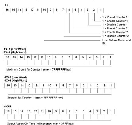
**NOTE:** Zero set into any 4X register pair for 32 bit values or any 4X register means no change.
