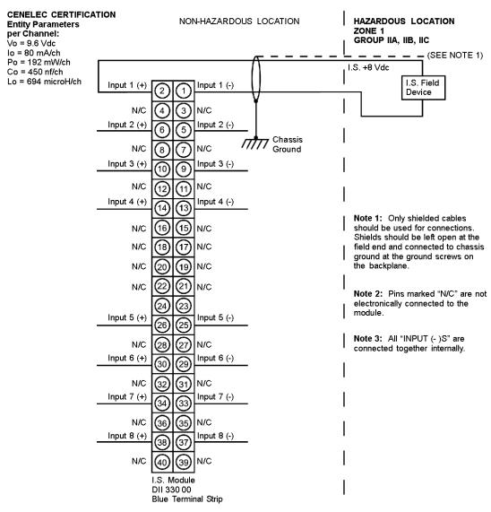
31001365 Rev 00 140 DII 330 00 Wiring Diagram
