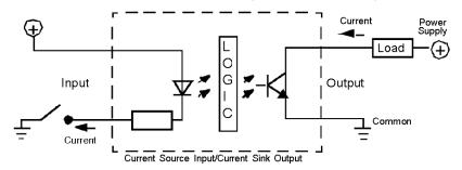
**Current Sinking** describes a physical implementation of the I/O hardware, which when in the *true state*, sinks current from the external load.
