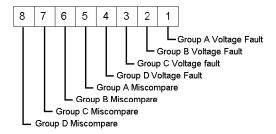
The voltage fault bit is set when the field supply is not present, or the group fuse is blown.
