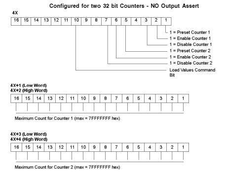
**NOTE:** Zero set into any 4X register pair for 32 bit values or any 4X register means no change.
