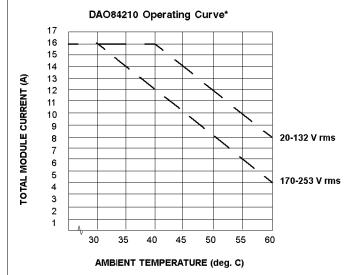
$^{*}$  The specifications stated are pending UL/CSA approval. This module was originally approved at 2 A each point; and 12 A, 0 ... 50° C (115 Vac) and 0 ... 50° C (230 Vac) per module.
