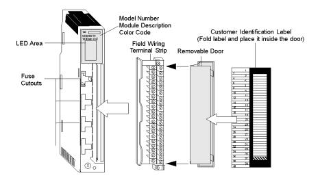
**NOTE:** When field wiring the I/O modules, the maximum wire size that should be used on a field wiring terminal is 1-14 AWG or 2-16 AWG; the minimum size is 20 AWG.
