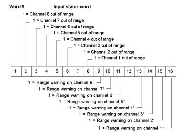
\* A range warning is issued when a channel input exceeds the rated input value, as shown in the following table. An out-of-range bit is set when a channel input exceeds the rated input value by 2.4% or when a broken wire is sensed on the channel. The warning bit is cleared when the out-of-range bit is set.
