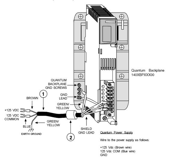
The following table provides a list of parts for the 125 Vdc Powered Installation Figure..
