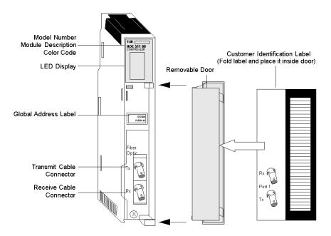
**NOTE:** The NOE51100 is equipped with one RJ45 connector instead of the fiber optic connectors (as shown above on the NOE55100).
