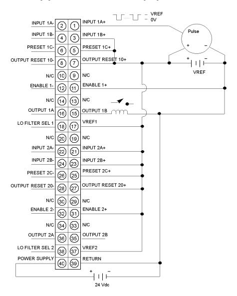
The preceding wiring diagram shows single ended connections for:.
