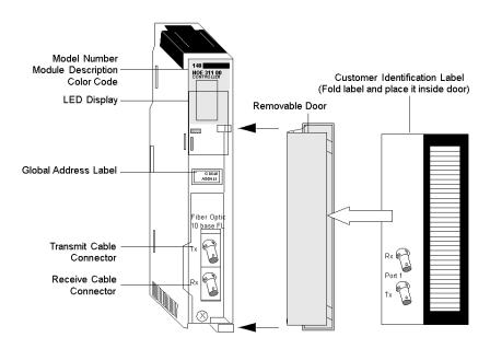
**NOTE:** The NOE31100 is equipped with one RJ-45 connector instead of the fiber optic connectors (as shown above on the NOE35100).
