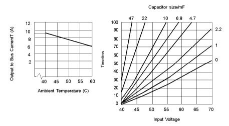
**NOTE:** Tolerance to input interruptions may be increased by adding  $a \ge 80$  Vdc electrolytic capacitor between 5 and 6 of the power terminal strip. Refer to the hold-up capacitor timing chart (above) for capacitor values.
