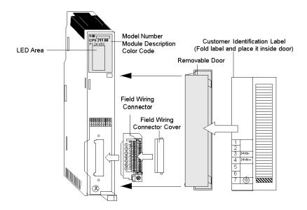
**NOTE:** When field wiring the power supply module, the maximum wire size that should be used is 1 - 14 AWG or 2 - 16 AWG; the minimum is 20 AWG.
