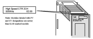
In modules prior to V02.00, when Rate Sample mode was selected, input was always handled as if it were generated by a pulse encoder. For example, 60 count per revolution encoders, either pulse or quadrature types, would give a rate of 60 for a one-second revolution when the interval was set for one second.
