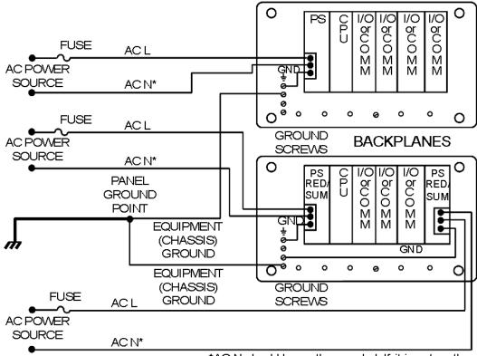
\*AC N should be earth grounded. If it is not earth grounded, it must be fused (refer to local codes).
