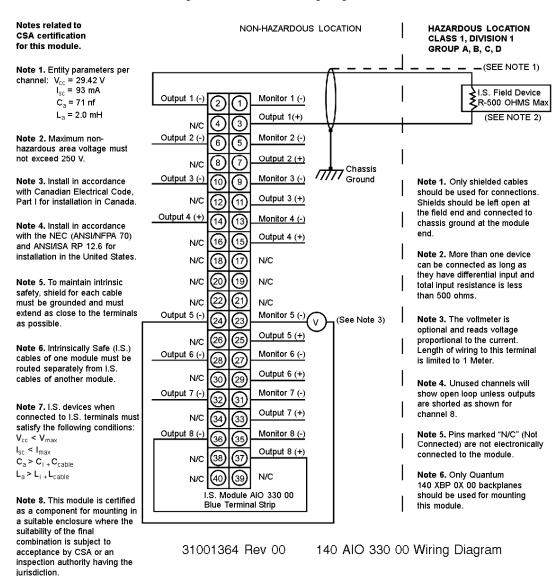
The following is a FM certified wiring diagram for this module.
