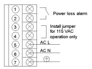
**NOTE:** A normally closed relay contact rated at 220 Vac, 6A / 30 Vdc, 5A is available on terminals 1 and 2 of the power terminal strip. This contact set may be used to signal input power OFF. The relay will de-energize when input power drops below 8 Vdc.
