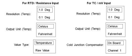
Configure each channel (1 through 8) appropriate to the module input type selected.
