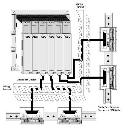
**NOTE:** Ensure that the wiring panduits are large enough to support 12 ft. cables.
