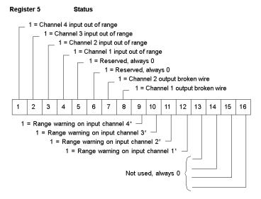
\* A range warning is issued when a channel input is outside the rated input value, as shown in the following table. Warning bits stay on after out of range bits are set. An out-of-range bit is set when a channel input exceeds the rated input value by 2.4%. Out of range bits are also set if inputs drop below 0.5V (1 ... 5V mode) or 2.08 mA (4 ... 20 mA mode).
