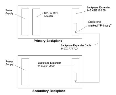
**NOTE:** Cable must be installed before powering up the backplanes.
