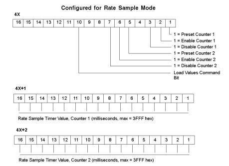
**NOTE:** Zero set into any 4X register or any 4X register pair for 32 bit values means no change.
