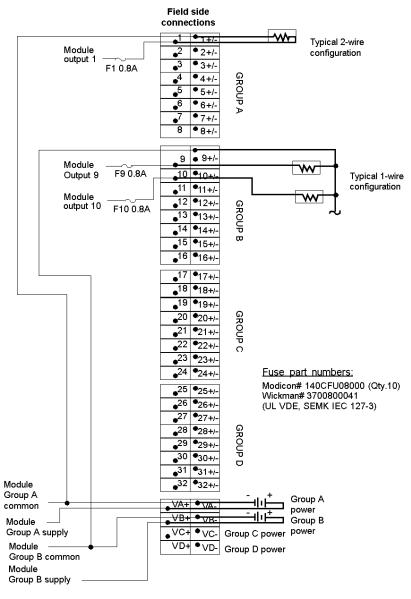
**NOTE:** The terminal block commoning strip, Modicon # 140 CFX 001 10 (QTY. 10), can be used to jumper the power between groups.
