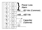
**NOTE:** A normally closed relay contact rated at 220 Vac, 6A / 30 Vdc, 5A is available on terminals 1 and 2 of the power terminal strip. This contact set may be used to signal input power OFF, or a power supply failure.
