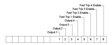
In Fast Trip Mode, each output can be turned ON by the Command Bit (e.g., Output 1) or by the corresponding Input Bit plus the Fast Trip Enable Bit (e.g., last order Input 1 controls Output 1 directly).
