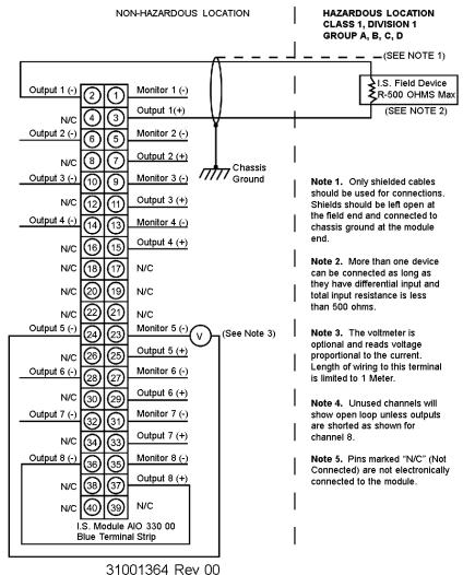
AIO 330 00 Wiring Diagram (Analog Output)
