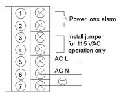
**NOTE:** A normally closed relay contact rated at 220 Vac, 6A / 30 Vdc, 5A is available on terminals 1 and 2 of the power terminal strip. This contact set may be used to signal input power OFF. The relay will de-energize when input power drops below 8 Vdc.
