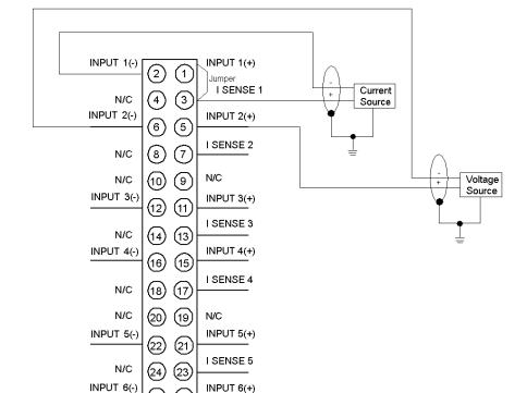
The following figure shows the wiring diagram for the 140ACl03000 module.
