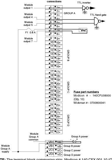
**NOTE:** The terminal block commoning strip, Modicon # 140 CFX 001 10 (Qty. 10) can be used to jumper the power between groups.
