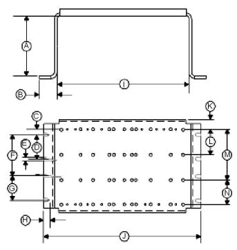
Diameter of the mounting holes: 6.6 mm / 0.26 inches
