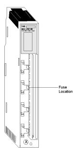
**NOTE:** Turn off power to the module and remove the field wiring terminal strip to gain access to the fuse.
