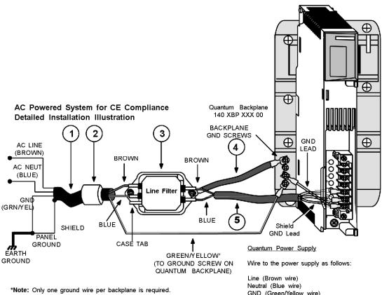
In redundant and summable systems, this lead is not connected for the additional line filter/power supply.
