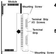
4 Install the appropriate terminal strip (if required) on the module, and with a philips screwdriver tighten the mounting screws at the top and bottom of the terminal.
