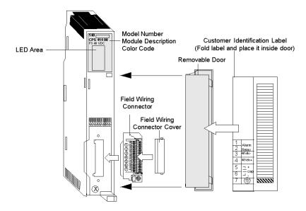
**NOTE:** When field wiring the power supply module, the maximum wire size that should be used is 1 - 14 AWG or 2 - 16 AWG; the minimum is 20 AWG.
