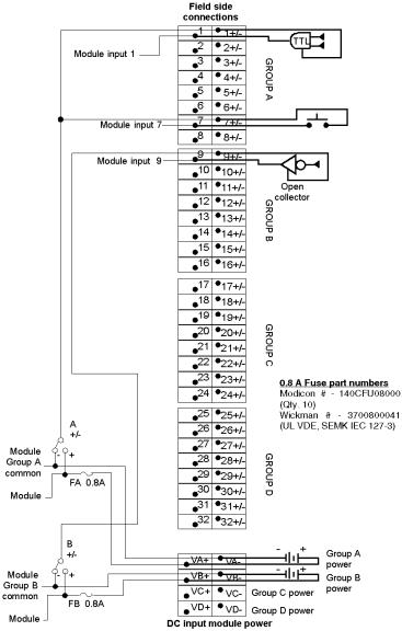
**NOTE:** The terminal block commoning strip, Modicon # 140 CFX 001 10 (Qty. 10), can be used to jumper the power between groups.
