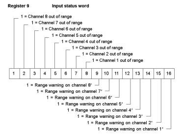
\* A range warning is issued when a channel input is outside the rated input value, as shown in the following table. Warning bits stay on after out of range bits are set. An out-of-range bit is set when a channel input exceeds the rated input value by 2.4%. Out of range bits are also set if inputs drop below 0.5 V (1 ... 5 V mode) or 2.08 mA (4 ... 20 mA mode).
