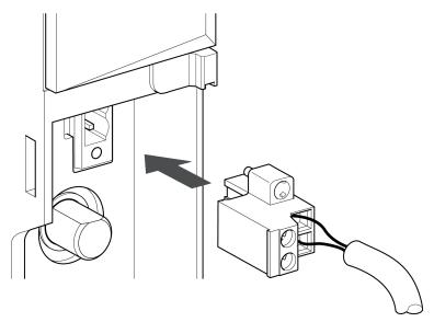
The contacts of the relay are open whenever an error is detected (internal or external), and the Fault LED is ON. In fact the status of the diagnostic relay provides an electric information when the Fault LED status provides a visual status when an error is detected (internal or external).
