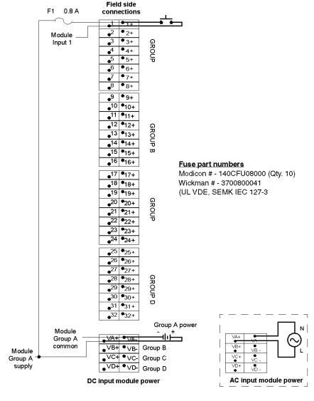
**NOTE:** The terminal block commoning strip, Modicon # 140 CFX 001 10 (Qty. 10) can be used to jumper the power between groups.
