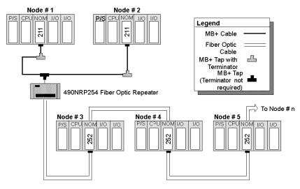
The following figure shows the pure fiber optic network.
