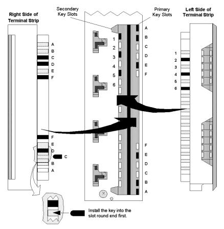
**NOTE:** The primary/secondary keys shown (in black) in this example reflect the recommended coding of a 24 Vdc module in slot 6 to its field wiring terminal strip.
