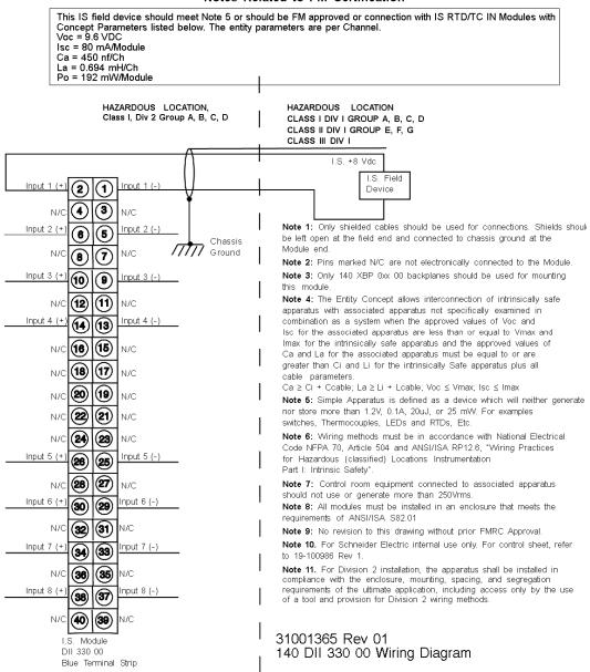
The following is a UL certified wiring diagram for this module.
