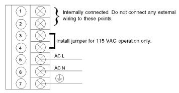
**NOTE:** See *Power and Grounding Considerations for AC and DC Powered Systems, page 787* for power and grounding wiring guidelines and operational information.
