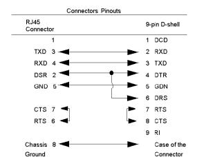
The following figure shows the 9-pin RJ45 connector schematic.
