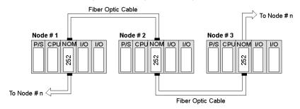
**NOTE:** The distance between nodes on fiber is limited by the maximum allowable power loss from end-to-end (3 km over 62.5 mm fiber). Power loss includes the fiber optic cable attenuation, connector losses at the Fiber Optic Receiver and Transmitter ports, and the system margin of 3 dB.
