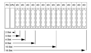
**NOTE:** A maximum of 448 digital I/O points (14, 4x8 digital I/O modules), or a maximum of 48 analog input channels (six 8-channel analog in modules) and 32 analog output channels (eight 4-channel analog out modules) may be serviced in a single local I/O rack.
