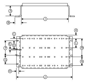
Diameter of the mounting holes: 6.6 mm / 0.26 inches
