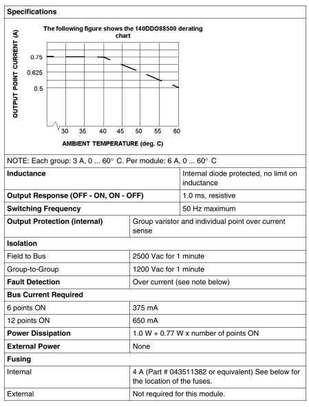
**NOTE:** Each output point is protected by an over current sense circuit. When an over current condition is detected, the point is turned OFF, its LED fault indicator is turned ON, and the appropriate bit is set in the module fault register.
