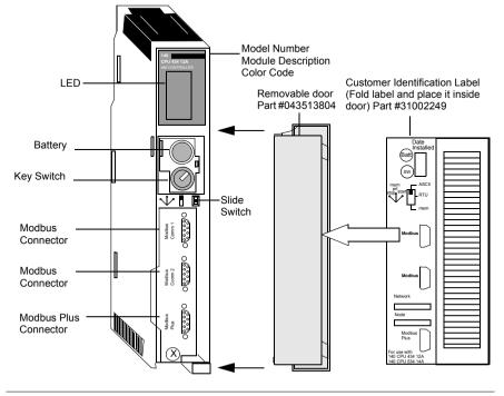
The following illustration shows the 140 CPU 434 12A module and its components. The 140 CPU 534 14A and 140 CPU 534 14B modules have the same components.
