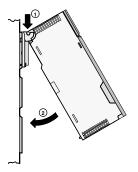
Mounting the Module onto the backplane
