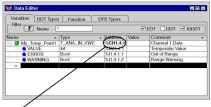
**Note**: Only %CH1.4.1 needs to be entered. The topological addresses related to this channel (%IW.. and %I..) are generated automatically.
