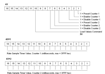
**NOTE:** Zero set into any 4X register or any 4X register pair for 32 bit values means no change.
