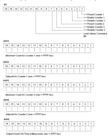
**NOTE:** Zero set into any 4X register means no change.
