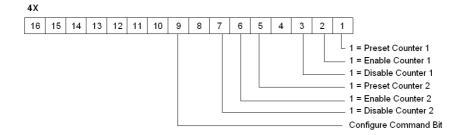
The following figure shows the 4x + 1 output register for command 1 (4X+1).
