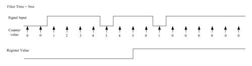
**NOTE:** Debounce time>=1 ms is recommended to ensure enough immunity against electromagnetic disturbances. This means that input signal states >= 2 ms and events up to 250 Hz can be processed. In non-critical electromagnetic environments, the debounce time can be set to 0 to avoid unnecessary filter delays. This means that input signal states >= 1 ms and events up to 500 Hz can be processed.
