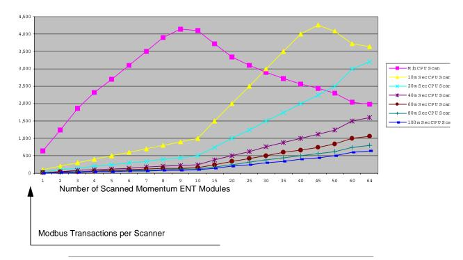
IO Scanner Performance of 140 NOE 771 00 with Quantum 534 CPU Appendix D NOE 771 00 Module I/O Scanner Performance Statistics
