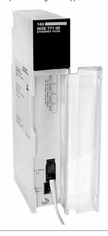
The NOE 771 00 provides real-time peer-to-peer communications, as well as, I/O scanning, and a Modbus/TCP server. The included HTTP services provide maintenance and configuration utilities to the module.
