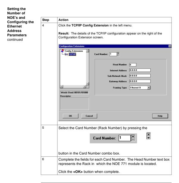
Setting Up the I/O Scanner Using ProWORX NxT At this point you are ready to set up the I/O Scanner. The I/O Scanner provides data transfer between two or more NOE 771 00 and other Modbus or TCP/IP devices. It allows you to simultaneously configure up to 64 connections. To configure the I/O Scanner, follow the steps below to do the following:
