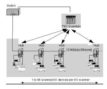
In the above figure, the Quantum NOE is configured to write 1 word from 400050, to the Momentum EIO at IP Address 198.202.137.2, and read 1 word from the EIO into register 400100.
