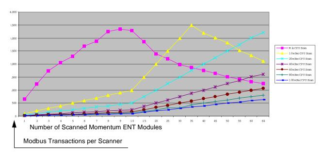
IO Scanner Performance of the 140 NOE 771 00 with the Quantum 113 CPU
