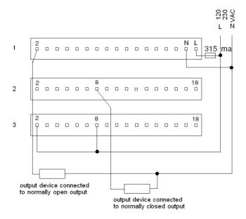
**NOTE:** The 6 relay outputs are individually isolated. This allows for the use of separate power sources for each output if individual isolation is required.
