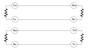
OR: 2 wire the terminals with 120  $\Omega$  only at each end of the network.
