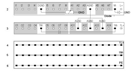
**NOTE:** AGND and DGND are seperated internally inside the module. External digital inputs must be returned the the DGND terminal. External analog circuits must be returned to AGND terminals.
