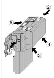
4 Once snaps 1 and 2 have been disengaged, use the screwdriver to release snaps 3 and 4 on the front of the assembly.
