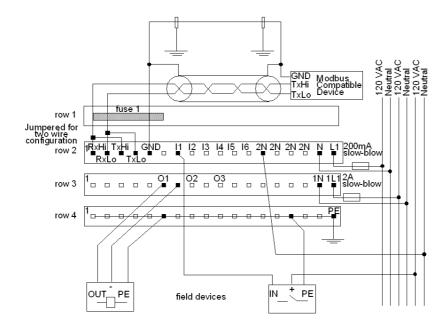
The communication cable should be twisted shielded cable. Tie shield on both ends to earth ground near the associated Modbus equipment.
