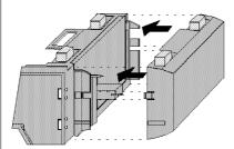
**Result:** The locking tabs on each side of the Processor Adapter slide inside the Option Adapter and out through the locking slot. The 12-pin ATI connectors on the two units are mated to each other in the process.
