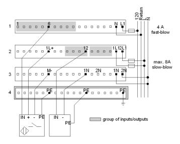
A 1-row busbar is used to provide PE for the 4-wire sensor. No busbar would be required if only 2-and/or 3-wire sensors were used.
