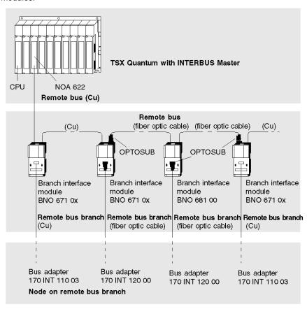
The conversion from copper cable to fiber optic cable is done with OPTOSUB or OPTOSUB PLUS, depending on the module used (see section *Transition from Copper Cable ↔ Fiber Optic Cable, page 14*).
