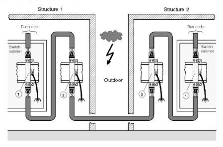
Type and number of the lightning arrestors from Dehn und Söhne GmbH &Co KG for a remote bus cable LiYCY (INTERBUS):
