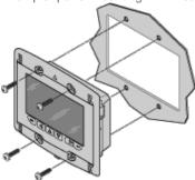
A front frame can be applied to the front of the device (included).
