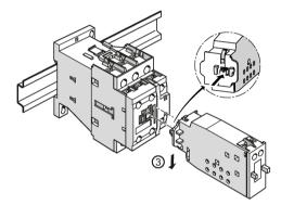
③ Snap the mechanical latch onto the center of the contactor until it engages.
