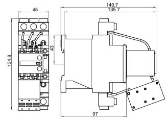
Figure C-38 3RT2628-1A... capacitor contactors (size S0)
