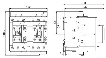
Figure C-55 3RA233.-8XB30-1 reversing contactor assemblies
