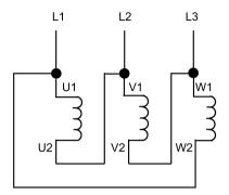
Figure 6-7 Motor phases connected incorrectly results in clockwise rotation
