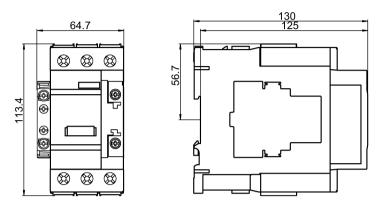
Figure C-41 3RT263.-1.... capacitor contactors (size S2)
