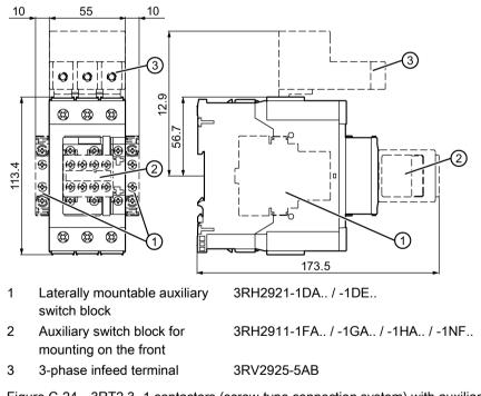
Figure C-24 3RT2.3.-1 contactors (screw-type connection system) with auxiliary switch blocks mounted and 3-phase infeed terminal
