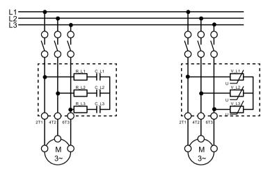
Figure 9-14 EMC suppression module, circuit diagram
