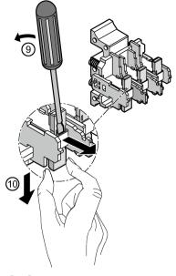
(9)/(10) Use a screwdriver to lever the fixed contacts from the contact piece carrier.
