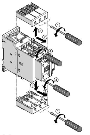
$(\underline{0})/(\underline{0})/$  Use screwdrivers to undo the screws of the detachable terminals.
