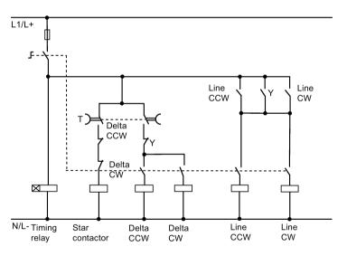
Figure 6-11 Control circuit of the contactor assembly for star-delta (wye-delta) start
