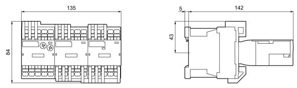
Figure C-59 3RA241.-8X.31-2 contactor assemblies for star-delta (wye-delta) start (size S00, spring-loaded connection system)
