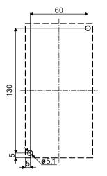
Figure C-44 Drilling diagram for 3RT264.-1.... capacitor contactors (size S3)
