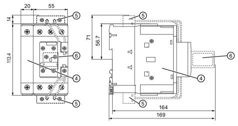
4 4-pole contactor for switching resistive loads 3RT233.-1 4-pole pole-changing contactor for changing 3RT253.-1 the polarity of hoisting gear motors (2 NO contacts and 2 NC contacts)
