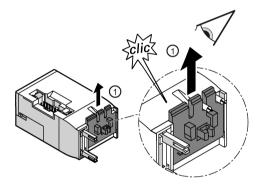
① Check that the locking slide is engaged in the topmost position.
