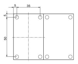
Figure C-46 Drilling diagram for the 3RA231.-8X.3.-1 reversing contactor assemblies (size S00, screw-type connection system)
