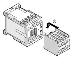
① Push the auxiliary switch, which can be mounted on the front, into the location hole on the contactor. Pull it down until it engages.
