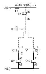
11.6 Contactor assemblies for star-delta (wye-delta) start (S00 / S0 / S2 / S3)
