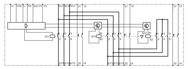
Figure 11-8 S0, S2 and S3 contactor assembly for star-delta (wye-delta) start, with mounted function modules for IO-Link
