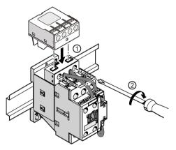
① Attach the coupling link to the coil terminal module using the two integrated mounting pins.
