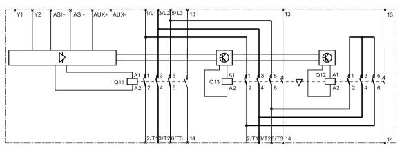
Figure 11-5 S00 contactor assemblies for star-delta (wye-delta) start, with mounted function modules for AS-Interface
