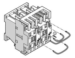
③ To connect the control current paths, strip the conductors and push them into the contactor terminals.
