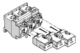
(4) Attach the basic module/coupling module to the contactor from the front. To do this, insert the contacts into the openings on the contactor.
