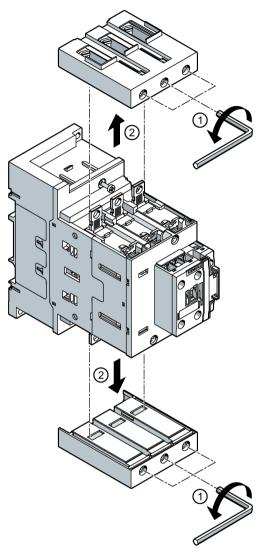
① Use an Allen key to undo the screws of the detachable terminals.
