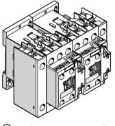
6 Connect contactors Q11 and Q12 together.
