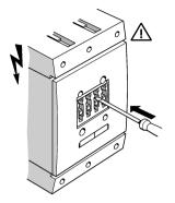
With 3RT10/14 air-break contactors, the lateral auxiliary contacts can be operated for test purposes by pressing the auxiliary switch receptacle / switch position indicator on the front. By doing this the main contacts would also touch, without resulting in contact resilience.
