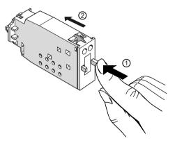
①/② When snapping on, the switch position indicator's rod must be unlocked. Unlock the rod by pressing on the switch position indicator and pushing the rod into the mechanical latch as far as it will go.
