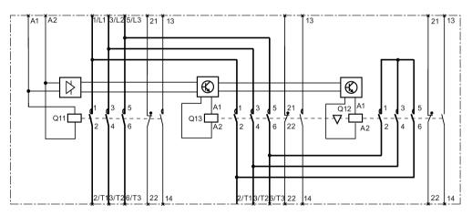
Figure 11-4 S0, S2 and S3 contactor assemblies for star-delta (wye-delta) start, with 3RA28 function modules for star-delta (wye-delta) start
