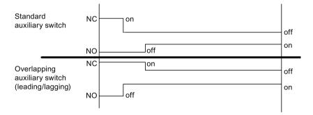
Figure 9-5 Travel diagrams for auxiliary switches (sizes S00 and S0)
