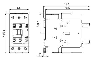
Figure C-26 3RT2.3.-3 contactor (spring-loaded connection system)
