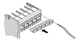
Figure 9-21 Insulating stop on spring-loaded connection
