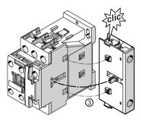
③ Attach the 4th pole to the other side of the same contactor by hooking it into the openings on the contactor and snapping the pole onto the contactor.
