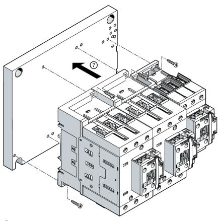
Mount the contactors on the mounting plate.
