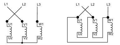
Figure 6-9 Correct connection of motor phases for counterclockwise motor rotation
