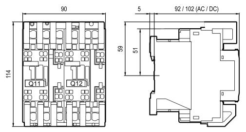
Figure C-52 3RA232.-8XB30-2 reversing contactor assemblies (size S0, spring-loaded connection system)
