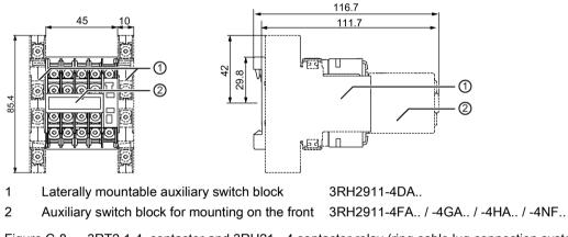
Figure C-8 3RT2.1-4. contactor and 3RH21..-4 contactor relay (ring cable lug connection system) with auxiliary switch blocks mounted
