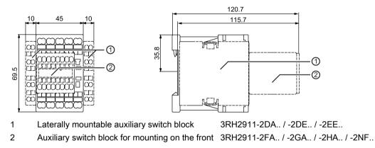
Figure C-5 3RT2.1.-2 contactor and 3RH21..-2 contactor relay (spring-loaded connection system) with auxiliary switch blocks mounted
