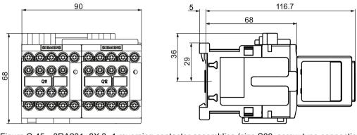
Figure C-45 3RA231.-8X.3.-1 reversing contactor assemblies (size S00, screw-type connection system)
