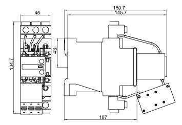
Figure C-39 3RT2628-1B... capacitor contactors (size S0)
