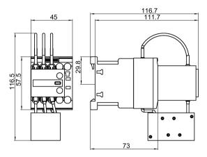
Figure C-34 3RT261.-1.... capacitor contactors (size S00)
