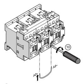
1 Screw the conductors tight with a screwdriver.
