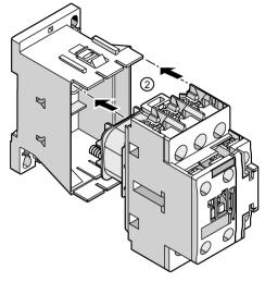
② Push the two halves of the contactor apart.
