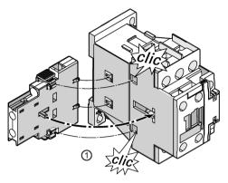
① Attach the lateral auxiliary switch to the contactor and snap it on.
