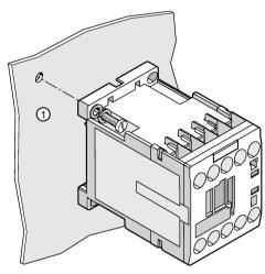
Using two M4 screws, plain washers, and spring washers, screw the contactor tight into the designated drill holes diagonally. Maximum tightening torque 1.2 to 1.6 Nm 7.2 Mounting
