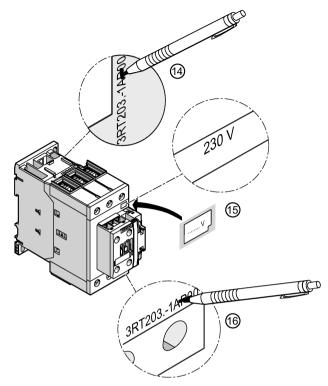
(1)/(5)/(6) To label the coil voltage of the newly inserted operating mechanism, cover the control supply voltage specification with the labels supplied. Thoroughly cross out the article number.
