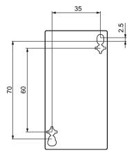
Figure C-40 Drilling diagram for 3RT262.-1.... capacitor contactors (size S0)
