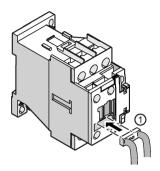
① Snap the LED display indicator module into the corresponding location hole provided on the front of the contactor.
