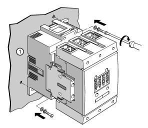
① Screw the contactor tight diagonally into the openings provided using two screws, plain washers and spring washers.
