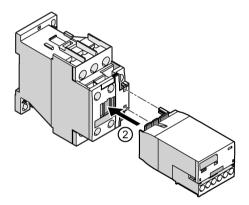
2 Attach the coupling module to the coil terminal module using the integrated mounting pins at the front.
