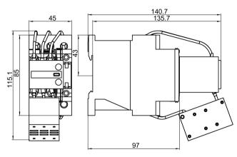
Figure C-36 3RT2625-1A... capacitor contactors (size S0)
