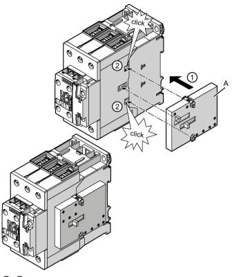
①/② Insert the mechanical interlock (3RA2934-2B) into the opening on the right-hand side of the contactor.
