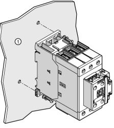
Screw the contactor tight diagonally into the openings provided using two M4 screws, plain washers and spring washers.
