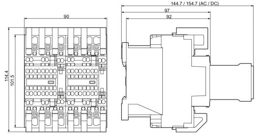
Figure C-53 3RA232.-8XD3.-2 reversing contactor assemblies (size S0, spring-loaded connection system)
