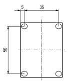
Figure C-12 Drilling plan for contactors and contactor relays with screw-type connections and ring cable lug connections (size S00)
