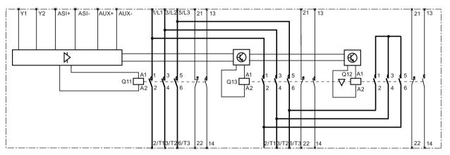
Figure 11-6 S0, S2 and S3 contactor assemblies for star-delta (wye-delta) start, with mounted function modules for AS-Interface
