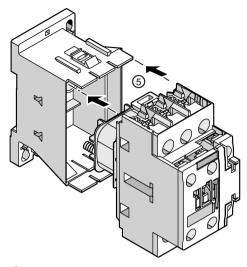
(5) Reattach the front part of the contactor onto the rear half until the retaining clips engage.
