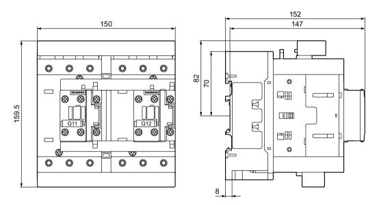
C.10.4.2 Drilling diagram for 3RA234.-8X.30-1 reversing contactor assemblies (size S3)
