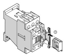
① Open the cover on the front panel of the contactor and push the surge suppressor into the opening until it engages.
