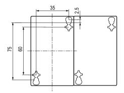
Figure C-54 Drilling diagram for 3RA232.-8XB30-2 and 3RA232.-8XD3.-2 reversing contactor assemblies (size S0, spring-loaded connection system)
