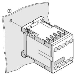
① Using two M4 screws (maximum tightening torque 1.2 to 1.6 Nm), plain washers, and spring washers, screw the OFF-delay device tight into the designated drill holes diagonally.
