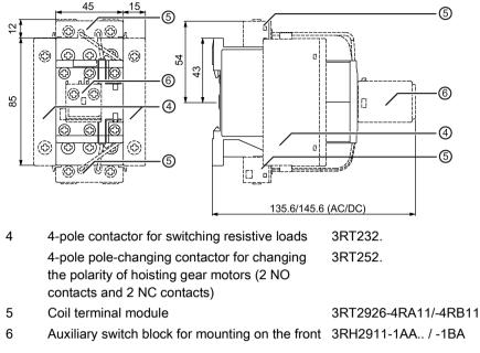
Figure C-16 3RT2.2.-1 contactors (screw-type connection system) with accessories mounted
