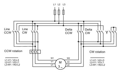
Figure 6-10 Main circuit of the contactor assembly for star-delta (wye-delta) start
