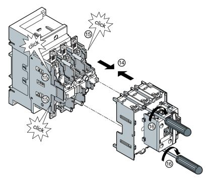
Slide the front part of the contactor back onto the rear half until the retaining clips engage.
