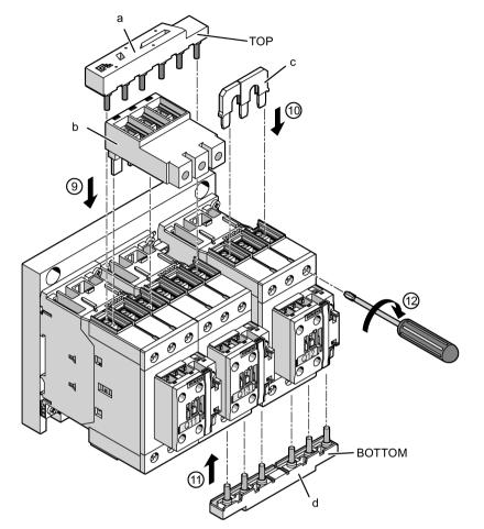
(9) Attach the wiring module for connecting the main current paths to contactors Q11 and Q13 from above (a).
