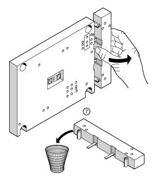
When using the mounting plate (for S2 3RA2932-2F; for S3 3RA2942-2F), you must remove its side section.
