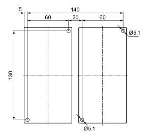
C.11 3RA24 contactor assemblies for star-delta (wye-delta) start
