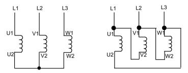
Figure 6-5 Correct connection of motor phases for clockwise rotation
