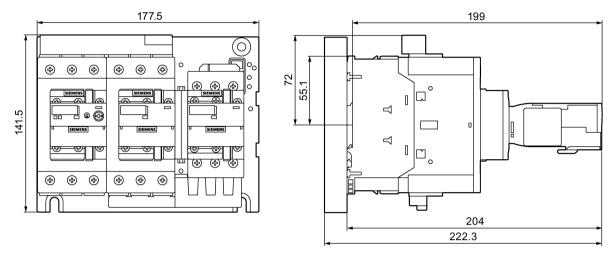
3RA243.-8X.32-1 contactor assemblies for star-delta (wye-delta) start (size S2)
