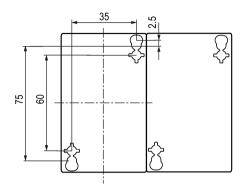
Figure C-51 Drilling diagram for 3RA232.-8XB30-1 and 3RA232.-8XD3.-1 reversing contactor assemblies (size S0, screw-type connection system)
