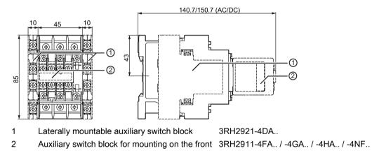
Figure C-21 3RT2.2.4 contactors (ring cable lug connection system) with auxiliary switch blocks mounted
