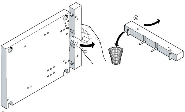
6 When using the mounting plate (for S2 3RA2932-2F; for S3 3RA2942-2F), you must remove its side section. (Note: The side section is required when mounting the 3RP25 or 3RP15 timing relay.)
