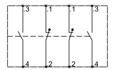
Auxiliary switch block, for mounting on the front, 4-pole, 2 NO contacts, 2 NC contacts
