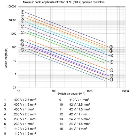
Figure 6-12 Graphical representation, switch-on
