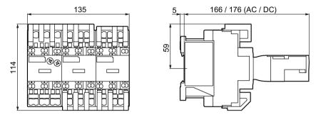
Figure C-63 3RA242.-8X.3.-2 contactor assemblies for star-delta (wye-delta) start (size S0, springloaded connection system)
