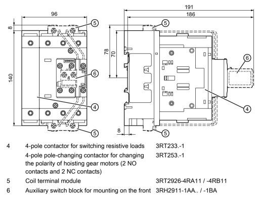
Figure C-31 3RT2.4.-1 contactors (screw-type connection system) with attached accessories
