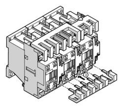
③ Attach the wiring modules for connecting the main current paths to contactors Q13 and Q12 from below.
