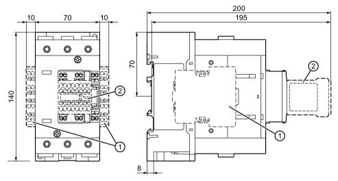
1 Laterally mountable auxiliary 3RH2921-1DA.. / -1DE.. switch block
