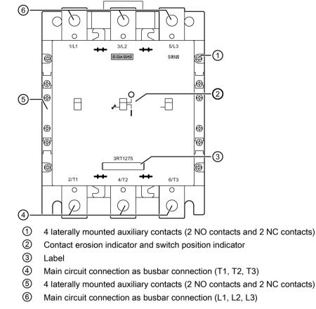
Figure 4-9 3RT1275-6LA06 vacuum contactor, size S12, overview
