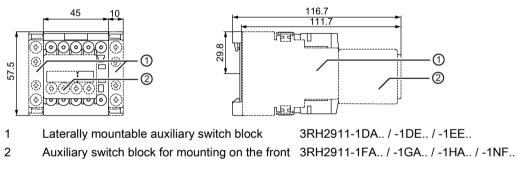
Figure C-2 3RT2.1.-1 contactor and 3RH21..-1 contactor relays (screw-type connection system) with auxiliary switch blocks mounted
