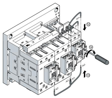
To connect the control current paths, push the conductors into the contactor terminals. To connect the coil contacts, push the conductors into the contactor terminals.
