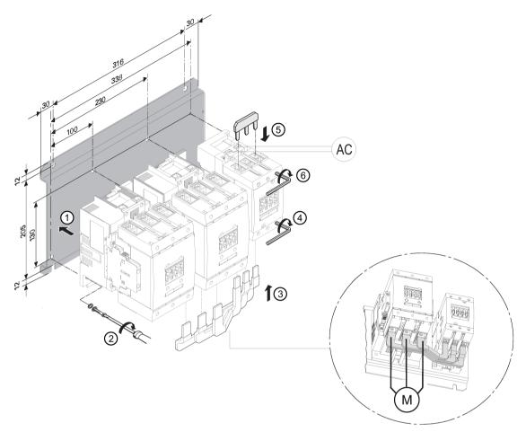
Mounting the contactor assembly for star-delta (wye-delta) start - size S6-S6-S3 (AC)
