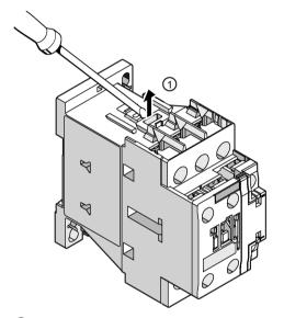
① Use a screwdriver to lift up the retaining clips between the rear and front halves of the contactor.
