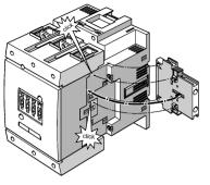
① Attach the lateral auxiliary switch to the contactor and snap it on.
