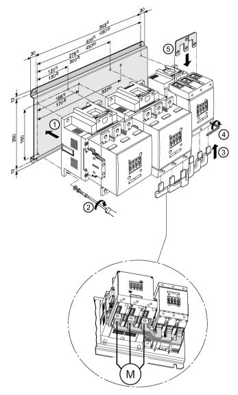
Mounting the contactor assembly for star-delta (wye-delta) start - size S10(S12)-S10(S12)-S6(S10)
