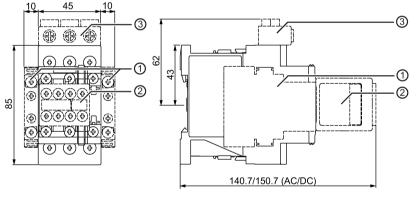
1 Laterally mountable auxiliary switch block 3RH2921-1DA.. / -1DE..
