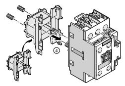
(a) Insert the new solenoid coil. In doing so, make sure that the springs between the solenoid coil and the front half of the contactor are properly located on the support.
