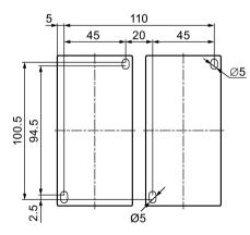
Figure C-56 Drilling diagram for 3RA233.-8XB30-1 reversing contactor assemblies
