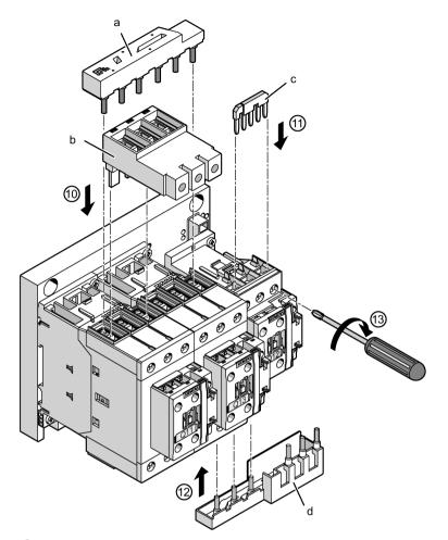
① Attach the wiring module for connecting the main current paths to contactors Q11 and Q13 from above (a).
