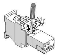
③ Use a screwdriver to press down the cover of the coupling module until it engages.
