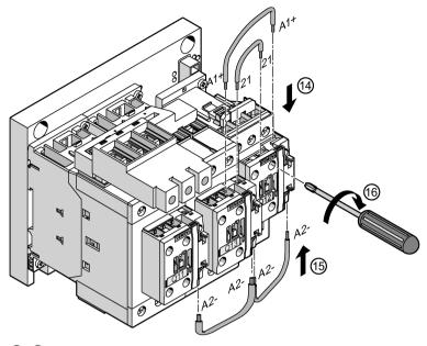
(4)/(5) To connect the control current paths, push the conductors into the contactor terminals. To connect the coil contacts, push the conductors into the contactor terminals.
