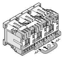
(4) Insert the screwdriver into the rectangular operating slot as far as it will go. The screwdriver blade keeps the spring-loaded terminal open automatically. Insert the conductor into the oval connection slot and then pull it back out again.
