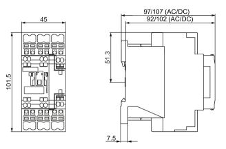
Figure C-17 3RT2.2.-2 and 3RT202.- ..... -0LA2 contactors (spring-loaded connection system)
