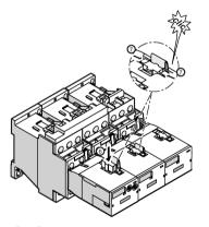
(6)/⑦ Insert the coded module connector into the slot in the correct position from above until the module connector engages in the locking mechanism.
