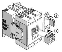
① Push the auxiliary switch, which can be mounted on the front, into the location hole on the contactor. Pull it down until it engages.
