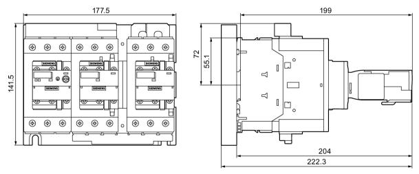
Figure C-66 3RA2437-8X.32-1 contactor assemblies for star-delta (wye-delta) start (S2-S2-S2) on mounting plate
