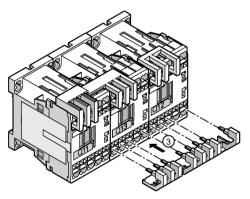
③ Attach the wiring module for connecting the main current paths to contactors Q13 and Q12 from below.
