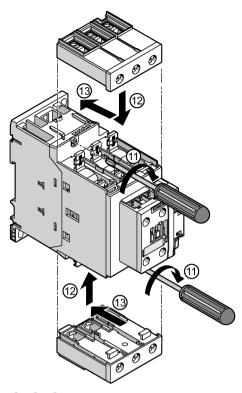
(1)/(2)/(3) Screw the two contactor halves together (1.1 - 1.3 Nm).
