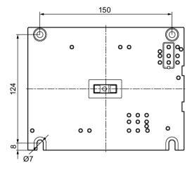
Figure C-67 Drilling diagram for the mounting plate for 3RA243.-8X.32-1 contactor assemblies for star-delta (wye-delta) start
