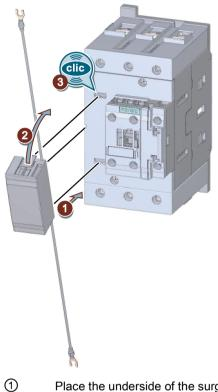
Place the underside of the surge suppressor onto the contactor.
