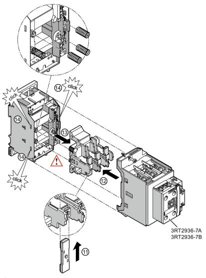
1) 12/13/14 Slide the new movable contact into the contact piece support.
