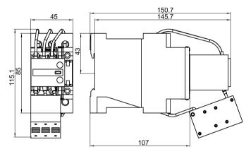
Figure C-37 3RT2625-1B... capacitor contactors (size S0)
