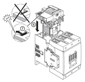
(6) / (7) When re-installing, ensure that the interlock clearly engages again:
