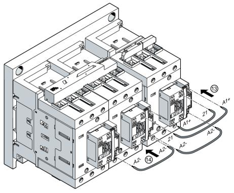
③ To connect the control current paths, push the conductor (e) into the contactor terminals. To connect the coil contacts, push the conductors (e) into the contactor terminals.
