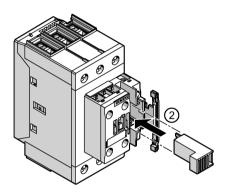
② Attach the control kit to the contactor from the front. Press the control kit down until it engages.
