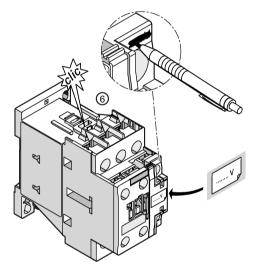
Write the coil voltage of the newly inserted operating mechanism onto the label supplied and stick the label onto the front panel of the contactor, as shown in the diagram.
