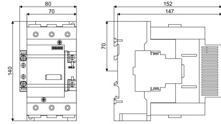
Figure C-43 3RT264.-1...capacitor contactors (size S3)
