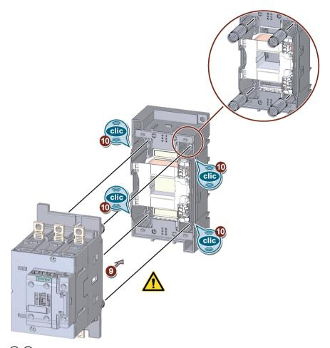
(9)(10) Slide the front part of the contactor (upper part of the enclosure) back onto the rear half (lower part of the enclosure) until the retaining clips engage.
