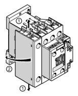
(1)/(2) Remove the 4th pole from one of the two contactors by releasing the snap hooks.
