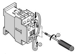
② Thread the cables into coil terminals A1 and A2 of the contactor.
