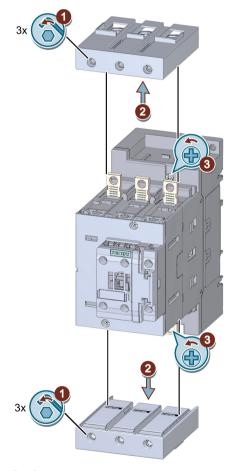
①/② Undo the screws of the detachable terminals. Pull the terminals forward slightly and remove the terminals.
