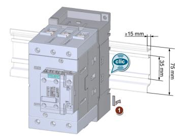
1 Position the device on the top edge of the mounting rail and press it down until it snaps onto the bottom edge of the rail.
