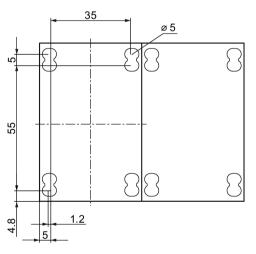
Figure C-48 Drilling diagram of the 3RA231.-8X.3.-2 reversing contactor assemblies (size S00, spring-loaded connection system)
