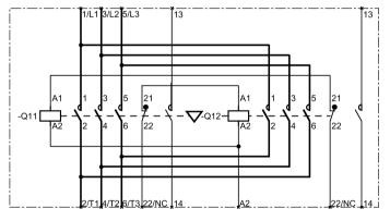
Figure 11-2 Reversing contactor assemblies S0, S2 and S3
