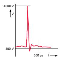
Figure 9-15 Counter-source voltage without RC circuit
