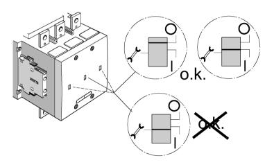
Figure 7-4 Contact erosion indicator and switch position indicator
