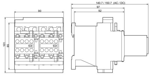
Figure C-50 3RA232.-8XD3.-1 reversing contactor assemblies (size S0, screw-type connection system)
