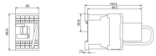
Figure C-11 3RH201. and 3RH21.. contactor relays with extended operating range (spring-loaded connection system)
