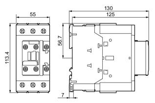
Figure C-23 3RT2.3.-1 contactor (screw-type connection system)
