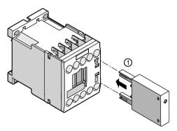
① Attach the surge suppressor onto the front of the contactor. Codes help you to identify which is the correct way up when inserting the device.
