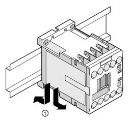
① Position the device on the top edge of the mounting rail and press it down until it snaps onto the bottom edge of the rail.
