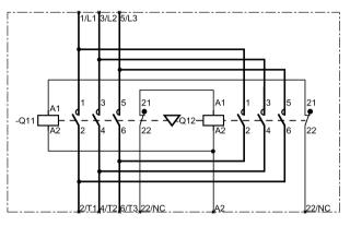
Figure 11-1 Reversing contactor assembly S00
