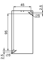
Figure C-42 Drilling diagram for 3RT263.-1.... capacitor contactors (size S2)
