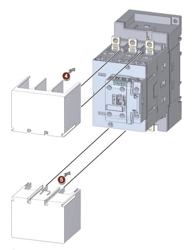
④/ Slide the terminal cover for cable lug connection and busbar connection into the guide tabs
