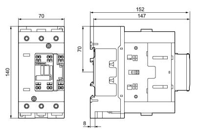
Figure C-32 3RT204.-3 (spring-loaded connection system)
