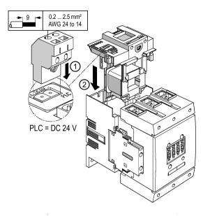
The control signal is connected via a 2-pin plug-in connection on the front side of the withdrawable coil (the spring-loaded connector is included in the scope of supply). The connector is labeled with the polarity.
