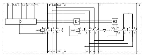
Figure 11-7 S00 contactor assembly for star-delta (wye-delta) start, with mounted function modules for IO-Link
