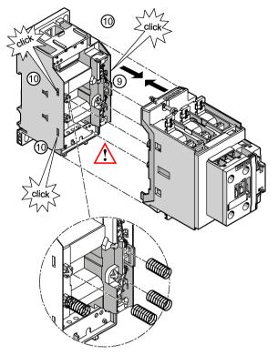
(9)/(10) Slide the front part of the contactor back onto the rear half until the retaining clips engage. In doing so, make sure that the springs between the solenoid coil and the front half of the contactor are properly located on the support.
