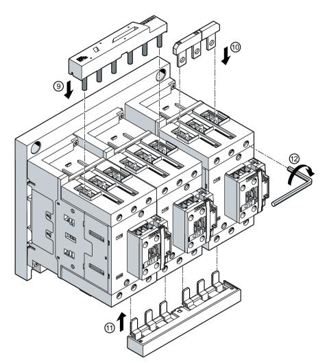
(9) Attach the wiring module for connecting the main current paths to contactors Q11 and Q13 from above.
