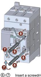
Insert a screwdriver into the spring-loaded connections and release them. Insert the cables into the spring-loaded terminals.
