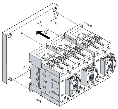
Mount the contactors on the mounting plate.
