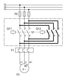
Figure 6-3 Main circuit of the reversing contactor assembly
