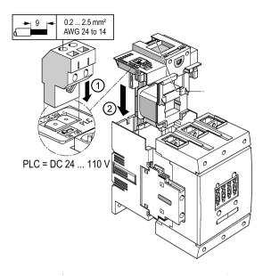
The control signal is connected via a 2-pin plug-in connection on the front side of the withdrawable coil (the spring-loaded connector is included in the scope of supply). The connector is labeled with the polarity.
