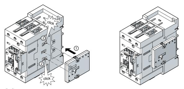
(1)(2) Insert the mechanical interlock (3RA2934-2B) into the opening on the right-hand side of the contactor.
