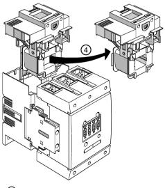
④ Remove the withdrawable coil.
