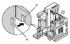
Insert the pins of the link module into the contactor's terminal openings from above until they are securely in position. Make sure that the wedge (a) engages in the groove (b) provided on the contactor for this purpose.
