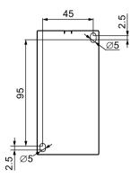
Figure C-28 Drilling plan for 3RT2.3. contactors (size S2)
