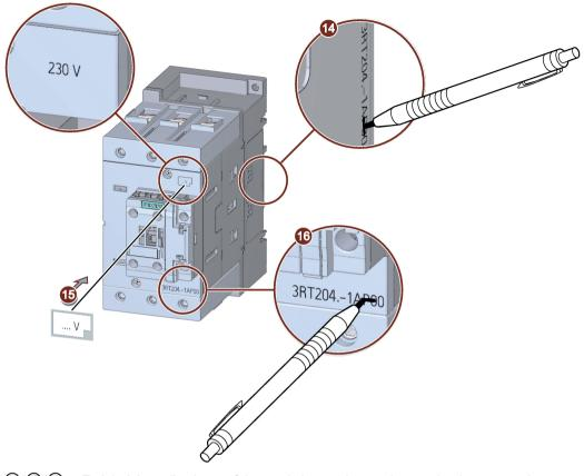
(④)(⑤)(⑥ To label the coil voltage of the newly inserted operating mechanism, cover the control supply voltage specification with the labels supplied. Thoroughly cross out the article number.
