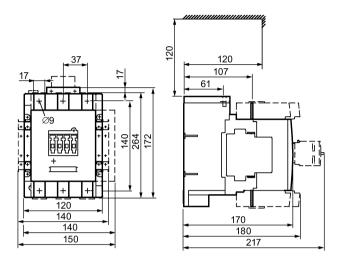
Drilling diagram for 3RT1.5. contactors
