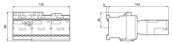
Figure C-57 3RA241.-8X.31-1 contactor assemblies for star-delta (wye-delta) start (size S00, screw-type connection system)
