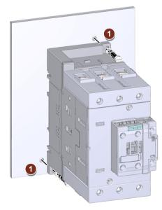
Screw the contactor tight diagonally into the openings provided using two M4 screws, plain washers and spring washers.
