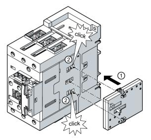
①/② Insert the mechanical interlock (3RA2934-2B) into the opening on the right-hand side of contactor Q11.
