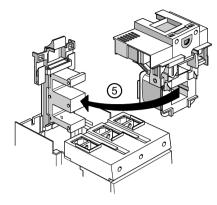
5 Insert a new withdrawable coil.
