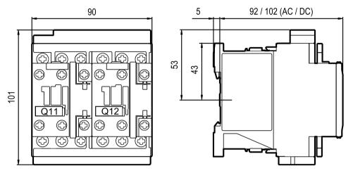
Figure C-49 3RA232.-8XB30-1 reversing contactor assemblies (size S0, screw-type connection system)
