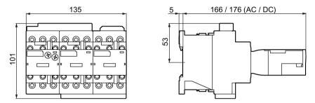
Figure C-61 3RA242.-8X.3.-1 contactor assemblies for star-delta (wye-delta) start (size S0, screwtype connection system)
