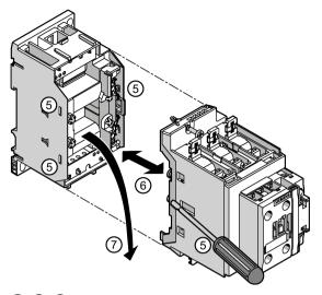
(5)/(6)/(7) Push the two halves of the contactor apart. Note the lateral latching here. Take the solenoid coil out of the rear half of the contactor.
