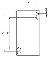
Figure C-22 Drilling plan for 3RT2.2. contactors (size S0)
