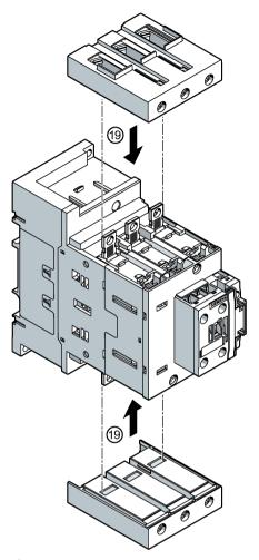
(9) Place the terminals on the device. Make sure the terminals engage.
