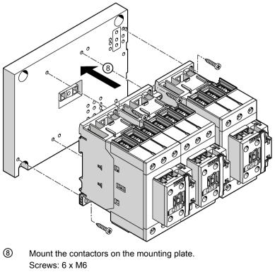
Tightening torque: 1.6 Nm
