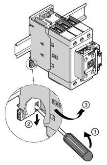
1/2 3 To disassemble, press the locking device down with a screwdriver.
