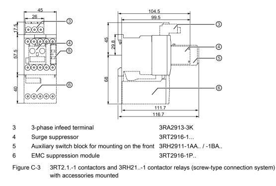
C.2 3RT2.1 contactors and 3RH2 contactor relays (size S00)
