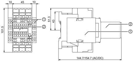
1 Laterally mountable auxiliary switch block 3RH2921-2DA.. / -2DE..
