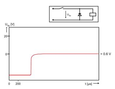
Figure 9-11 RC circuit with diode (DC operation)
