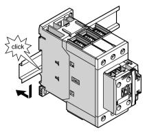
① Position the device on the top edge of the mounting rail and press it down until it snaps onto the bottom edge of the rail.
