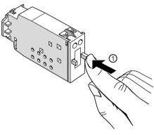
① Release the mechanical latch.
