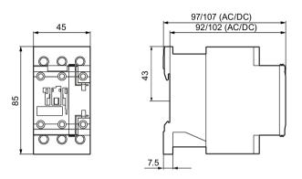
Figure C-14 3RT2.2.-1 contactors (screw-type connection system)
