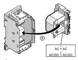
(8) Insert the new solenoid coil.
