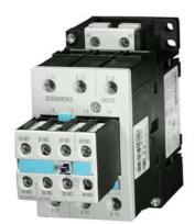
Power contactor, AC-3 50 A, 22 kW / 400 V 230 V AC, 50 Hz, 2 NO + 2 NC, 3-pole, Size S2, Screw terminal !!! Phased-out product !!! Successor is SIRIUS 3RT2 Preferred successor type is >>3RT2036-1AP04<<
