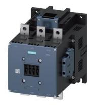
power contactor AC-1 690 A / 690 V / 40  $^{\circ}$ C 3-pole, Uc: 220-240 V AC(50-60 Hz) / DC drive: conventional auxiliary contacts 2 NO + 2 NC main circuit: busbar control and auxiliary circuit: screw terminal
