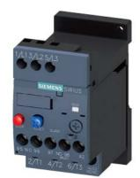
Overload relay 1.8...2.5 A Thermal For motor protection Size S00, Class 10 Standalone installation Main circuit: Screw Auxiliary circuit: Screw Manual-Automatic-Reset
