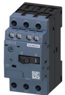
Circuit breaker size S00 for motor protection, CLASS 10 A-release 9...12 A N-release 156 A 1 NO+1 NC transverse Screw terminal Standard switching capacity
