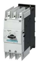
Circuit breaker size S3 for system protection with approval circuit breaker UL 489, CSA C22.2 No.5-02 A-release 15 A Short-circuit release 225 A Screw terminal Standard switching capacity !!! Phased-out product !!! Successor is SIRIUS 3RV2 Preferred successor type is >>3RV2742-5BD10<<
