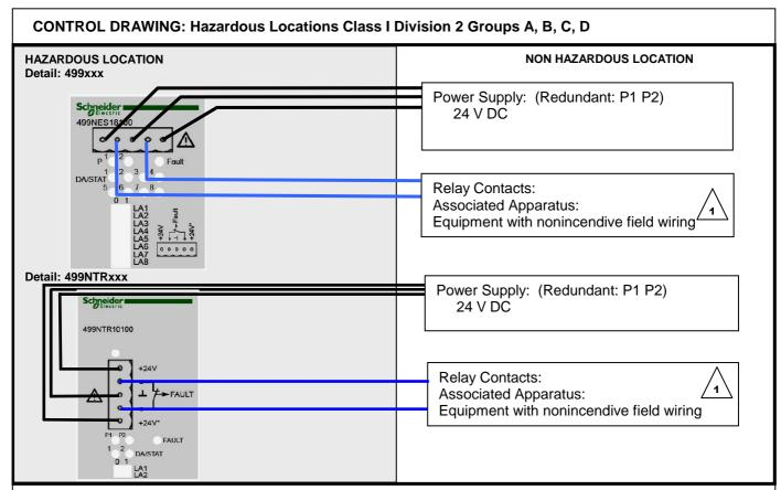
The Use in Hazardous Locations is only allowed for ConneXium Switches and ConneXium Transceiver model No´s which are individually labelled "FOR USE IN CLASS I, DIVISION 2 HAZARDOUS LOCATIONS"
