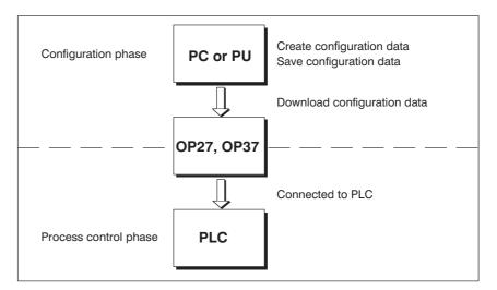
Figure 1-1 Configuration and process control phase
