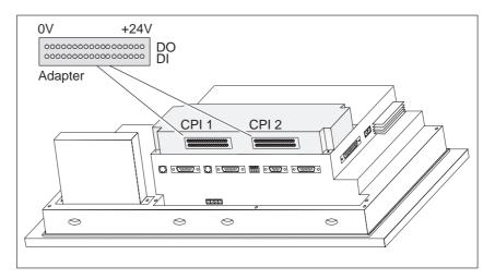
Figure 18-11 Location of connection elements on large module housing (example: OP37)
