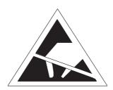
**ESDs** may be destroyed by voltages and energies well below the perception threshold of persons. Voltages of this kind occur as soon as a device or an assembly is touched by a person who is not electrostatically discharged . Devices exposed to such overvoltages cannot immediately be detected as defective in the majority of cases since faulty behavior may occur only after a long period of operation.
