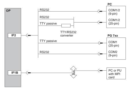
Figure 13-2 Connection configuration diagram for configuration computer
