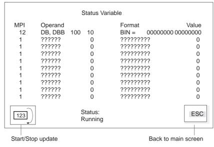
Figure 10-1 Status Variable standard screen (example: OP37 with SIMATIC S7)
