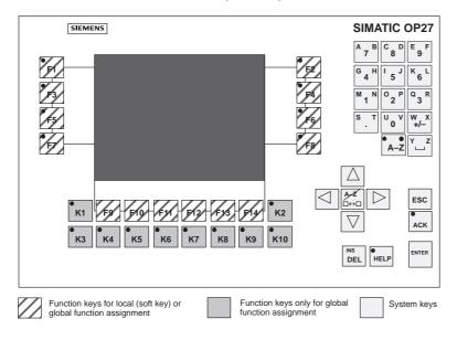
Figure 3-2 Arrangement of keypads on the OP27
