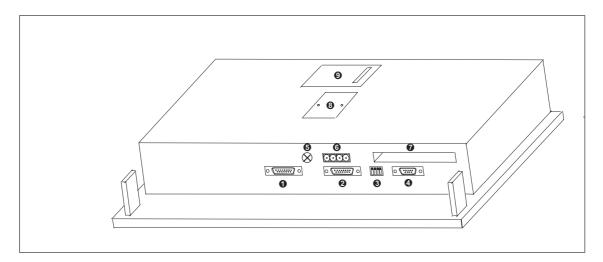
Figure 16-2 OP27: Arrangement of connections
