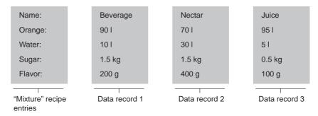
All data records are stored in the OP. Only the currently active data record is stored on the PLC. This saves memory space on the PLC.
