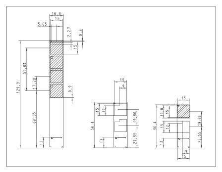
Figure 16-5 Dimensions of labeling strips for OP27
