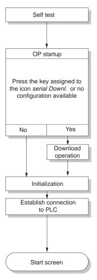
After the power supply has been switched on, the OP performs a self test. In the test, it checks the operability of the most important OP components and displays the test results. The test results are then deleted.
