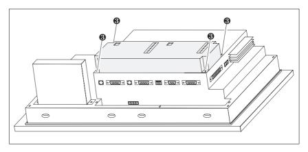
Figure 18-6 Securing the direct key module to the OP (example OP37)
