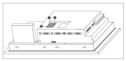
Figure 18-4 Removing the cover (example OP37)
