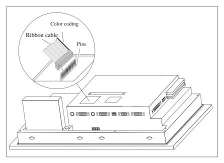
Figure 18-5 Connecting the plug of the direct key module (example OP37)
