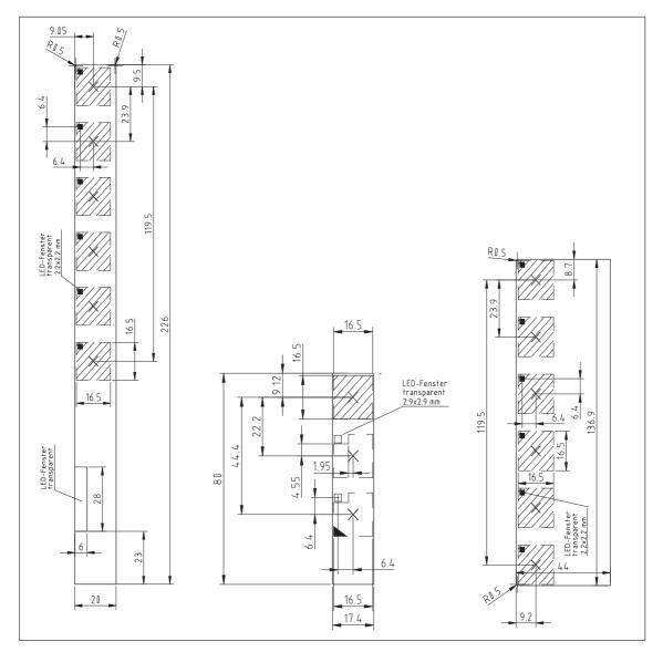
Figure 17-6 Dimensions of Labeling Strips for OP37
