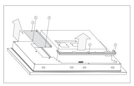
Figure 17-3 Undo screws
