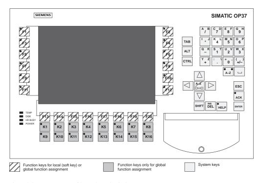
Figure 3-3 Arrangement of keypads on the OP37
