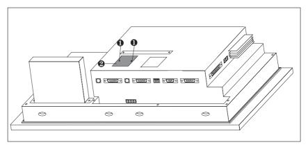
Figure 18-8 Removing the cover (example OP37)
