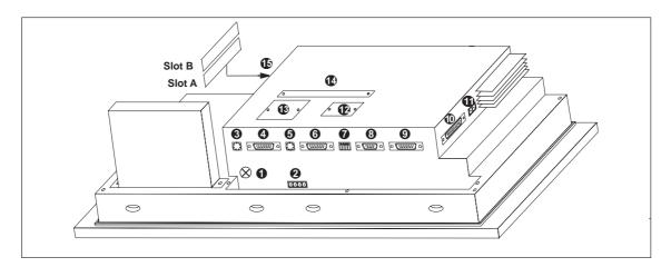
Figure 17-2 OP37: Arrangement of connections
