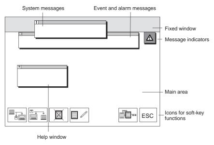
Figure 3-1 Screen partitioning on the OP (example OP37)
