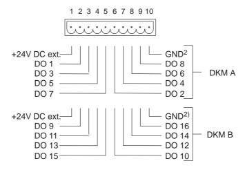
2) Optocouplers electrically isolate the digital outputs from the OP.
