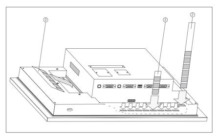
Figure 17-4 Inserting Labeling Strips
