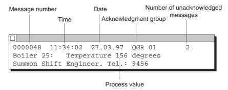
Figure 6-1 Alarm message window (example)
