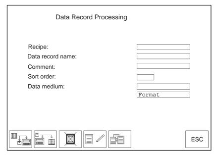
Figure 8-2 Input fields and soft keys in the standard screen *Data Record Processing* (example: OP37)
