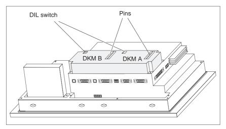
Figure 18-7 Location of connection and adjustment elements on large module housing (example OP37)
