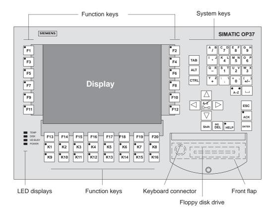
Figure 17-1 Operating and Display Element Arrangement
