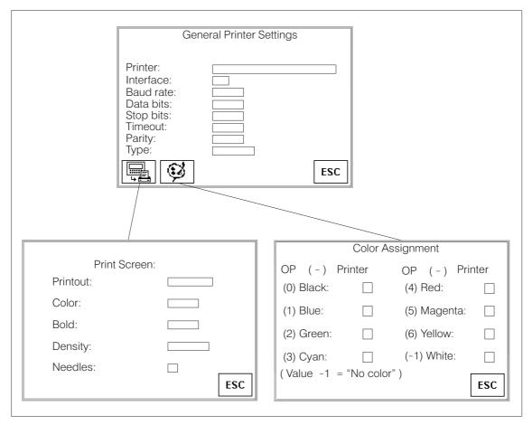
Figure 7-1 Standard screens for printer settings (example OP27)
