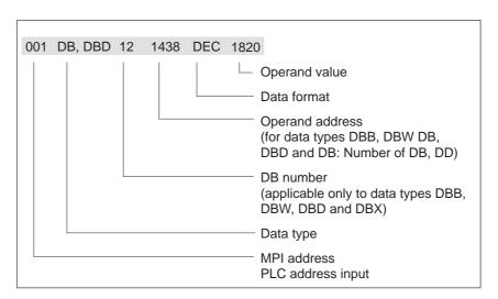
Figure 10-3 Display of PLC operands for the SIMATIC S7
