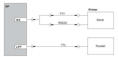
Figure 13-4 Connection configuration diagram for printers
