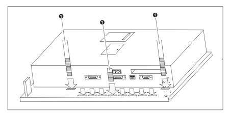
Figure 16-3 Inserting labeling strips
