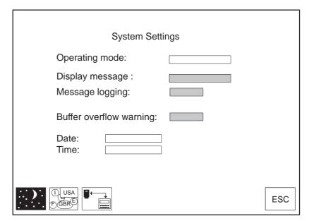
Figure 6-7 System Settings standard screen (example OP37)
