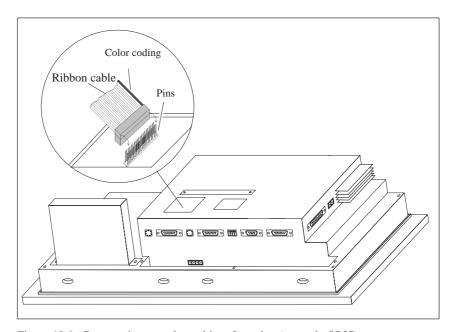
Figure 18-9 Connect the control panel interface plug (example OP37)
