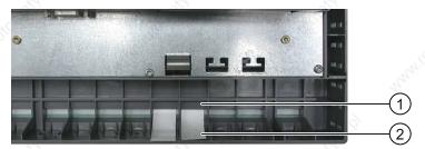
6. Slide the labeling strips into the slot up to the stop.
