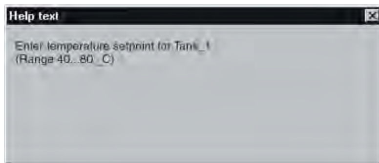
Figure 9-4 Operator note for an I/O field (Example)
