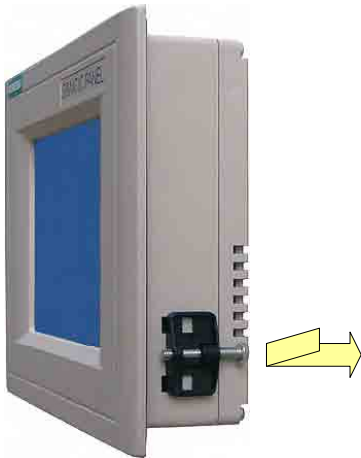
Figure 4-1 Inserting the spring terminals in the TP 170micro, TP 170A and TP 170B
