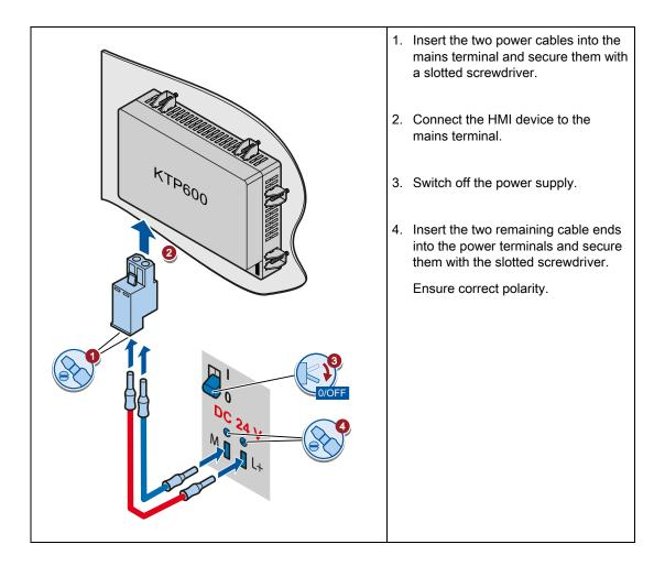
Mounting and connecting 3.3 Connecting the HMI device
