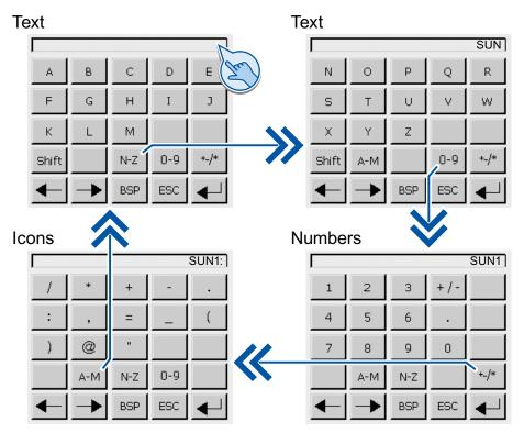
The screen keyboard appears on the HMI device touch screen when you touch an operating element that requires input.
