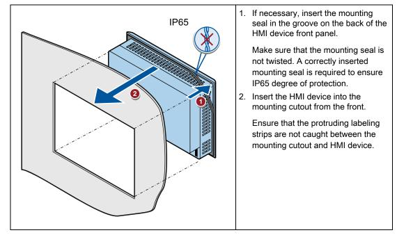
3.2 Mounting the HMI device
