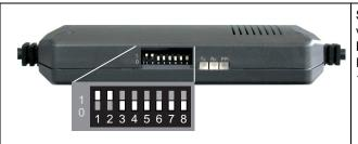
Set the DIP switches 1 to 3 to the same value as in WinCC flexible or WinCC. DIP switches 4 to 8 must be set to "0". In the figure, the bit rate is set to 115.2 kbps.
