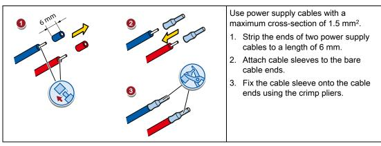
3.3 Connecting the HMI device
