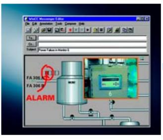
•WinCC/Messenger supports both operator-controlled and automatic transmission of messages from WinCC with important information on the process. These messages can be received by any computer with e-mail access
