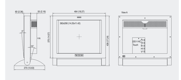
SCD 1815-I, dimensioned drawing, dimensions in mm (inch)
