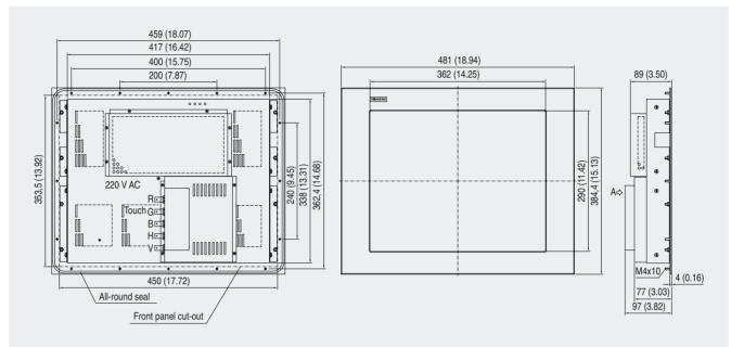
SCD 1815-E, dimensioned drawing, dimensions in mm (inch)
