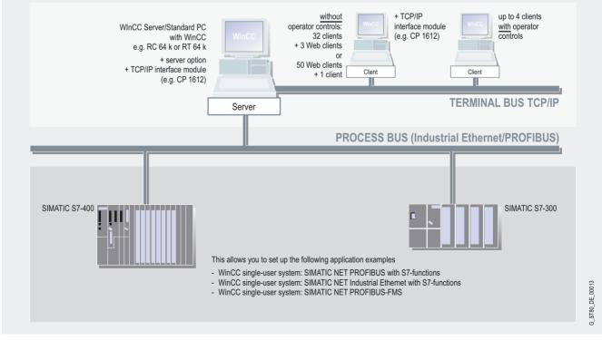
WinCC multi-user system with operator-accessible server (for WinCC V6)
