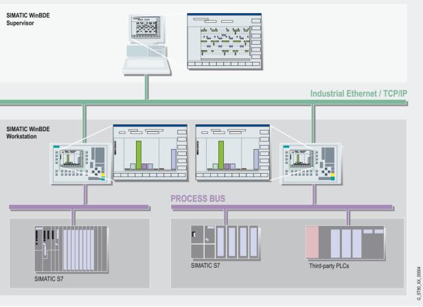
•SIMATIC WinBDE is the machine data management software for acquisition, evaluation and analysis of machine data
