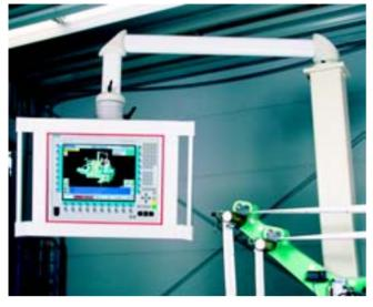
SIMATIC Panel PCs are suitable for use in standard control cabinets, control panels and switchboards. Typical fields of application can be found in both manufacturing automation and process automation.
