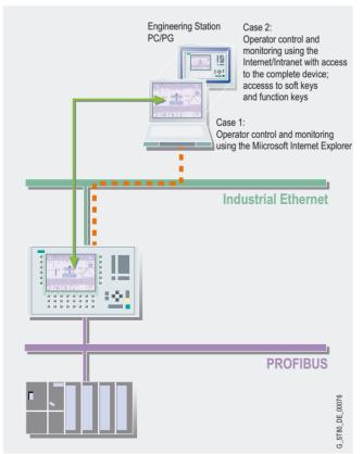
Remote operator control and monitoring of SIMATIC HMI systems via Industrial Ethernet or intranet/Internet
