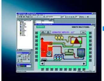
Standard configuration software for SIMATIC Operator Panels and for the HMI part of the SIMATIC C7
