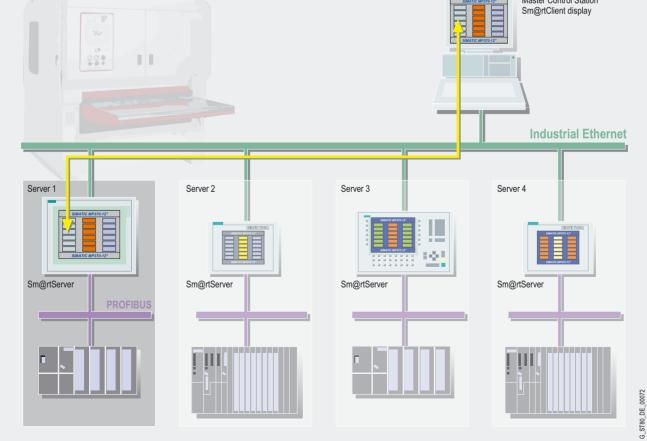
Application of Sm@rtClient display: operator control and monitoring of HMI systems used at machine level from a central station
