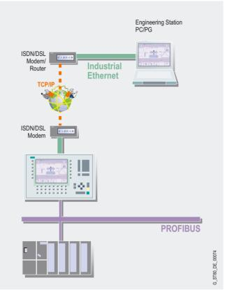
Remote operator control and monitoring of SIMATIC HMI systems via Industrial Ethernet or intranet/Internet
