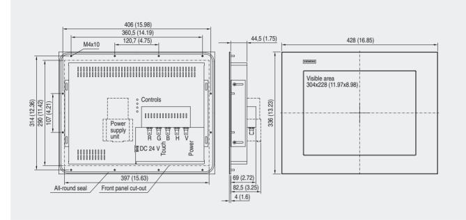
SCD 1515-E, dimensioned drawing, dimensions in mm (inch)
