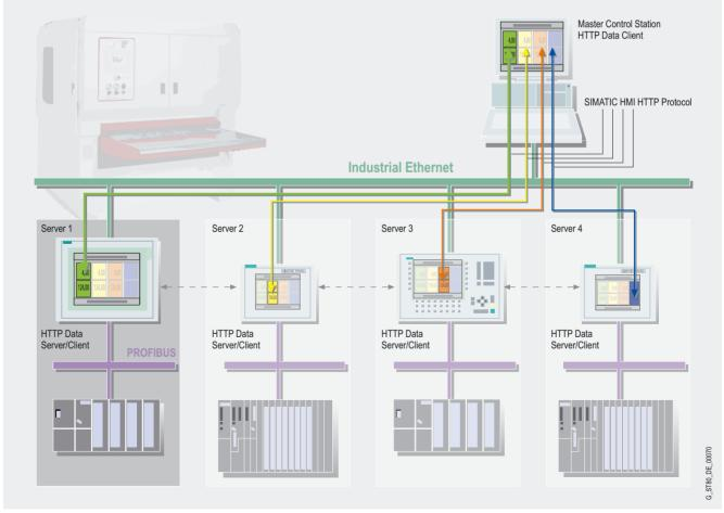
Communication between HMI systems using Industrial Ethernet:
