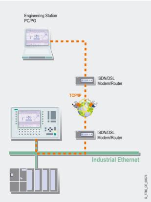
Remote operator control and monitoring of SIMATIC HMI systems via Industrial Ethernet or intranet/Internet
