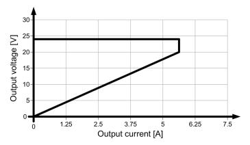
Figure 6-14 6EP1333-3BA00 latching shutdown output characteristic
