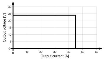
Figure 6-6 6EP1337-3BA00 single operation output characteristic
