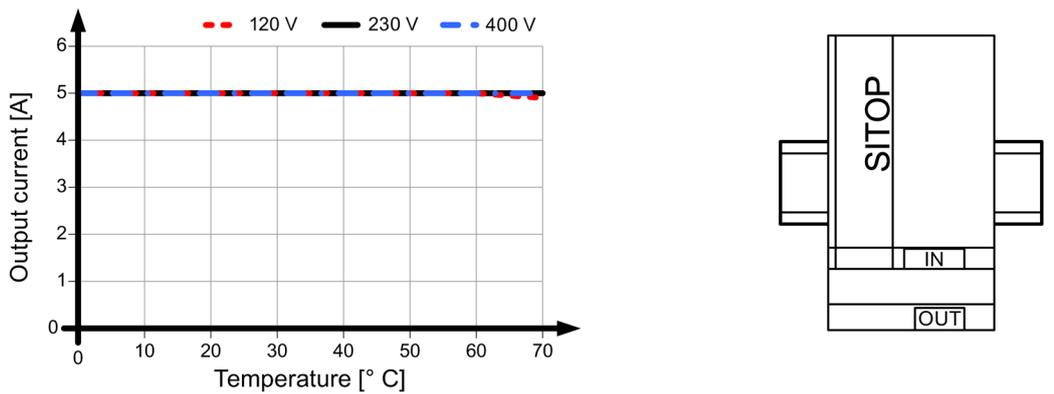
Figure 4-1 6EP1333-3BA00: Output current in the standard mounting position
