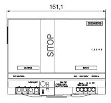
Figure 2-13 Dimension drawing for 6EP1336-3BA00
