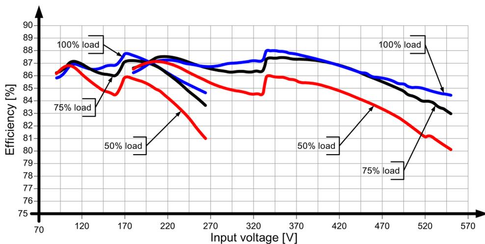
Figure 6-18 6EP1333-3BA00 efficiency
