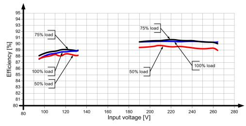
Figure 6-21 6EP1337-3BA00 efficiency
