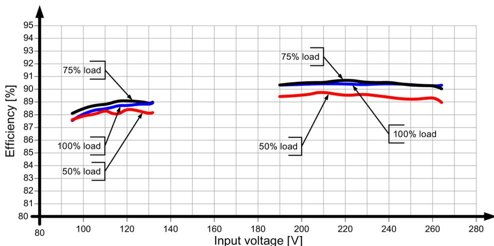
Figure 6-21 6EP1337-3BA00 efficiency
