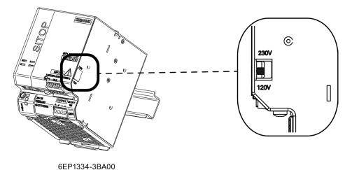
Selector switch for the input voltage range for 6EP1333-3BA00 (24 V / 5 A) and 6EP1334-3BA00 (24 V / 10 A)
