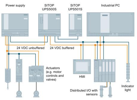
Figure 9-7 24 V buffering to allow the saving of process data and controlled shutdown of PCs
