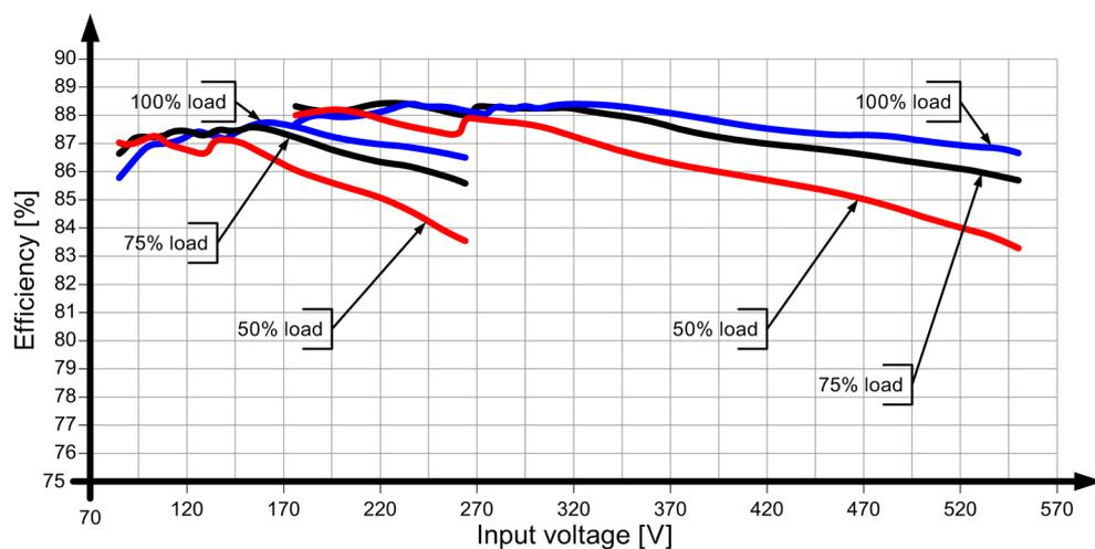
Figure 6-19 6EP1334-3BA00 efficiency
