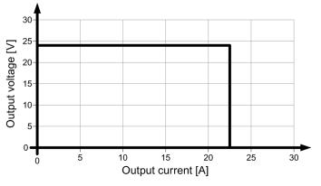
Figure 6-5 6EP1336-3BA00 single operation output characteristic
