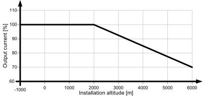
Figure 4-5 Mounting height derating
