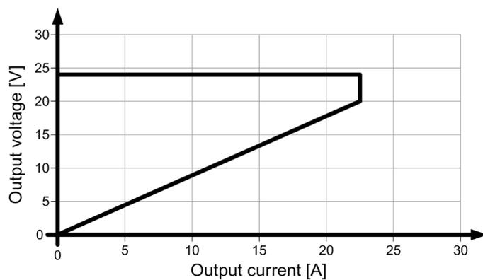
Figure 6-16 6EP1336-3BA00 latching shutdown output characteristic
