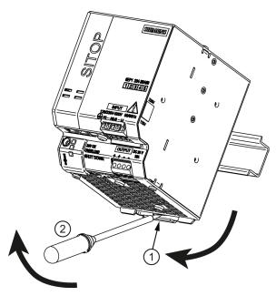
Figure 3-1 Removal (example: 6EP1334-3BA00)
