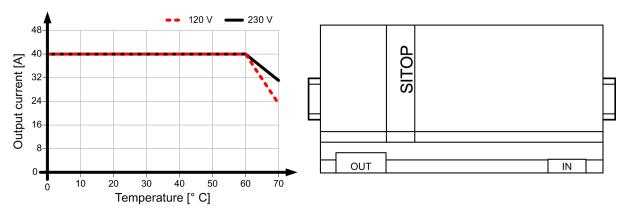
Figure 4-4 6EP1337-3BA00: Output current in the standard mounting position
