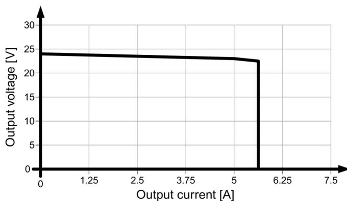
Figure 6-10 6EP1333-3BA00 parallel operation output characteristic
