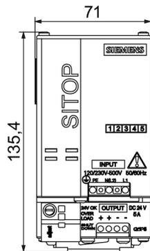
Figure 2-11 Dimension drawing for 6EP1333-3BA00
