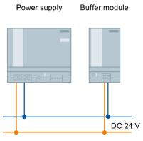
Figure 9-6 Buffering brief power failures using the SITOP PSE201M buffer module
