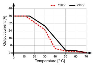
Figure 4-24 6EP1337-3BA00 mounting position (4)
