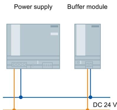
Figure 9-6 Buffering brief power failures using the SITOP PSE201M buffer module
