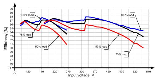
Figure 6-18 6EP1333-3BA00 efficiency
