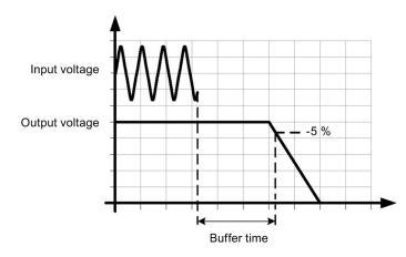
Figure 6-1 Power-failure buffering
