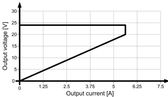
Figure 6-14 6EP1333-3BA00 latching shutdown output characteristic
