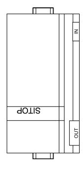
Figure 4-21 6EP1337-3BA00 mounting position (1)
