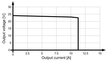
Figure 6-11 6EP1334-3BA00 parallel operation output characteristic
