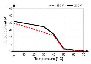
Figure 4-25 6EP1337-3BA00 mounting position (5)
