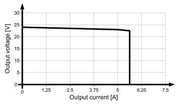
Figure 6-10 6EP1333-3BA00 parallel operation output characteristic
