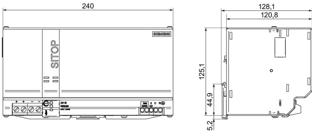
Figure 2-14 Dimension drawing for 6EP1337-3BA00
