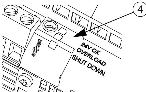
Figure 2-6 Status indicators and signals (example of 6EP1337-3BA00)
