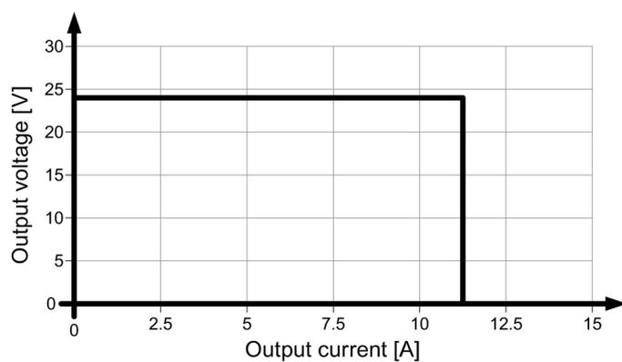
Figure 6-4 6EP1334-3BA00 single operation output characteristic
