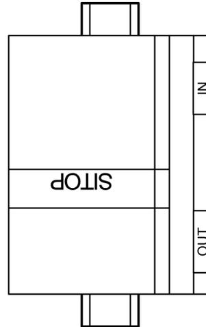
Figure 4-16 6EP1336-3BA00 mounting position (1)
