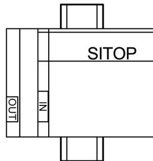
Figure 4-12 6EP1334-3BA00 mounting position (2)
