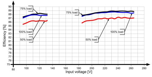
Figure 6-20 6EP1336-3BA00 efficiency
