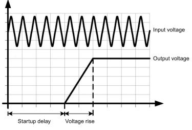
Figure 6-2 Startup delay/voltage rise
