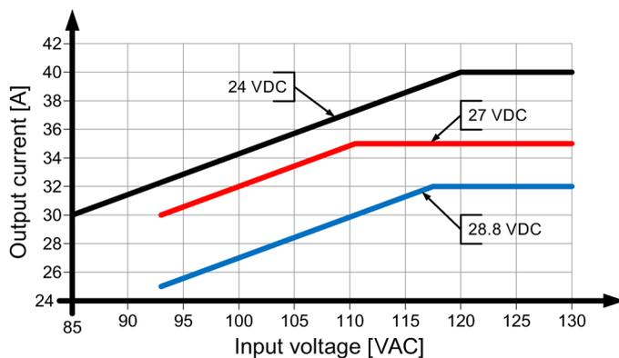
Figure 6-9 Output derating depending on the input voltage
