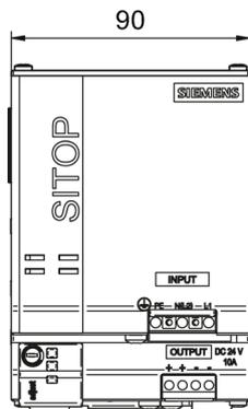
Figure 2-12 Dimension drawing for 6EP1334-3BA00
