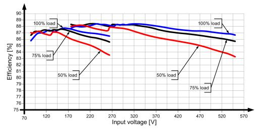
Figure 6-19 6EP1334-3BA00 efficiency
