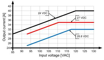
Derating for Ua >24 V depending on the input voltage (only valid for 6EP1337-3BA00):
