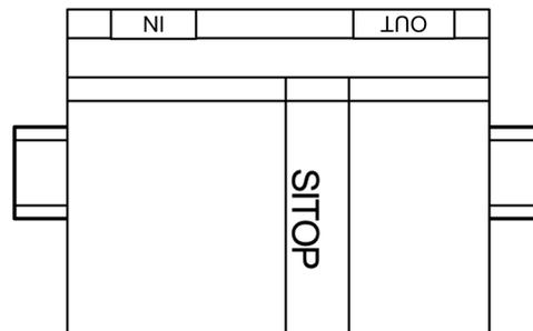
Figure 4-18 6EP1336-3BA00 mounting position (3)
