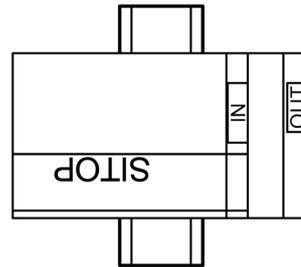
Figure 4-6 6EP1333-3BA00 mounting position (1)
