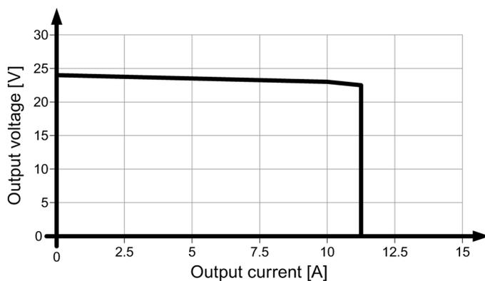
Figure 6-11 6EP1334-3BA00 parallel operation output characteristic
