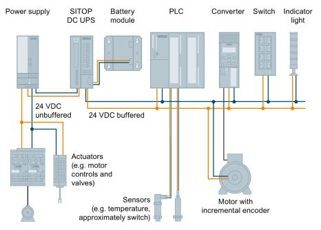
Using DC-UPS with battery modules (lead acid accumulators), buffer times in the range of hours can be implemented.
