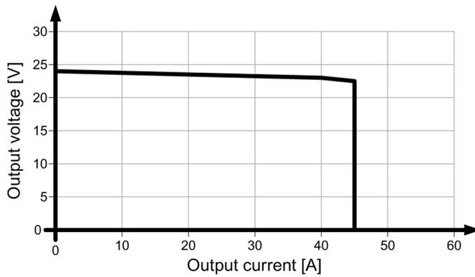
Figure 6-13 6EP1337-3BA00 parallel operation output characteristic
