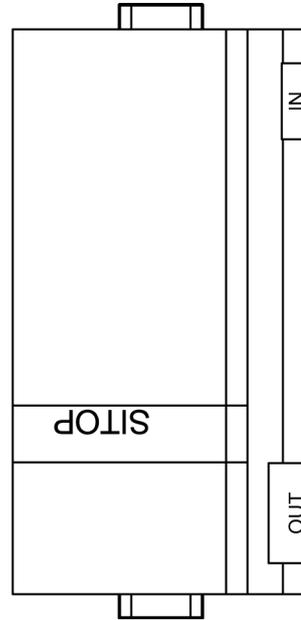
Figure 4-21 6EP1337-3BA00 mounting position (1)
