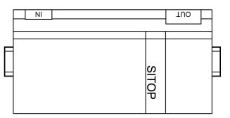
Figure 4-23 6EP1337-3BA00 mounting position (3)
