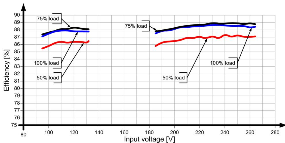
Figure 6-20 6EP1336-3BA00 efficiency
