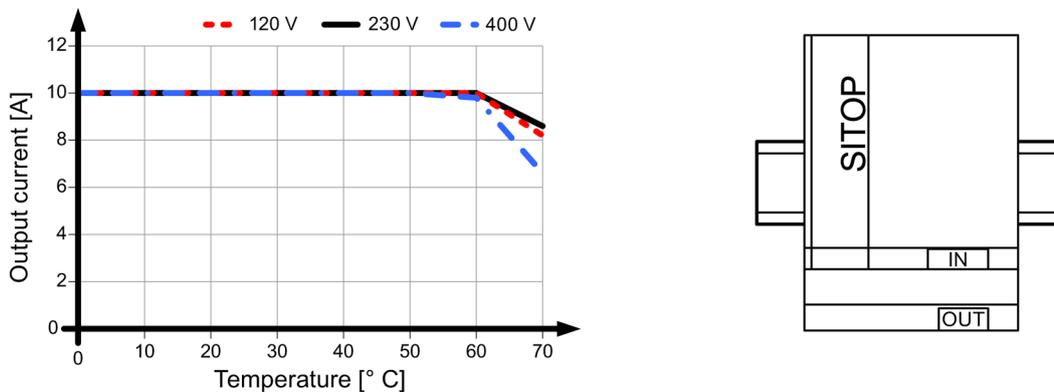
Figure 4-2 6EP1334-3BA00: Output current in the standard mounting position
