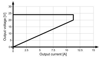
Figure 6-15 6EP1334-3BA00 latching shutdown output characteristic
