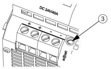
Figure 2-5 Potentiometer (example of 6EP1337-3BA00)
