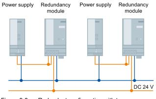
Figure 9-3 Redundant configuration with two power supplies and two SITOP PSE202U redundancy modules
