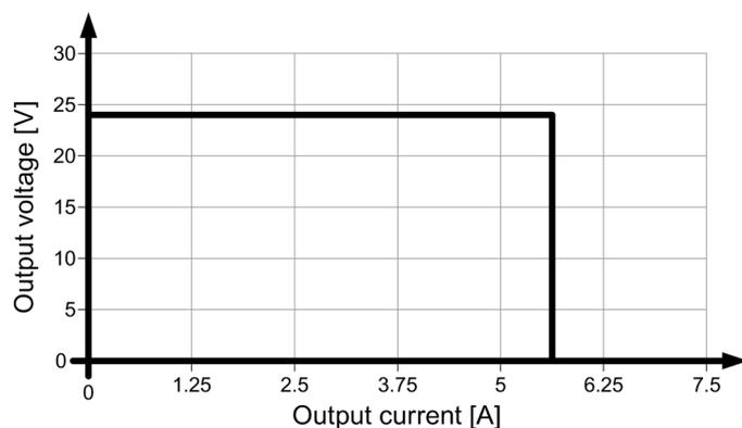
Figure 6-3 6EP1333-3BA00 single operation output characteristic
