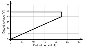
Figure 6-16 6EP1336-3BA00 latching shutdown output characteristic
