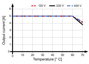
Figure 4-8 6EP1333-3BA00 mounting position (3)
