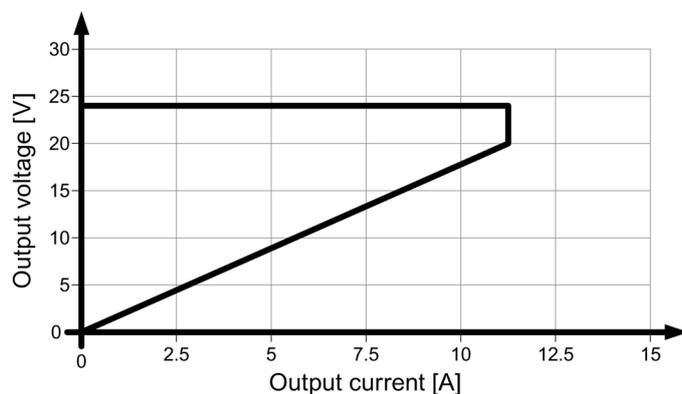
Figure 6-15 6EP1334-3BA00 latching shutdown output characteristic
