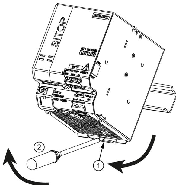
Figure 3-1 Removal (example: 6EP1334-3BA00)
