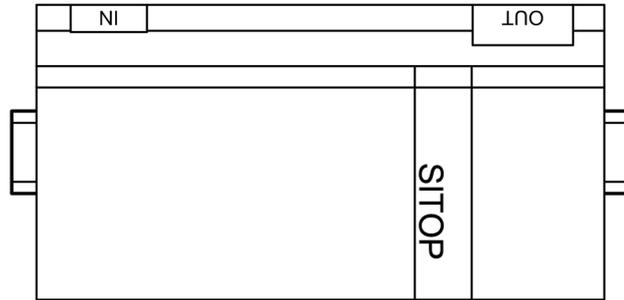
Figure 4-23 6EP1337-3BA00 mounting position (3)
