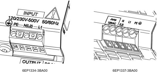
Figure 5-1 Line connection 6EP1337-3BA00
