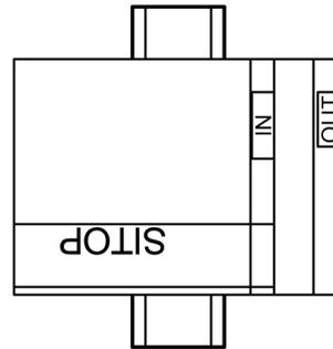
Figure 4-11 6EP1334-3BA00 mounting position (1)
