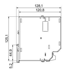
Figure 2-14 Dimension drawing for 6EP1337-3BA00
