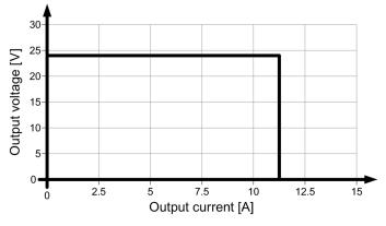
Figure 6-4 6EP1334-3BA00 single operation output characteristic
