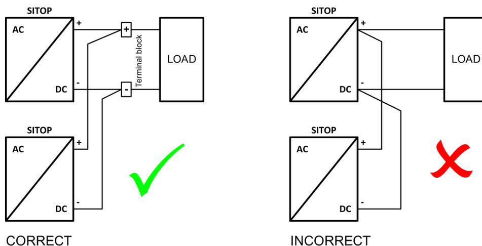
Figure 9-1 Parallel connection
