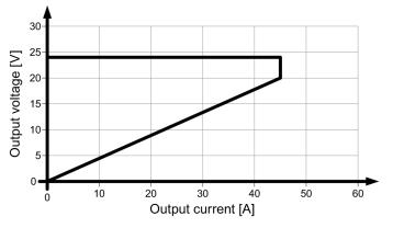
Figure 6-17 6EP1337-3BA00 latching shutdown output characteristic
