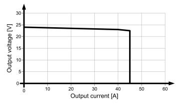
Figure 6-13 6EP1337-3BA00 parallel operation output characteristic
