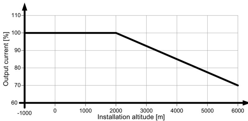
Figure 4-5 Mounting height derating
