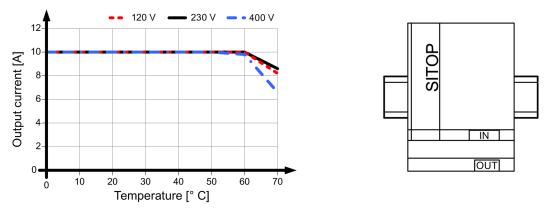
Figure 4-2 6EP1334-3BA00: Output current in the standard mounting position
