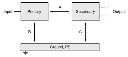
Figure 7-1 Test voltage diagram
