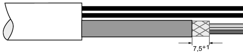
Figure 5-9 PROFIBUS Hybrid cable with heat-shrink tubing
