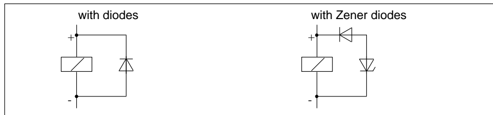
Figure 4-8 Suppressor Circuit with DC-Operated Coils with Diodes and Zener Diodes
