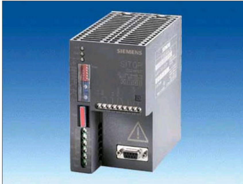
Fig. 2-27 View: SITOP POWER, DC-UPS MODULE 10
