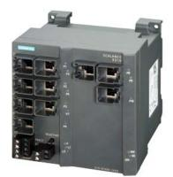
SCALANCE X310, managed plus IE switch, 3x 10/100/1000 Mbit/ and 7x 10/100 Mbit/s RJ45 ports LED diagnostics, error signaling Contact with select/set button, PROFINET IO device, network management, Integrated redundancy manager, office features (RSTP, VLAN, IGMP,..) C-plug in scope of delivery
