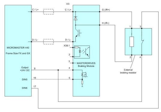
Figure 3-1 Connecting the braking module to drive inverters MM440, FX and GX
