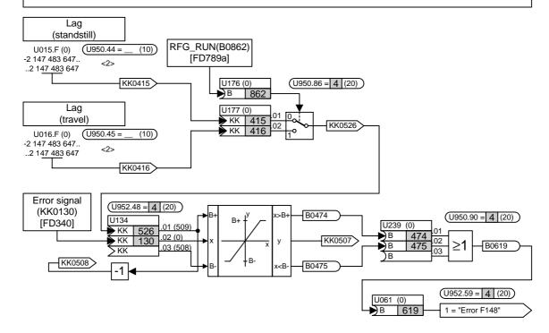
Fig. 7-12 Implement lag monitoring using free blocks
