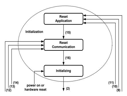
Fig. 8.5-2 Structure of the initialization state
