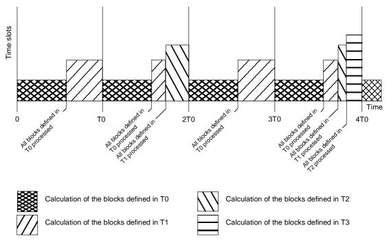
Fig. 7-1 Processing sequence of the time slots
