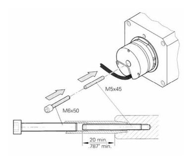
Fig. 7-13 Forcing off an encoder of old design
