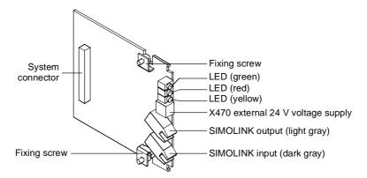
Fig. 8.3-6 SLB optional board (SIMOLINK board)
