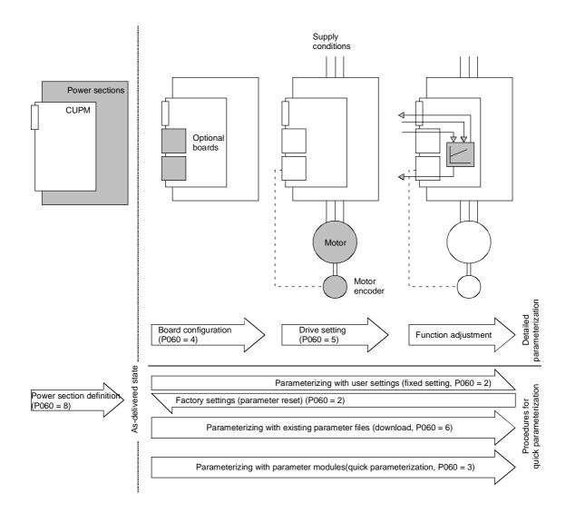
Fig. 6-1 Detailed and quick parameterization
