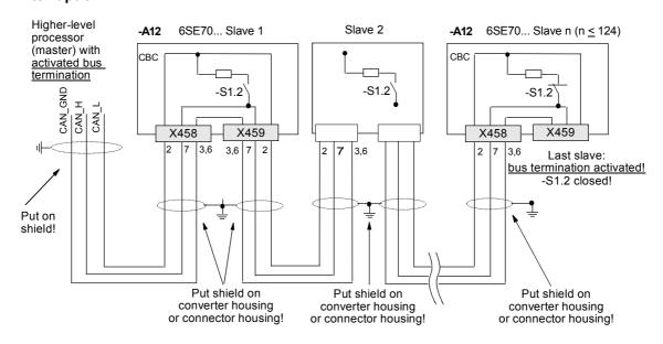
Fig. 8.4-13 Bus connection interrupted when connector X458 or X459 is pulled out
