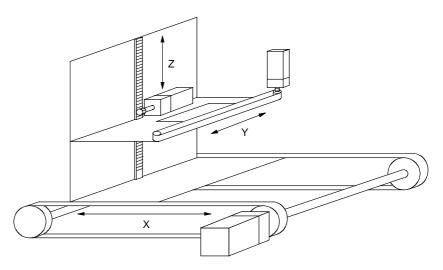
Fig. 11-12 Line drawing of a three-axis conveyor vehicle
