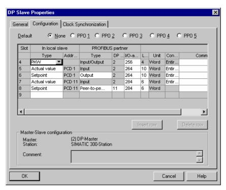
Fig. 9-51 Master axis CBP address 11
