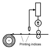
If the printing index comes too late, short-time acceleration has to take place to make up the position delay again. Beforehand, the position setpoint and actual value are set in the counter-direction in order to create the correct reference to the mechanical system.
