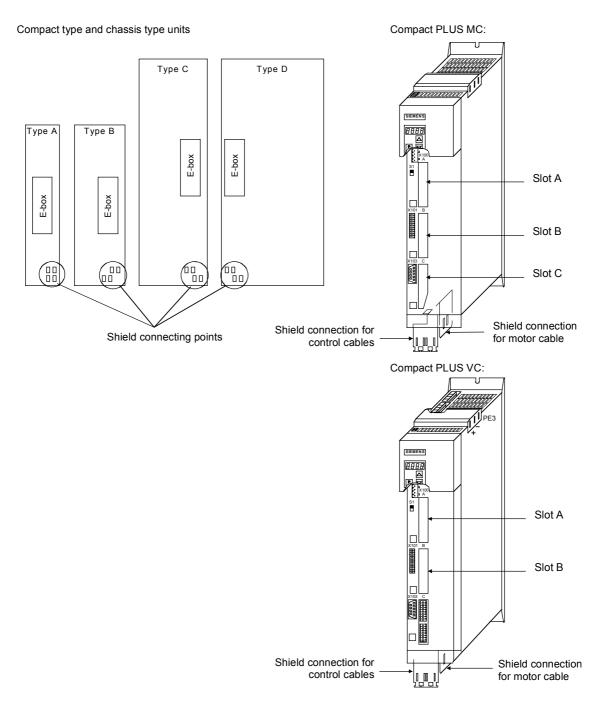
Fig. 8.1-11 Position of the shield connecting points
