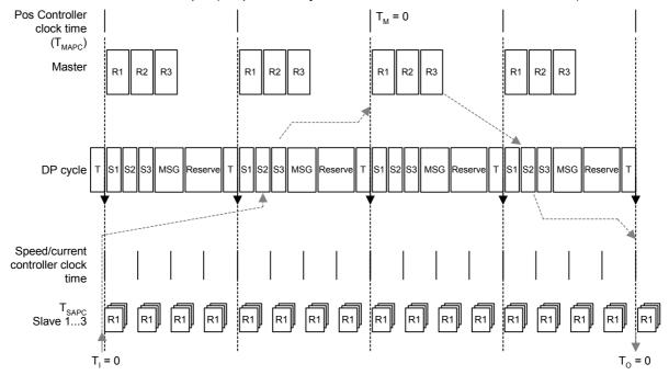
Fig. 8.2-37 Example: simplest DP cycle
