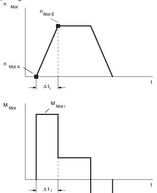
Fig. 11-9 Example of motor speed and motor torque in a time segment  $\Delta t_i$
