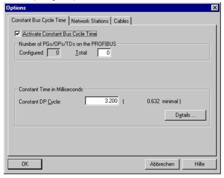
Fig. 9-54 Activation of the equidistance on the CPU
