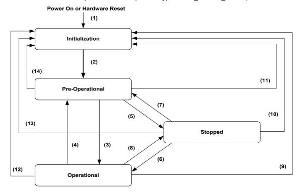
Fig. 8.5-1 State diagram of a device
