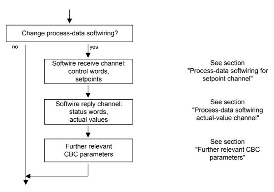
Fig. 8.4-18 Procedure for altering process data
