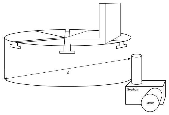
Fig. 7-11 Example of rotary axis, the rotary table
