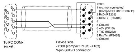
Fig. 5-7 Connecting cable for connecting PC COM(1-4) to SIMOVERT MASTERDRIVES X300
