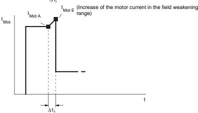
Fig. 11-10 Example of motor speed and motor current in a time segment  $\Delta t_i$
