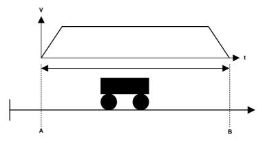
Fig. 7-2 Moving from A to B
