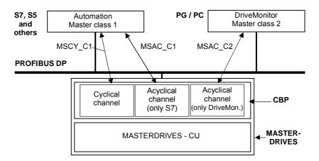
Fig. 8.2-3 Data-traffic channels of the CBP
