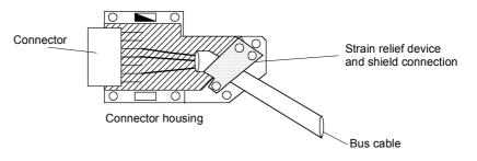
Fig. 8.4-8 Connecting the bus cables
