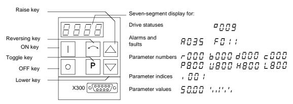
Fig. 5-3 PMU parameterizing unit
