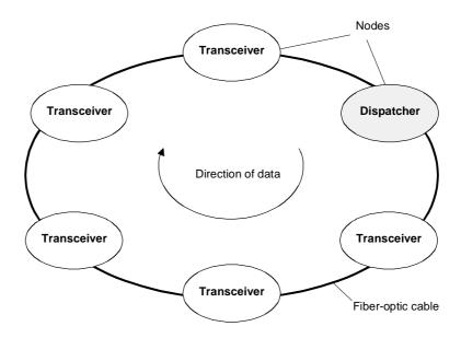
Fig. 8.3-3 SIMOLINK with dispatcher
