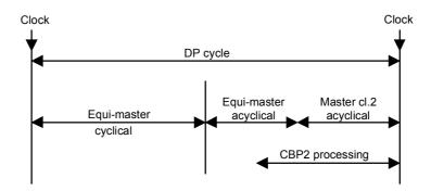
Fig. 8.2-26 Breakdown of the DP cycle at the isochronous PROFIBUS
