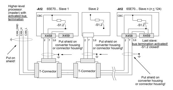
Fig. 8.4-14 Bus connection not interrupted when connector X458 is pulled out
