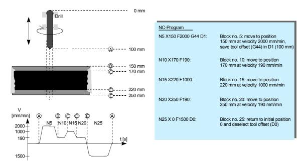
Fig. 9-5 Example of an automatic program
