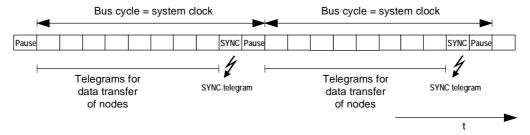
Fig. 8.3-2 SIMOLINK telegram traffic
