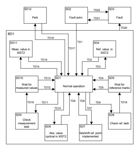
Fig. 8.2-39 Status diagram of encoder interface showing the statuses and transitions
