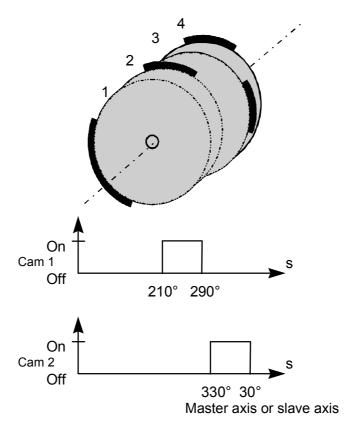
Fig. 9-9 Cam controller with MASTERDRIVES MC
