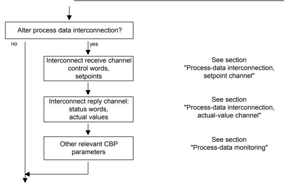
Fig. 8.2-20 Procedure for changing process data
