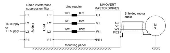
Fig. 3-4 Arrangement of the components
