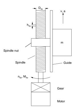
Fig. 11-6 Vertical spindle drive
