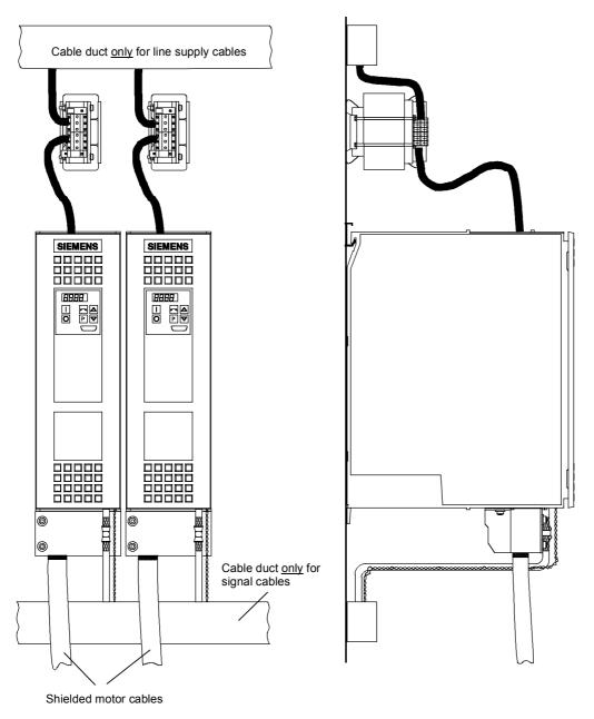
Fig. 3-19 Installation with separate cable ducts
