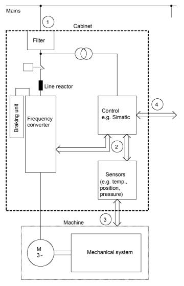
Fig. 3-7 Block diagram of a drive system
