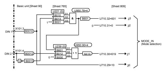
Fig. 9-48 Application example 2: circuit for generating the modes
