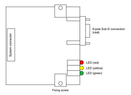
Fig. 8.2-1 View of the communications board
