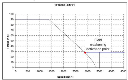
e.g. 1FT6086-8AF71, 27.5 Nm at 2900 rev/min to 4500 rev/min,  $U_{(no\ load\ 2900)}=296\ V,\ U_{(no\ load\ 4500)}=174\ V\ I_{k}$  (P105) = 60 A
