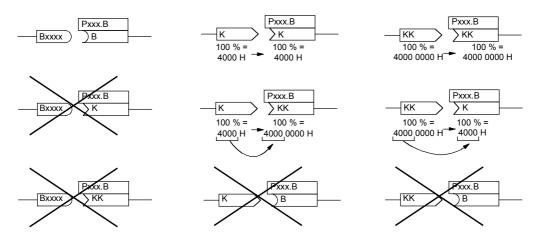
Fig. 4-9 Possible and impossible BICO connections
