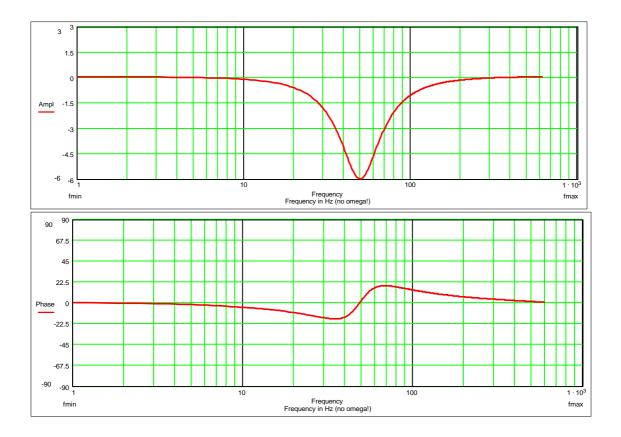
Example 3 Band-stop filter with full suppression and high quality: (P256 = 1; P254 = 50 Hz; P253 = 3.0; P257 = 0 %)
