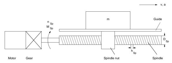
Fig. 11-5 Horizontal spindle drive
