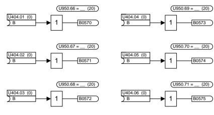
The block does not have any logic function. It only transfers a digital signal consistently from a faster sampling time to a slower one. The block ensures that the signal has the same value in the slow sampling time for all "consumers" (signal sinks).
