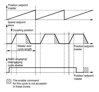
Fig. 9-35 Example: engaging cycle for rotary axis
