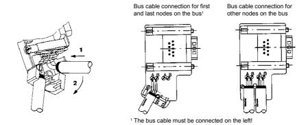
Fig. 8.2-11 Connecting up the bus cable to the bus connector
