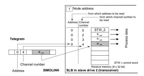
Fig. 8.3-10 Slave drive 2, reading data
