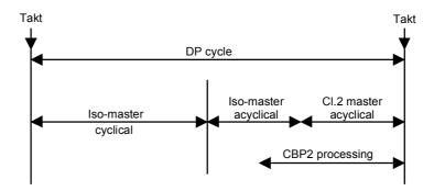
Fig. 8.2-27 Splitting of DP cycle on isochronous PROFIBUS
