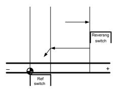
The reversing switch is always active in homing mode. A digital output (MD45 = 8) can be used for connecting the reversing switch.
