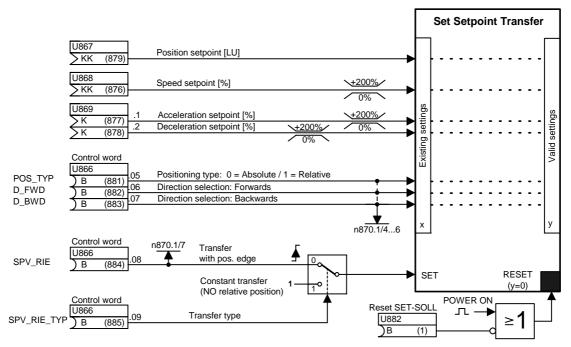
Fig. 7-3 Setpoint transfer input
