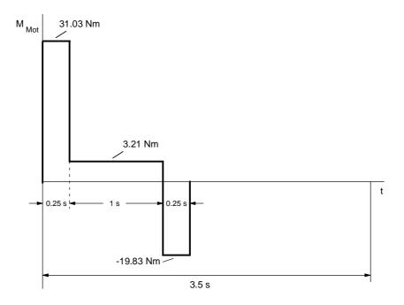
Fig. 11-15 Torque characteristic for forwards travel
