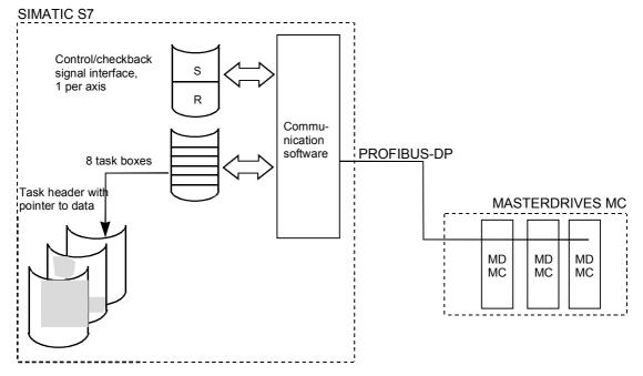
Fig. 9-44 Communication interfaces from GMC-BASIC to technology
