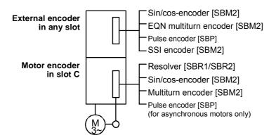
Fig. 9-10 Overview of suitable sensor boards
