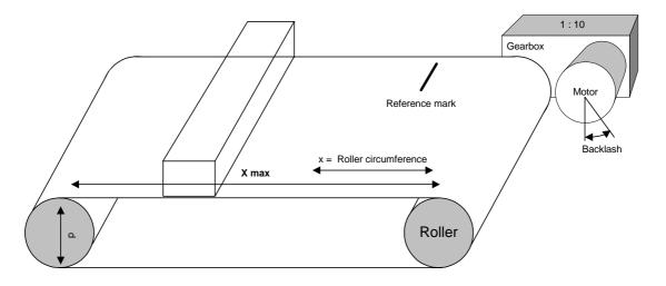
Fig. 7-7 Typical positioning application
