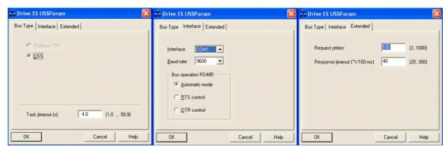
Fig. 5-9 Interface configuration
