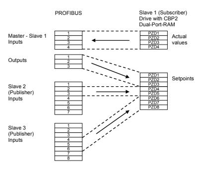
Fig. 8.2-25 Example of a cross-traffic configuration
