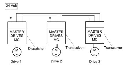
Fig. 8.3-7 Configuration example of peer-to-peer functionality
