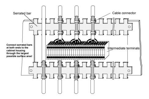
Fig. 3-13 Connecting signal cable shields in the cabinet
