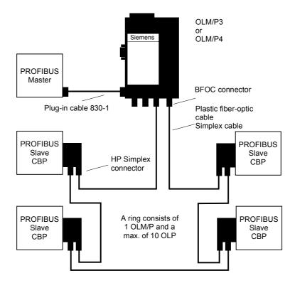
Fig. 8.2-15 Example of a system configuration with OLPs
