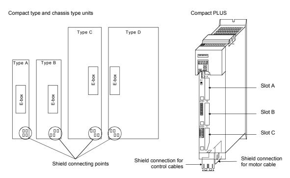
Fig. 8.4-10 Position of the shield connecting points
