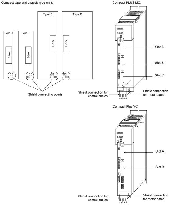
Fig. 8.2-17 Position of the shield connecting points
