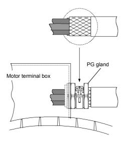
Fig. 3-11 Shield connection at the motor
