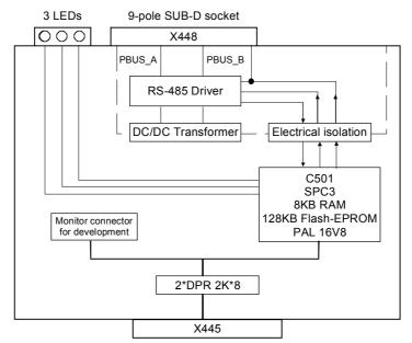
Fig. 8.2-40 Block diagram of the CBP
