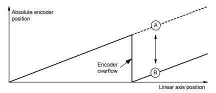
When the encoder overflows, the absolute encoder starts counting from zero again. The position of the linear axis is position A, but position B is output by the absolute encoder.
