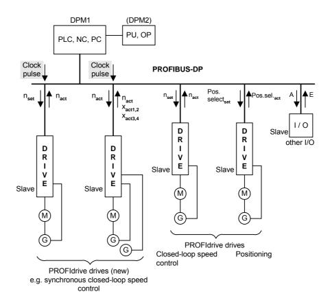
Fig. 8.2-30 Clock synchronous monomaster operation (DPM1)
