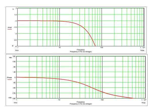
Example 2 Band-stop filter of average quality and semi-suppression of the resonant frequency (P256 = 1; P254 = 50 Hz; P253 = 1.0; P257 = 50 %)
