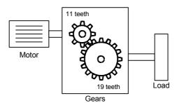
In the example, the motor makes 19 revolutions for 11 revolutions of the load. The value 11 must be entered in U810.01, and the value 19 in U810.02.
