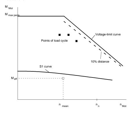
Fig. 11-7 Limit curves for 1FK6/1FT6 motors (synchronous servomotors)
