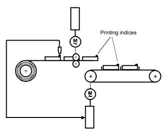
The drive being taken into consideration is normally arranged behind the drive transporting the material with the printing index (and not itself evaluating the printing index). If the printing index comes too late, the drive must brake briefly in order to "wait" for the printing index.
