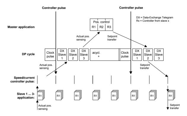
Fig. 8.2-31 Clock synchronous communication
