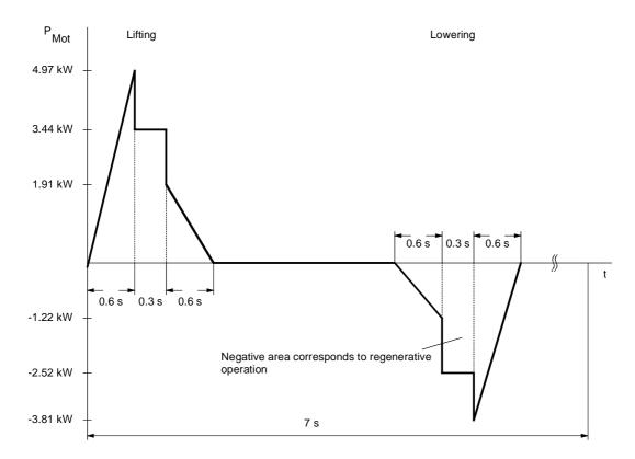
Fig. 11-22 Curve of motor power output for lifting and lowering
