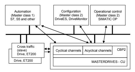
Fig. 8.2-4 Data-traffic channels of the CBP2
