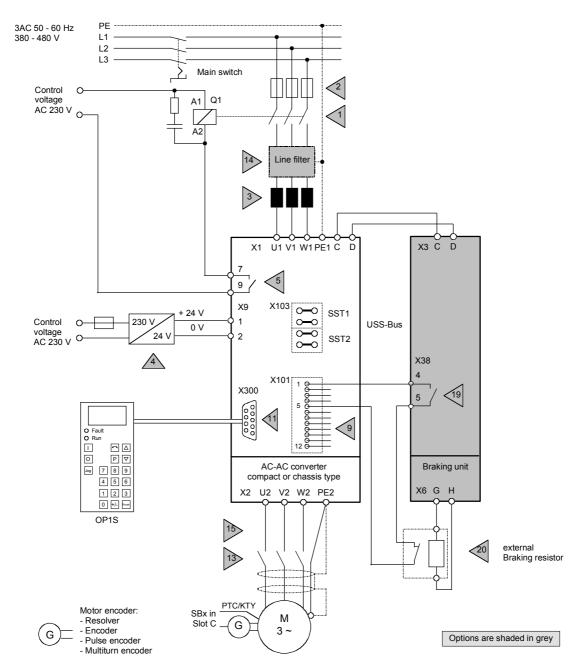
Fig. 2-4 Configuring example: single-axis drive with Compact or chassis-type
