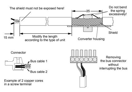
Fig. 8.1-9 Connecting up the bus cables
