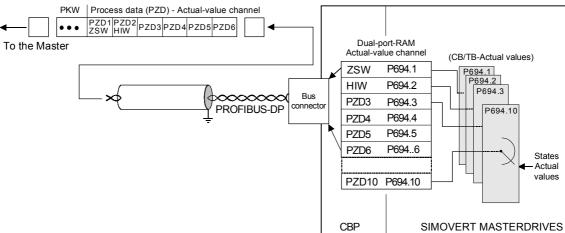
Fig. 8.2-22 Example of process data interconnection for function classes FC (CU1), VC (CU2) and SC (CU3)
