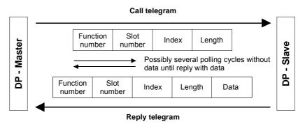
Fig. 8.2-5 Sequence of a Read and Write function
