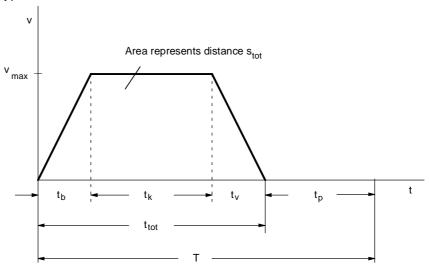
Fig. 11-1 Example of a simple travel curve
