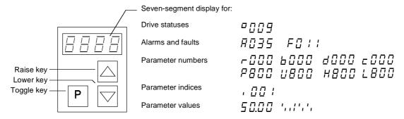
Fig. 5-2 PMU in units of the Compact PLUS type
