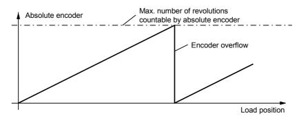
To save costs, an absolute encoder is fitted on the motor and used both for torque and speed control and for position control (EQN 1325). One advantage of this is that fitting the encoder on the motor is much less critical but much more precise than fitting it on the load side.
