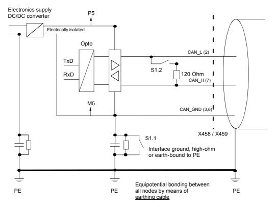
Fig. 8.4-12 Function of jumper strip S1
