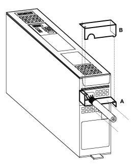
Fig. 3-17 Mounting the connecting adapter
