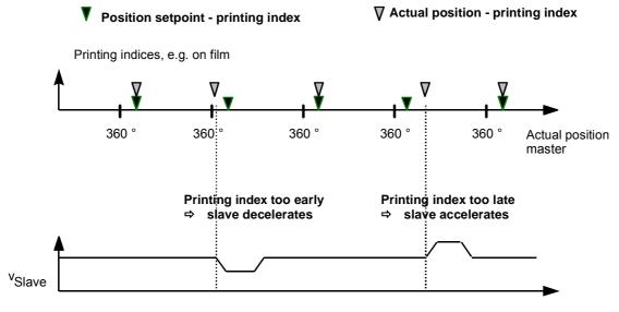
Fig. 9-8 Principle of printing index synchronization
