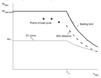
Fig. 11-8 Limit curves for 1PA6 motors (induction servomotors)
