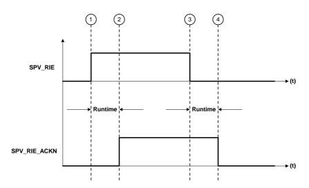
Fig. 7-4 Signal sequence of acknowledgement controlled setpoint transfer
