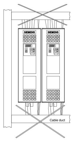
Fig. 3-20 Installation with cable ducts
