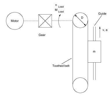
Fig. 11-3 Lifting drive
