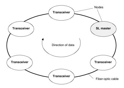
Fig. 8.3-12 SIMOLINK ring with SL master
