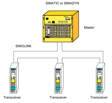
Fig. 8.3-13 Application example of master/slave functionality
