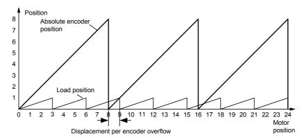
Example: Gear ratio 1:3, absolute encoder can count 8 revolutions
