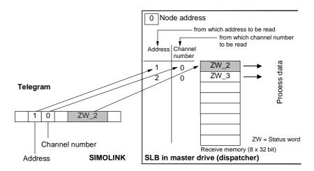
Fig. 8.3-8 Master drive 1, reading data
