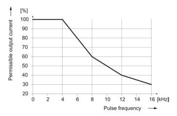
Figure 7-18 Output current as a function of the pulse frequency for the Motor Module ≥ 9 A
