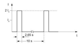
Figure 7-10 Duty cycle without initial load
