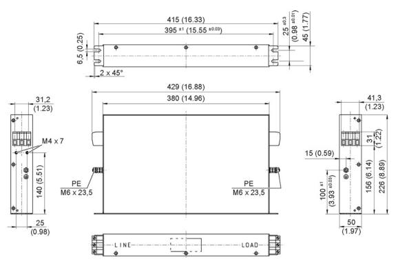
Figure 3-6 Dimension drawing of the Basic Line Filter for Active Line Modules 16 kW, all data in mm and (inches)
