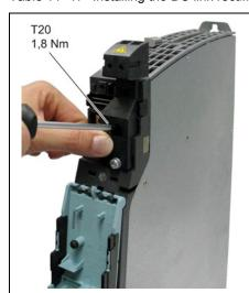
Attach and screw (upper and lower screws) the DC link rectifier adapter at the right-hand side of the component using the original M4x20 screws.
