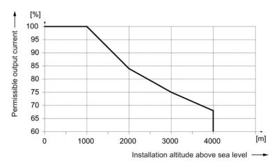
Figure 4-60 Output current as a function of the installation altitude
