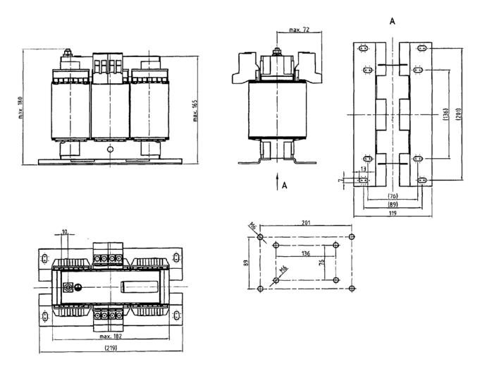
Figure 3-48 Dimension drawing of line reactor for Smart Line Module 16 kW
