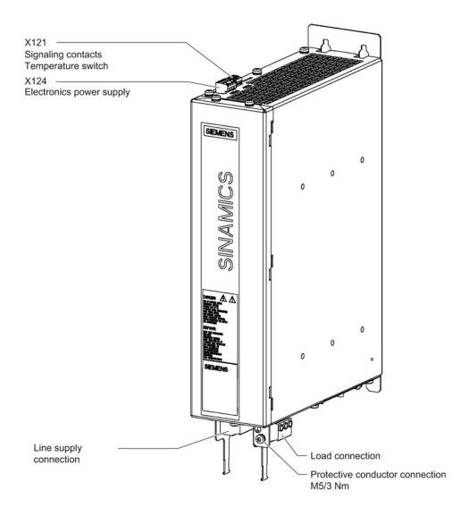
Figure 3-51 Interface overview, Active Interface Module 16 kW
