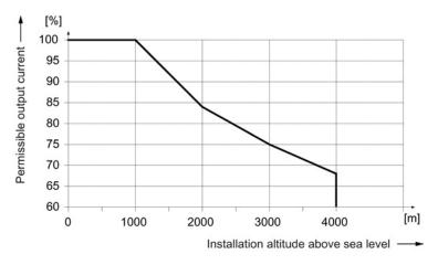
Figure 6-21 Output current as a function of the installation altitude
