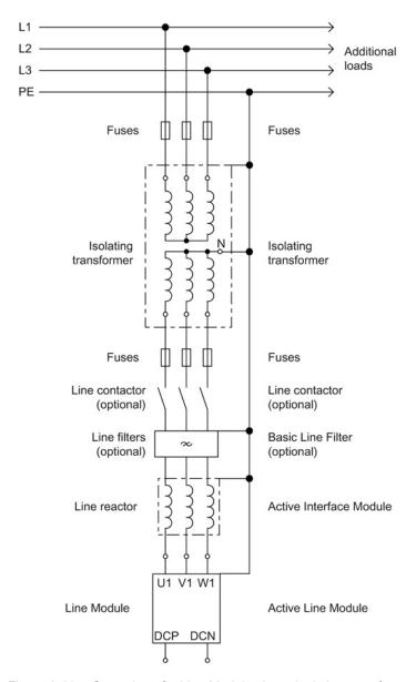
Figure 3-68 Operation of a Line Module via an isolating transformer
