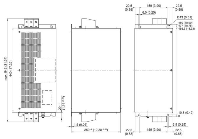
Figure 3-14 Dimension drawing of Wideband Line Filter 80 kW for Active Lines Modules, all dimensions in mm and (inches)
