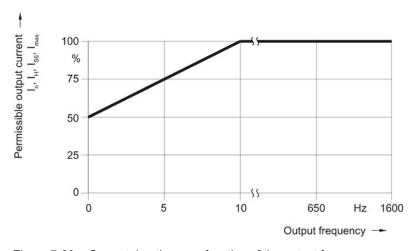
Figure 7-20 Current derating as a function of the output frequency
