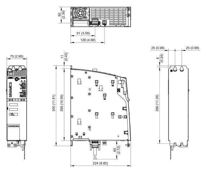
Figure 7-5 Dimension drawing of 18 A Motor Module Booksize Compact, all dimensions in mm and (inches)
