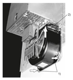
Figure 4-8 Mounting the fan for Active Line Modules 80 kW and 120 kW
