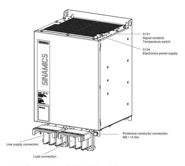
Figure 3-54 Interface overview, Active Interface Module 80 kW and 120 kW
