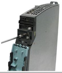
Remove the lower left-hand screw and the DC link bridge
