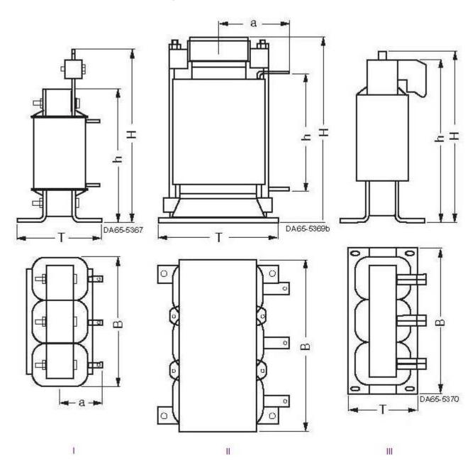
Figure 10-1 Dimension drawings of motor reactors
