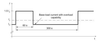
Figure 6-65 Duty cycle with 60 s overload for a duty cycle duration of 300 s
