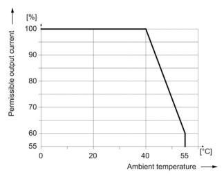
Figure 4-59 Output current as a function of the ambient temperature
