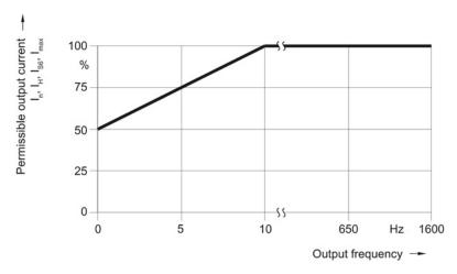
Figure 6-70 Output current as a function of the output frequency
