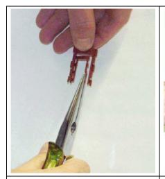
Adapt a restrictor collar (using a suitable tool) for the touch protection.
