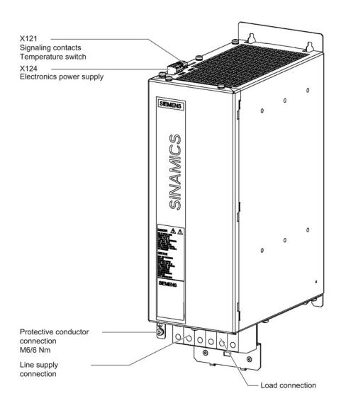
Figure 3-52 Interface overview, Active Interface Module 36 kW
