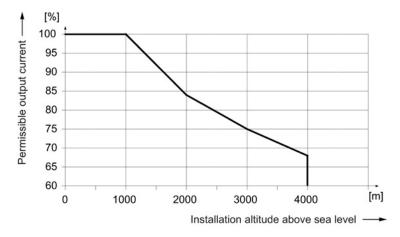
Figure 4-87 Output current as a function of the installation altitude
