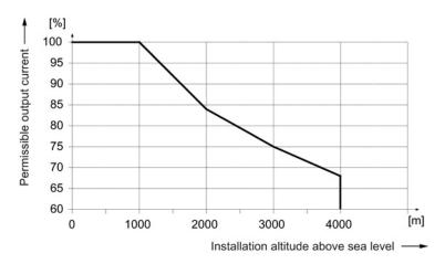
Figure 6-116 Output current as a function of the installation altitude
