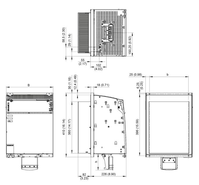
Figure 6-41 Dimension drawing of 132 A and 200 A Motor Modules Booksize, all dimensions in mm and (inches); example: 200 A Single Motor Module
