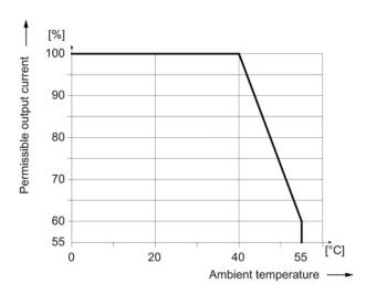
Figure 6-18 Output current as a function of the ambient temperature
