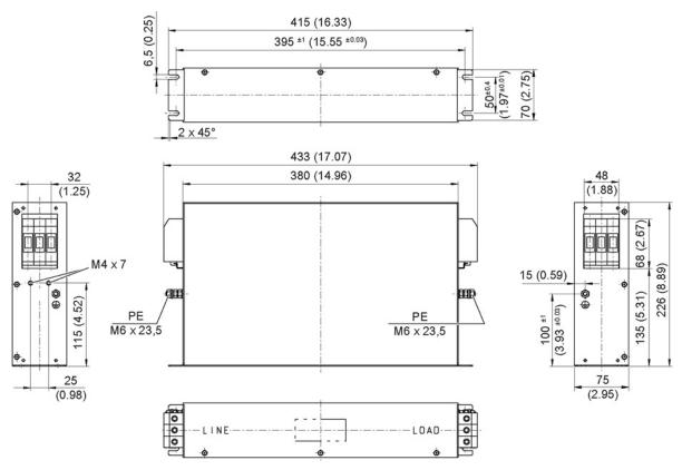
Figure 3-18 Dimension drawing of Basic Line Filter for Basic Line Modules 40 kW, all data in mm and (inches)
