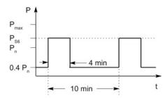
Figure 4-70 S6 duty cycle with pre-load condition
