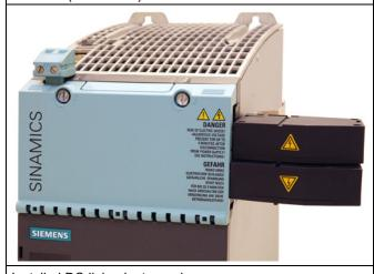
Installed DC-link adapter and 24 V terminal adapter
