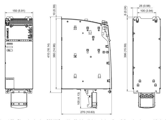
Figure 4-82 Dimension drawing of 36 kW Smart Line Module with internal air cooling, all dimensions in mm and (inches)
