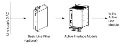
Figure 3-1 Overview diagram, line connection with Active Interface Module
