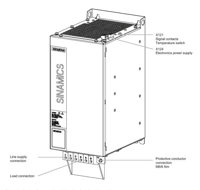
Figure 3-53 Interface overview, Active Interface Module 55 kW
