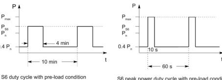
S6 peak power duty cycle with pre-load condition
