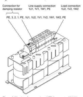
Figure 3-26 Interface overview, HFD line reactor 36 kW
