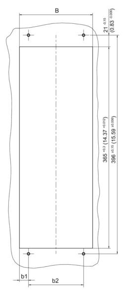
Figure 4-98 Opening to mount Smart Line Modules 50 mm to 200 mm with external air cooling, all data in mm and (inches)
