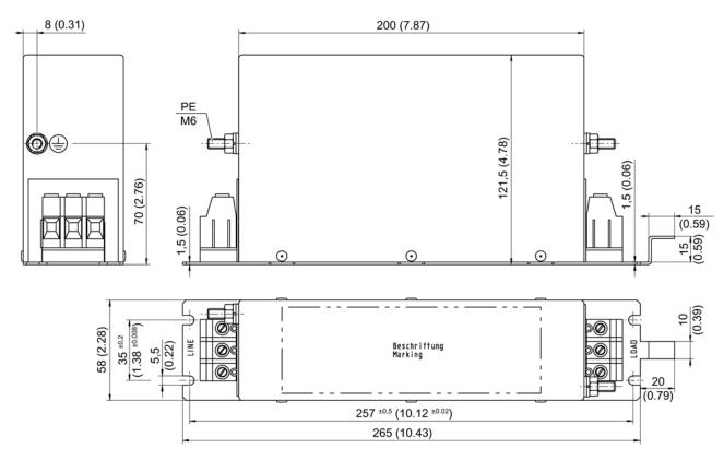
Figure 3-21 Dimension drawing of Basic Line Filter for 5 kW and 10 kW Smart Line Modules, all dimensions in mm and (inches)
