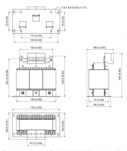
Figure 3-42 Dimension drawing of line reactor for Basic Line Module 20 kW, all dimensions in mm and (inches)
