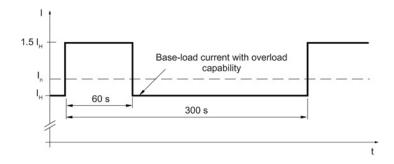
Figure 6-85 Duty cycle with 60 s overload for a duty cycle duration of 300 s
