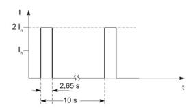
Figure 6-25 Duty cycle without initial load
