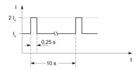
Figure 6-92 Duty cycle with initial load
