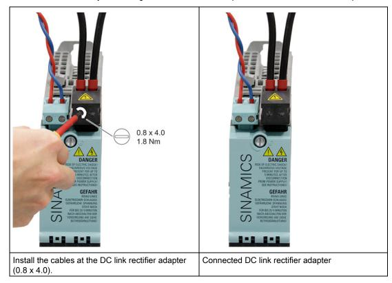
Install the cables at the DC link rectifier adapter (hexagon socket-head screw)
