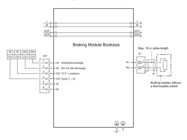
Figure 8-2 Connection example of a Braking Module Booksize
