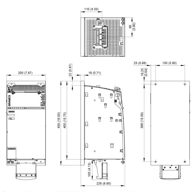
Figure 4-66 Dimension drawing of 100 kW Basic Line Module with cold plate, all dimensions in mm and (inches)
