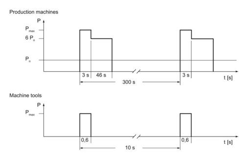
Figure 4-58 Braking duty cycle for Basic Line Modules
