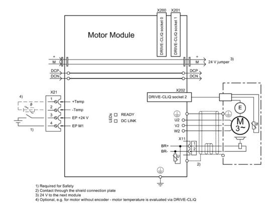
Figure 6-103 Connection example for Motor Module Liquid Cooled (200 A)
