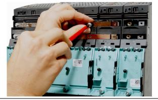
Attach the DC link busbars using the original M4x20 screws at the right-hand side of the component.
