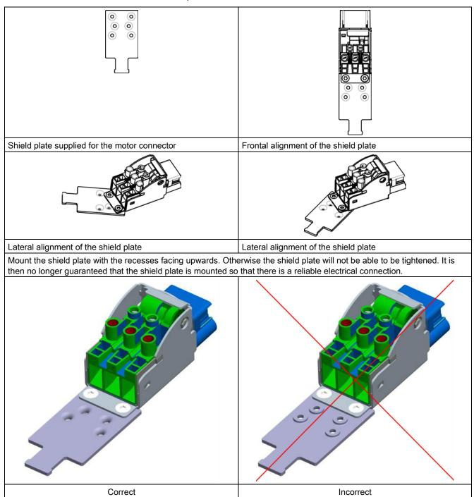
The shield plate can be mounted at various angles at the motor connector using two screws (M4) that are provided (tightening torque: 1.8 Nm).
