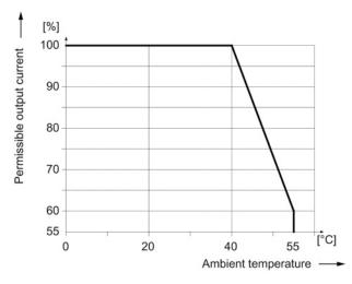
Figure 6-86 Output current as a function of the ambient temperature
