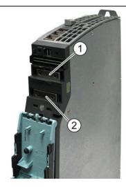
To install the DC link rectifier adapter, it is essential to leave the DC link busbars ① and ② in the components (hold firmly to prevent them falling out).
