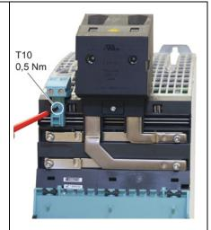
Attach the adapter busbars using the previously removed DC link screws.
