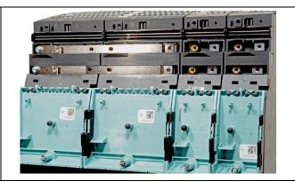
Install the reinforced DC link busbars, starting at the left.
