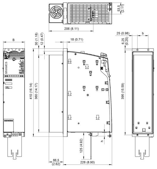
Figure 4-16 Dimension drawing of 16 kW Active Line Module with external air cooling, all dimensions in mm and (inches)
