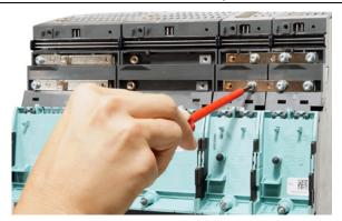
Release the screws and remove the DC link bridges and busbars at all of the other components.
