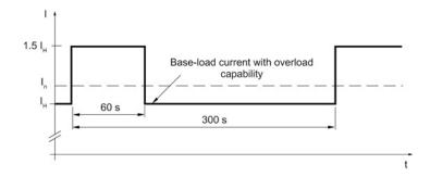
Figure 6-111 Duty cycle with 60 s overload for a duty cycle duration of 300 s
