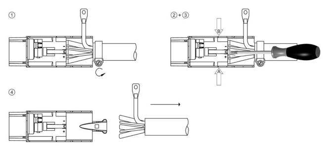
Figure 12-32 Removing the motor connector, crimped version
