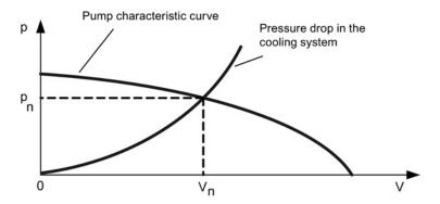
Figure 13-1 Pump characteristic curve
