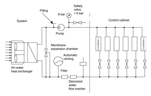
Figure 13-5 Air-to-water heat exchanger
