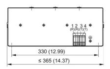
1, 2 (R) Power cable connection 3, 4 (T) Temperature sensor connection
