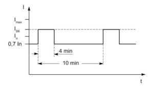
Figure 7-11 S6 duty cycle with initial load for a duty cycle duration of 600 s
