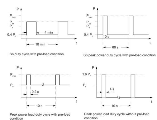
Figure 4-85 Rated duty cycles of Smart Line Modules
