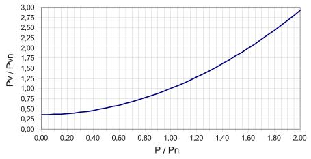
Figure 12-49 Losses in the partial load range for Active Interface Modules
