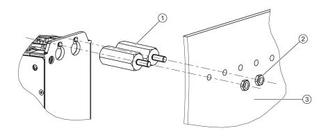
Spacing bolt M6 nuts Mounting wall
