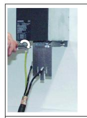
Attach the protective conductor (PE) Tightening torque: 3 Nm
