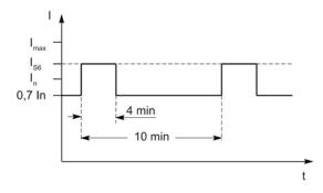
Figure 6-82 S6 duty cycle with initial load with a duty cycle duration of 600 s (for servo drives)
