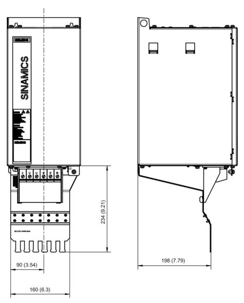
Figure 11-19 Dimension drawing of shield connecting plate on the 55 kW Active Interface Module, all dimensions in mm and (inches)
