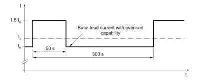
Figure 7-14 Duty cycle with 60 s overload for a duty cycle duration of 300 s
