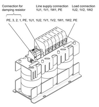
Figure 3-27 Interface overview, HFD line reactor 55 kW
