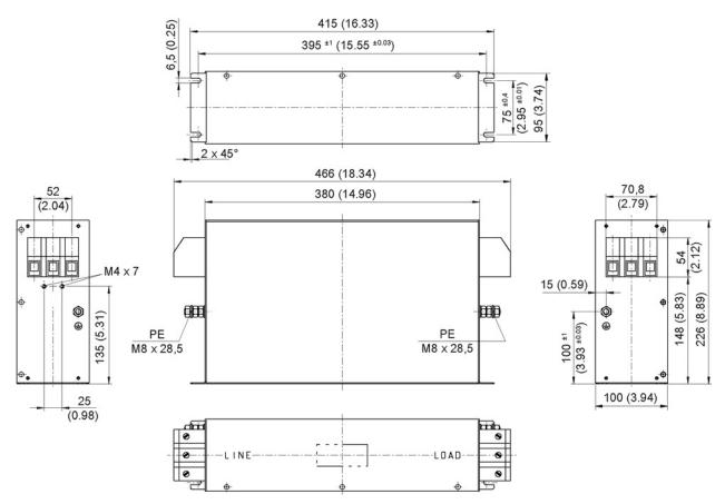
Figure 3-8 Dimension drawing of Basic Line Filter for Active Line Modules 55 kW, all data in mm and (inches)
