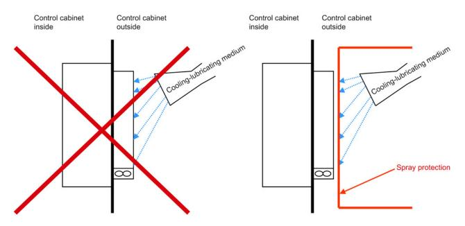
Figure 12-44 Spray protection for a drive line-up with external air cooling
