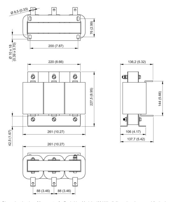
Figure 3-44 Dimension drawing of line reactor for Basic Line Module 100 kW, all dimensions in mm and (inches)
