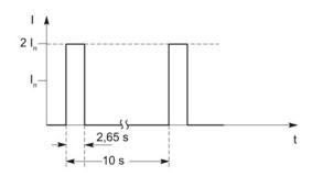
Figure 6-93 Duty cycle without initial load
