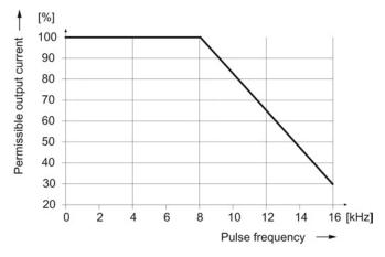
Figure 7-17 Output current as a function of the pulse frequency for the Motor Module ≤ 5 A
