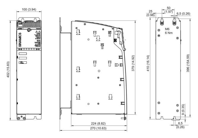
Figure 8-18 Dimension drawing of Capacitor Module, all dimensions in mm and (inches)
