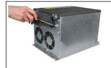
Remove the connection bracket to the noise suppression capacitor using a Tx25 screwdriver
