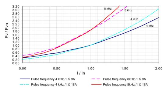
Figure 12-48 Losses in the partial load range for Motor Modules
