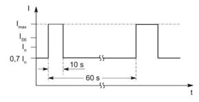
Figure 6-15 S6 duty cycle with initial load with a duty cycle duration of 60 s (for servo drives)
