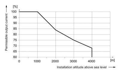
Figure 6-69 Output current as a function of the installation altitude
