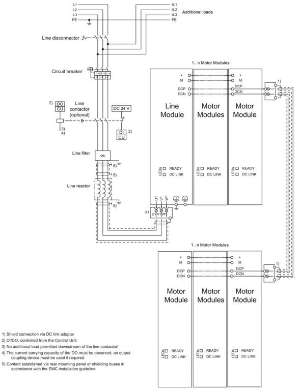
Figure 12-14 Connection example for a two-tier drive line-up
