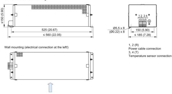
Figure 9-3 Dimension and installation drawing (roof and wall mounting) of braking resistor 6SE7018-0ES87-2DC0 where  $P_n/P_{max} = 1.25 \text{ kW}/7.5 \text{ kW}$ , all dimensions in mm and (inches)
