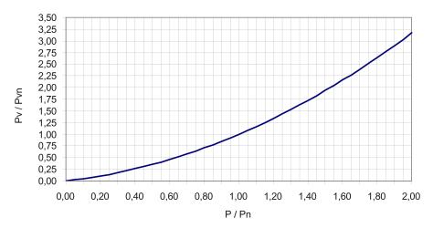
Figure 12-51 Losses in the partial load range for line reactors for Basic Line Modules
