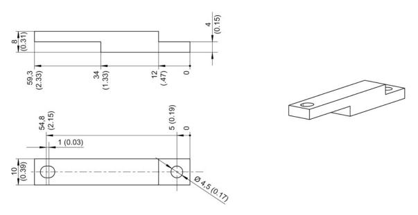
Figure 11-21 Dimension drawing of reinforced DC link busbar 50 mm, all dimensions in mm and (inches)
