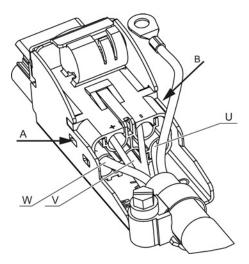
Figure 12-31 Motor connector, crimped version
