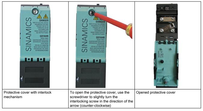
To lock, press the protective cover back on until you hear the interlock engage.
