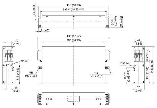
Figure 3-7 Dimension drawing of Basic Line Filter for Active Line Modules 36 kW, all data in mm and (inches)
