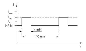
Figure 6-94 S6 duty cycle with initial load for a duty cycle duration of 600 s
