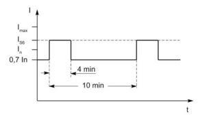
Figure 6-108 S6 duty cycle with initial load with a duty cycle duration of 600 s (for servo drives)
