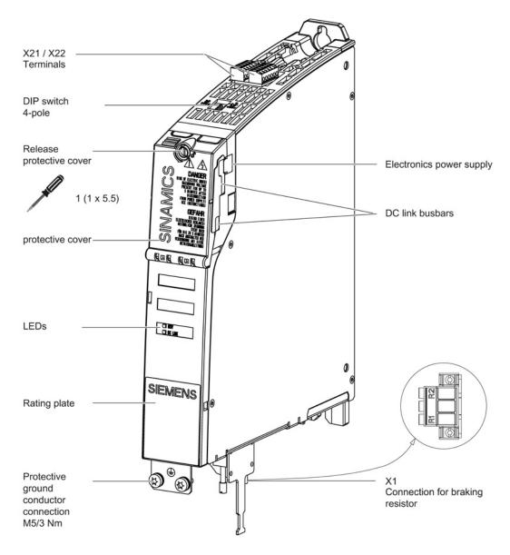
Figure 8-6 Interface overview, Braking Module Booksize Compact
