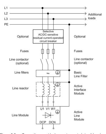
Figure 3-3 Connecting a residual-current operated circuit breaker
