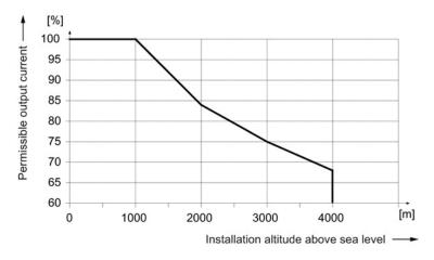
Figure 6-89 Output current as a function of the installation altitude
