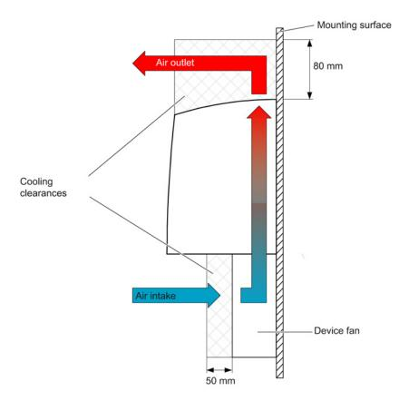
Figure 12-41 Cooling clearances for 300 mm wide components with internal air cooling with mounted unit fan
