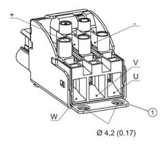
① Connection for shield plate supplied with the equipment
