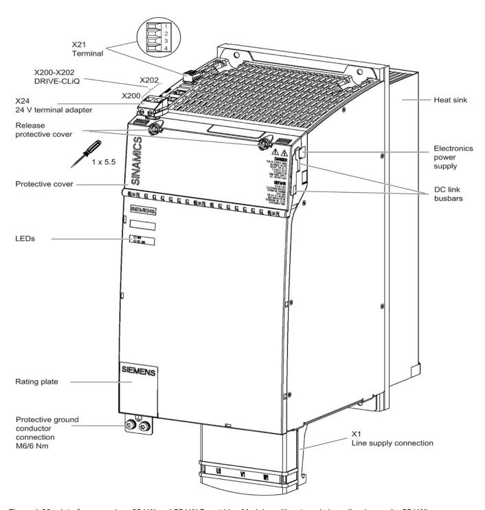
Figure 4-90 Interface overview, 36 kW and 55 kW Smart Line Modules with external air cooling (example: 55 kW)
