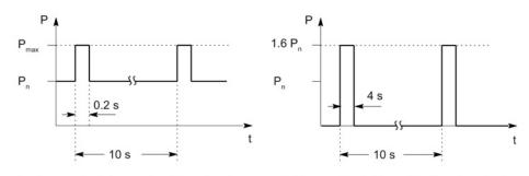
Peak power load duty cycle with pre-load condition
