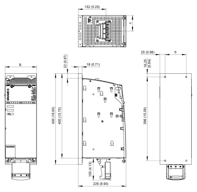
Figure 6-77 Dimension drawing of Motor Modules Booksize 45 A, 60 A, and 85 A with cold plate, all dimensions in mm and (inches); example for Motor Module 45 A
