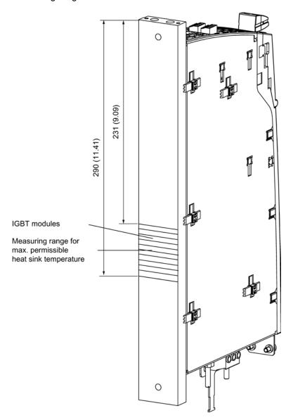
Figure 4-112 Measuring range for max. permissible heat-sink temperature for a Smart Line Module with cold plate
