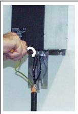
Attach the power cable. Tightening torque: 1.8 Nm
