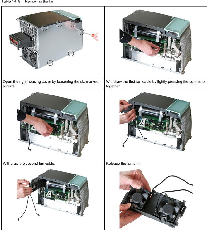
Completely remove the fan unit.
