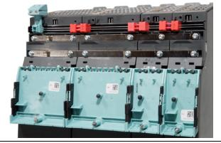
For 100 mm wide components, additionally attach the DC link busbars using the original M4x16 screws at the left-hand side of the component.
