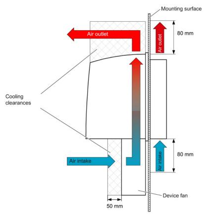
Figure 12-43 Cooling clearances for 300 mm wide components with external air cooling with mounted unit fan
