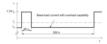
Figure 6-53 Duty cycle with 30 s overload for a duty cycle duration of 300 s
