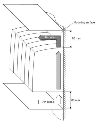
Figure 12-40 Cooling clearances for a drive line-up with internal air cooling (components up to 200 mm width)
