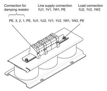
Figure 3-25 Interface overview, HFD line reactor 16 kW
