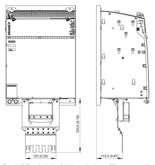
Figure 11-16 Dimension drawing of shield connecting plate on a 300 mm component with cold plate, all dimensions in mm and (inches)
