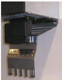
Installed shield connecting plate
