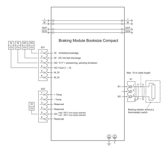
Figure 8-7 Connection example for Braking Module Booksize Compact and braking resistor without a thermostatic switch
