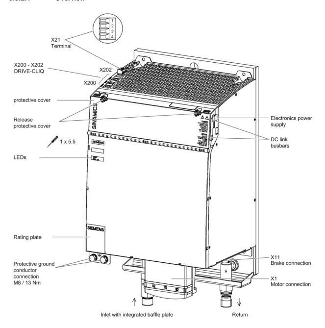
Figure 6-102 Interface overview, Motor Module Liquid Cooled (200 A)
