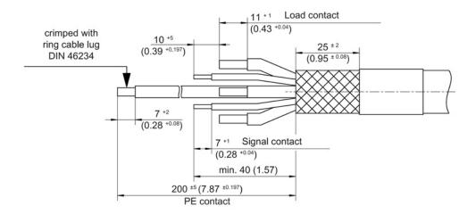
Figure 12-28 Stripped lengths for self-fabricated motor power cables, all data in mm and (inches)
