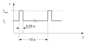
Figure 6-12 Duty cycle with initial load (for servo drives)
