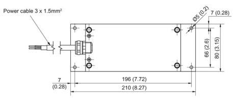
Figure 3-35 300 W damping resistor for HFD line reactors, all dimensions in mm and (inches)
