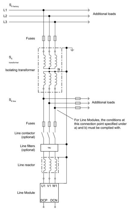
Figure 3-66 Operation of a Line Module and additional loads via an isolating transformer
