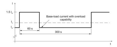
Figure 6-54 Duty cycle with 60 s overload for a duty cycle duration of 300 s
