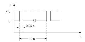
Figure 6-24 Duty cycle with initial load
