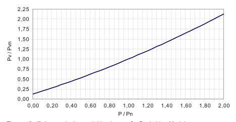
Figure 12-47 Losses in the partial load range for Basic Line Modules
