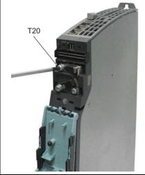
Remove the upper left-hand screw and the DC link bridge
