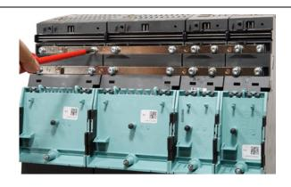
Remove the installed DC link bridges and busbars, starting at the second component.
