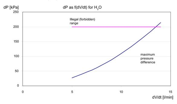
Figure 13-2 Pressure difference as a function of volumetric flow
