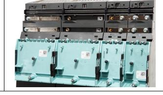
Remove the DC link busbar of the component.
