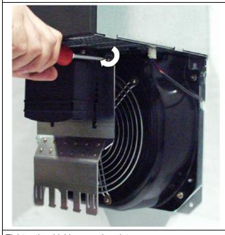
Tighten the shield connecting plate. Tightening torque: 3 Nm
