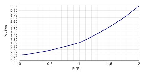
Figure 12-46 Losses in the partial load range for Active Line Modules and Smart Line Modules
