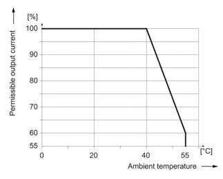
Figure 6-112 Output current as a function of the ambient temperature
