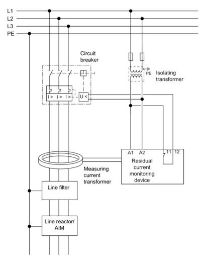
Figure 3-4 Connecting a differential current monitoring device
