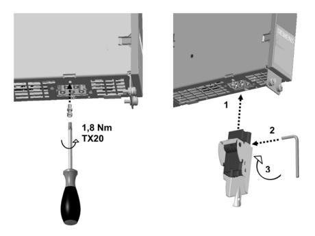
Figure 12-26 Installation example: Crimp plug
