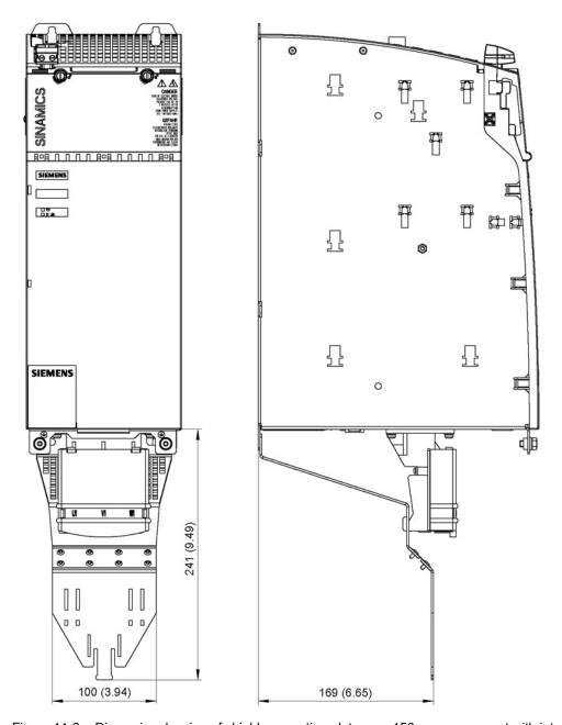
Figure 11-6 Dimension drawing of shield connecting plate on a 150 mm component with internal air cooling, all dimensions in mm and (inches)
