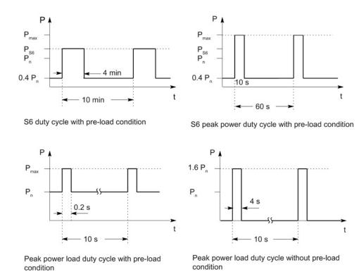
Figure 5-6 Rated duty cycles of Smart Line Modules
