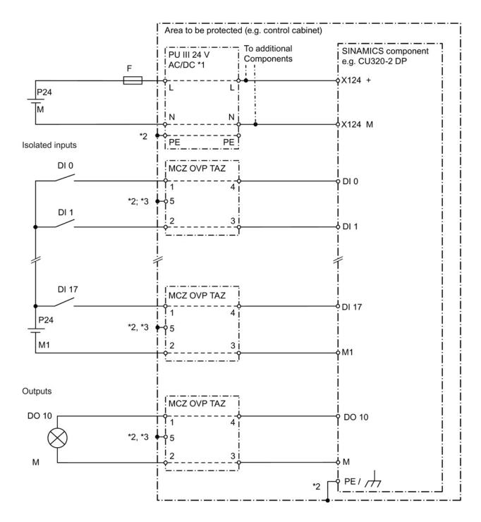
Figure 12-21 Connection example: Overvoltage protection components from Weidmüller connected to SINAMICS components
