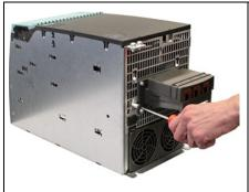
Remove the connection bracket to the noise suppression capacitor using a Tx25 screwdriver.
