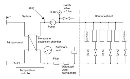
Figure 13-4 Water-to-water heat exchanger
