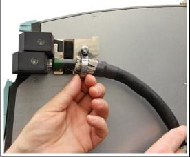
3. Slide the cable clamp onto the tongue, and then insert the end of the cable into the DCN connection of the DC link adapter.
