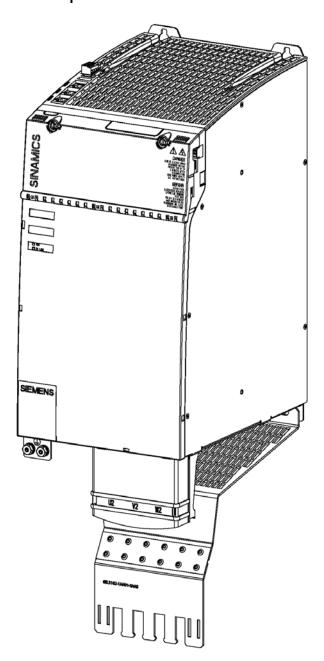
Figure 11-1 Shield connecting plate for a 200 mm module with internal air cooling
