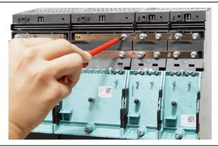
Loosen the screws and remove the installed DC link bridge of the component.
