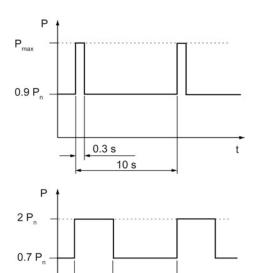
Figure 4-69 Duty cycles with initial load
