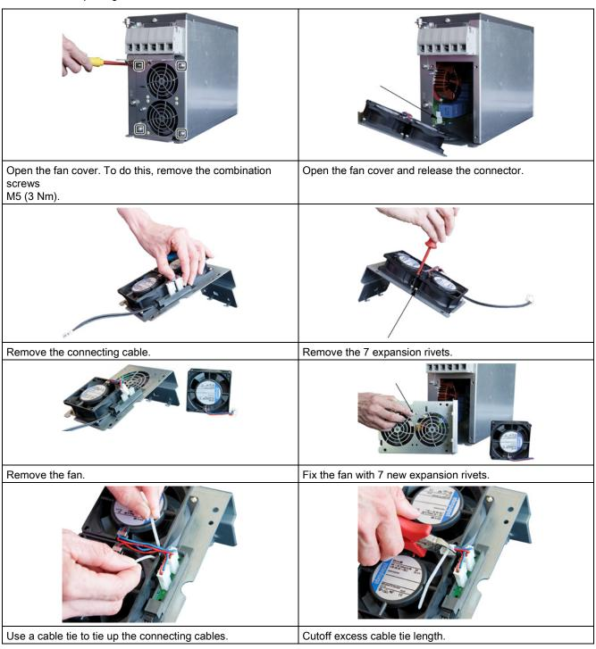
Table 14-6 Replacing the fan in an Active Interface Module, 55 kW
