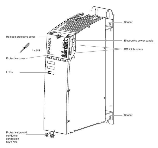
Figure 8-17 Interface overview, Capacitor Module
