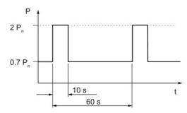
Figure 4-57 Duty cycle with pre-load condition for 20 kW and 40 kW Basic Line Modules
