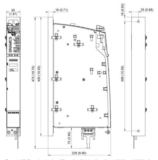
Figure 4-107 Dimension drawing of Smart Line Module with cold plate (5 kW and 10 kW), all dimensions in mm and (inches)
