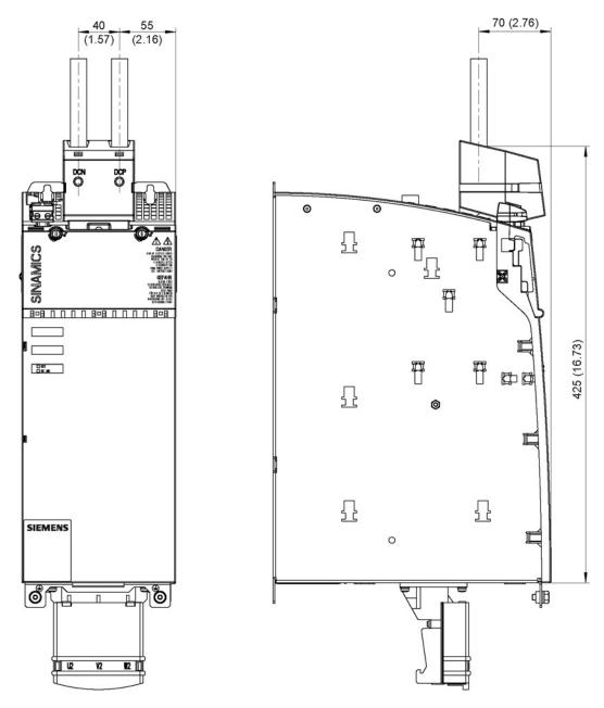
Figure 11-25 Dimension drawing of 150 mm wide component with DC link rectifier adapter for 35 to 95 mm², all dimensions in mm and (inch)
