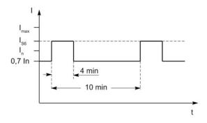
Figure 6-14 S6 duty cycle with initial load with a duty cycle duration of 600 s (for servo drives)
