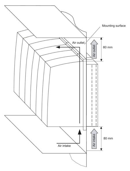
Figure 12-42 Cooling clearances for a drive line-up with external air cooling (components up to 200 mm width)
