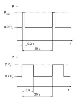
Figure 4-55 Duty cycles with initial load
