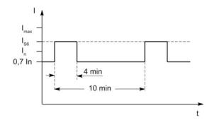
Figure 6-51 S6 duty cycle with initial load with a duty cycle duration of 600 s (for servo drives)
