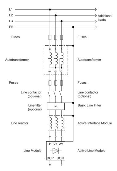
Figure 3-67 Operation of a Line Module via an autotransformer
