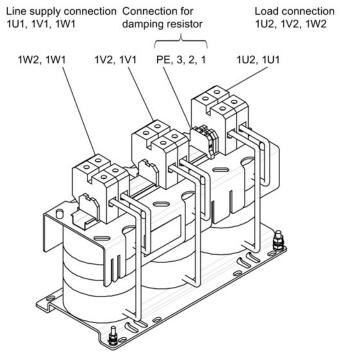
Figure 3-28 Interface overview, HFD line reactor 80 kW
