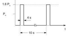
Peak power load duty cycle with pre-load condition
