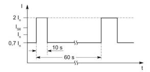
Figure 6-27 S6 duty cycle with initial load for a duty cycle duration of 60 s
