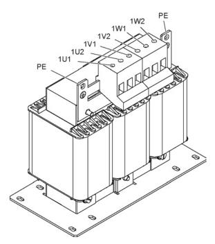
Figure 3-39 Interface overview, line reactor for Basic Line Modules (20 kW)
