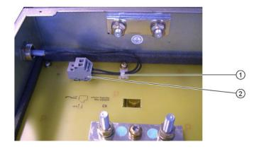
Figure 10-15 Connection of the signaling contact using the VPM200 as an example
