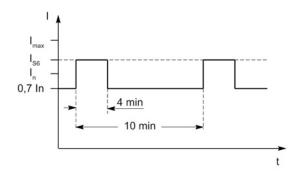
Figure 6-63 S6 duty cycle with initial load for a duty cycle duration of 600 s
