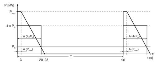
Figure 8-13 Duty cycles for braking resistors with a thermostatic switch
