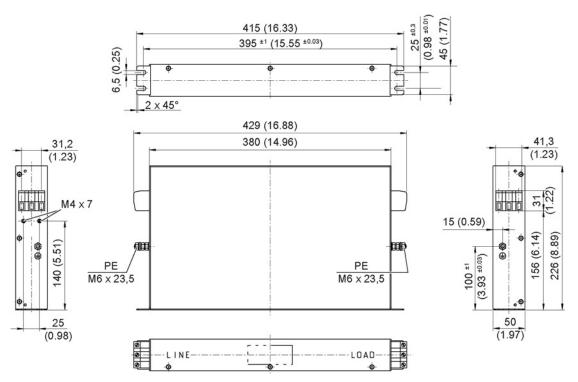
Figure 3-17 Dimension drawing of Basic Line Filter for Basic Line Modules 20 kW, all data in mm and (inches)
