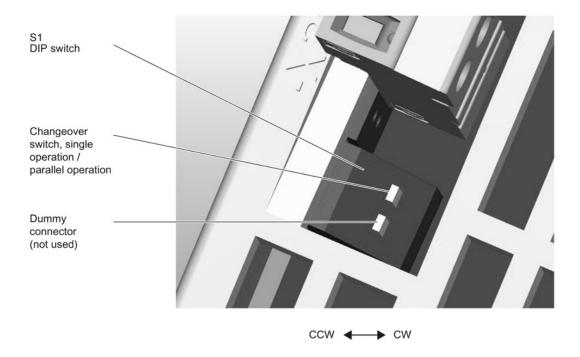
Figure 8-21 DIP switch on the upper side of the component
