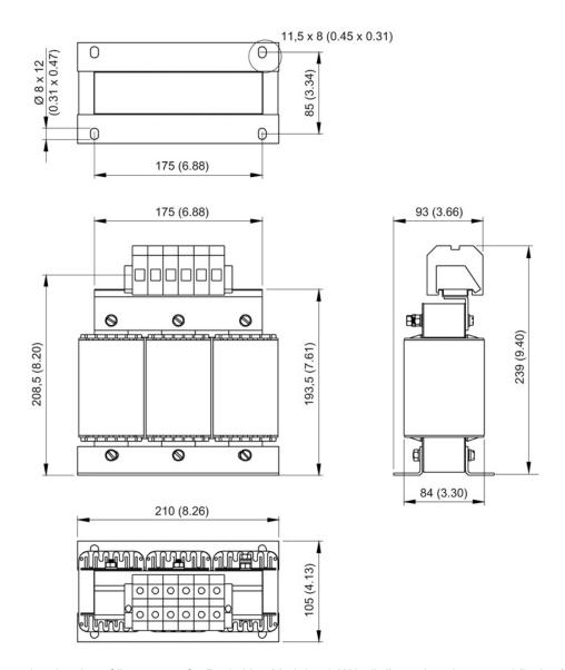
Figure 3-43 Dimension drawing of line reactor for Basic Line Module 40 kW, all dimensions in mm and (inches)
