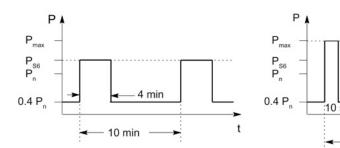
S6 peak power duty cycle with pre-load condition
