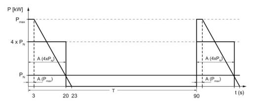
Figure 9-9 Duty cycles for braking resistors with a thermostatic switch
