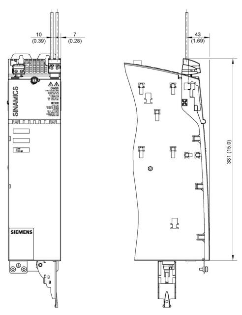
Figure 11-24 Dimension drawing of 100 mm wide component with DC link rectifier adapter for 0.5 to 10 mm², all dimensions in mm and (inch)
