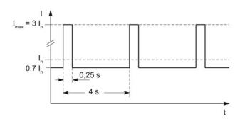
Figure 7-13 Peak current duty cycle with initial load
