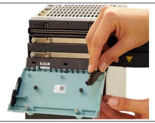
Remove the DC-link side cover, install the 24 V terminal adapter (if required) and close the protective cover until it audibly clicks into place.
