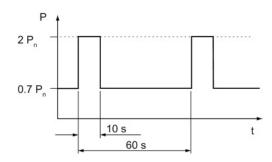
Figure 4-71 Duty cycle with pre-load condition for 20 kW and 40 kW Basic Line Modules
