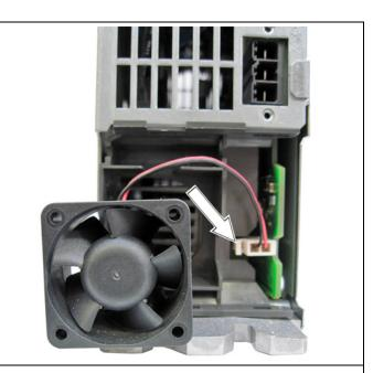
• Release the connector and remove the connecting cable.
