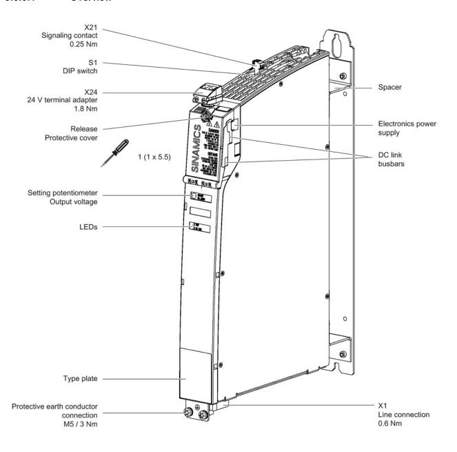
Figure 8-20 Interface overview, Control Supply Module
