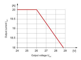
Figure 8-29  $\,$  Current derating for ambient temperatures >40  $\,^{\circ}$ C as a function of the output voltage
