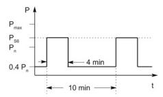
Figure 4-56 S6 duty cycle with pre-load condition
