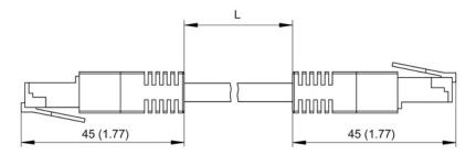
Figure 12-22 DRIVE-CLiQ signal cables without 24 V DC cores (IP20)
