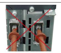
**WRONG**: Measurement via the device sockets
