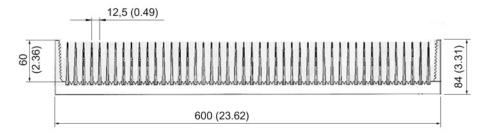
Figure 12-37 External air heat sink, all data in mm and (inches); height: 500 mm (19.69 inch)
