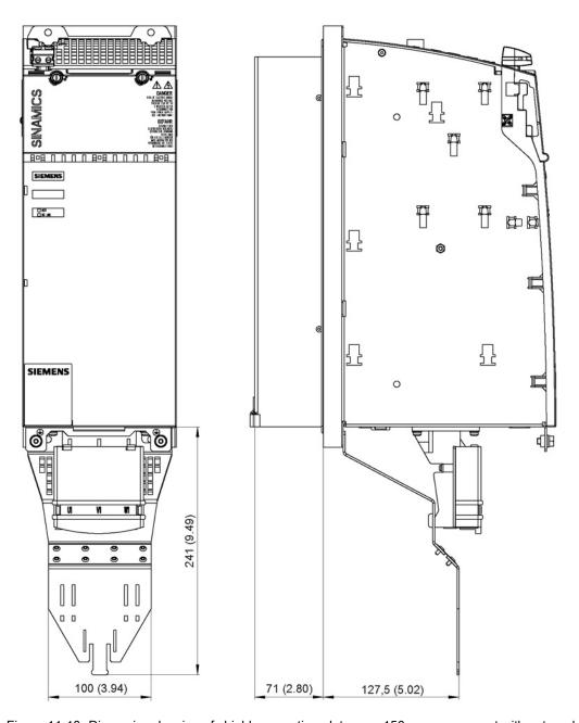
Figure 11-10 Dimension drawing of shield connecting plate on a 150 mm component with external air cooling, all dimensions in mm and (inches)
