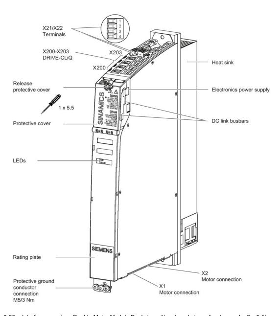
$Figure \ 6-35 \quad Interface \ overview, \ Double \ Motor \ Module \ Booksize \ with \ external \ air \ cooling \ (example: 2 \ x \ 5 \ A)$
