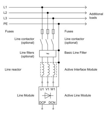
Figure 3-65 Direct operation on the line supply
