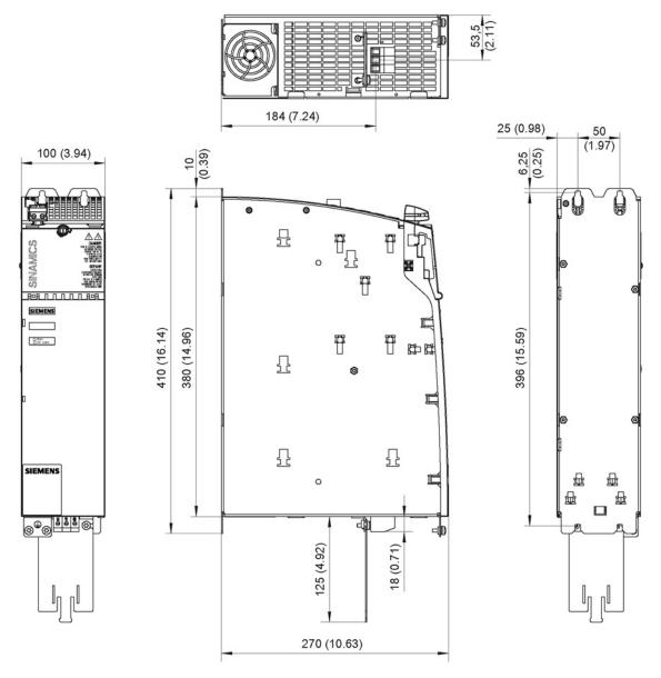
Figure 4-3 Dimension drawing of 16 kW Active Line Module with internal air cooling, all dimensions in mm and (inches)
