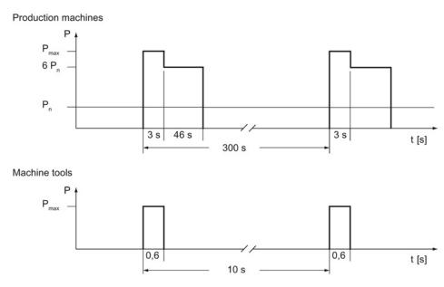
Figure 4-72 Braking duty cycle for Basic Line Modules
