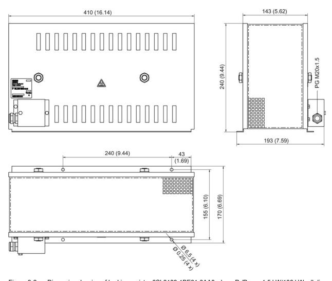
Figure 9-2 Dimension drawing of braking resistor 6SL3100-1BE31-0AA0 where P<sub>n</sub>/P<sub>max</sub> = 1.5 kW/100 kW, all dimensions in mm and (inches)
