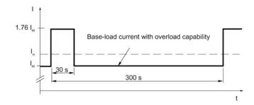
Figure 6-97 Duty cycle with 30 s overload for a duty cycle duration of 300 s
