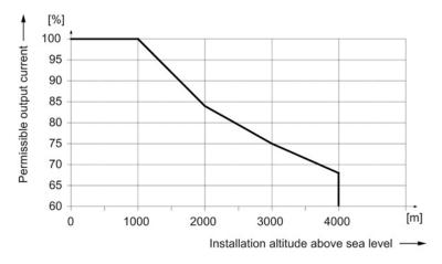
Figure 4-29 Output current as a function of the installation altitude
