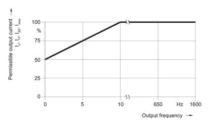
Figure 6-22 Output current as a function of the output frequency
