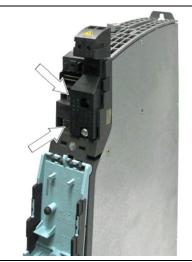
Do **NOT** use the screw holes at the left-hand side of the component.
