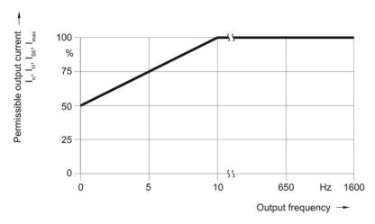
Figure 6-101 Output current as a function of the output frequency
