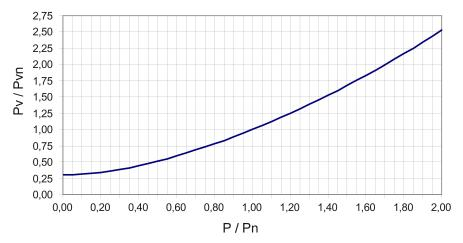
Figure 12-50 Losses in the partial load range for line reactors for Smart Line Modules
