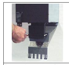
Release and open the cover of the terminal strip.
