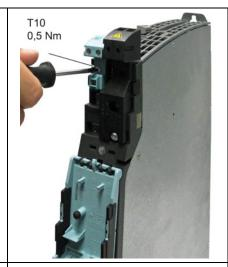
Attach and screw on the 24 V terminal adapter using the associated screw (provided in the accessories pack).
