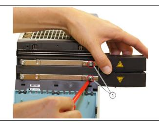
Attach the DC-link adapter (1.8 Nm) with the DC-link screws that were previously removed<sup>1)</sup>.
