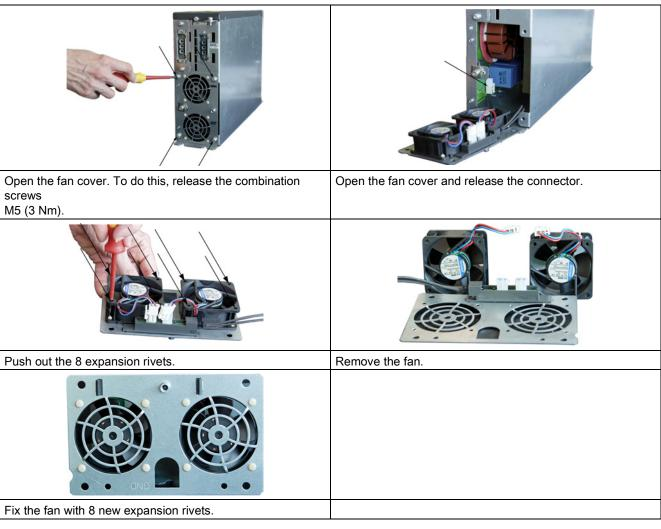
To install, carry out the above steps in reverse order. The torques must be carefully observed.
