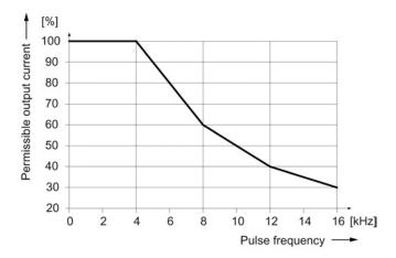
Figure 6-114 Output current as a function of the pulse frequency
