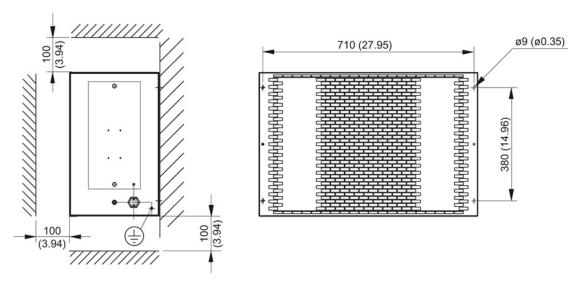
Figure 9-7 Installation drawing (wall mounting) of braking resistor 6SE7028-0ES87-2DC0 where  $P_n/P_{max}$  = 12.5 kW/75 kW, all dimensions in mm and (inches)
