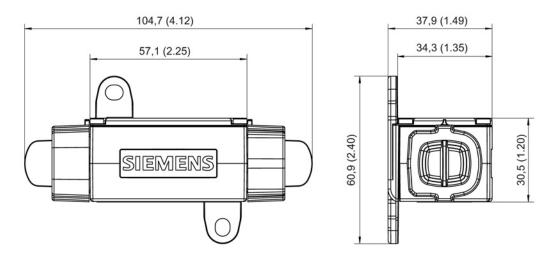
Figure 11-41 Dimension drawing of the DRIVE-CLiQ coupling, all dimensions in mm and (inches)
