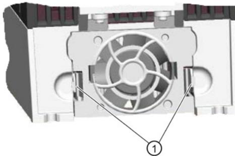
Figure 11-1 Fan replacement PM240-2, frame size FSB
