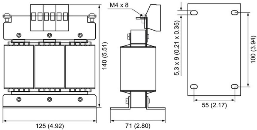
Figure 3-10 Dimensional drawing of line reactors, PM240-2 frame size FSA, 1.5 ... 4.0 kW, all dimensions in mm and (inch)
