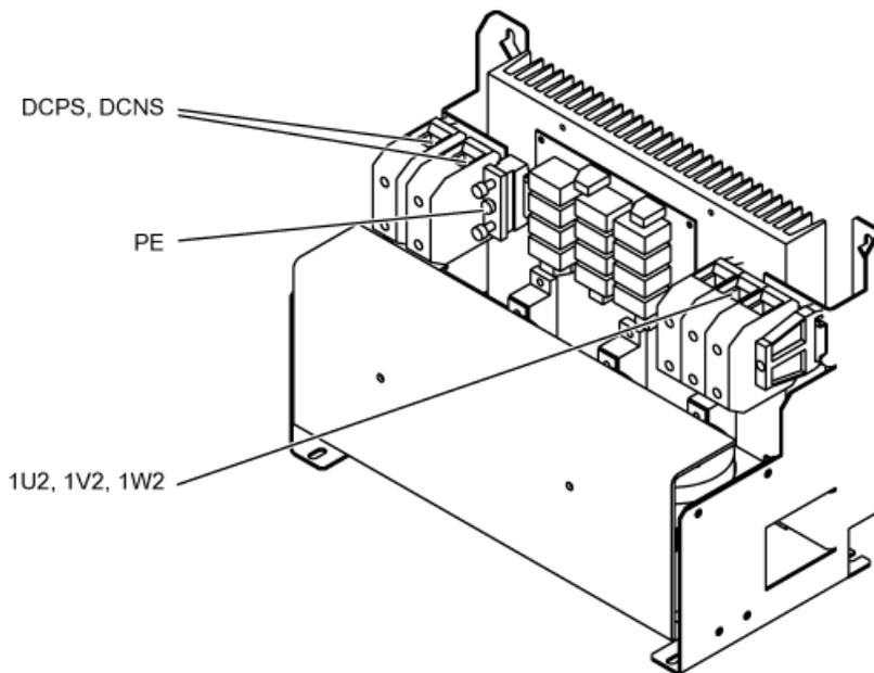
Figure 6-17 Interface overview, Voltage Peak Limiter, type 2
