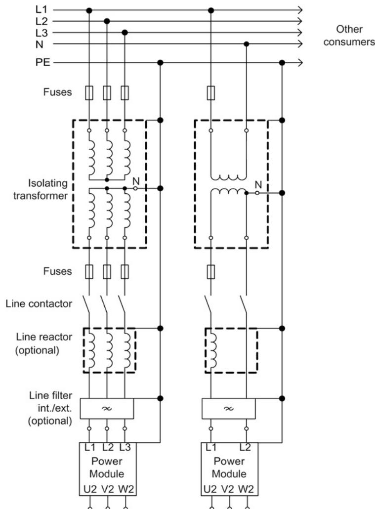
Figure 3-33 Isolating transformer
