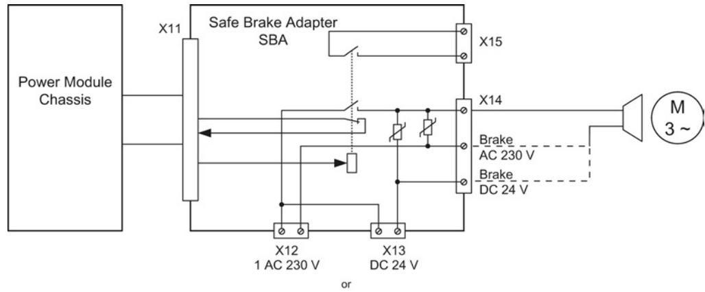
Figure 8-26 Connection example for a Safe Brake Adapter
