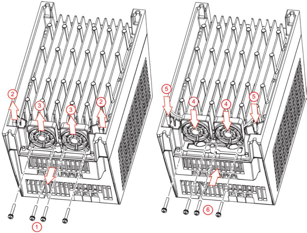
Figure 11-3 PM340 fan replacement, frame size FSB/FSC (0.4 Nm tightening torque)
