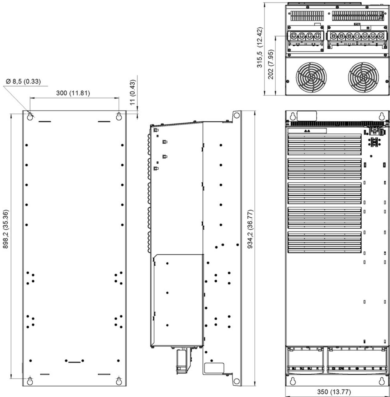
Figure 4-43 Dimension drawing, PM340 Power Module, frame size FSF (with integrated line filter); all dimensions in mm and (inches)
