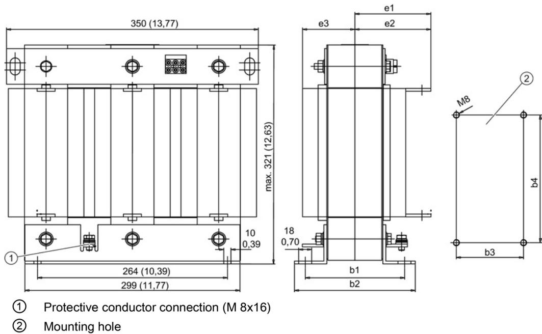
Figure 6-8 Dimension drawing motor reactor, PM340 frame size FSF
