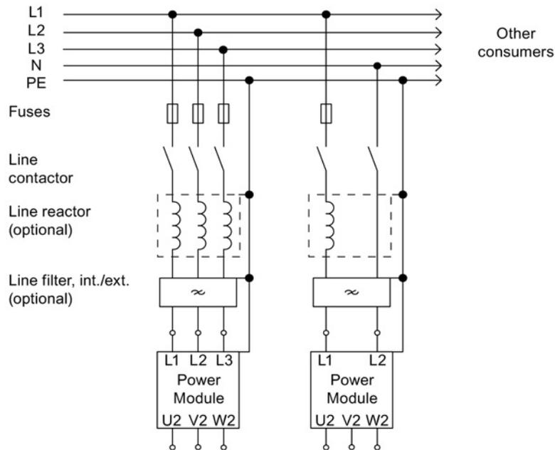
Figure 3-30 Direct operation on the line supply
