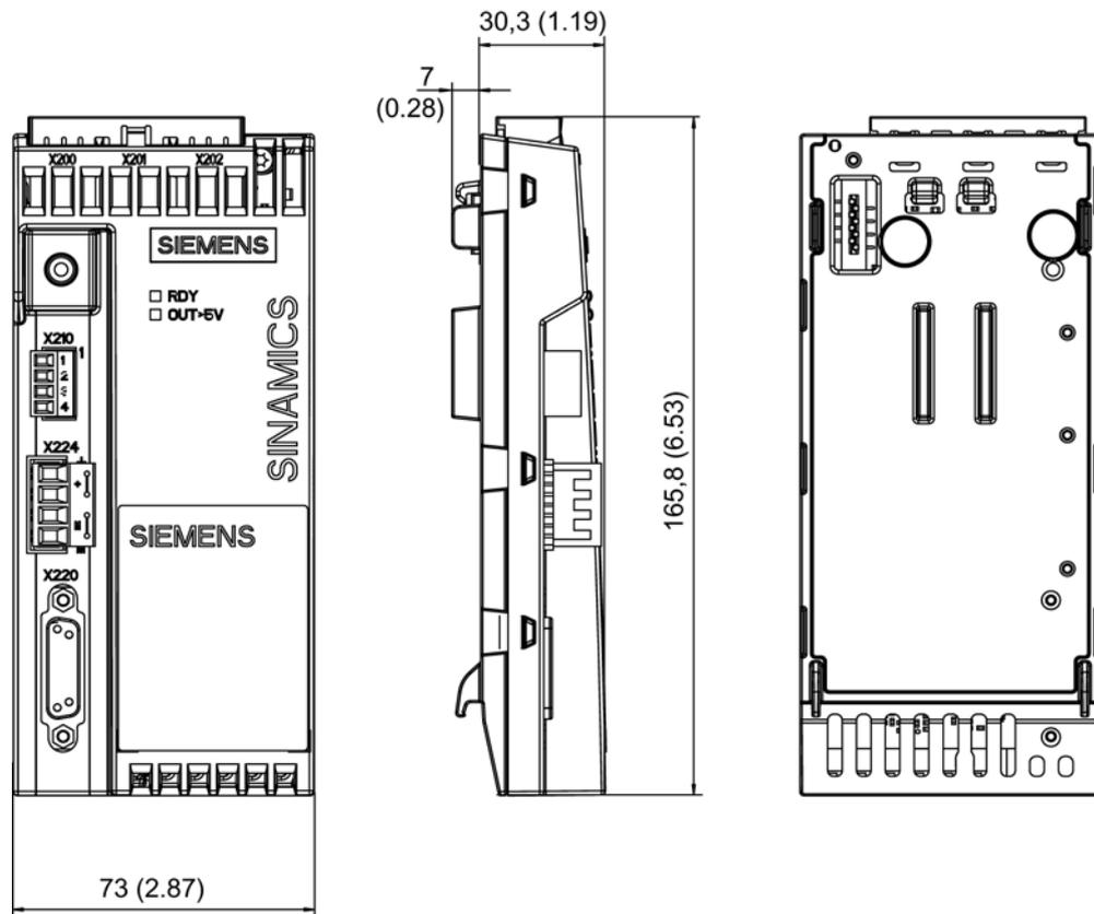
Figure 7-21 Dimension drawing of Control Unit Adapter CUA32, all data in mm and (inches)
