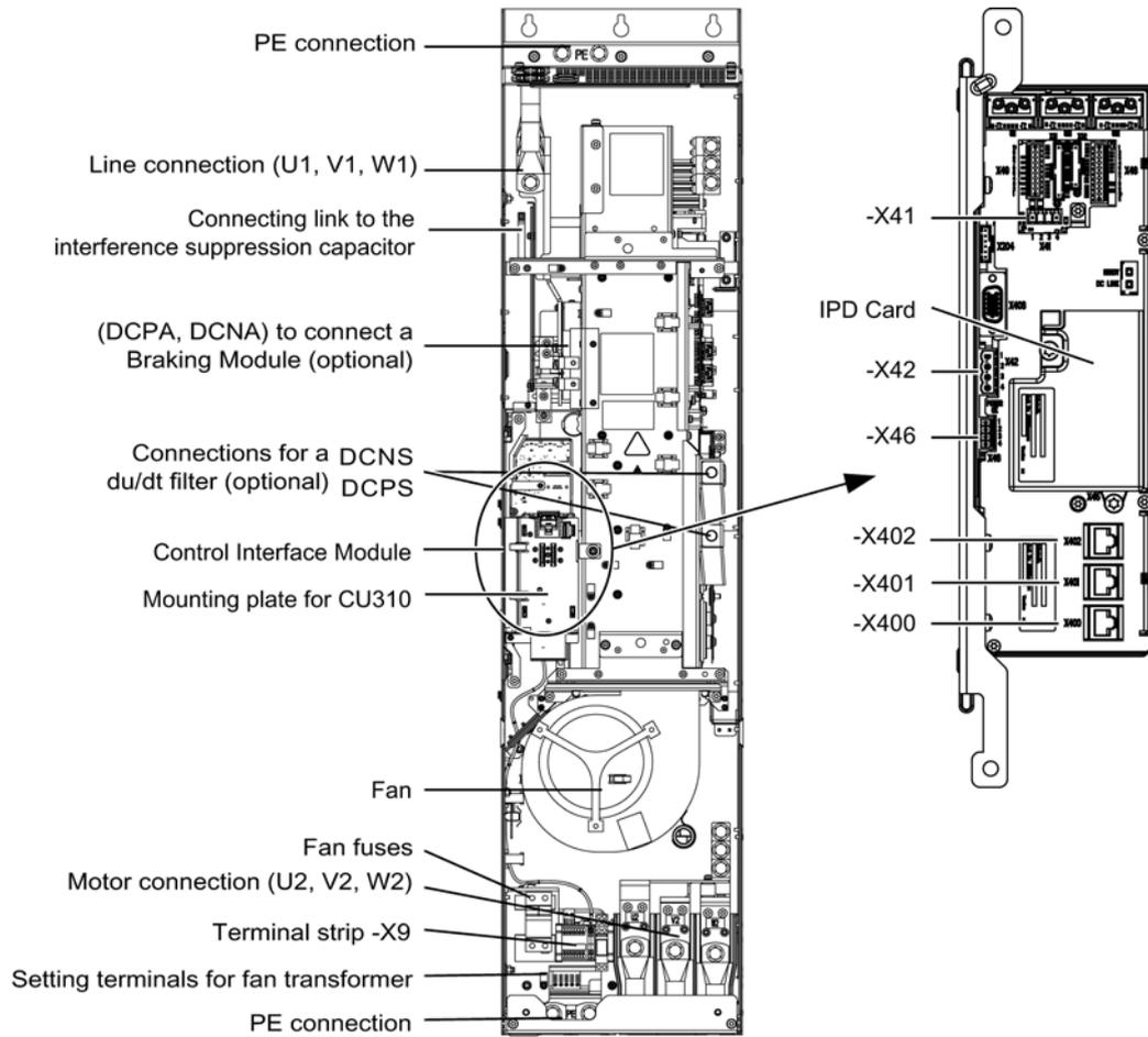
Figure 4-57 Power Module, frame size FX
