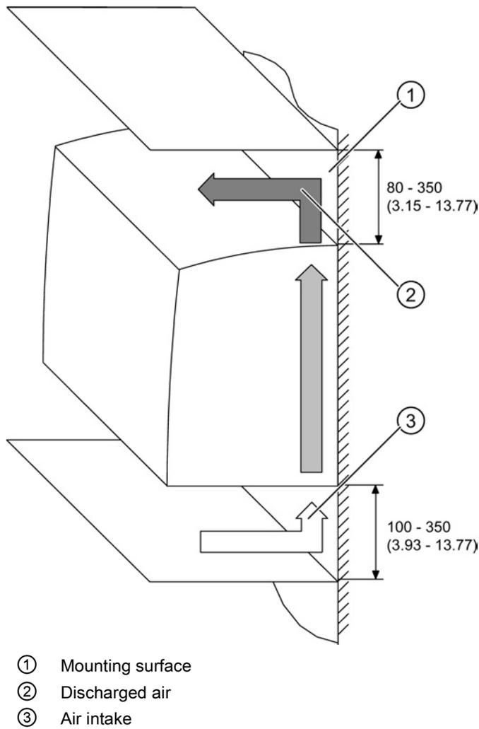
Figure 10-6 Ventilation clearances
