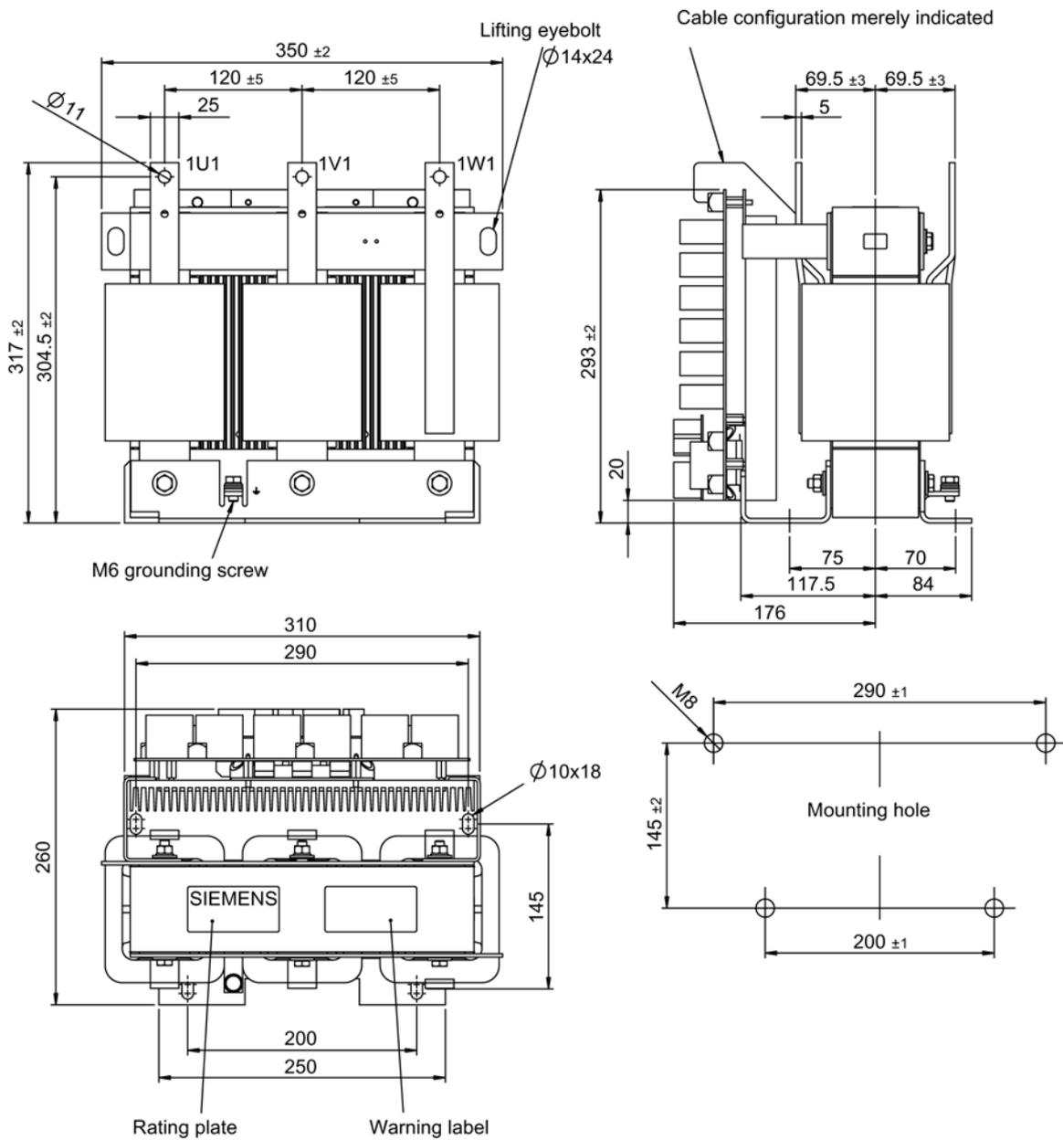
Figure 6-26 Dimension drawing of dV/dt filter compact plus Voltage Peak Limiter, type 2
