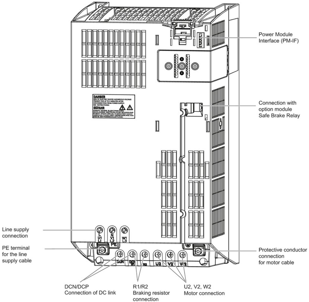
Figure 4-30 PM340, frame size FSC
