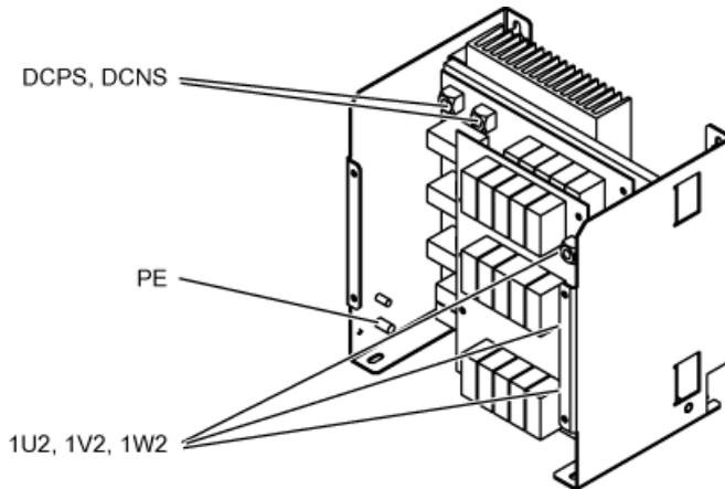
Figure 6-16 Interface overview, Voltage Peak Limiter, type 1
