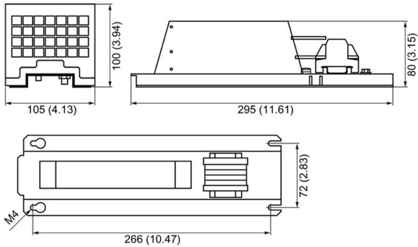
Figure 5-2 Dimension drawing of braking resistor for PM240-2, frame size FSA, 0.55 ... 1.5 kW, all dimensions in mm and (inch)
