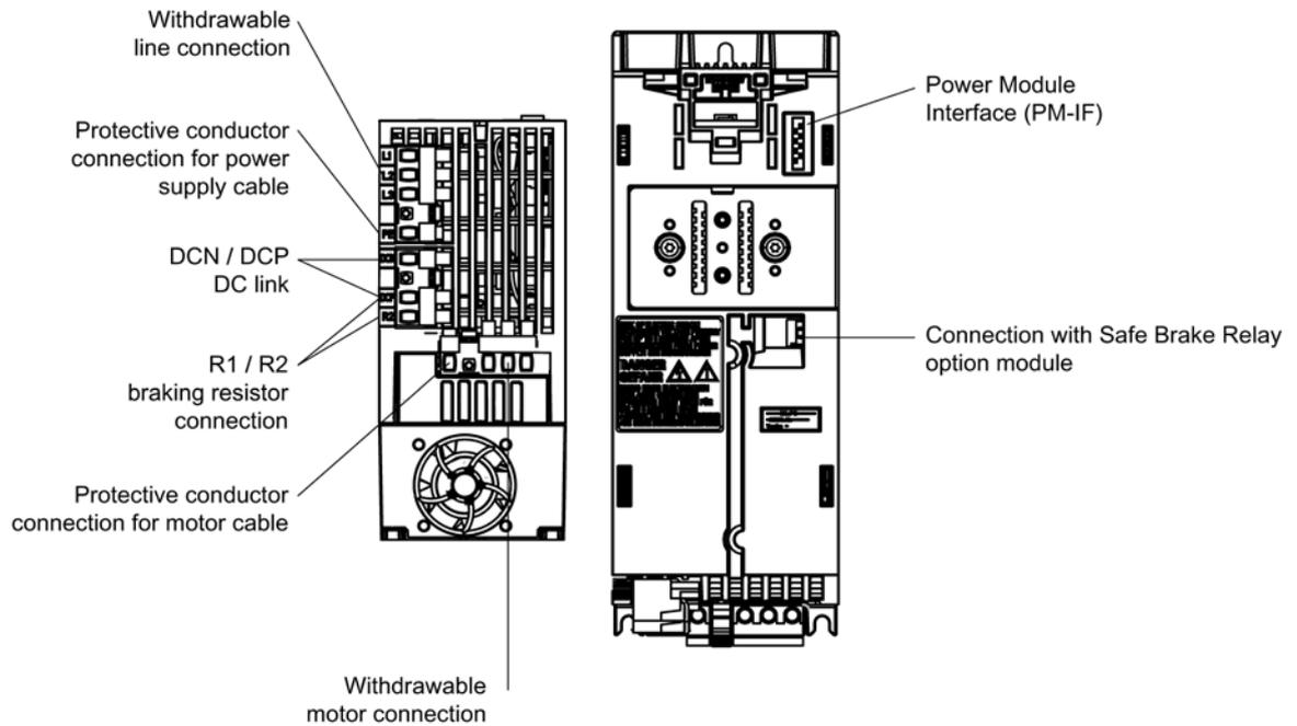
Figure 4-1 PM240-2, frame size FSA (view from below and front)
