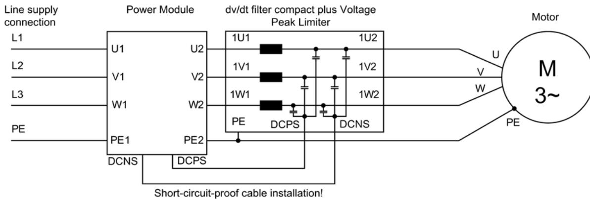
Figure 6-24 Connecting the dV/dt filter compact plus Voltage Peak Limiter
