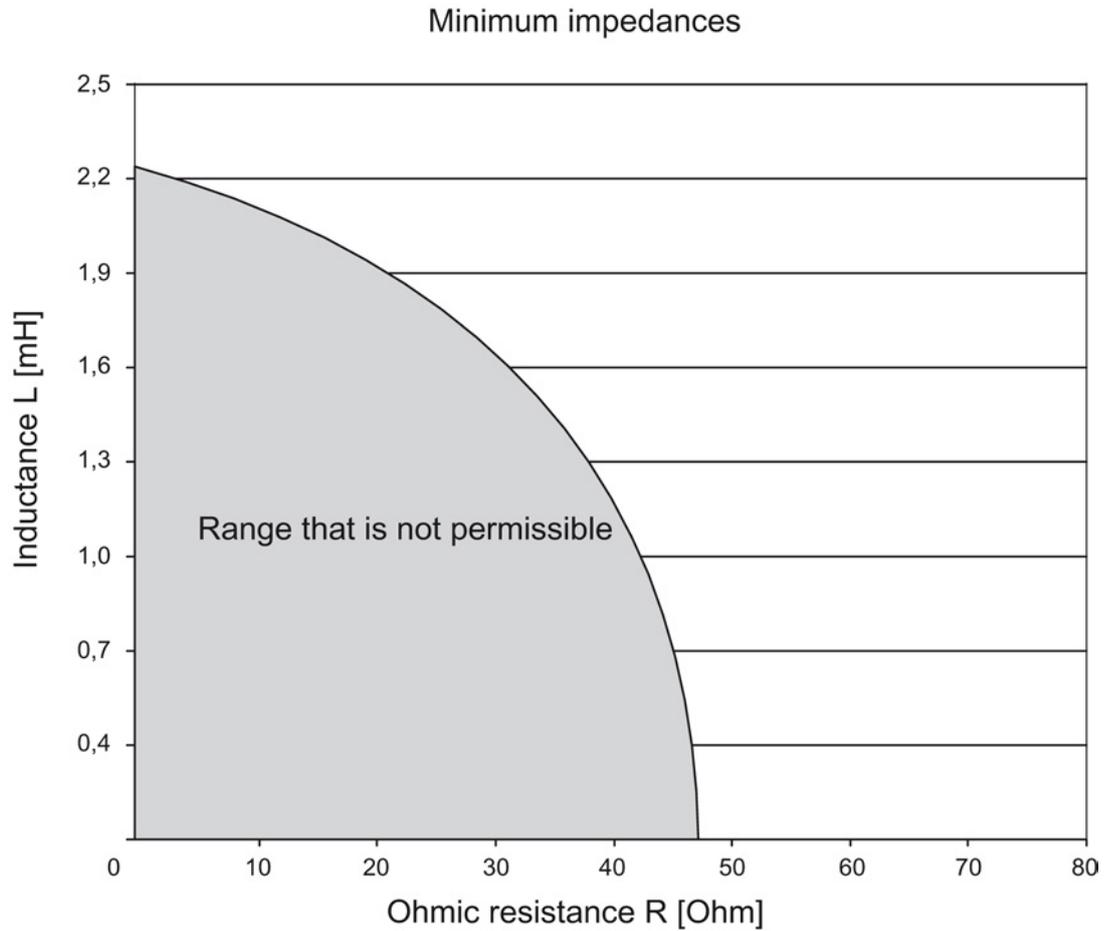
Figure 8-4 Connectable impedances with an excitation frequency  $f = 5000$  Hz
