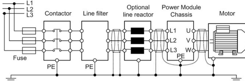
Figure 3-2 Example of a chassis line connection
