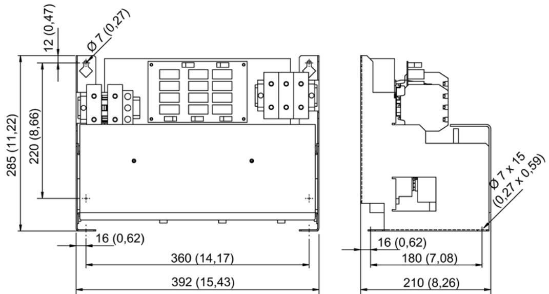
Figure 6-21 Dimension drawing of the Voltage Peak Limiter, type 2
