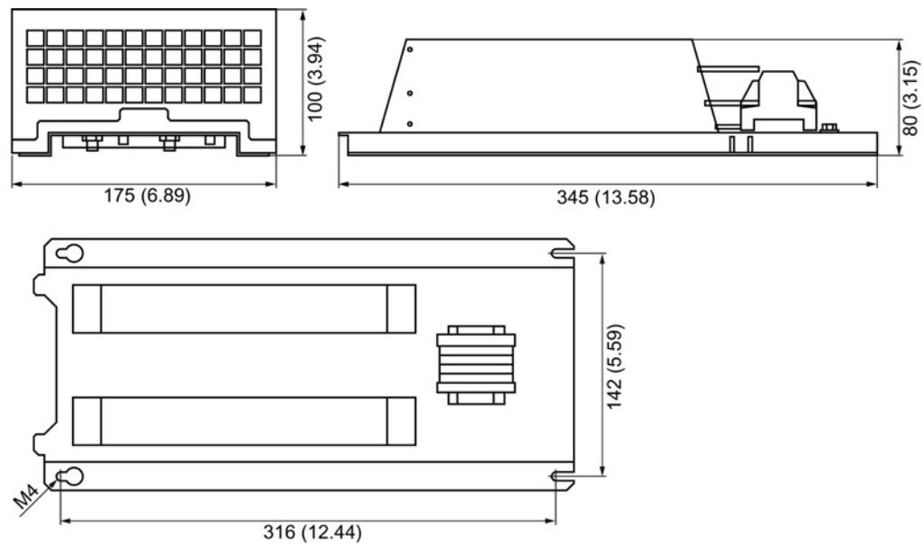
Figure 5-4 Dimension drawing braking resistor for PM240-2, frame size FSB, all data in mm (inches)
