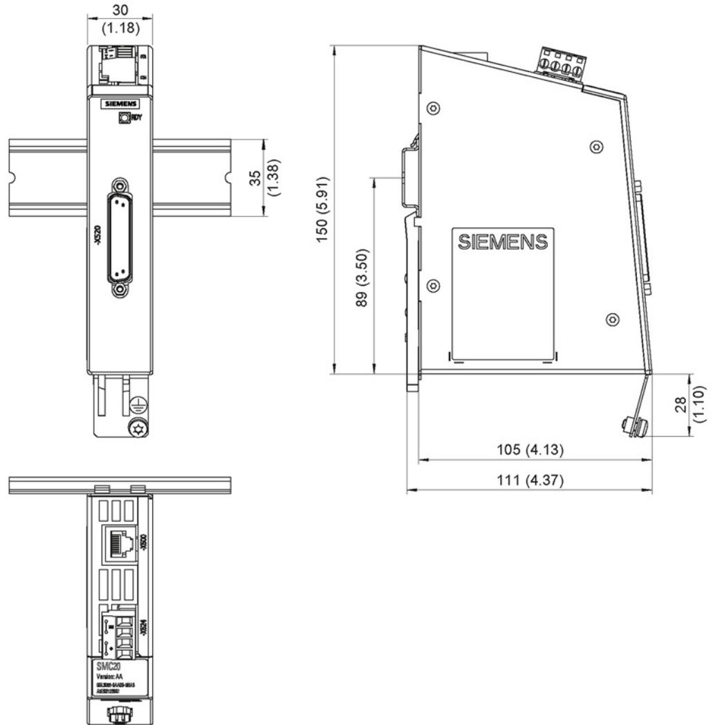
Figure 8-6 Dimension drawing of the Sensor Module Cabinet SMC20, all data in mm and (inches)
