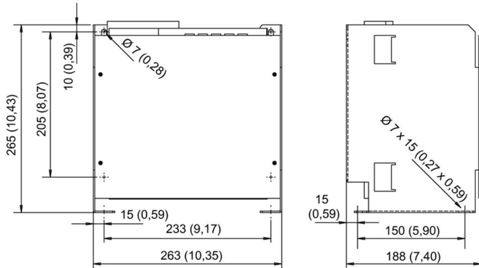
Figure 6-20 Dimension drawing of the Voltage Peak Limiter, type 1
