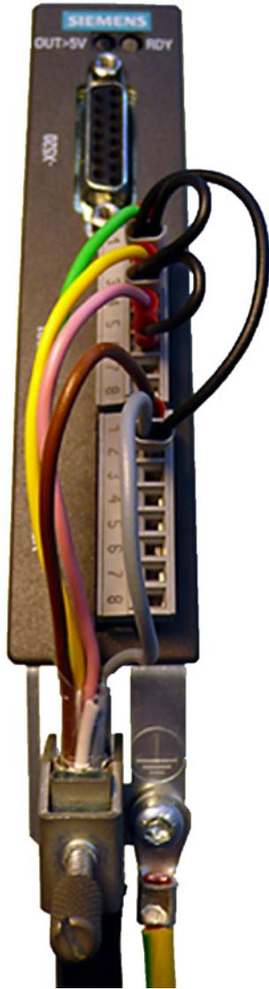
Figure 8-12 Photo of connection example 2: SMC30, 30 mm wide
