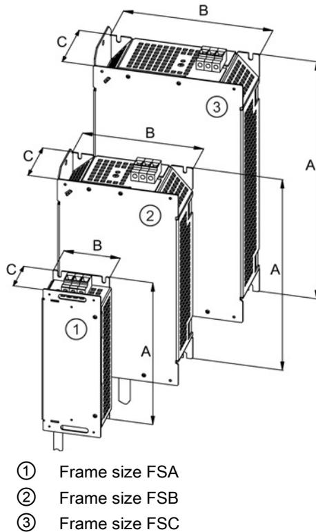
Figure 3-13 Dimension drawing of line reactors, PM340 frame sizes FSA, FSB, FSC
