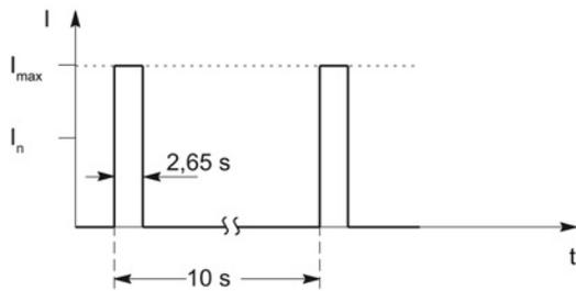
Figure 4-46 Duty cycle without initial load (for servo drives)
