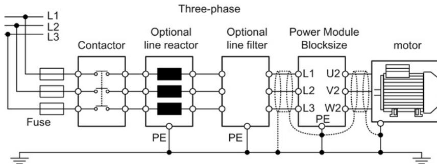
Figure 3-1 Example of a Blocksize line connection
