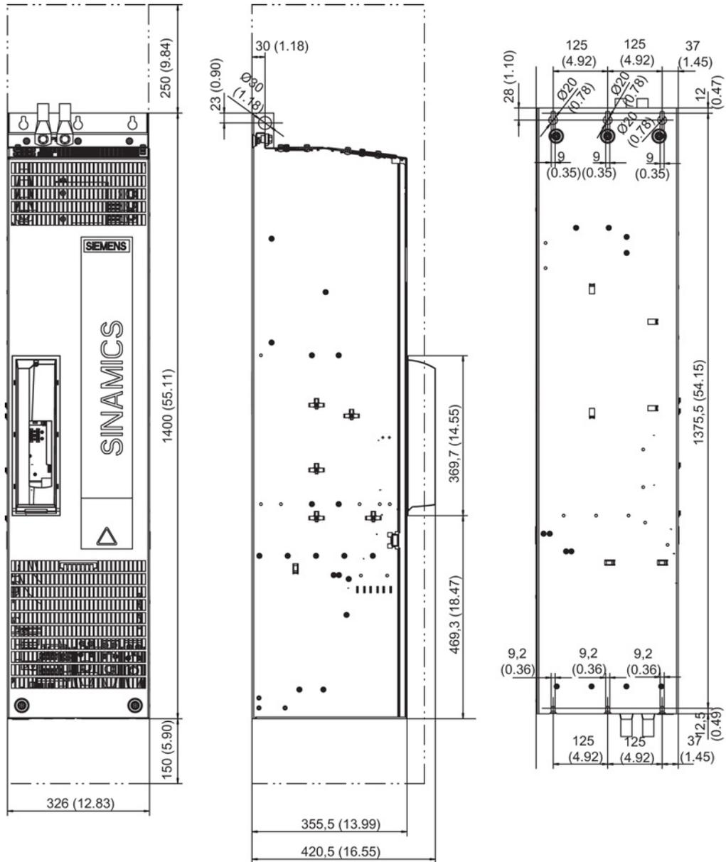
Figure 4-60 Dimension drawing Power Module, frame size FX
