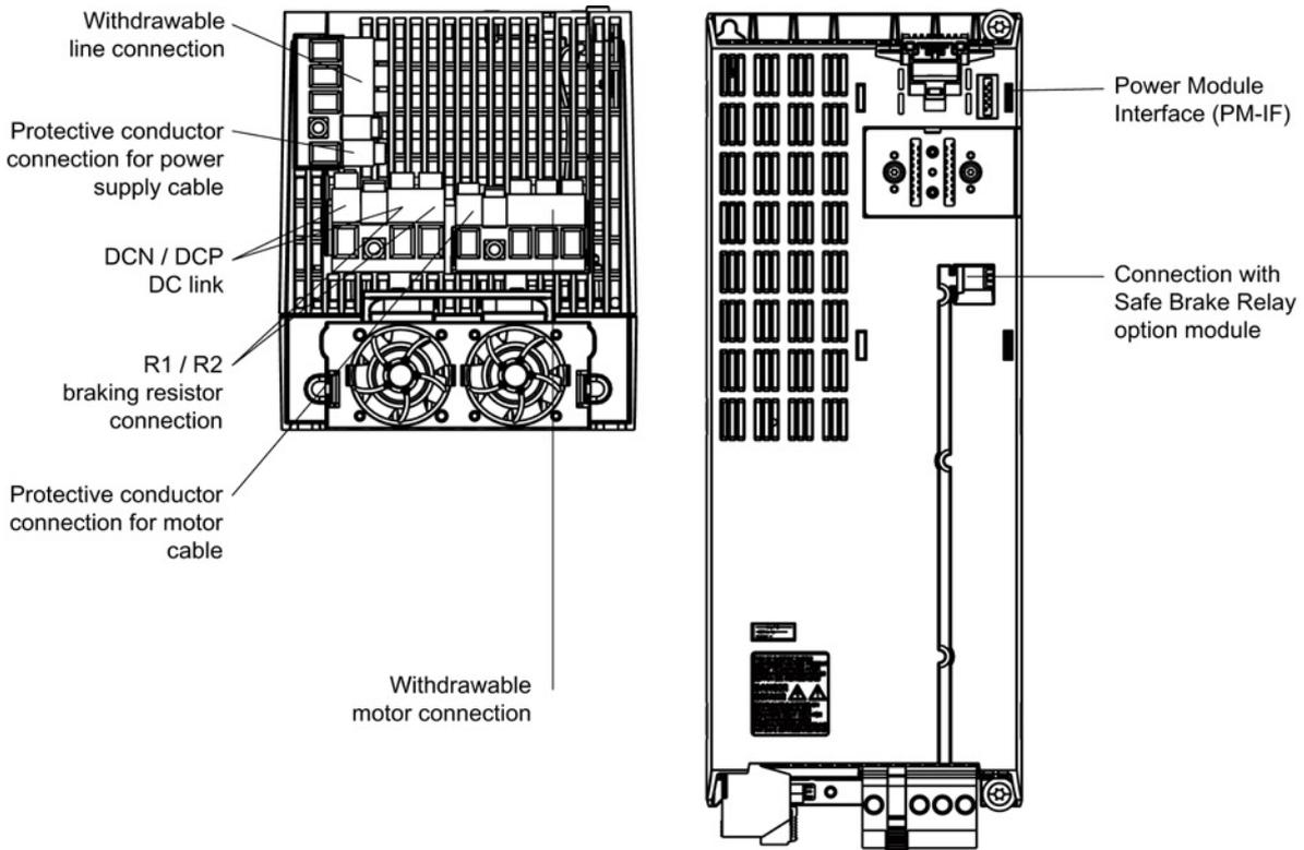
Figure 4-3 PM240-2, frame size FSB (view from below and front)
