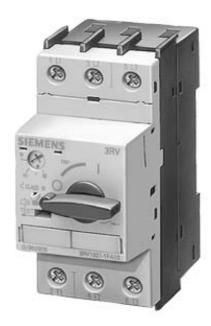
CIRCUIT-BREAKER SIZE S0, FOR MOTOR PROTECTION, CLASS 10, A-REL.4.5A...6.3A, N-REL.82A, SCREW TERMINAL, STANDARD SWITCHING CAPACITY
