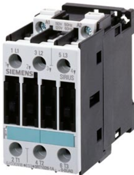
CONTACTOR, AC-3 11 KW/400 V, DC 24 V, 3-POLE, SIZE S0, SCREW CONNECTION
