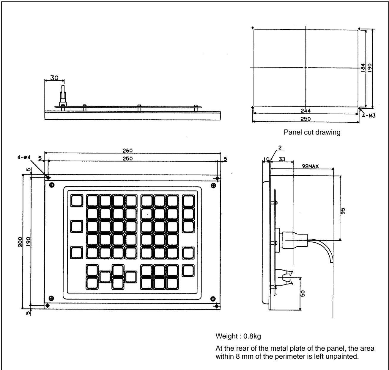
**Fig.U29 Separate type MDI unit (full-key) (for 7.2" LCD/8.4" LCD)**
