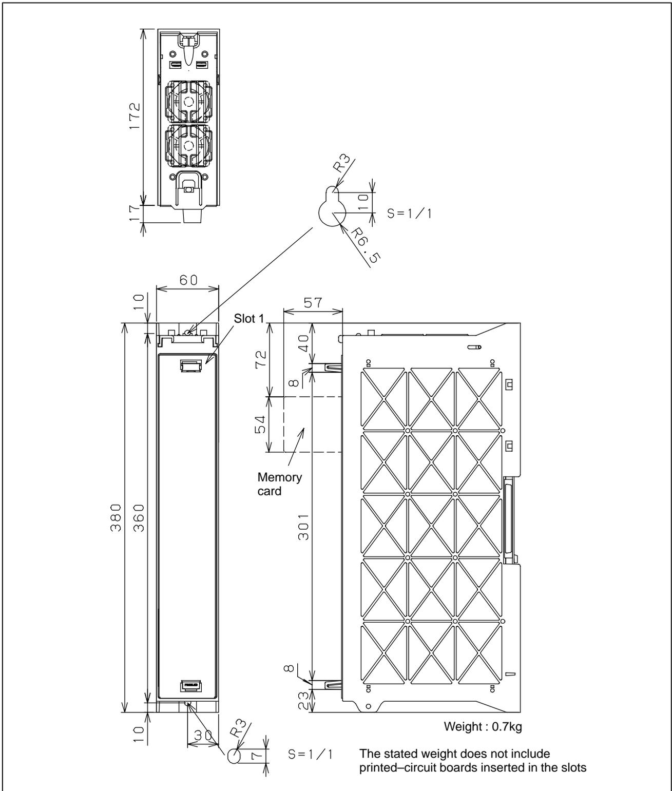
**Fig.U1 Series 0i Mate-B basic unit (1-slot)**
