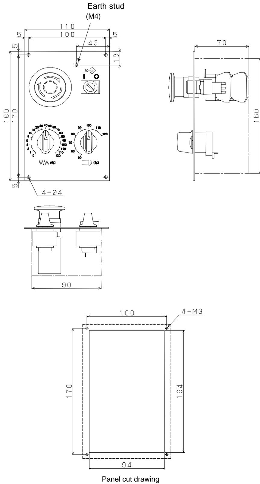
Fig.U27 Machine operator's panel (Sub panel B1)
