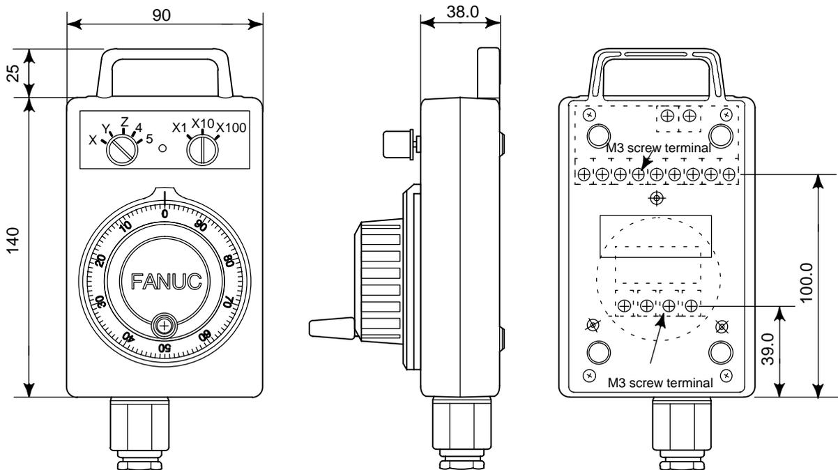
Fig.U19 Pendant type manual pulse generator
