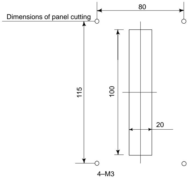
**Fig.U23 Punch panel (wide width type)**
