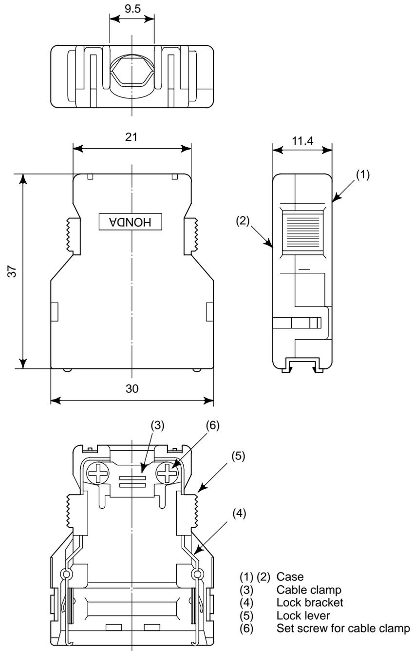
Fig.C2 (a) Connector case (HONDA PCR type)
