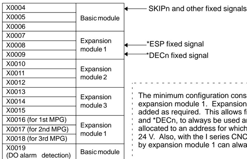
The minimum configuration consists of the basic module and expansion module 1. Expansion modules 2 and 3 may be added as required. This allows fixed signals, such as SKIPn and \*DECn, to always be used and the \*ESP fixed signal to be allocated to an address for which the common voltage is fixed to 24 V. Also, with the I series CNC, the MPG interface provided by expansion module 1 can always be used.
