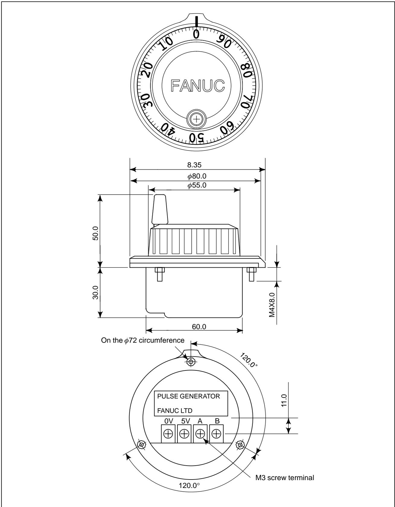
**Fig.U18 Manual pulse generator**
