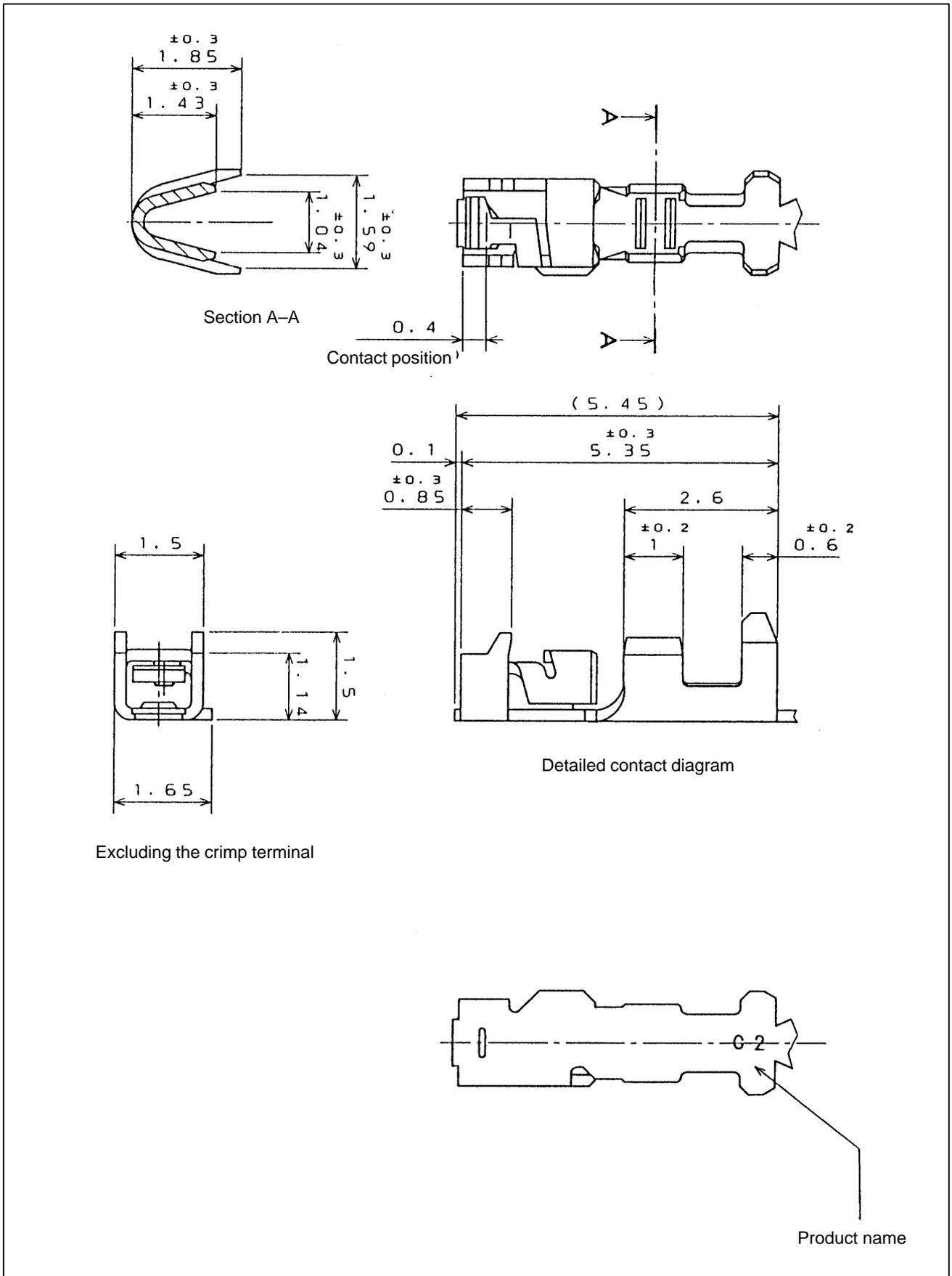
Fig.C7 (b) Contact (Japan Aviation Electronics)(for MDI)
