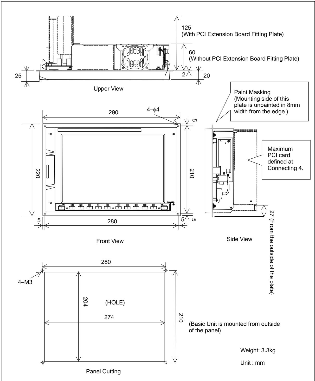
Fig.U10 (a) 10.4" TFT color LCD of CNC display unit with PC functions
