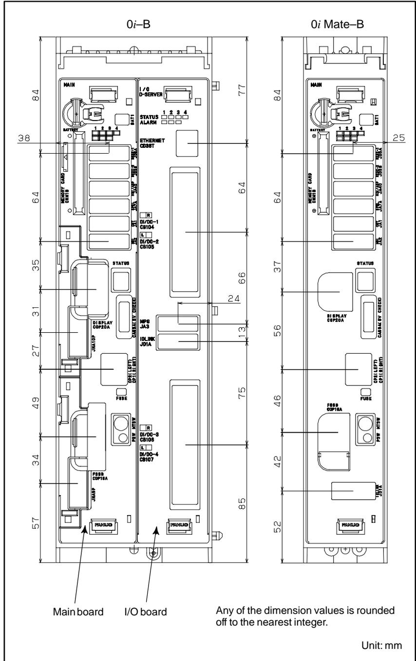
Fig.3.7 (a) Grid of connector location
