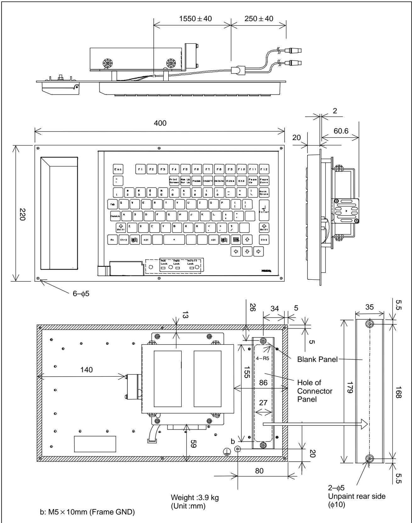
Fig.U12 (c) FA Full Keyboard 15.0" LCD Type
