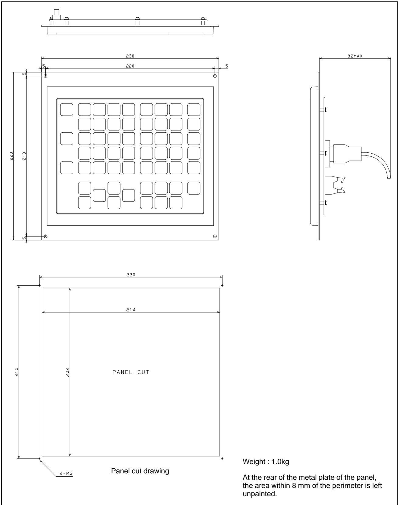
**Fig.U30 Separate type MDI unit (full-key)**
