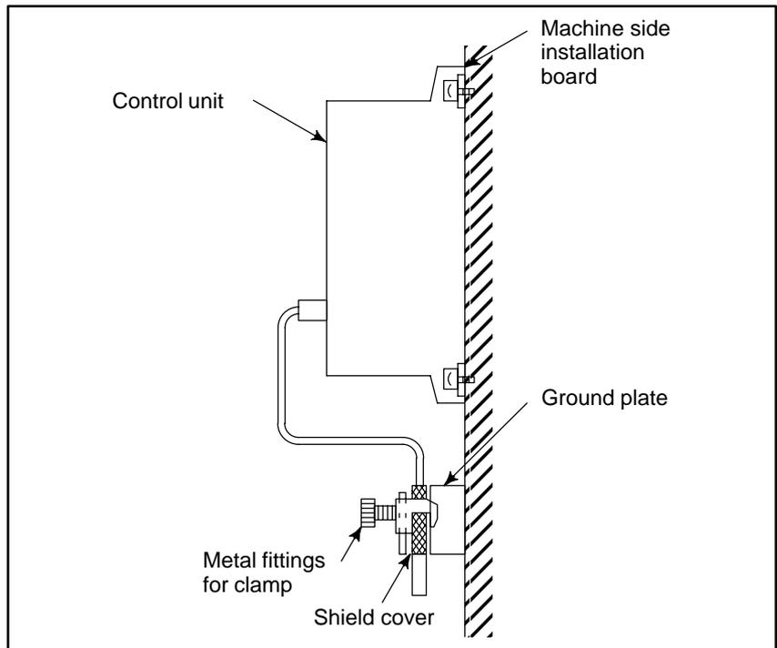
**Fig.3.5.5(b) Cable clamp (2)**
