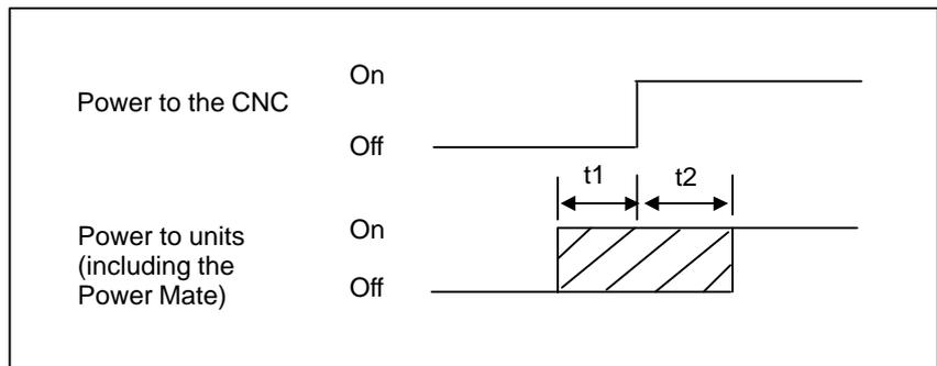
t1 : 200 ms Means that the power to units (including the Power Mate) is turned on within 200 ms before the power to the CNC is turned on.
