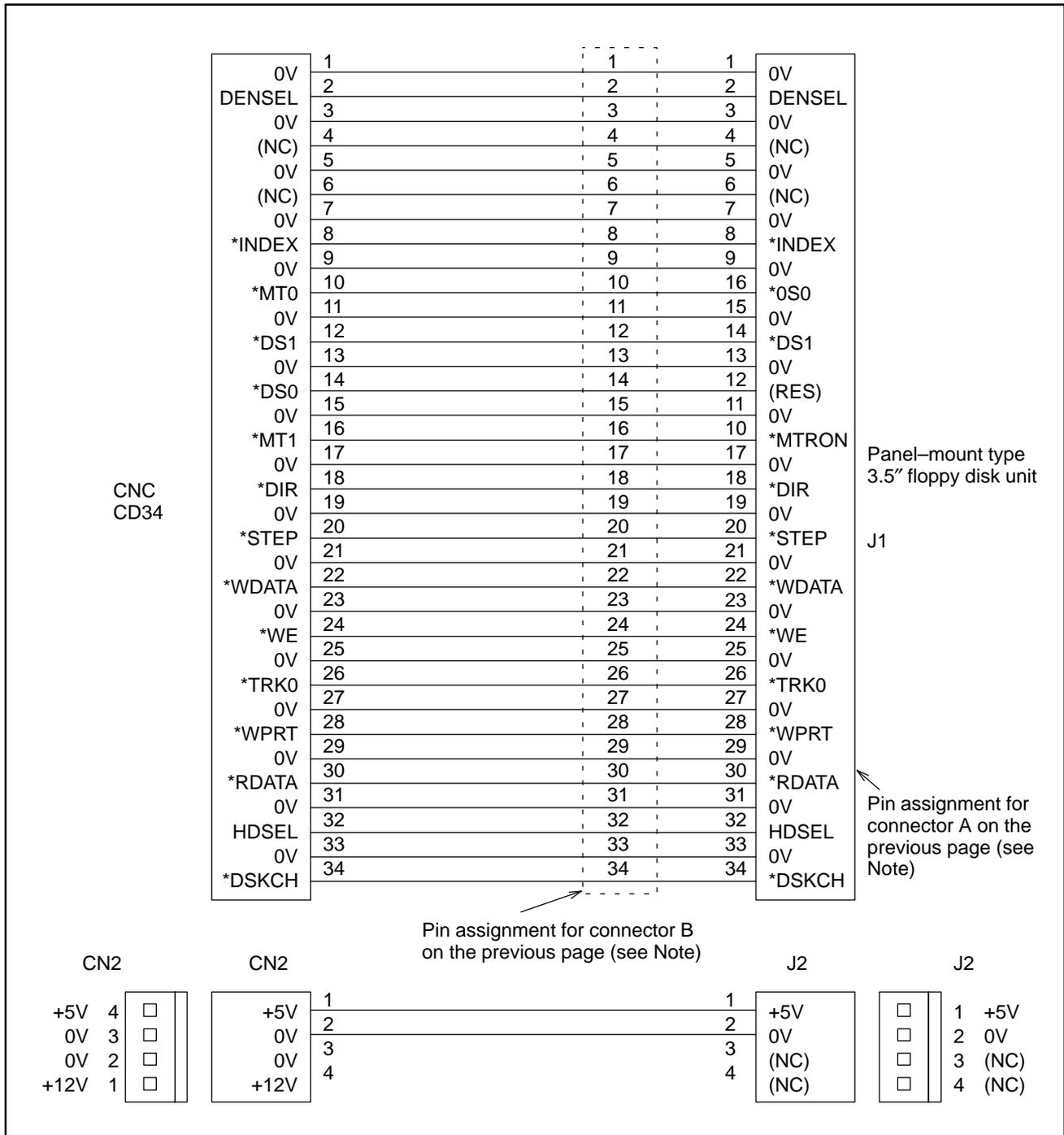
This is the standard interface for the IBM PC compatible. Commercially available cables are cross-connected between pins 10 and 16 (between the CNC and drive A) as shown above. In this case, "drive No. setting pin" on drive A should be set to 1 (second drive).
