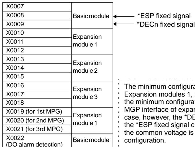
The minimum configuration consists of the basic module only. Expansion modules 1, 2, and 3 may be added as required. In the minimum configuration, SKIP and other fixed signals and the MPG interface of expansion module 1 cannot be used. In this case, however, the \*DECn fixed signal can always be used and the \*ESP fixed signal can be allocated to an address for which the common voltage is fixed to 24 V in the minimum configuration.
