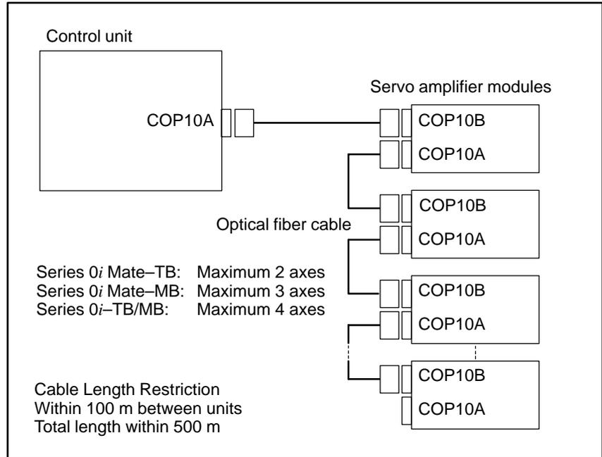
The connection between the CNC control unit and the servo amplifiers should use only one optical fiber cable, regardless of the number of controlled axes. See APPENDIX D for details on the optical fiber cable. In the control unit, the COP10A connector is placed on the servo card installed on the main board.
