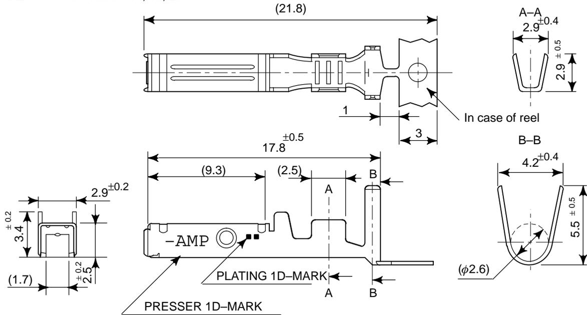
Fig.C3 (e) Contact for AMP connector
