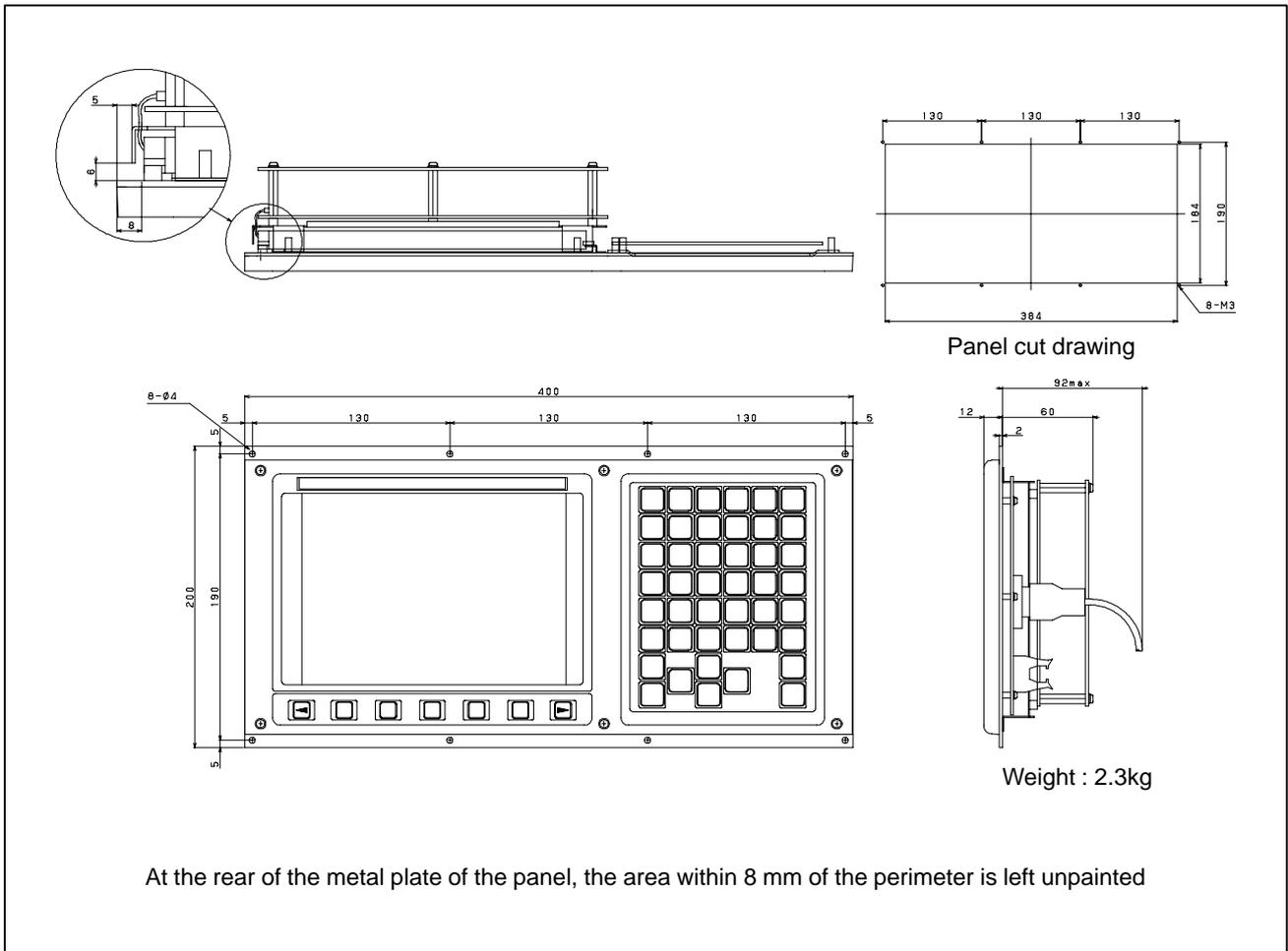
At the rear of the metal plate of the panel, the area within 8 mm of the perimeter is left unpainted
