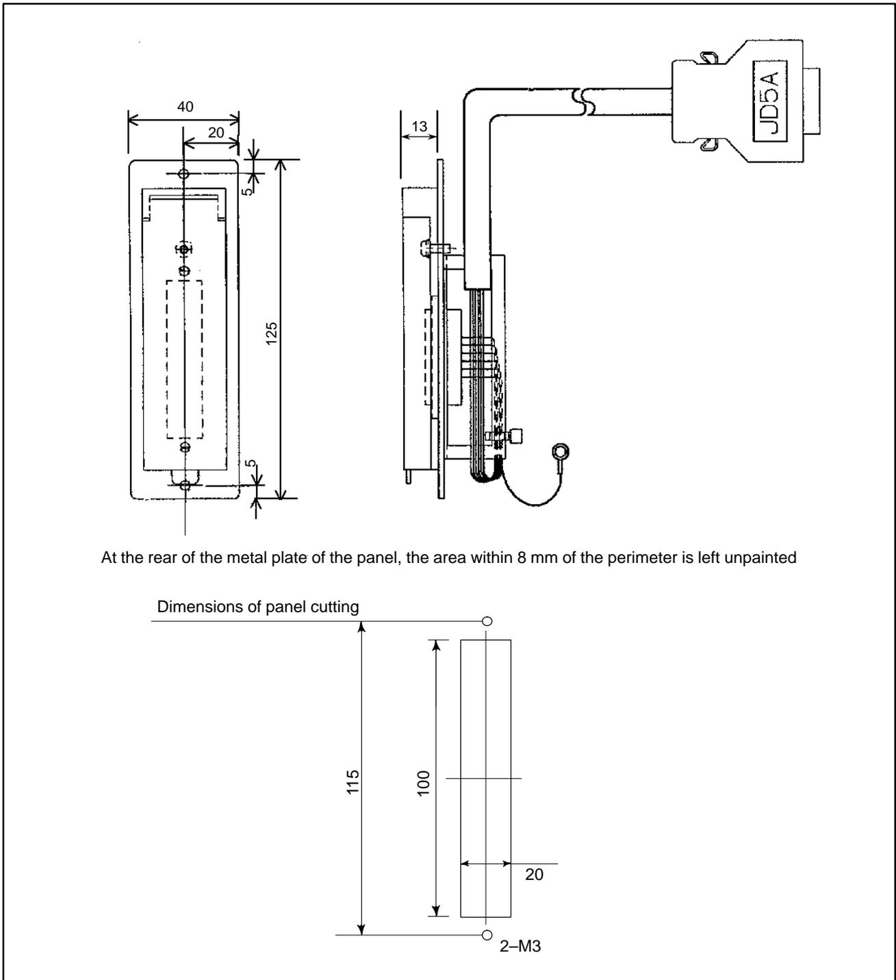
**Fig.U24 Punch panel (narrow width type)**
