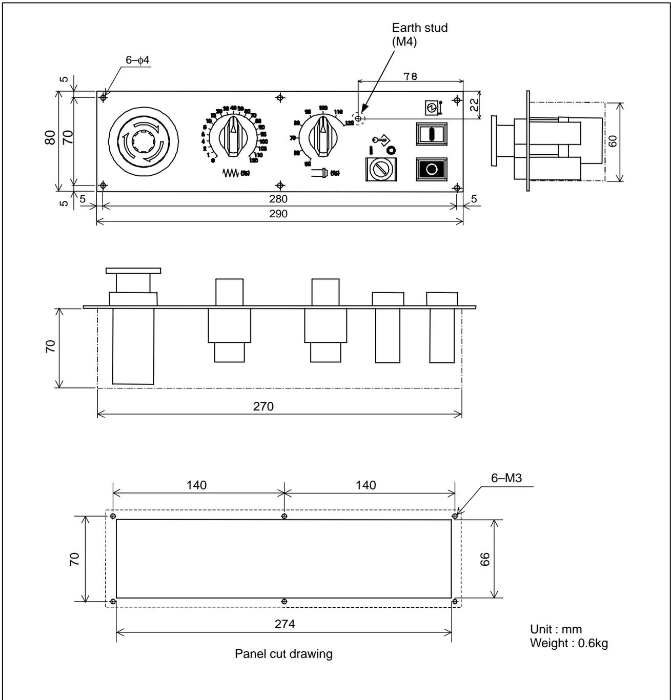
Fig.U26 Machine operator's panel (Sub panel A)
