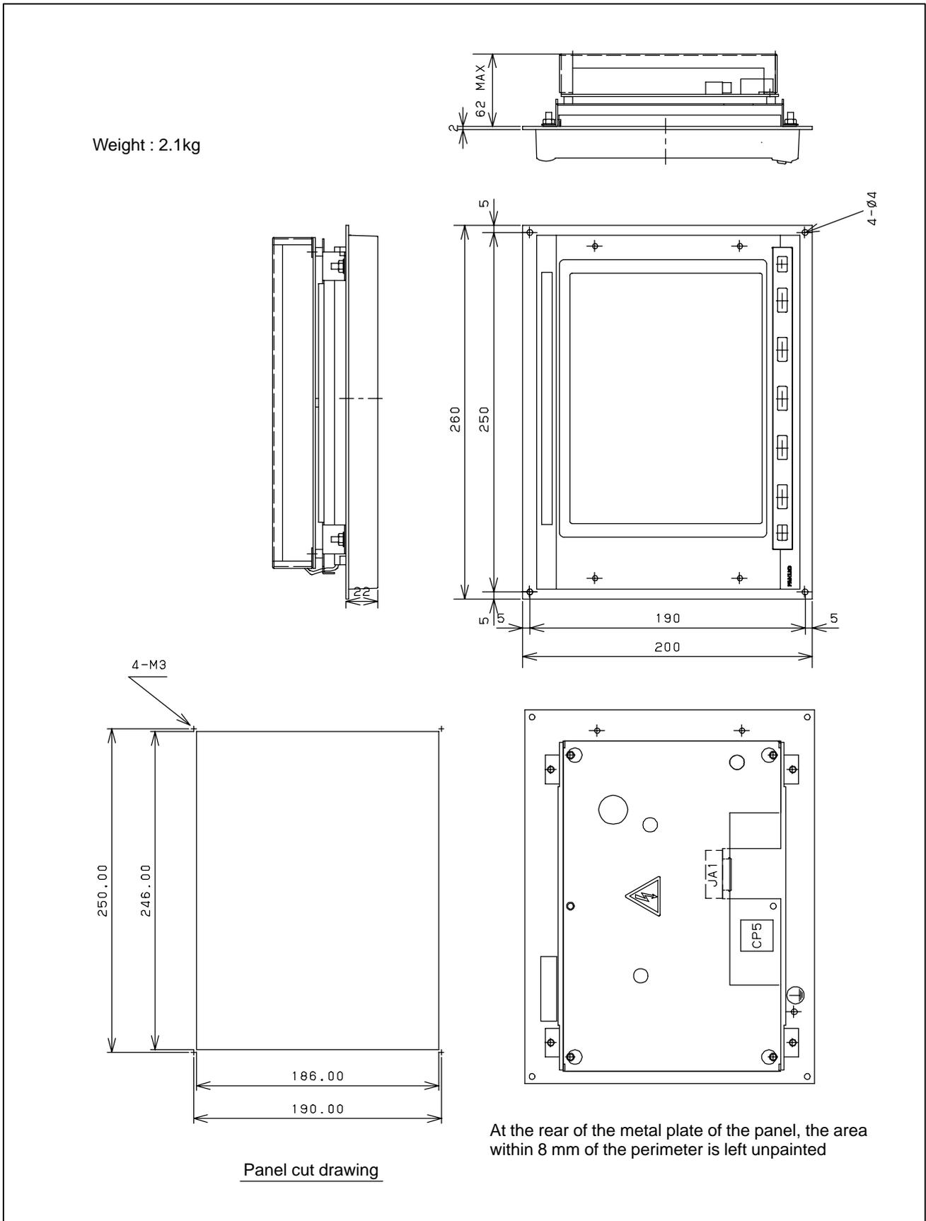
Fig.U6 8.4" TFT color LCD unit
