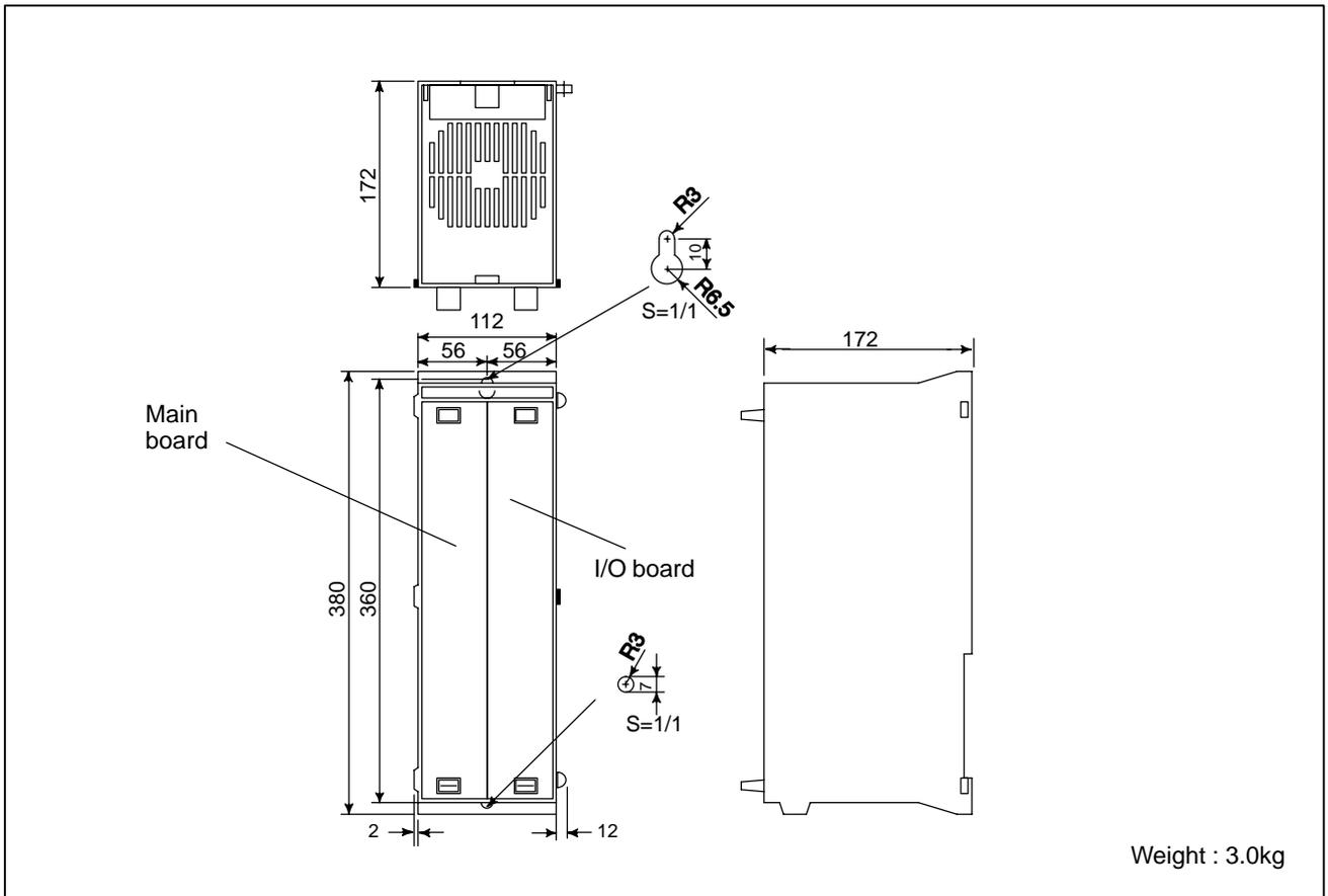
**Fig.U2 Series 0i-B basic unit (2-slot)**
