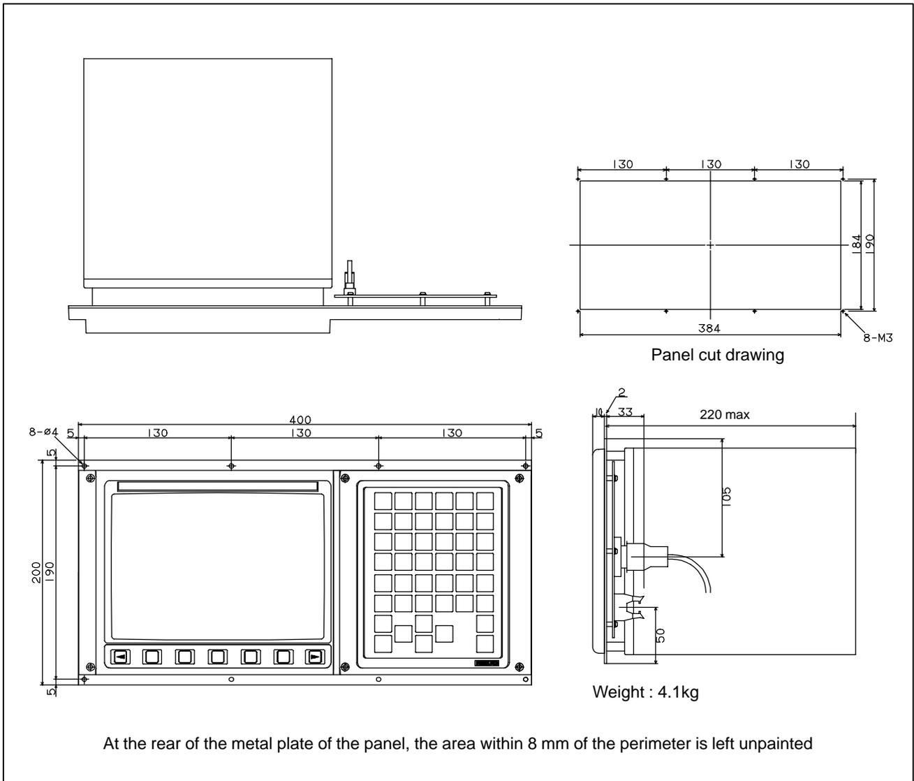
**Fig.U3 9" monochrome CRT/MDI (small size)**
