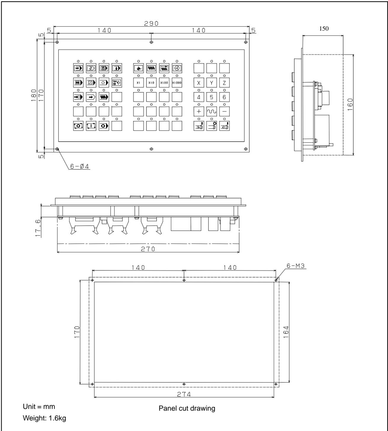
**Fig.U25 Machine operator's panel (Main panel B)**
