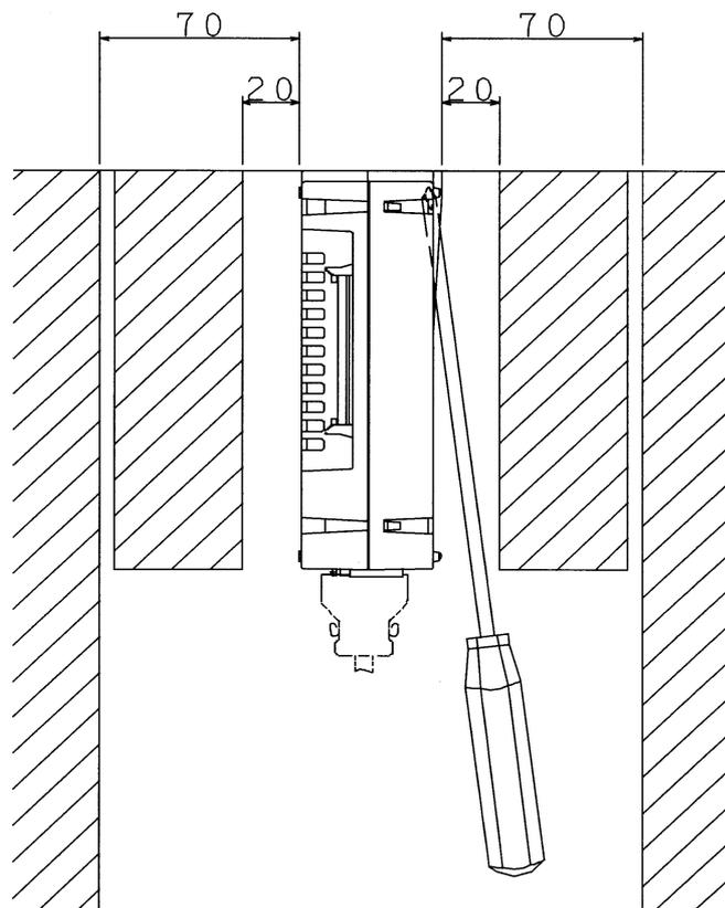
Access clearance near a separate detector interface unit
