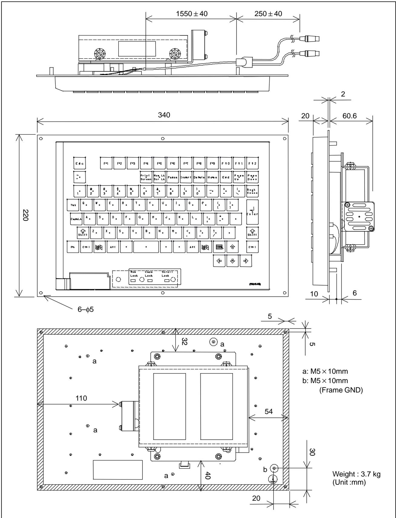
Fig.U12 (b) FA Full Keyboard 12.1" LCD Type
