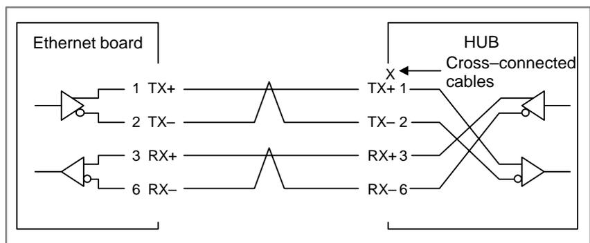
Be sure to use a Category 5 shielded twisted pair (STP) cable for improvement of noise immunity in FA environments, although various types of unshielded twisted pair (UTP) cables for 10BASE-T are currently on the market.
