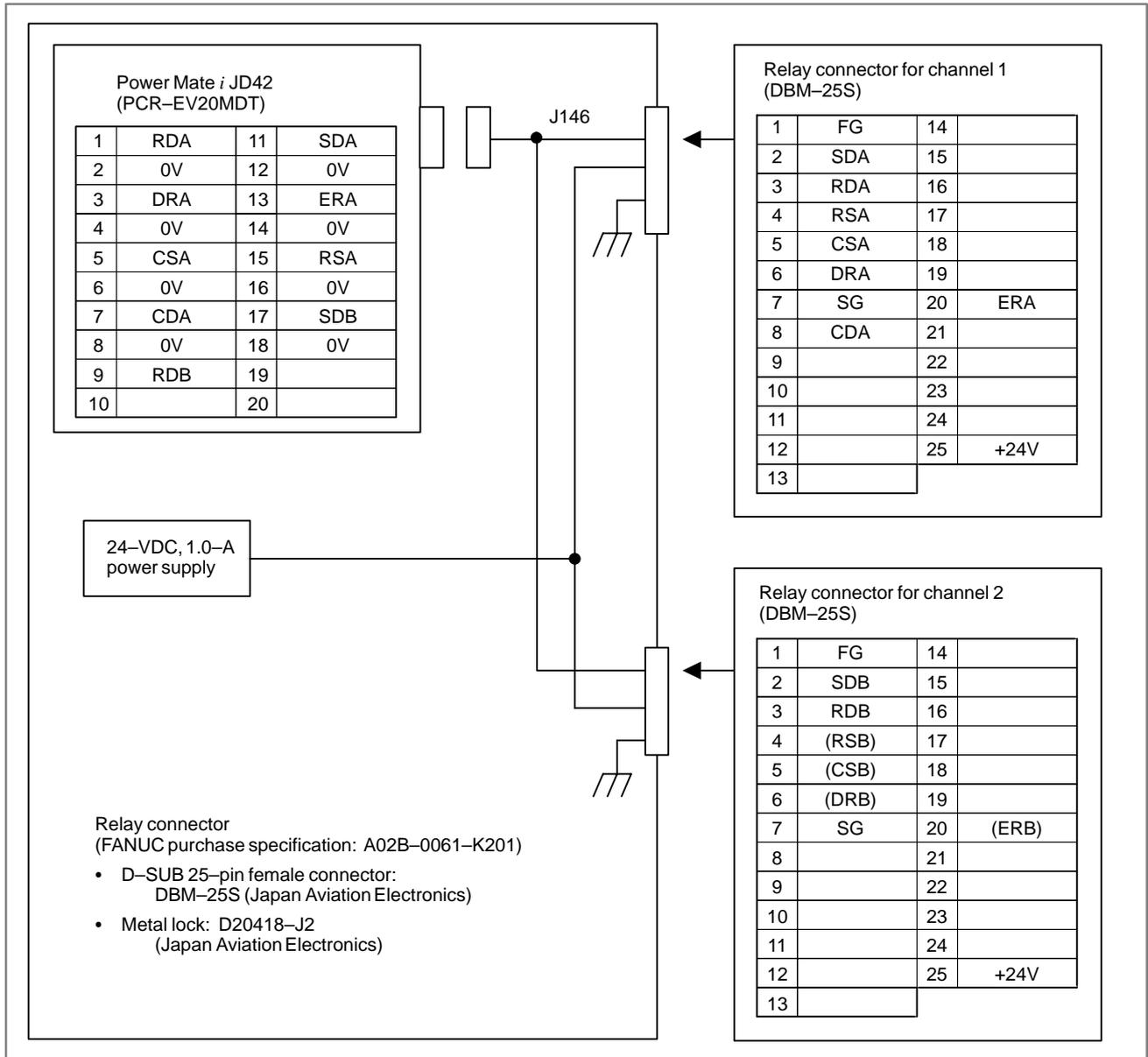
Cable-side connector (FANUC purchase specification: A02B-0118-K895)
