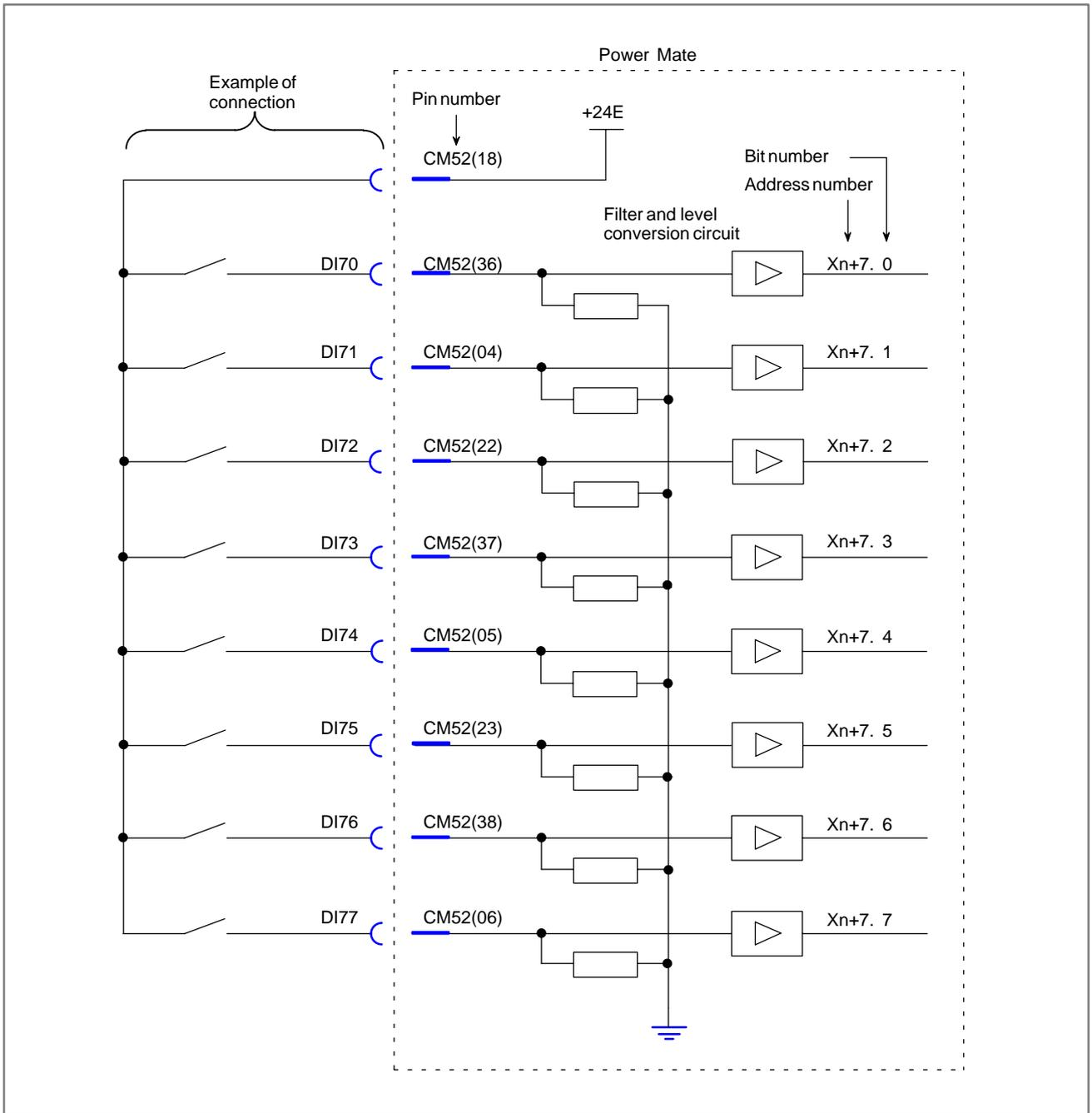
Fig. 6.6.3 (h) I/O card machine interface (8)
