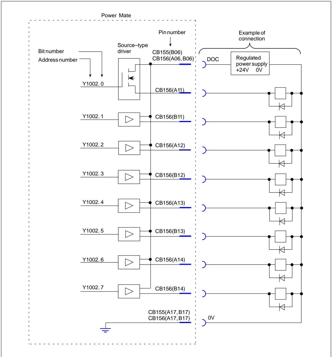
Fig. 6.4.5 (c) Built-in I/O machine interface (7)
