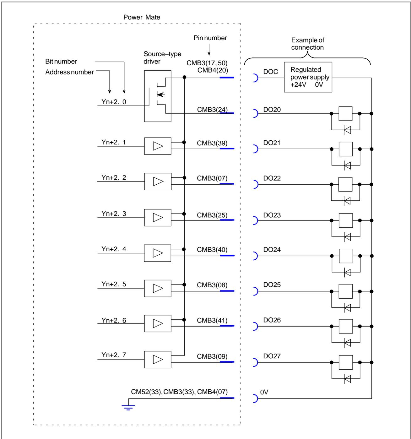
Fig. 6.6.4 (c) I/O card machine interface (15)
