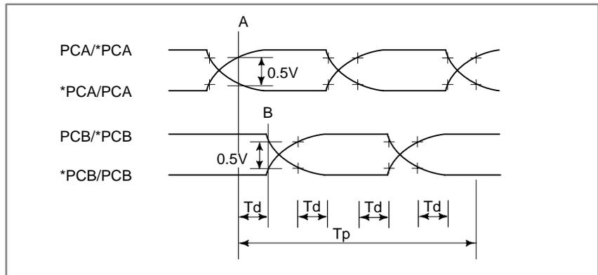
Requirements for the signals at the input pins of input connectors JF101 to JF108
