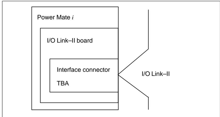
The interface connector for the I/O Link-II board of the Power Mate *i* is a 5-pin connector, and two I/O Link-II cable wires are installed. Terminating resistors are built into the I/O Link-II board. So, connect T1 with T2 by using a wire.
