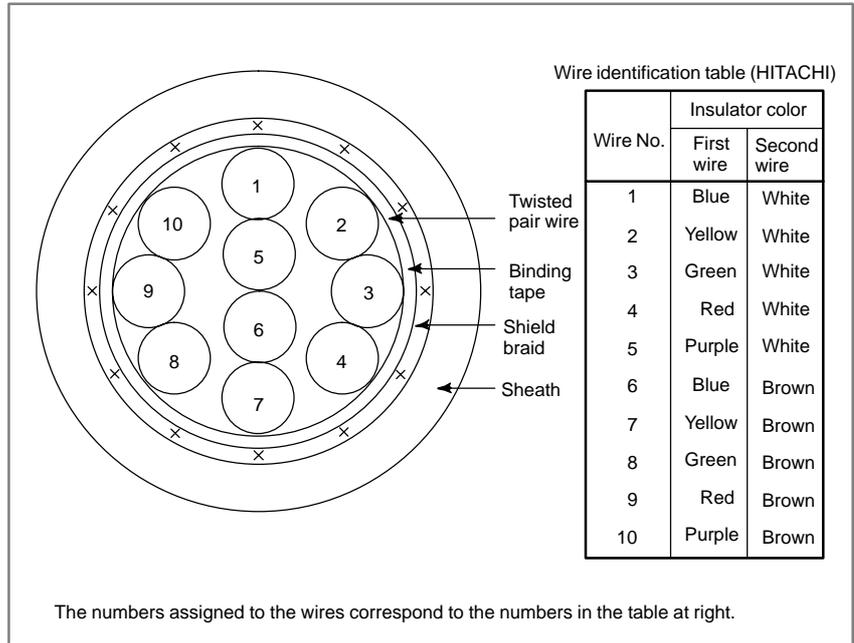
Fig. C.5 (a) Cable made by Hitachi Cable
