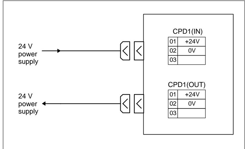
Recommended cable-side connector: A02B-0120-K324
