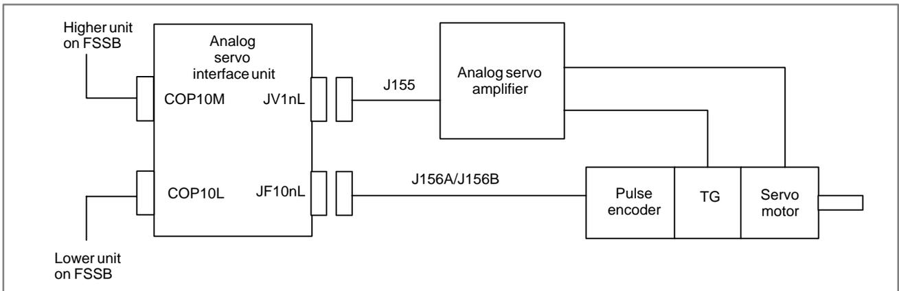
2) Configuration when a separate detector is used
