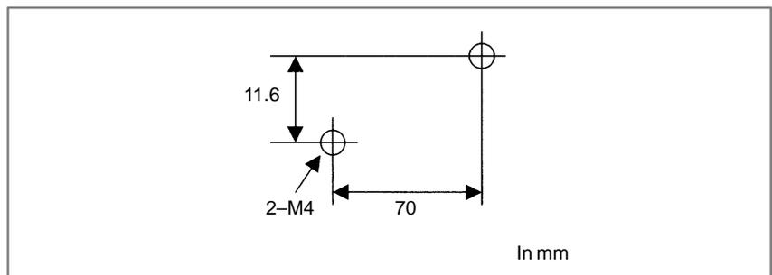
**Fig. 8.1.10 (c) Sheet metal hole drilling diagram**
