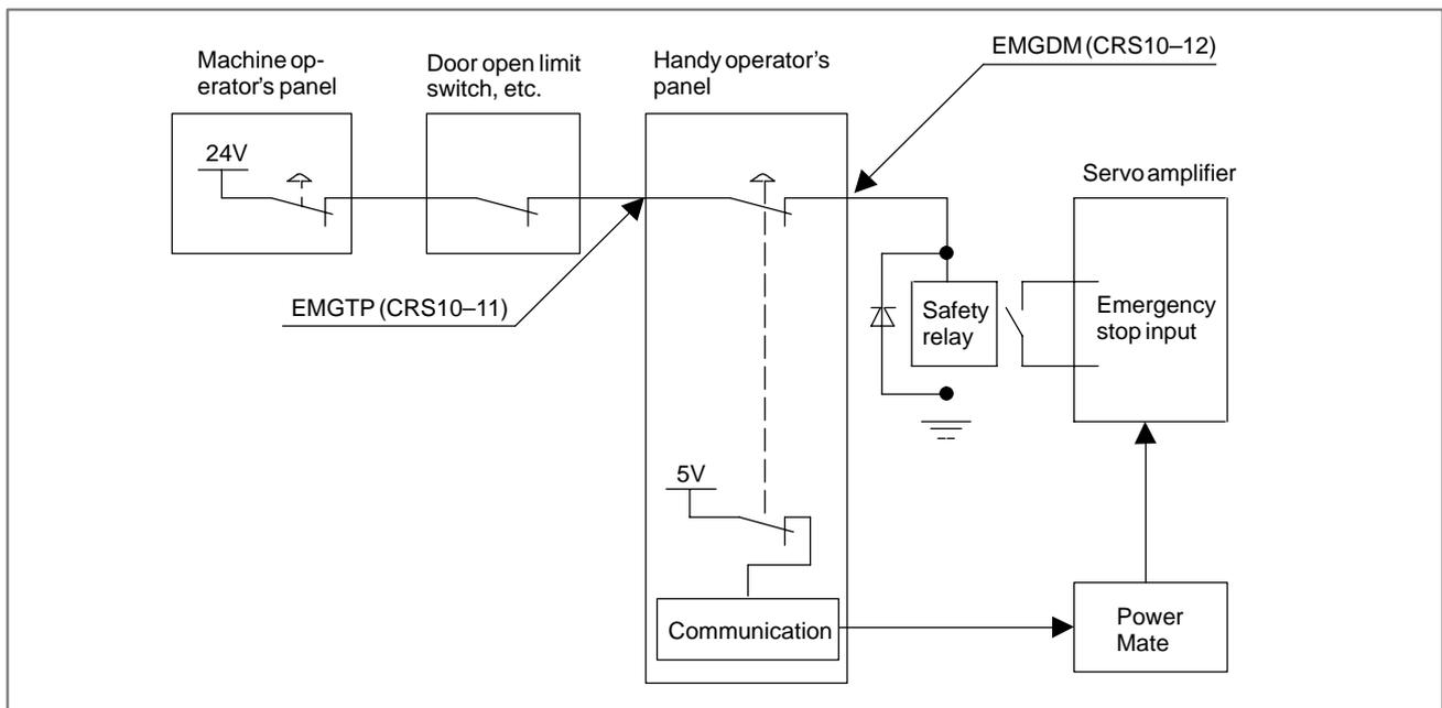
The allowable current of the emergency stop line of the handy operator's panel is as follows:
