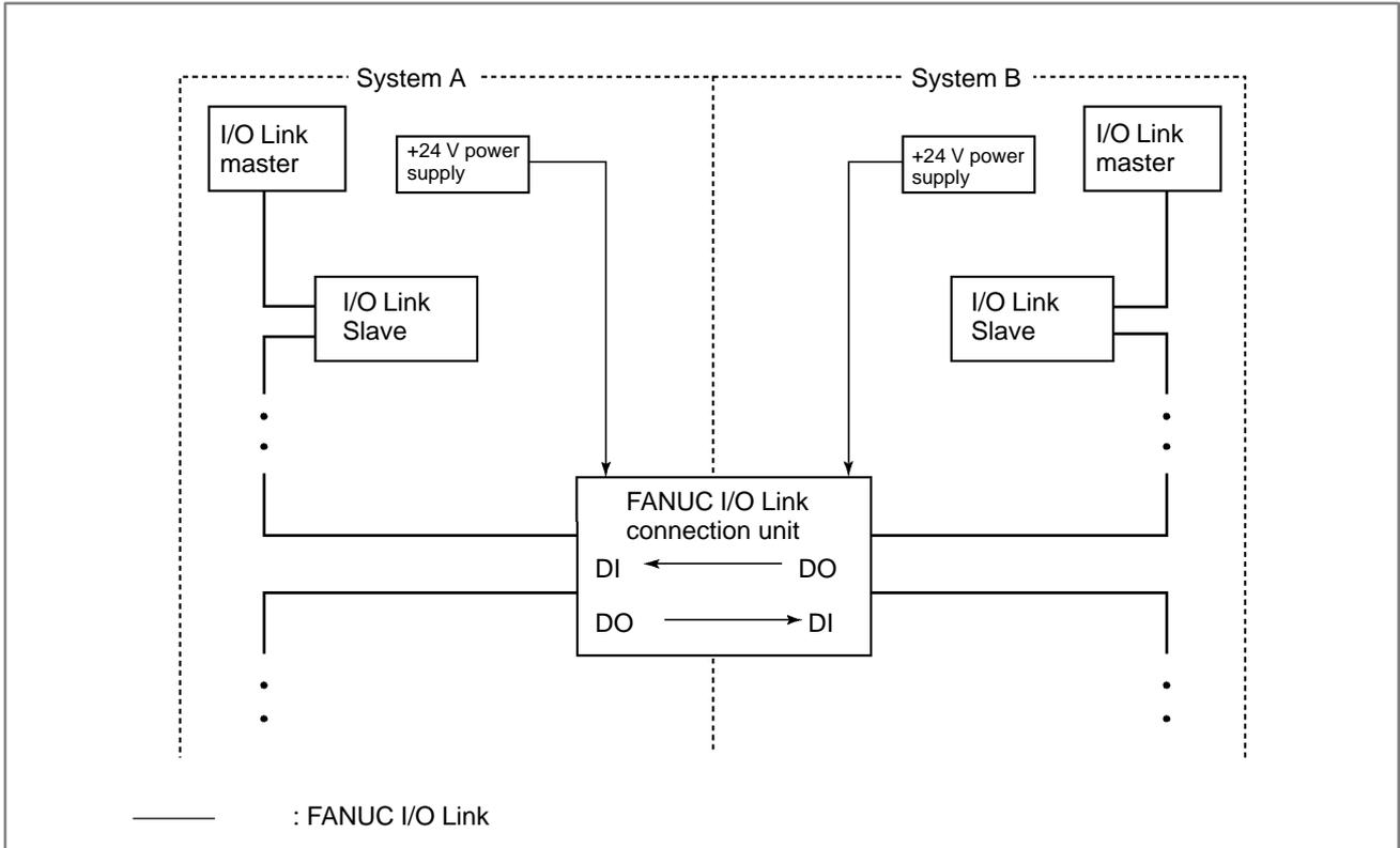
Fig. 6.11.1 System which uses FANUC I/O Link connection units
