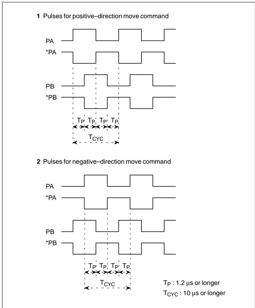
**Fig. 10.2 (a) Input pulse waveforms**
