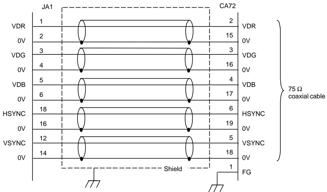
Recommended cable: A66L-0001-0371 (5-conductor coaxial cable, common shield) <Hitachi Cable, Ltd.>
