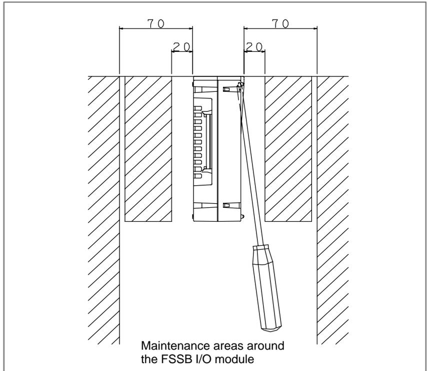
4) Mounting the unit on the DIN rail
