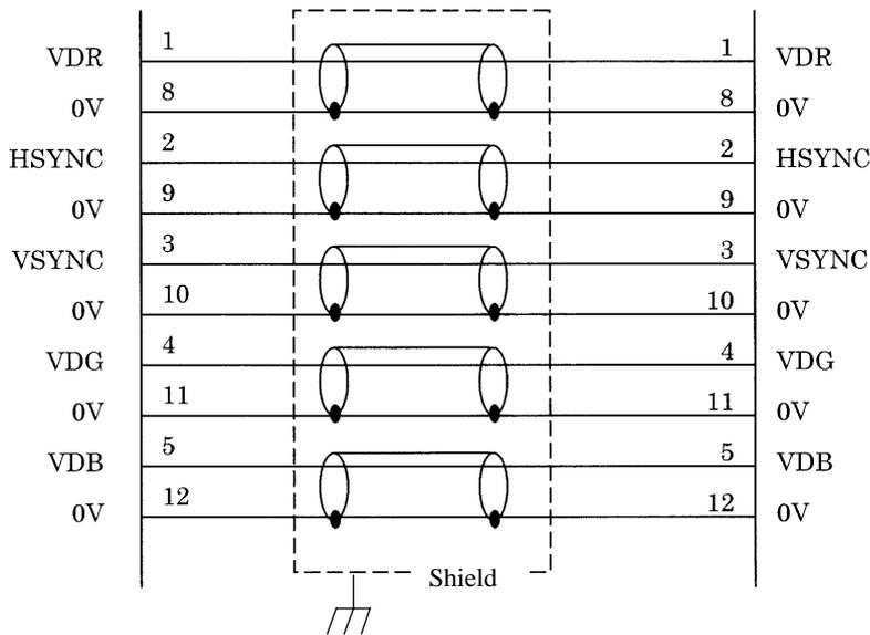
Recommended wire: A66L-0001-0371 . . . . Coaxial cable (five conductors, common shield)
