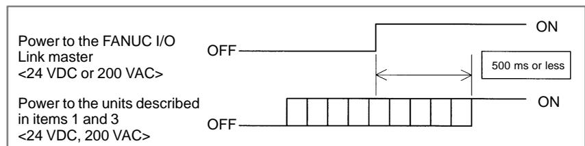
If a separate detector (scale) of parallel interface is used and its power is supplied from a power source other than a separate detector interface unit, turn on the power to the separate detector (scale) before turning on the power to the separate detector interface unit. The A/B-phase signal of the separate detector (scale) must be stabilized before the separate detector interface unit is turned on.
