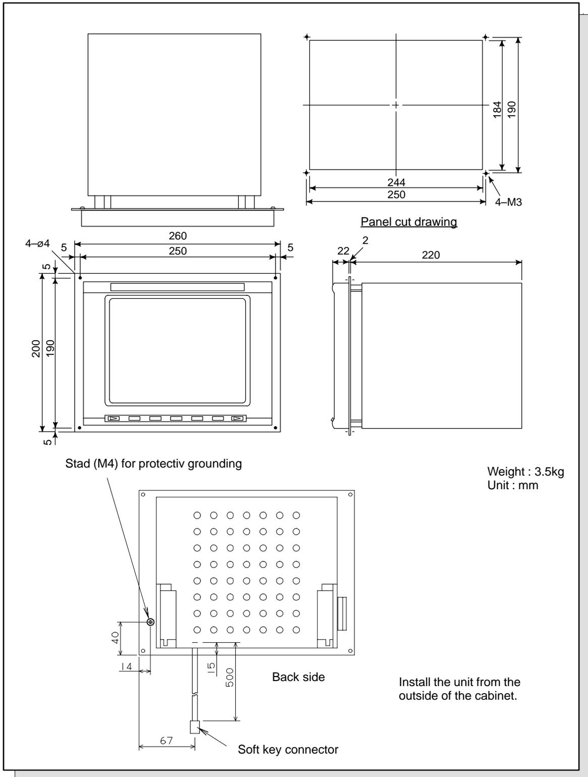
**Fig. 7** Separate MDI, separate MDI with picture display
