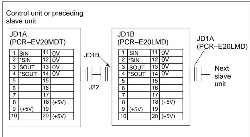
+5 V terminals are for an optical I/O link adapter. They are not necessary when connecting with a optical cable.
