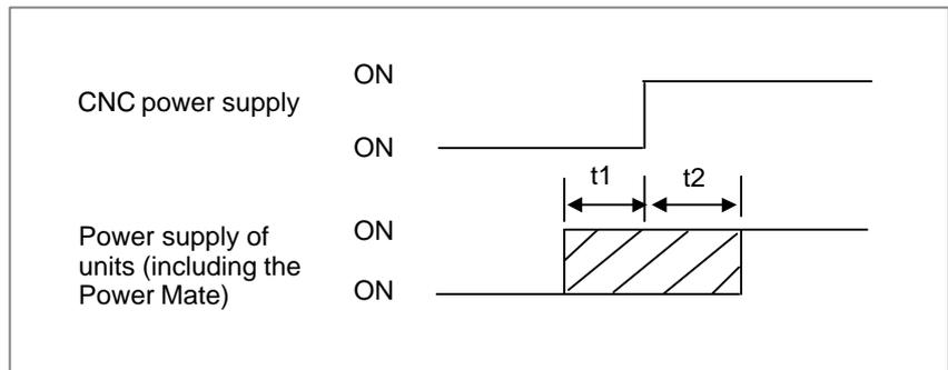
$t_1$ : 200 ms The units (including the other Power Mate as slave) are turned on within 200 ms before the power to the Power Mate *i* is turned on.
