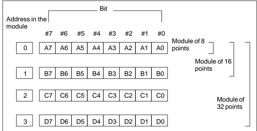
Addresses in a module are defined relatively, with the beginning address as 0. Real addresses viewed by the sequence program of the PMC are set by the programmer.
