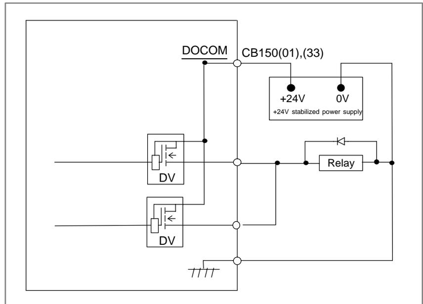
**DO (output signal) alarm detection**
