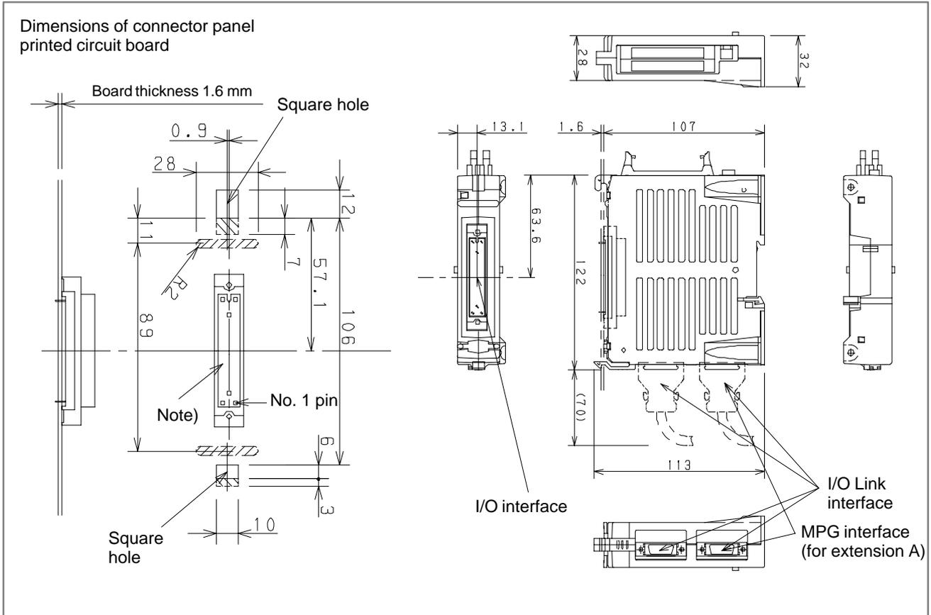
Connector panel printed circuit board connector specification:
