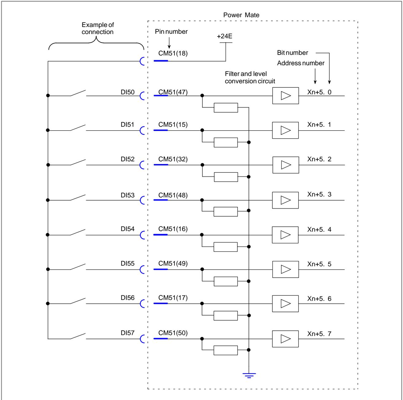
Fig. 6.6.3 (f) I/O card machine interface (6)
