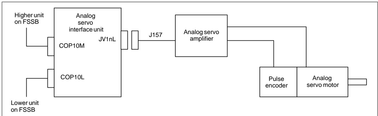
2) Configuration when a separate detector is used
