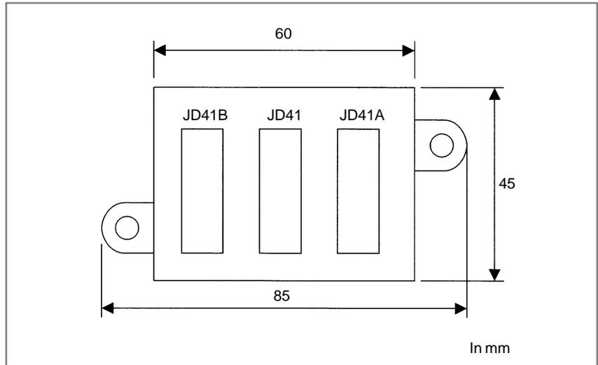
**Fig. 8.1.10 (a) Display link adaptor manufactured by FANUC**
