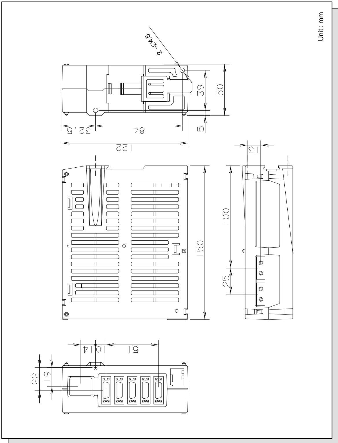
**Fig. 16** Battery case for separate absolute pulse coder
