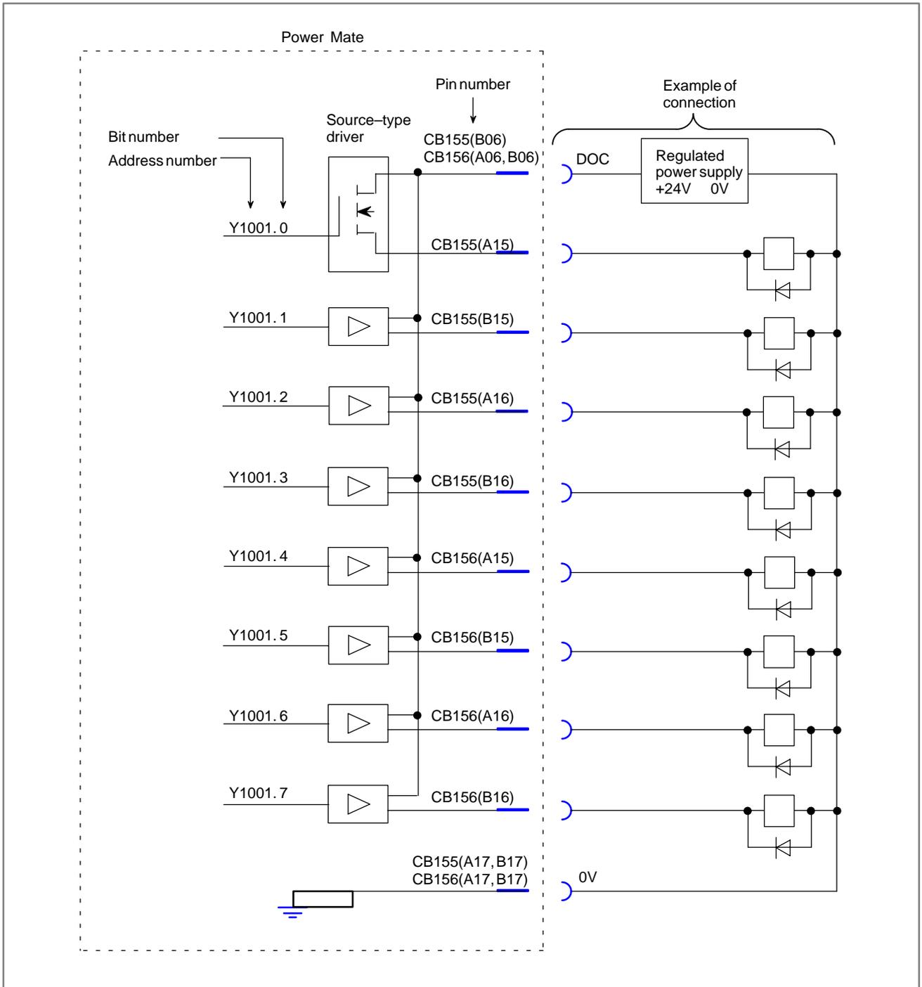
Fig. 6.4.5 (b) Built-in I/O machine interface (6)
