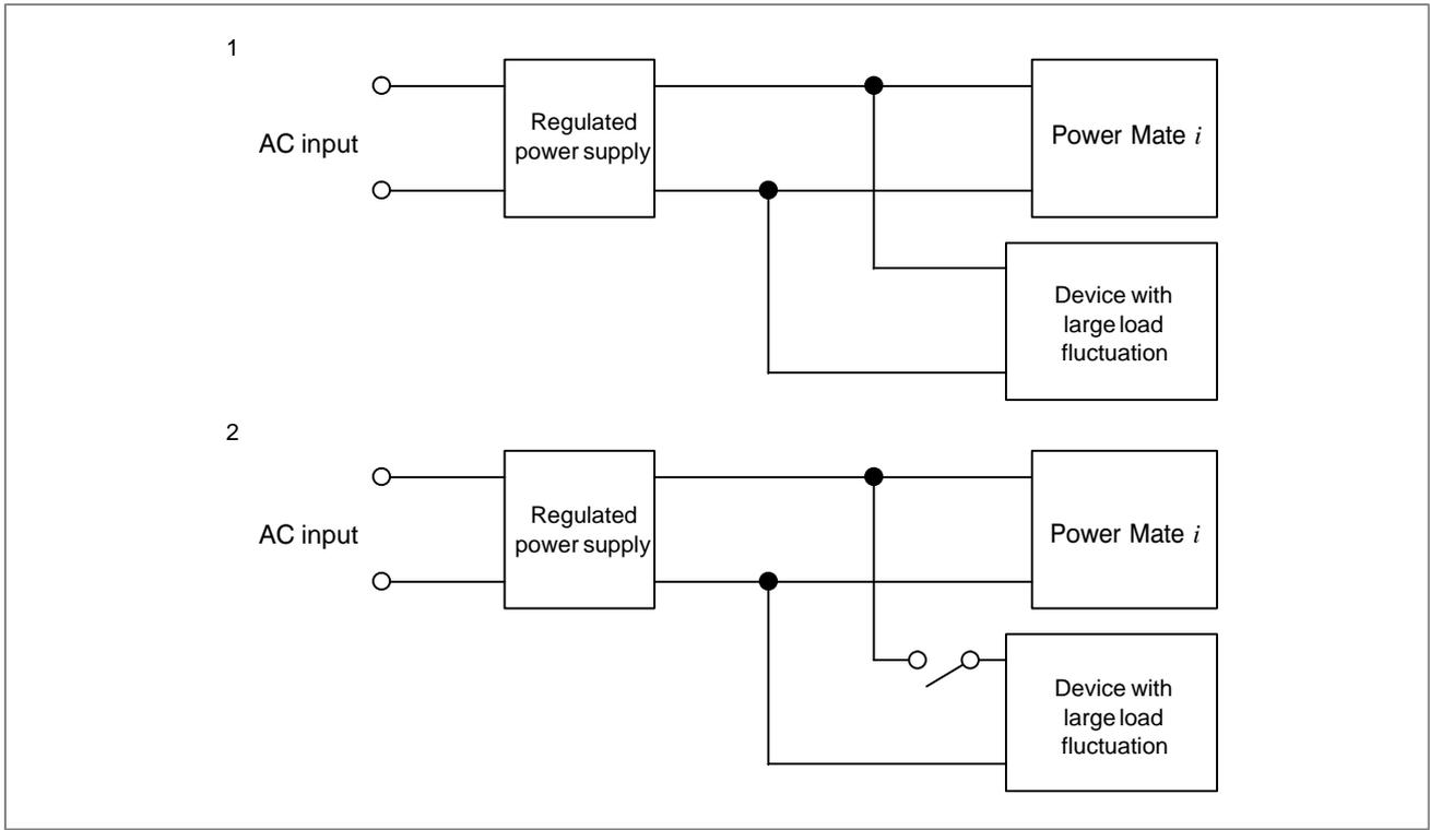
In case of <2>, prepare another regulated power supply specially for the device with abrupt change in load to prevent the change from influencing the Power Mate *i* and other units.
