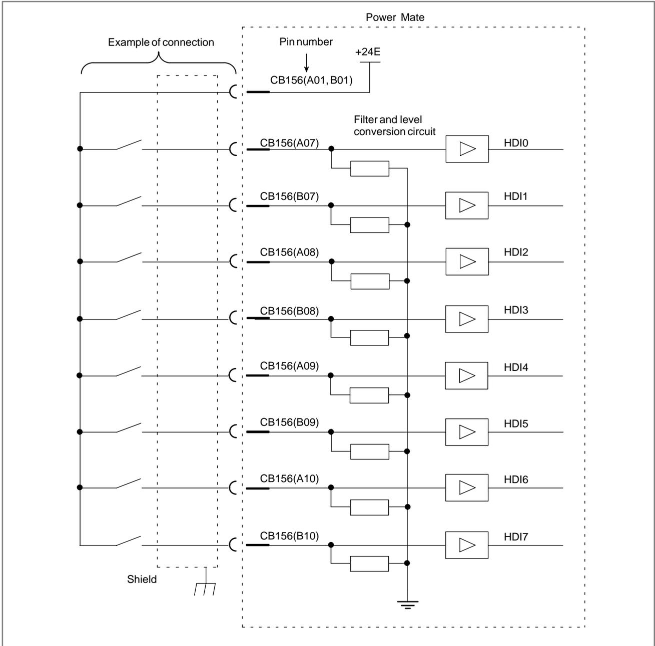
Fig. 6.5.5 High-speed DI signal interface
