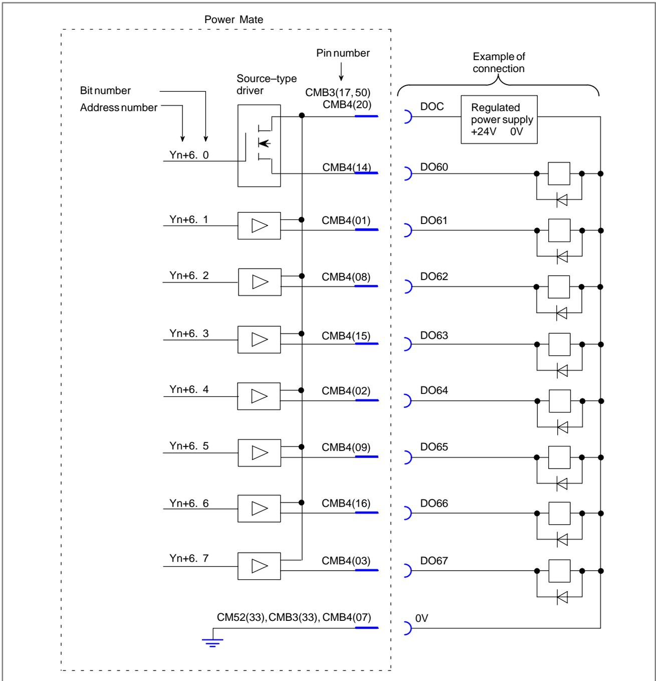
Fig. 6.6.4 (g) I/O card machine interface (19)
