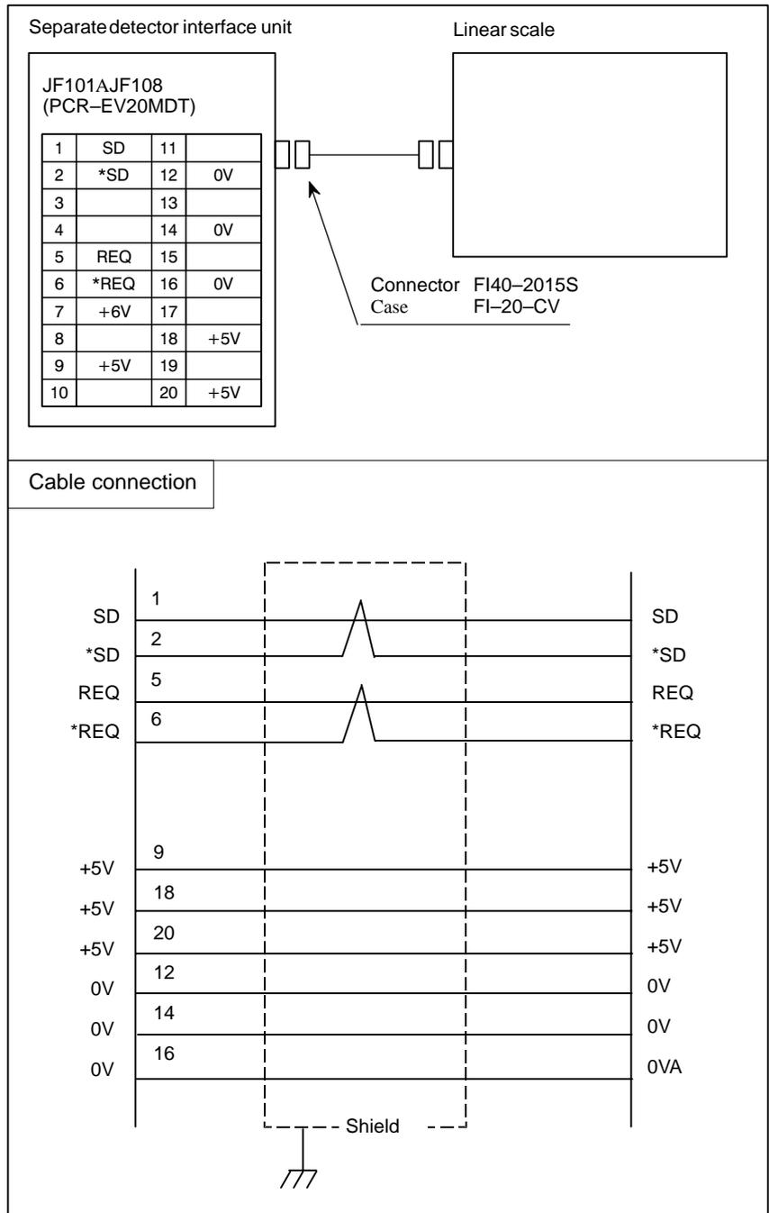
The recommended cable and connectors (JF101 to JF108) are the same as for the parallel interface.
