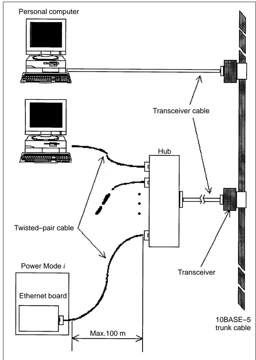
Some devices (hub, transceiver, etc.) that are needed for building a network do not come in a dust-proof construction. Using such devices in an atmosphere where they are subjected to dust or oil mist will interfere with communications or damage the Ethernet board. Be sure to install such devices in a dust-proof cabinet.
