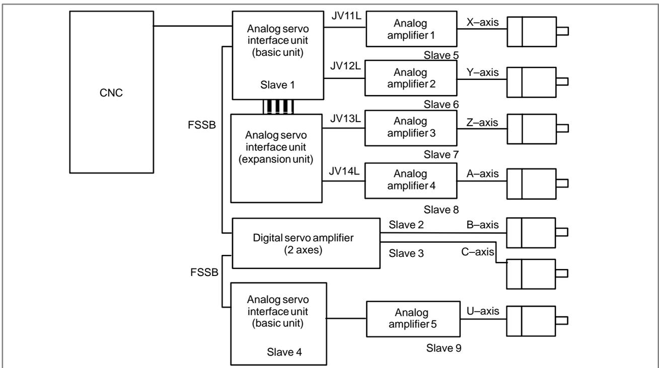
In the order of connection to the FSSB, the first analog servo interface unit (including the expansion unit) is assigned slave 1, the digital servo amplifier (two axes) is assigned slaves 2 and 3, and the second analog servo interface unit is assigned slave 4. The analog amplifiers are assigned slaves 5 to 9 on the assumption that they are connected after the analog servo interface unit.
