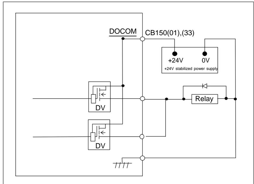
**DO (output signal) alarm detection**
