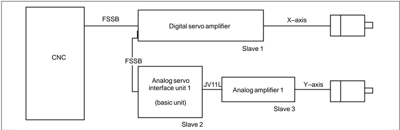
In the order of connection to the FSSB, the digital servo amplifier is assigned slave 1, and the analog servo interface unit is assigned slave 2. The axis connected to the analog amplifier is assumed to be connected next to the analog servo interface unit, and the analog amplifier is assigned slave 3.
