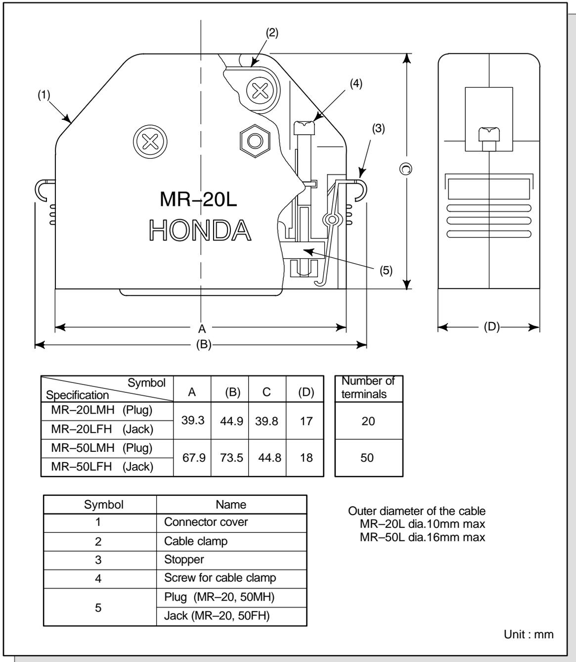
**Fig. 11** Honda connector (angled-type case)
