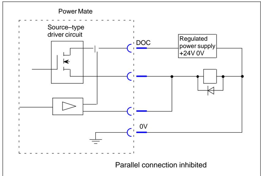
When using a dark-light resistance, connect a leakage prevention diode to it.
