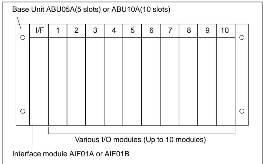
AIF01A is used for connection to FANUC I/O Link
