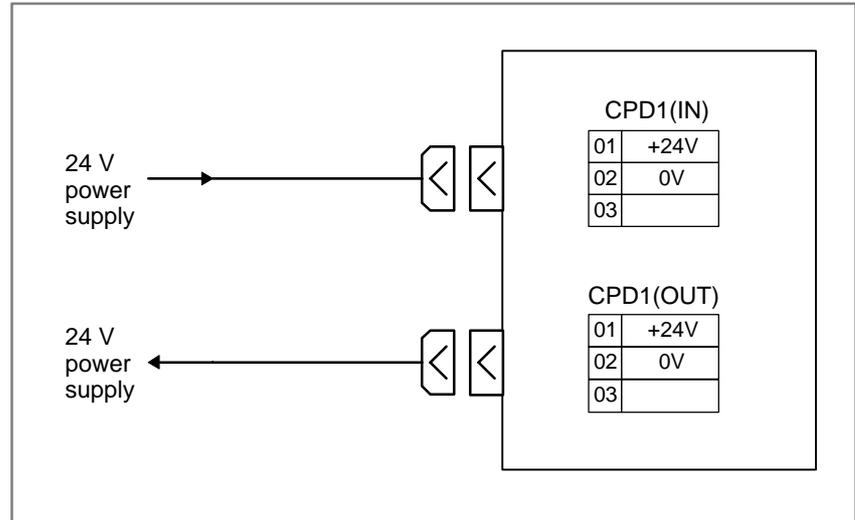
Recommended cable-side connector: A02B-0120-K324
