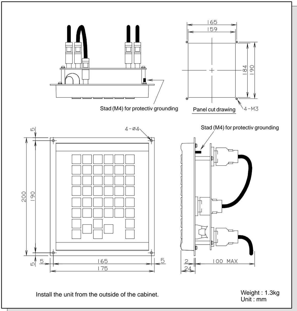
**Fig. 8** Separate PDP
