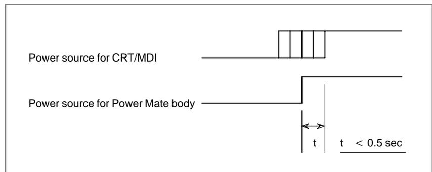
If the power for the CRT/MDI is turned on after the power for Power Mate body is turned on, it becomes impossible to execute special operations while the power for Power Mate is on such as memory all clear (See Subsec. 8.1.6).
