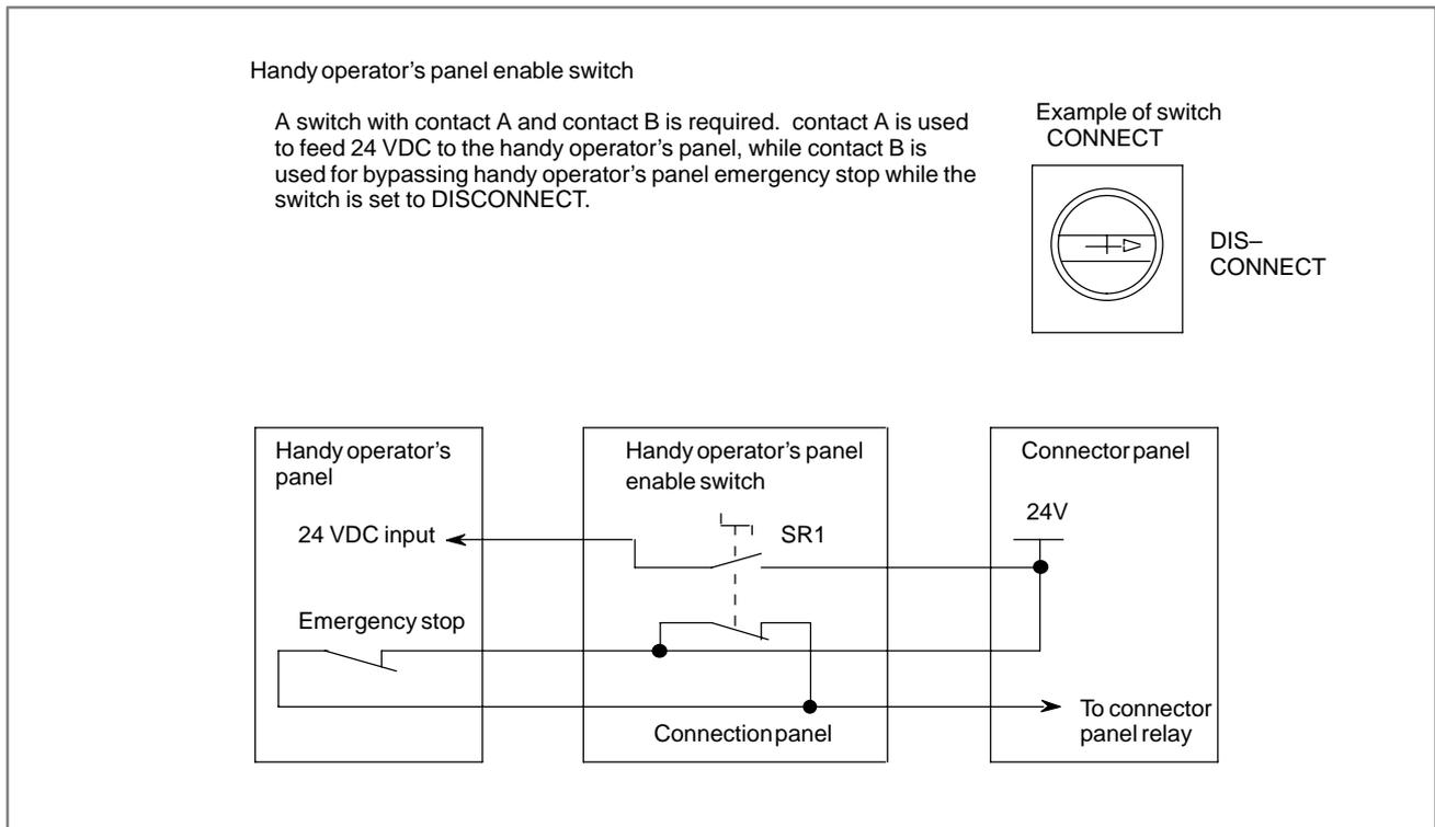
(1) While the enable switch is set to DISCONNECT (while the switch is off)
