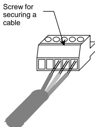
Detach the cable connector from the board by removing the mounting screws. Connect the communication cable to the connector according to the procedure below.
