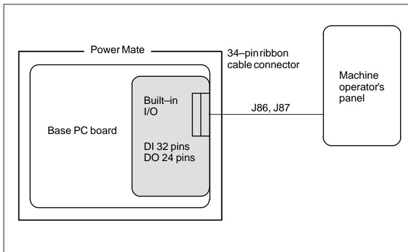
This is built-in I/O mounted on the base PC board of Power Mate.
