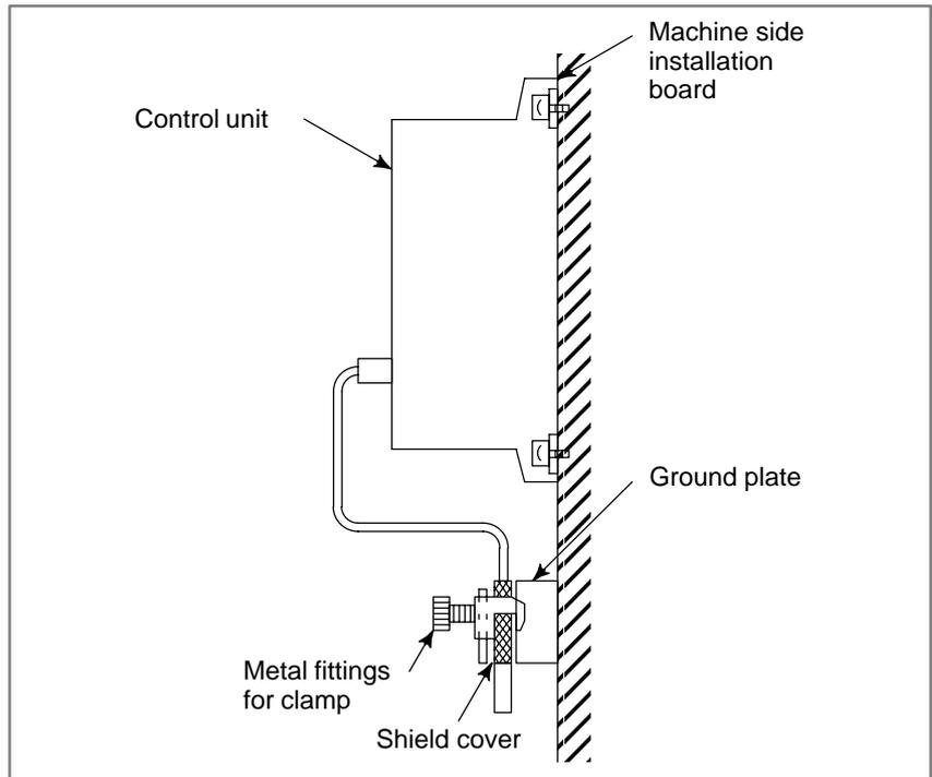
**Fig. 3.6.5 (b) Cable clamp (2)**
