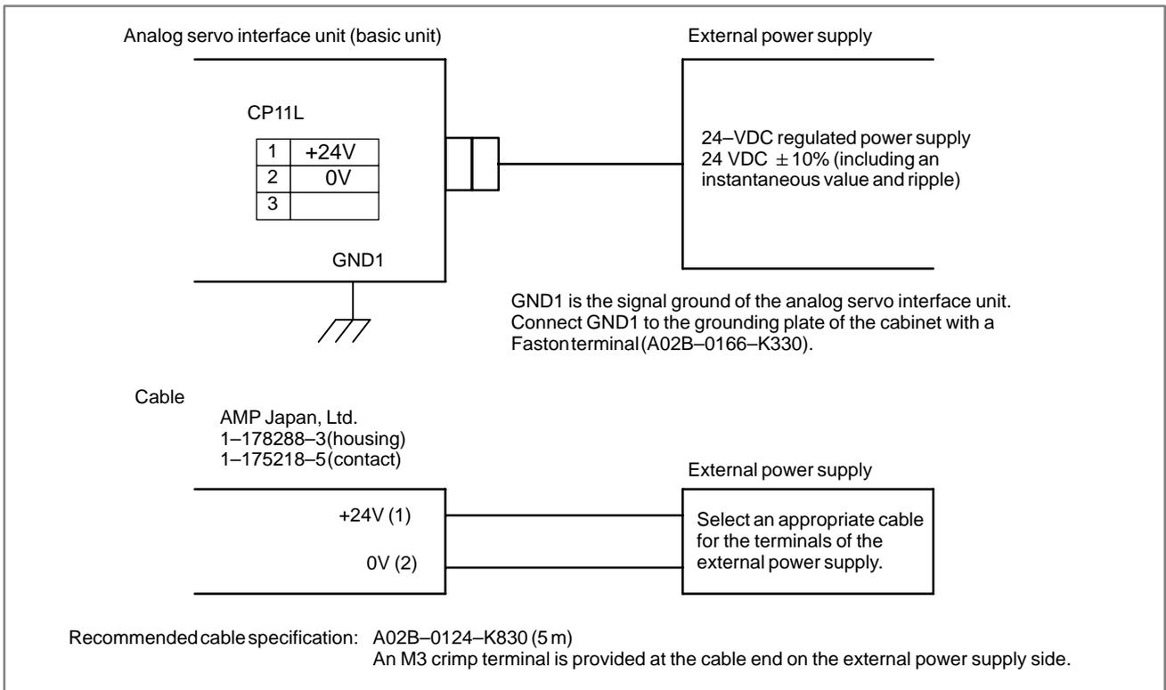
The 24-VDC signal input to CP11L can be taken out from CP11M for the purpose of branching. CP11M connection is the same as for CP11L.
