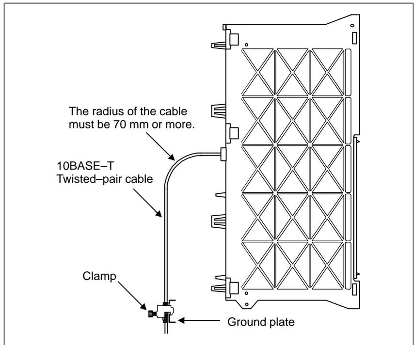
The Ethernet cable must be fastened by a cable clamp to prevent tension being applied to the connector that connects the cable to the control unit (RJ-45) even if the Ethernet cable is pulled directly. This clamp is also used to ground the cable shield.
