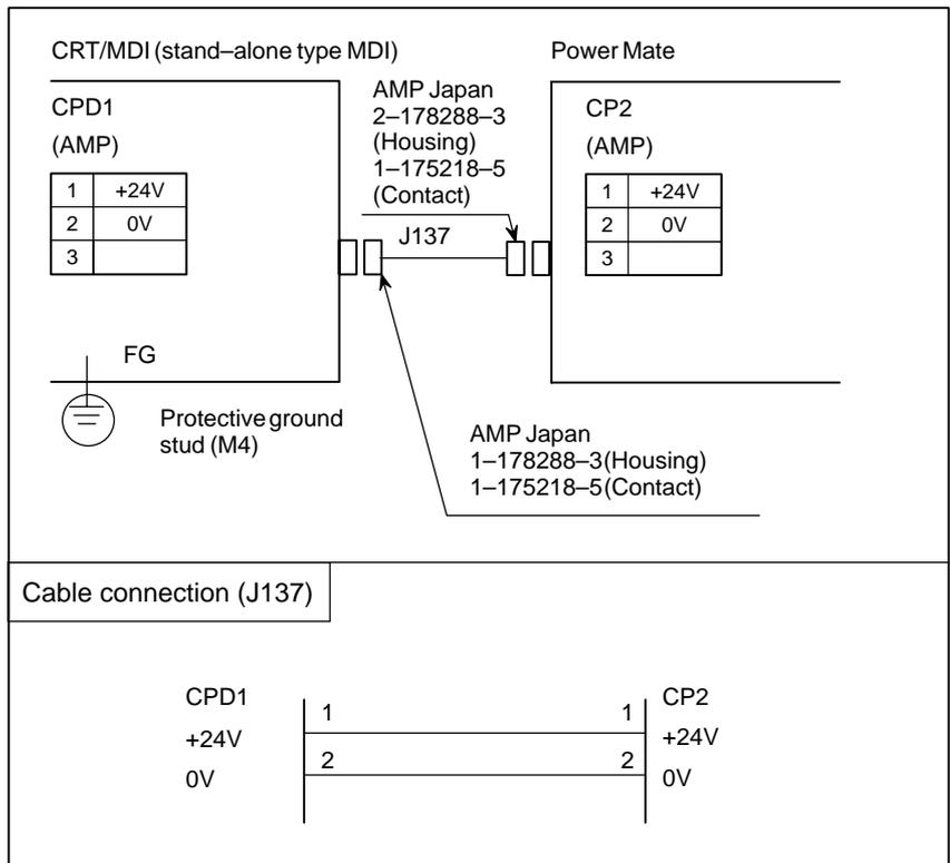
CRT/MDI unit-side cable connector A02B-0120-K324
