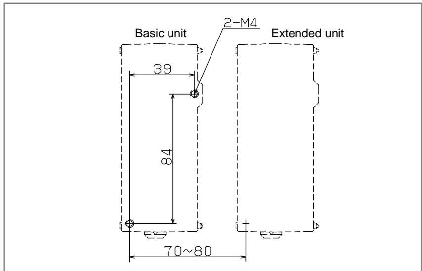
**Mounting hole drilling diagram**
