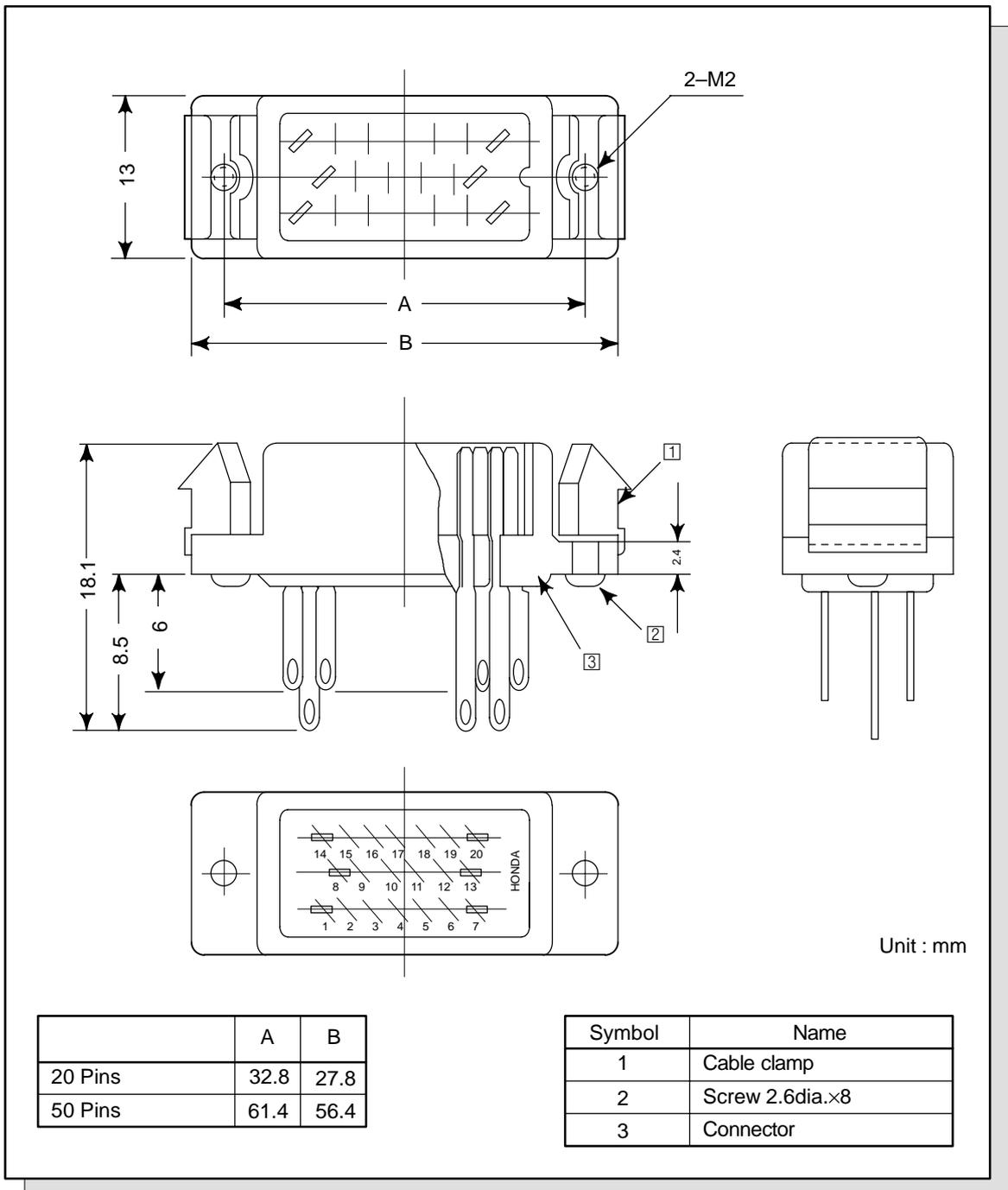
**Fig. 14** Honda connector (Terminal layout)
