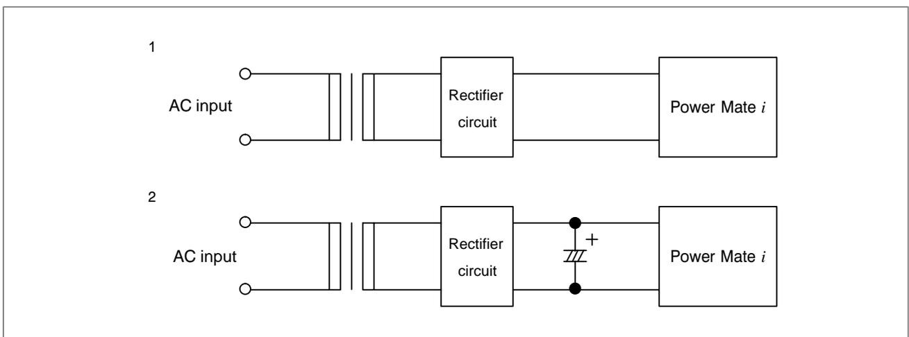
Rectifier circuits perform full-wave rectification by using diodes.
