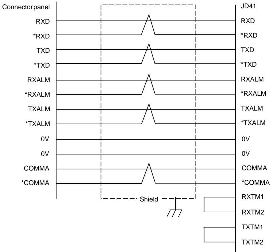
Recommended cable: A66L-0001-0284#10P (#28AWG 10 pairs, common shield) <Hitachi Cable, Ltd., Oki Electric Cable Co., Ltd.>
