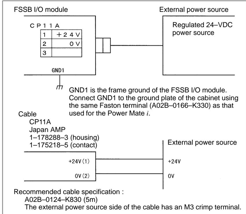
The 24-VDC power input to CP11A can be extracted from CP11B. The connection of CP11B is the same as that of CP11A.
