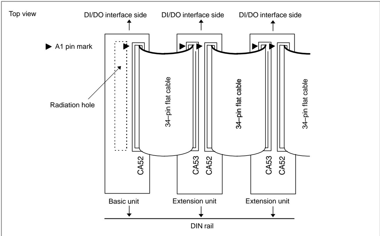
Flat cable-side connector specification:
