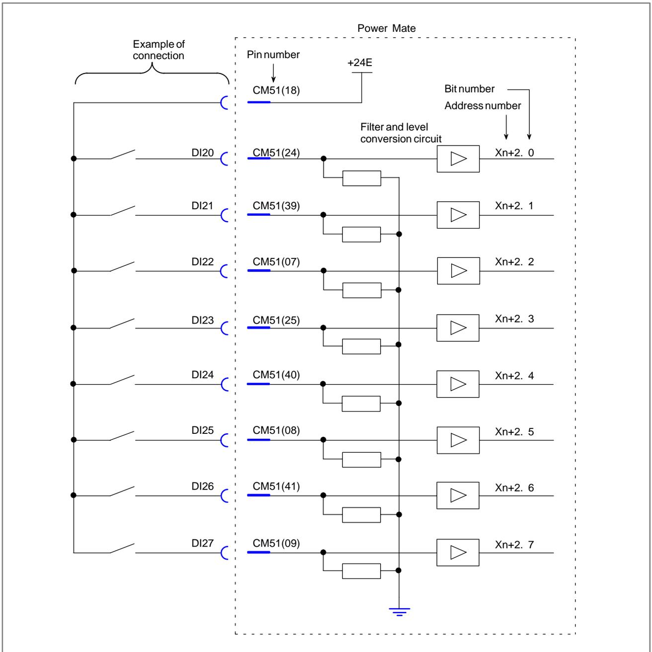
Fig. 6.6.3 (c) I/O card machine interface (3)
