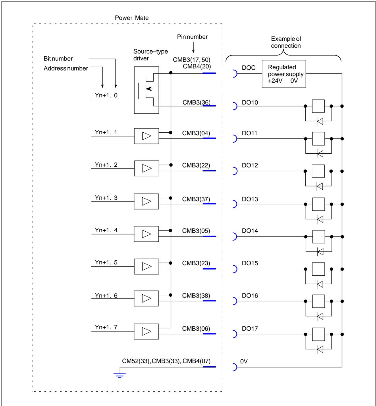
Fig. 6.6.4 (b) I/O card machine interface (14)
