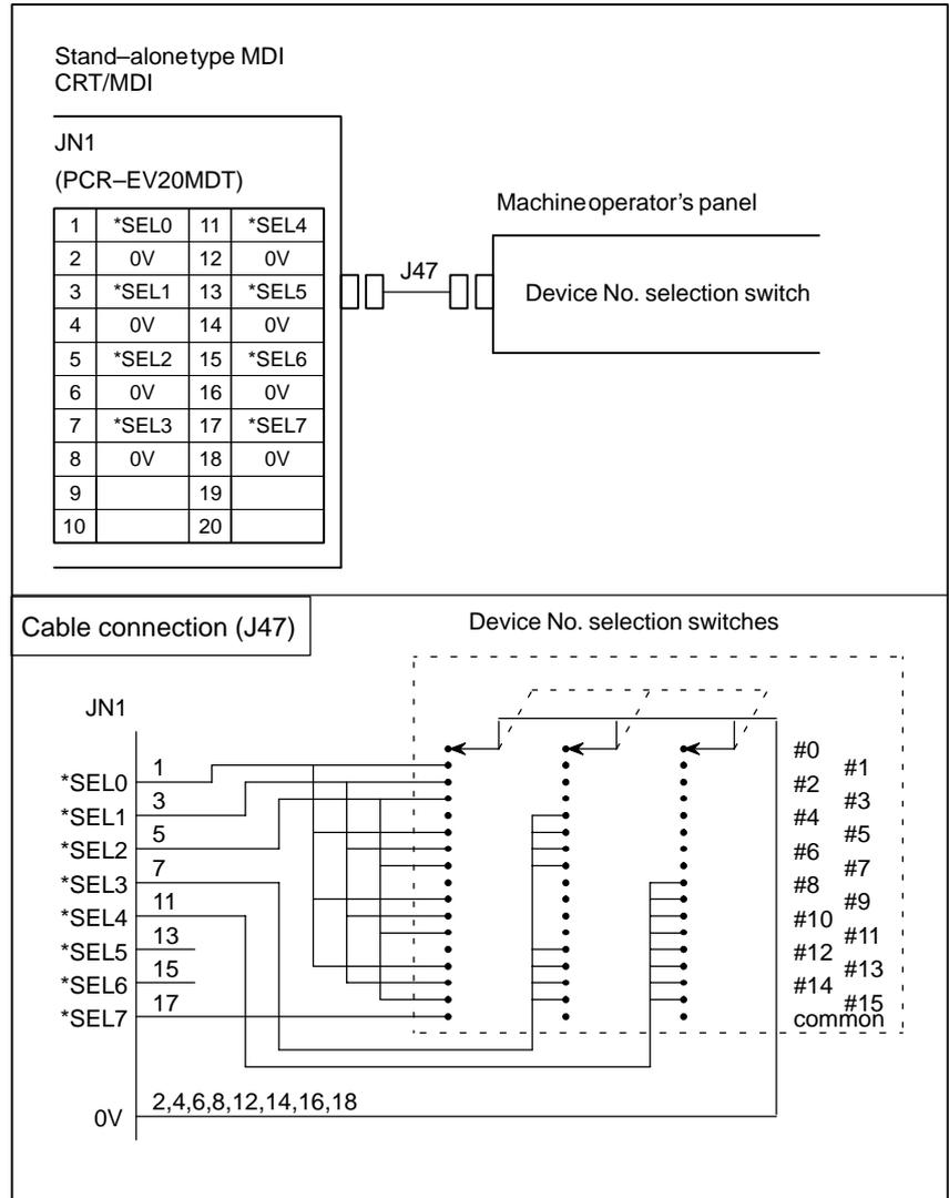
If the total length of the display link cables is 50 to 100 m, connect \*SEL5 to a potential of 0 V. This total length should include all display interface cables. If the total length exceeds 50 m, the Power Mate cannot be made detachable.
