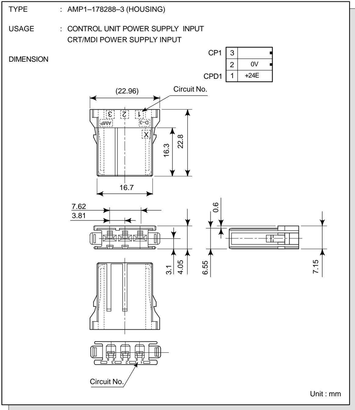
**Fig. 8** AMP Connector (2) type Y
