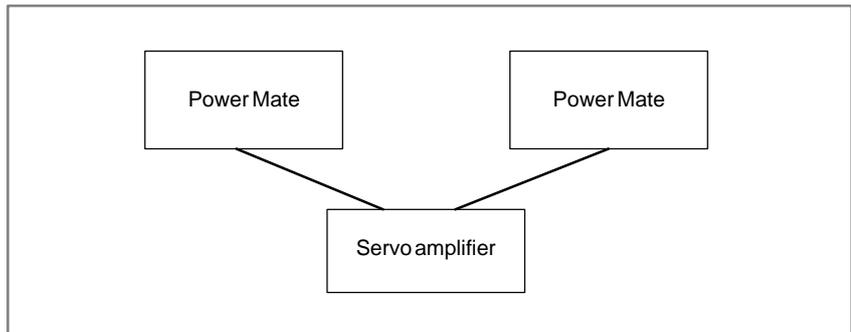
The servo amplifier does not turn on the servo amplifier ready signal until all the Power Mates have started.
