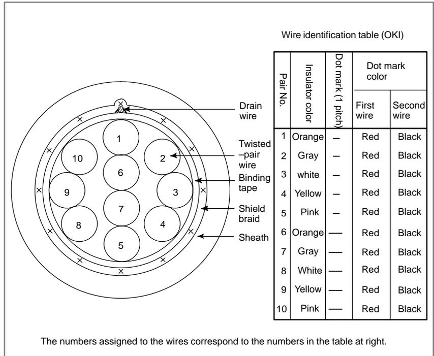
Fig. C.5 (b) Cable made by Oki Electric Cable
