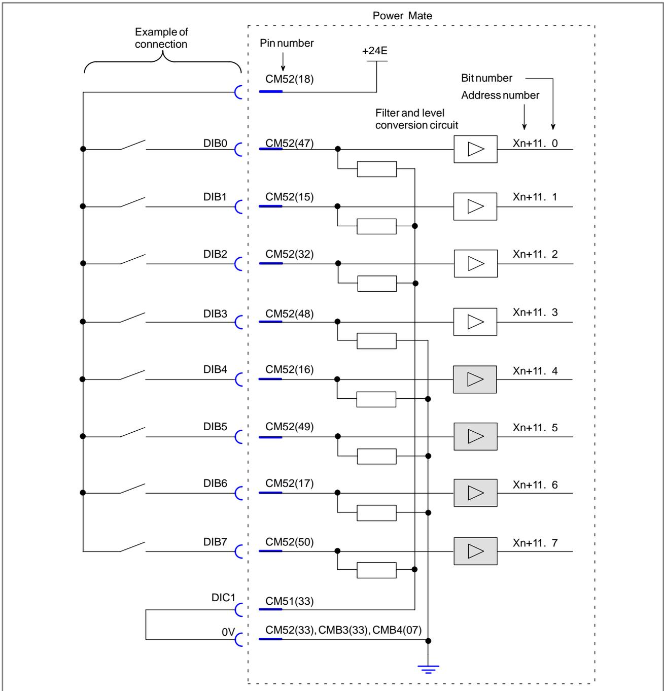
Fig. 6.6.3 (I) I/O card machine interface (12)
