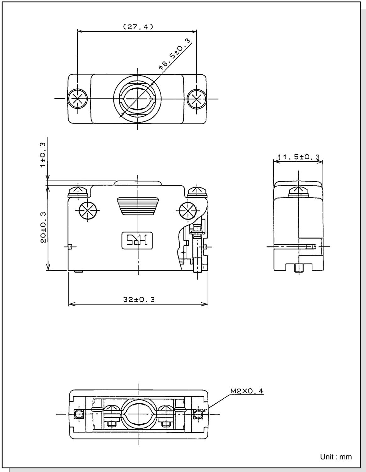
**Fig. 7** AMP Connector (1) type X
