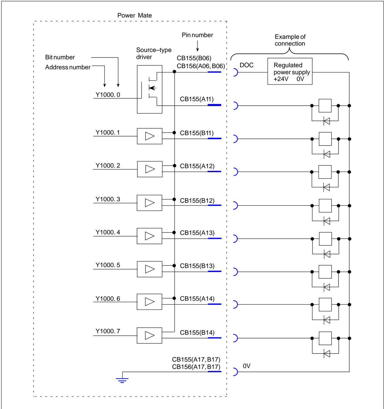
Fig. 6.4.5 (a) Built-in I/O machine interface (5)
