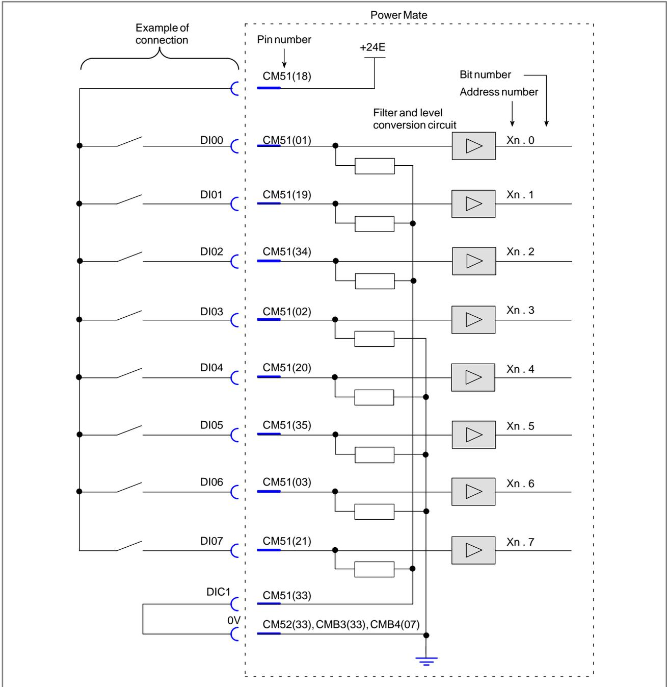
Fig. 6.6.3 (a) I/O card machine interface (1)
