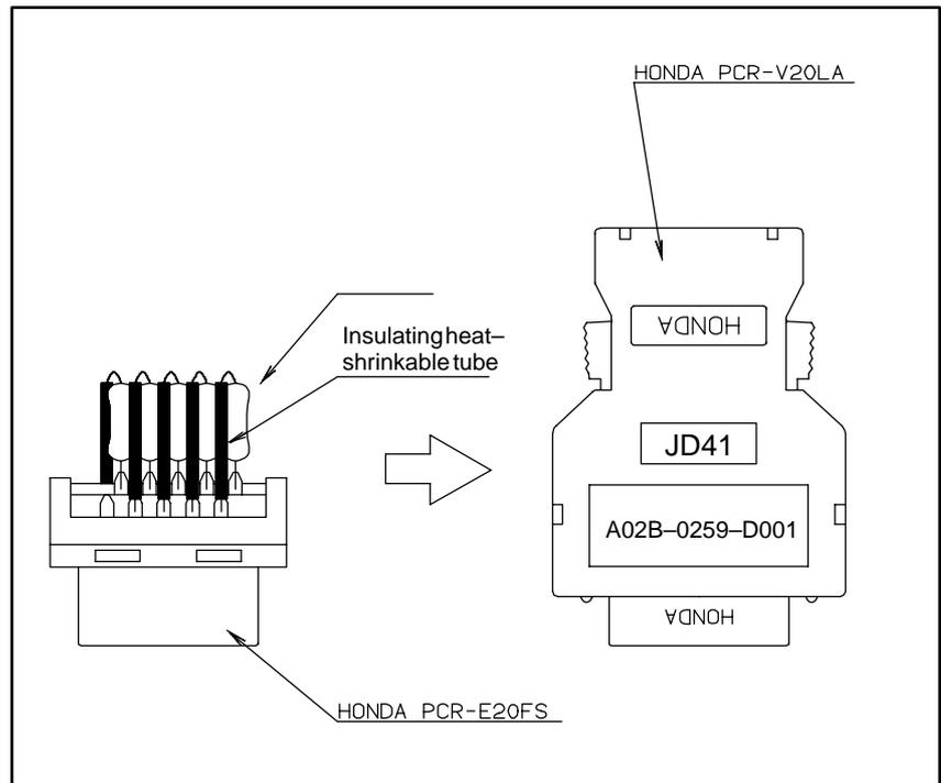
Fig. 8.1.9 Display link terminal unit manufactured by FANUC
