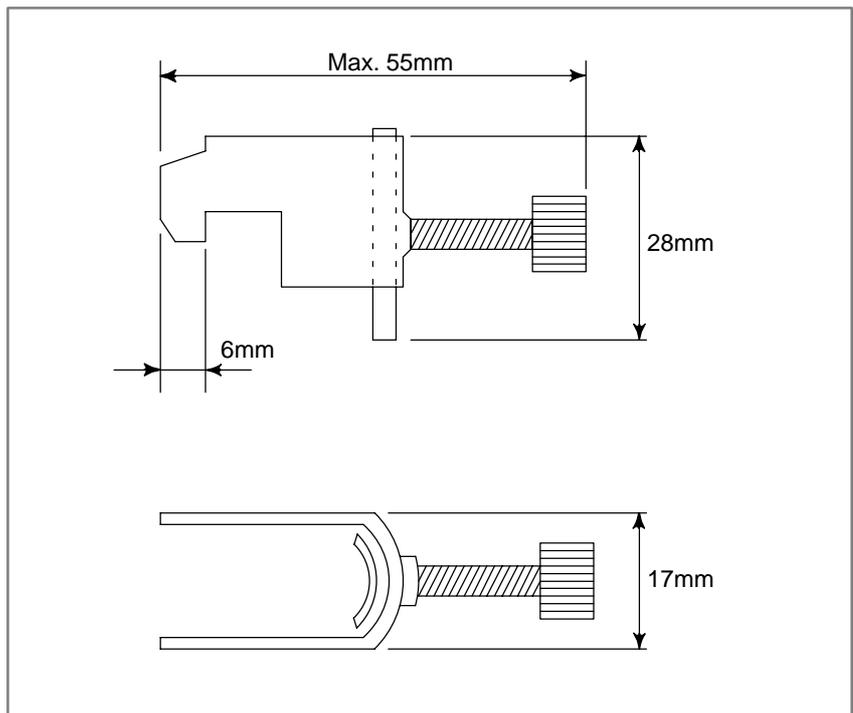
**Fig. 3.6.5 (e) Outer drawings of metal fittings for clamp**
