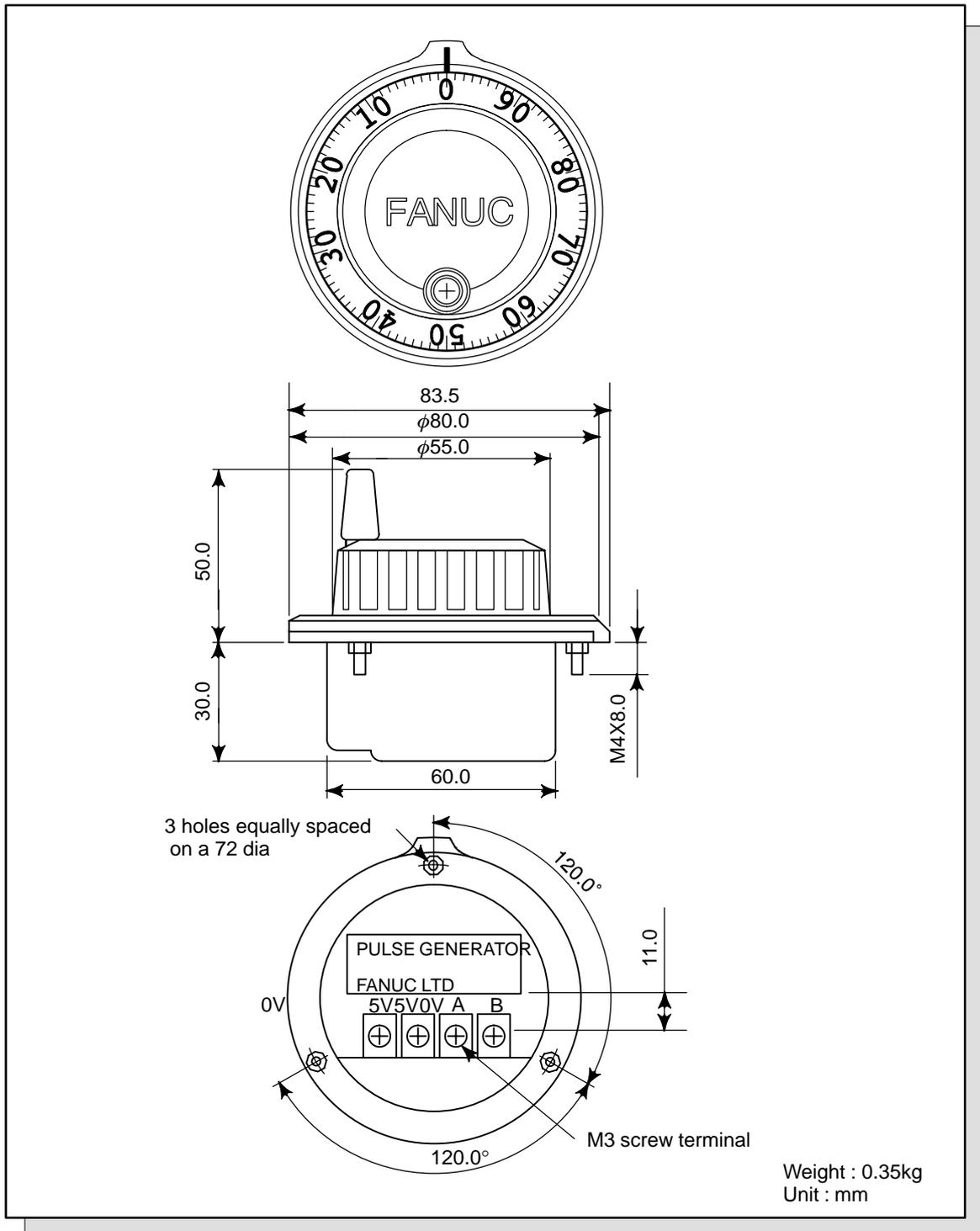
**Fig. 14** Manual pulse generator (Pendant type)
