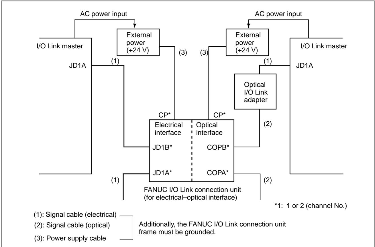
[Name of I/O Link connection unit connectors]
