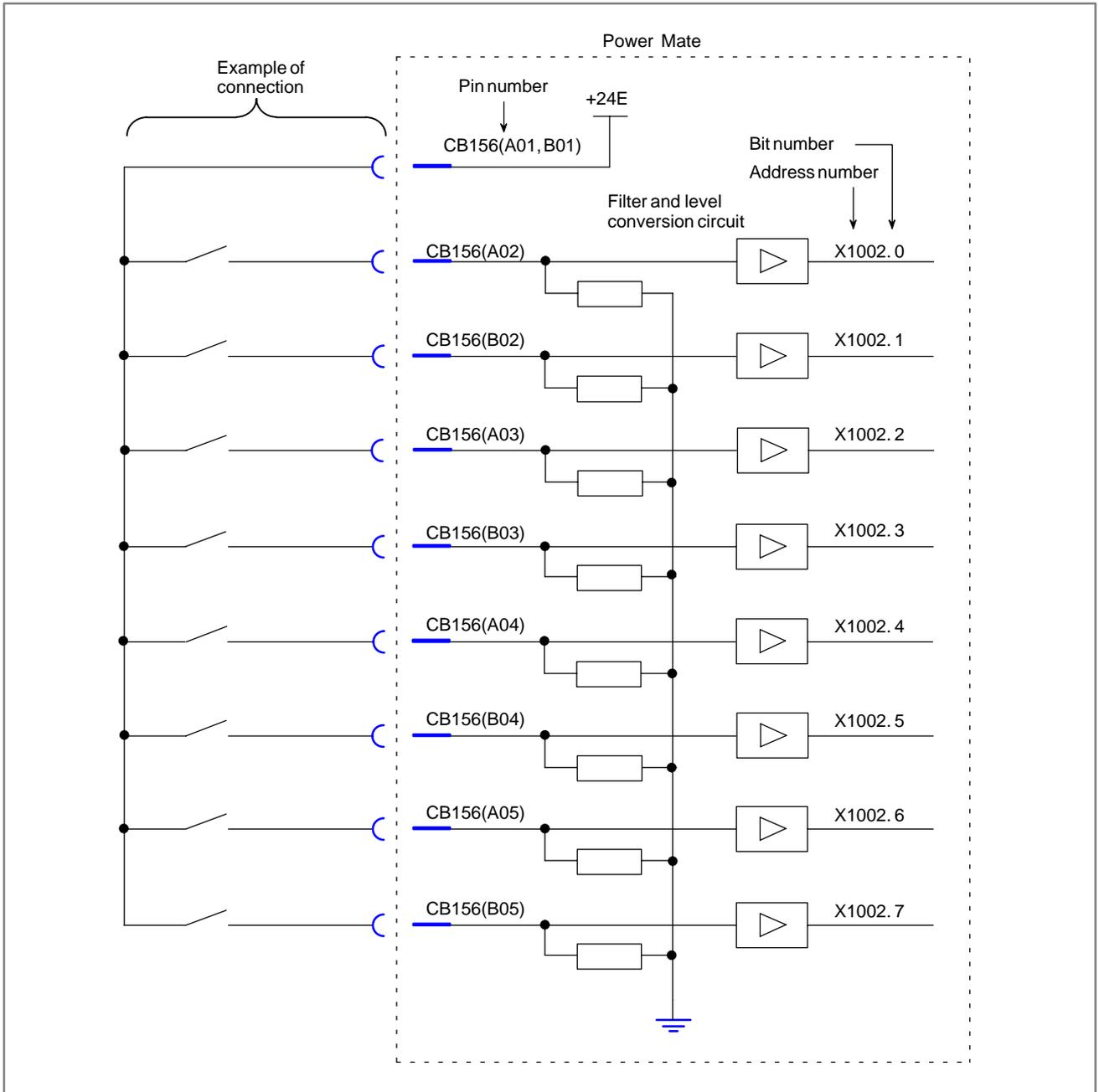
Fig. 6.4.4 (c) Built-in I/O machine interface (3)
