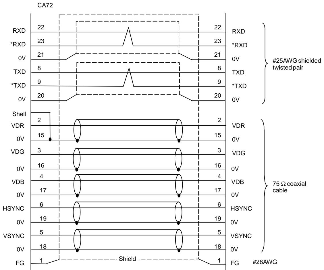
Recommended cable: A66L-0001-0450 (#25AWG shielded twisted pair × 2, 75 Ω coaxial cable × 5, common shield)
