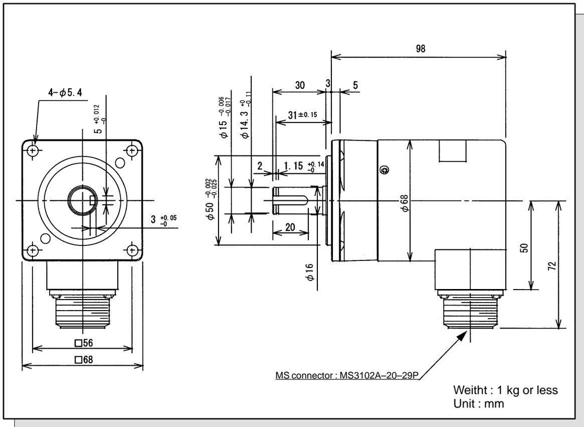
**Fig. 13** Manual pulse generator
