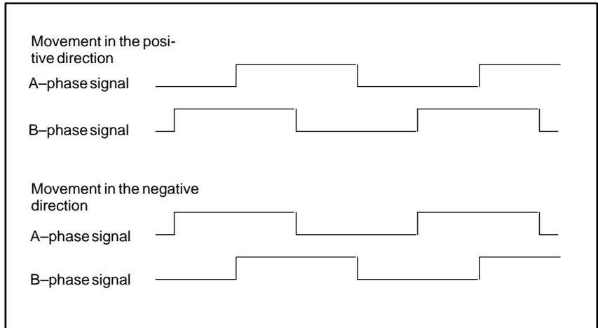
The differential input signals shown below are applied to the connectors. The time duration,  $T_D$ , from point  $\alpha$  where the relative potential difference between A and \*A becomes 0.5 V or more, to point  $\beta$  where the relative potential difference between B and \*B becomes 0.5 V or less, must satisfy the condition indicated below. (This condition may restrict the maximum speed of movement.)
