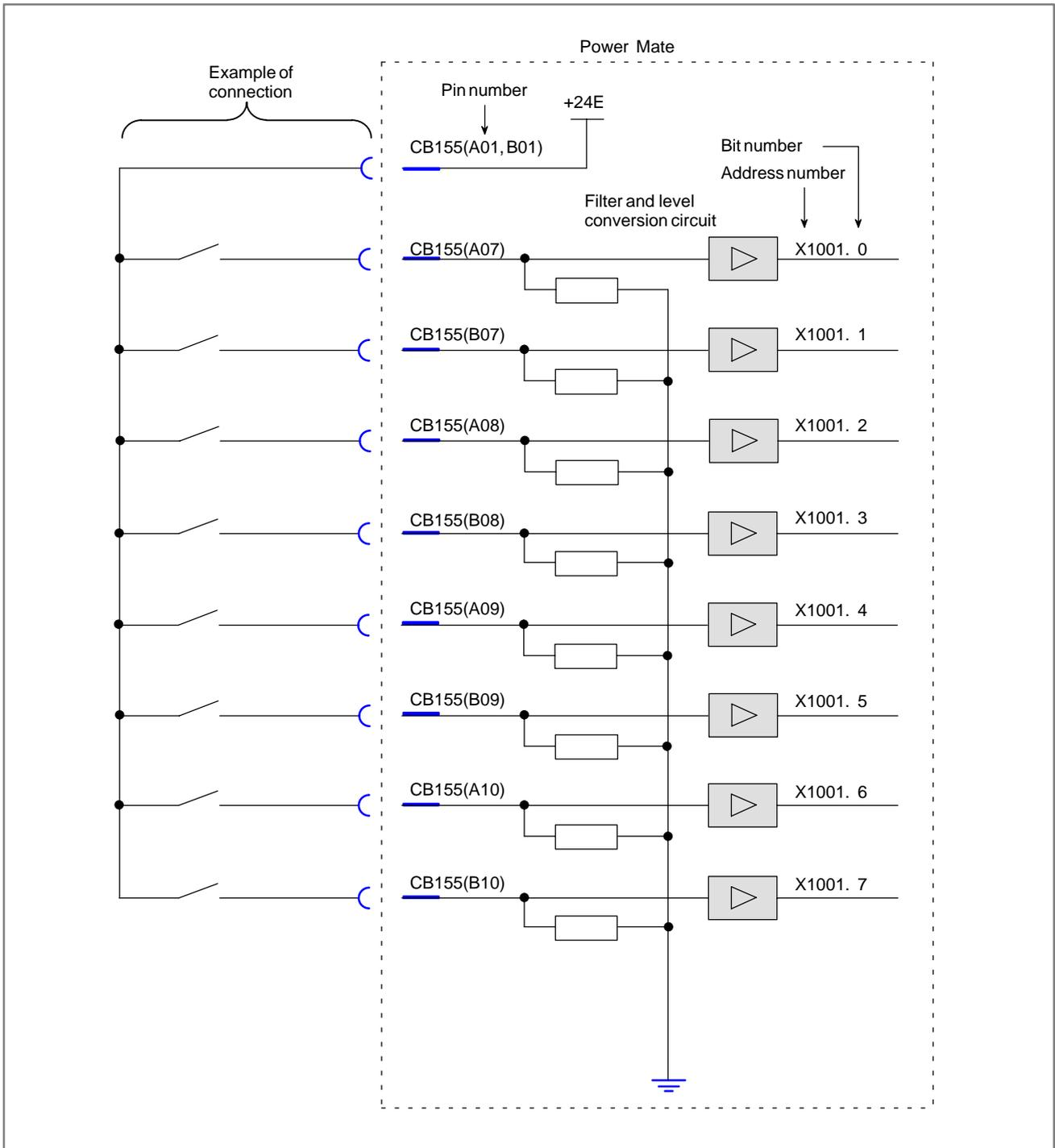
Fig. 6.4.4 (b) Built-in I/O machine interface (2)
