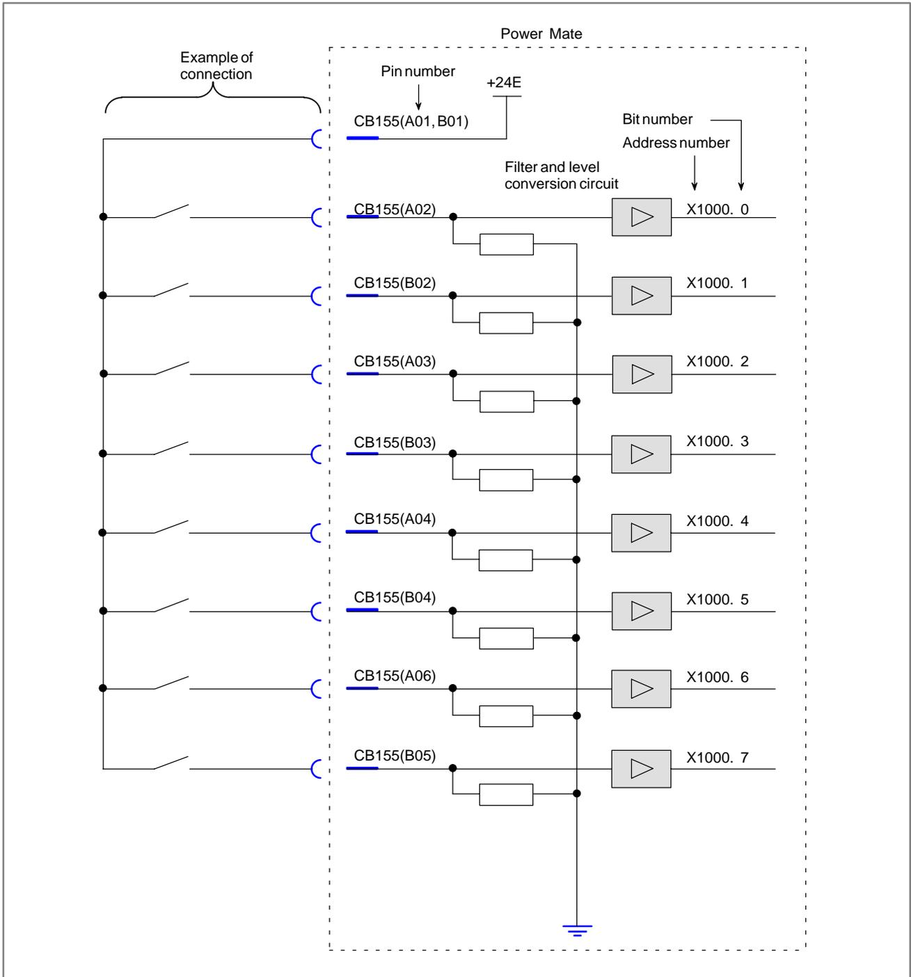
Fig. 6.4.4 (a) Built-in I/O machine interface (1)
