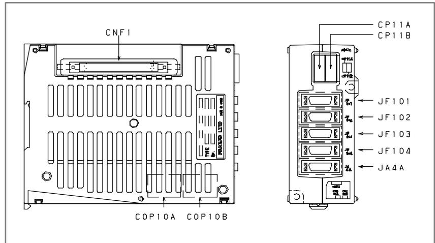
Positions of the connectors of an additional unit
