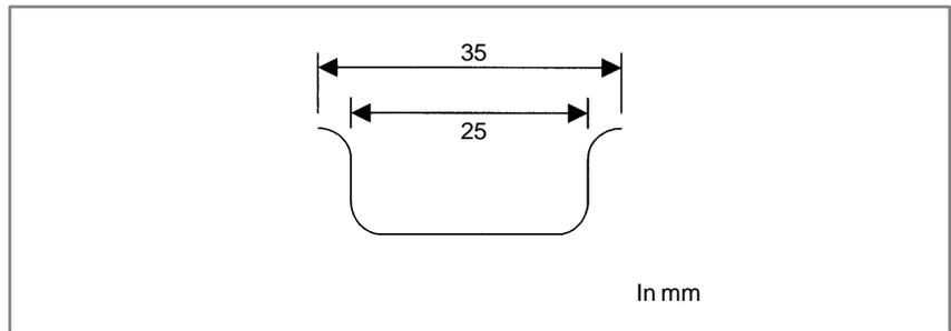
**Fig. 8.1.10 (b) Recommended DIN rail**
