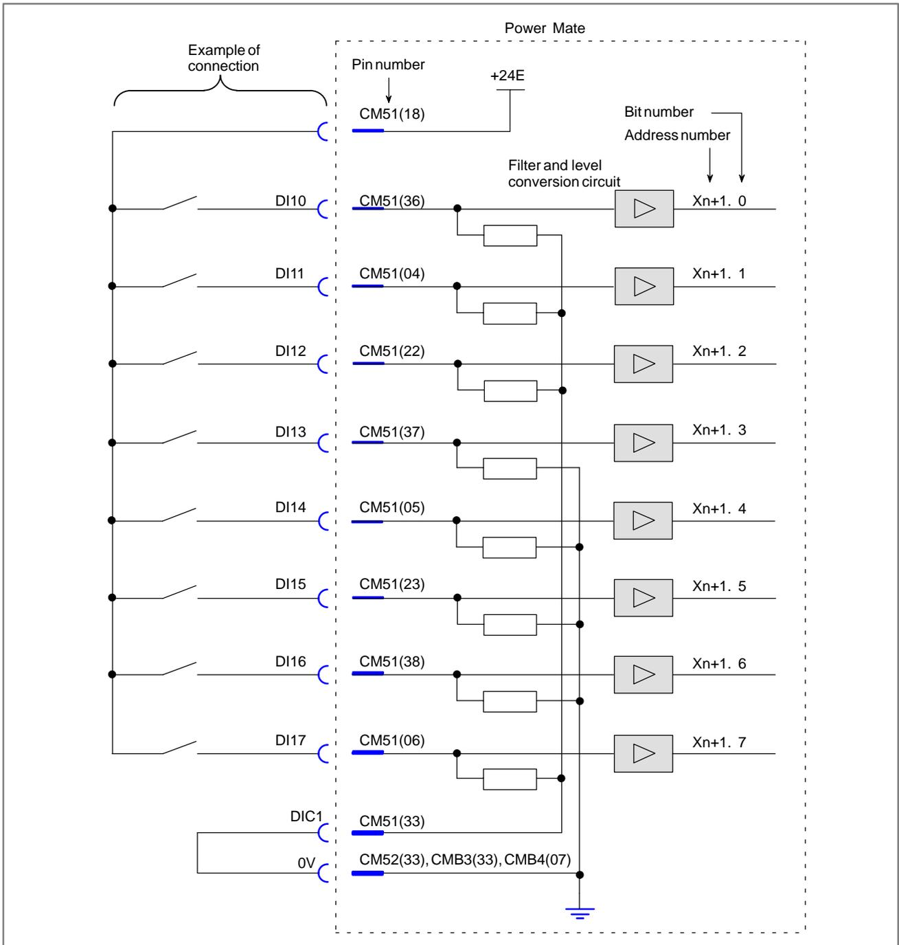
Fig. 6.6.3 (b) I/O card machine interface (2)
