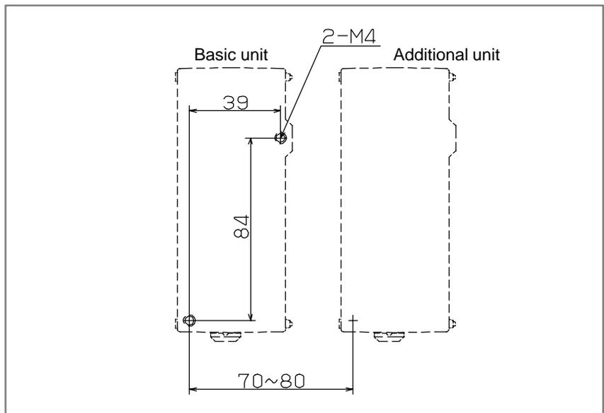
**Mounting hole drilling diagram**
