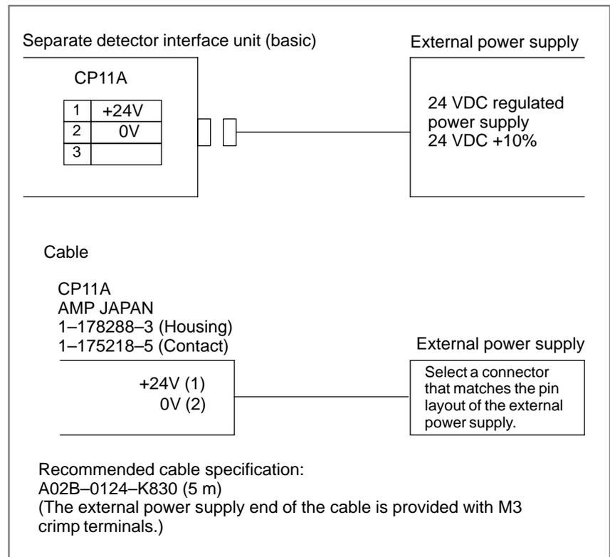
The 24 VDC input to CP11A can be output at CP11B for use in branching. The connection of CP11B is identical to that of CP11A.
