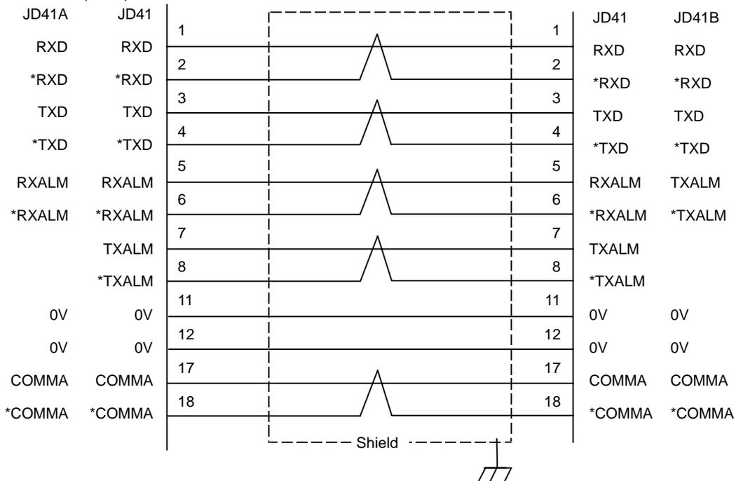
Recommended cable: A66L-0001-0284#10P (#28AWG 10 pairs, common shield)
