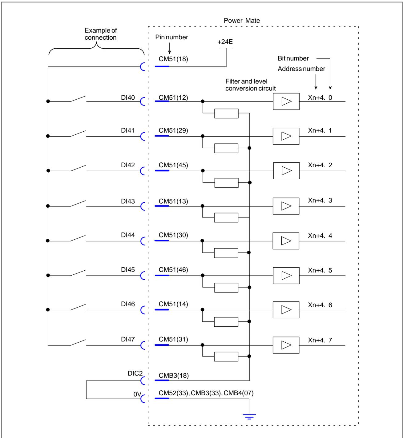
Fig. 6.6.3 (e) I/O card machine interface (5)
