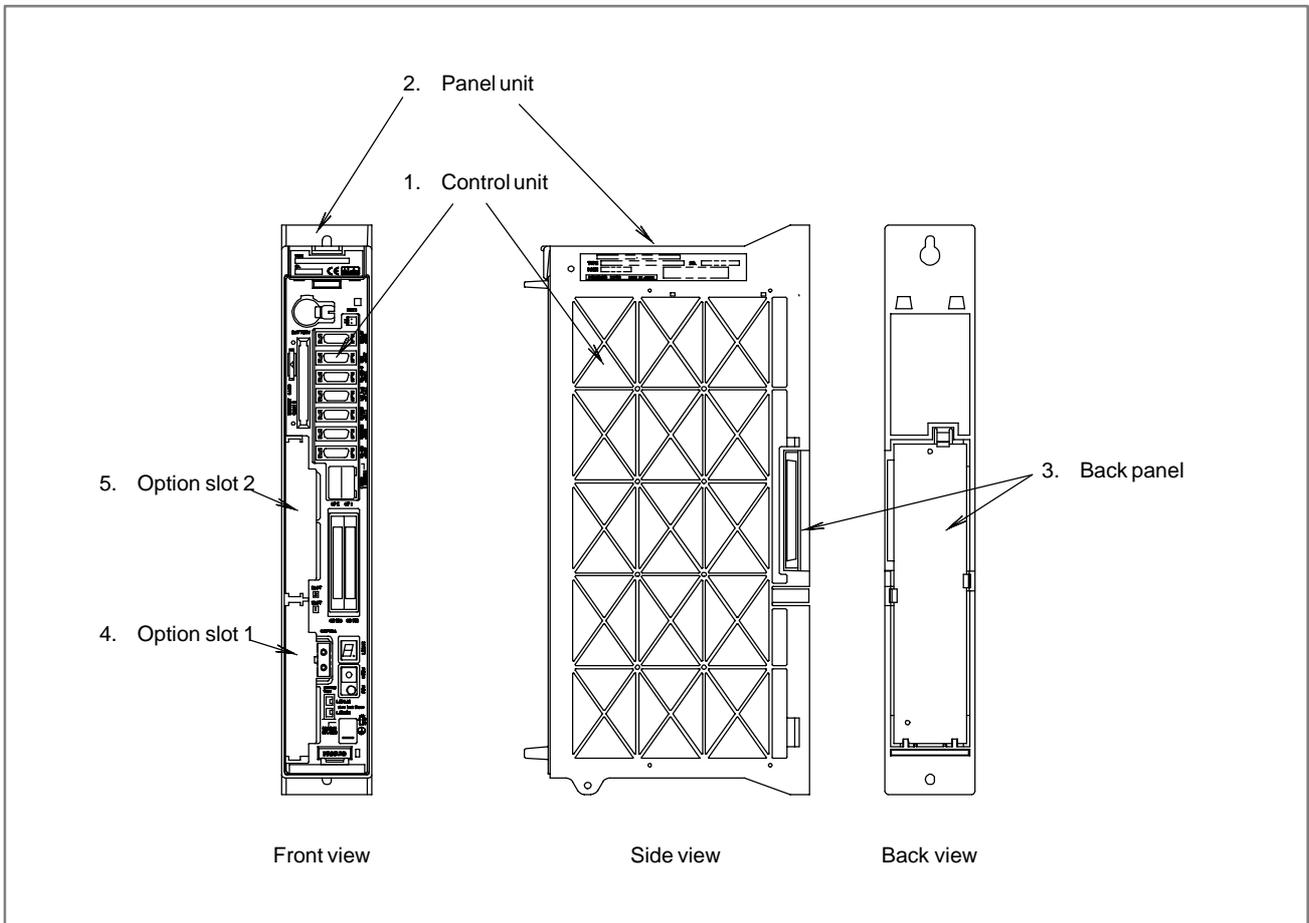
**Fig. 3.7.1 Configuration of the control unit**
