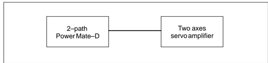
The servo amplifier does not turn on the servo amplifier ready signal until both paths of the two-path Power Mate *i*-D have been started.
