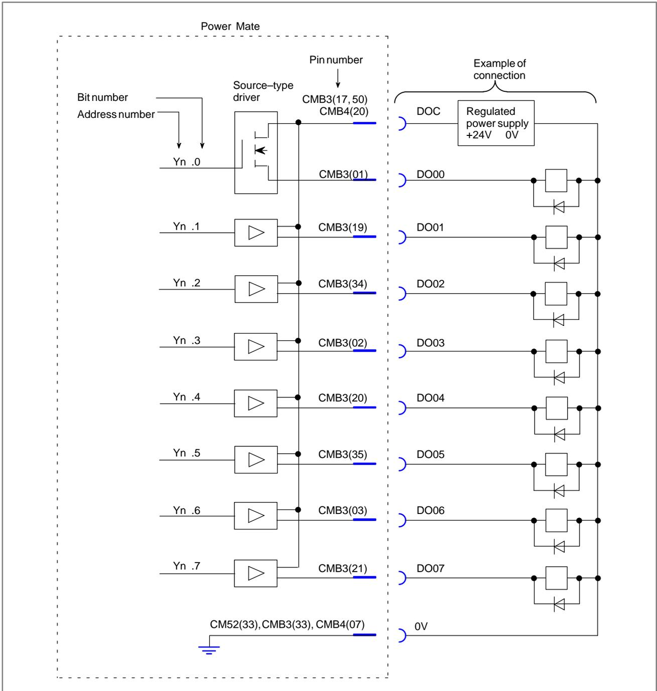
Fig. 6.6.4 (a) I/O card machine interface (13)
