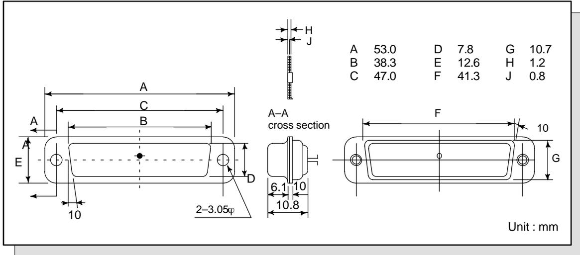
**Fig. 18** RS-232-C serial port connector metal fitting for lock
