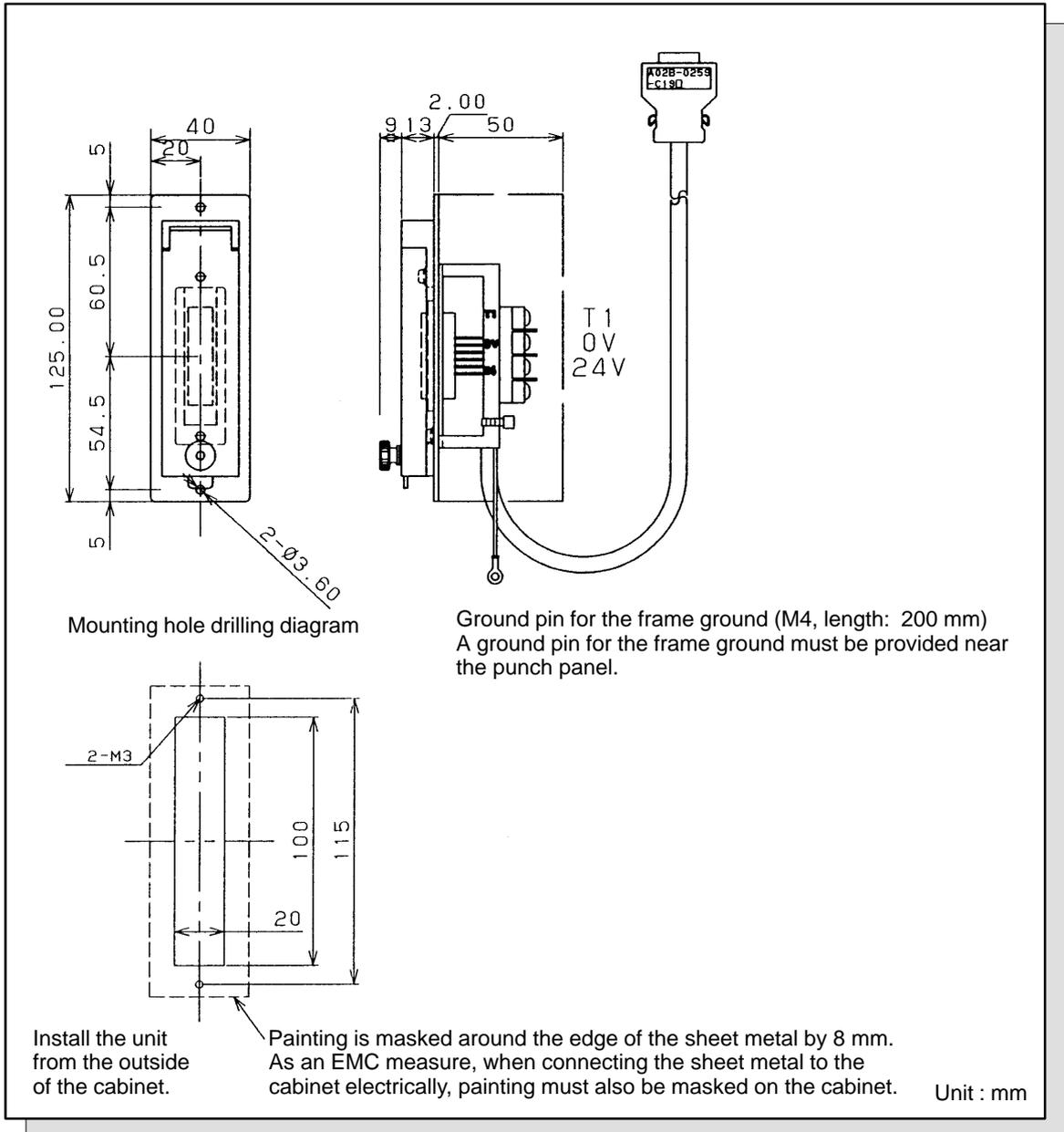
**Fig. 19** Punch panel (for 2 channels)
