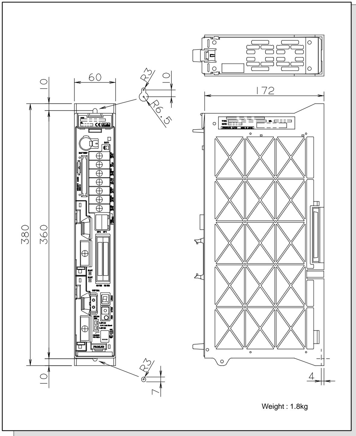
**Fig. 3** FSSB I/O Module
