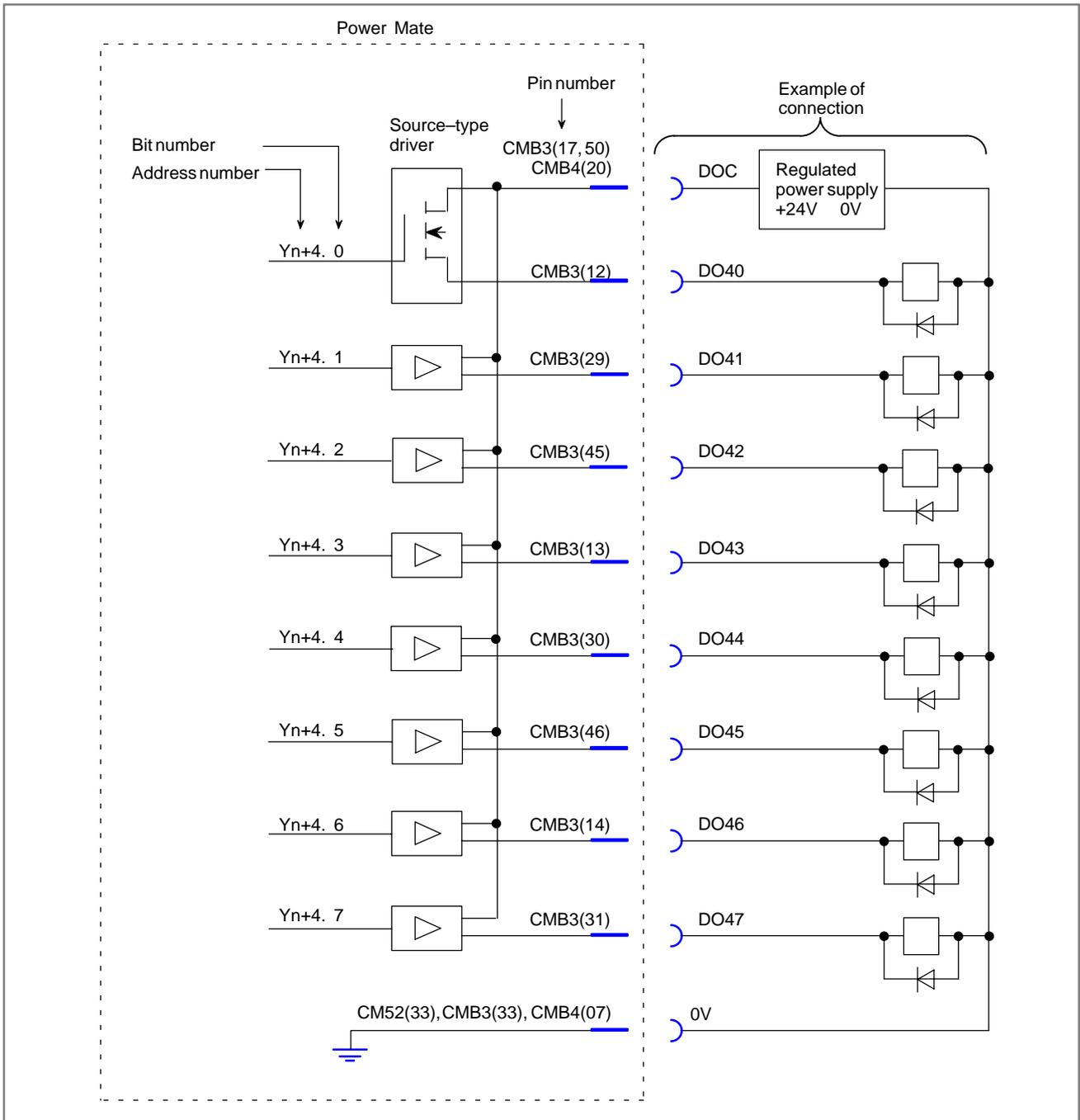
Fig. 6.6.4 (e) I/O card machine interface (17)
