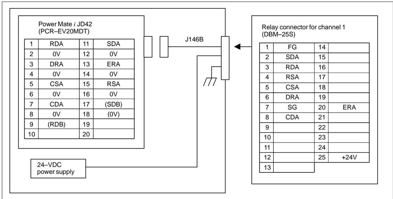
Relay connector (FANUC purchase specification: A02B-0061-K201)
