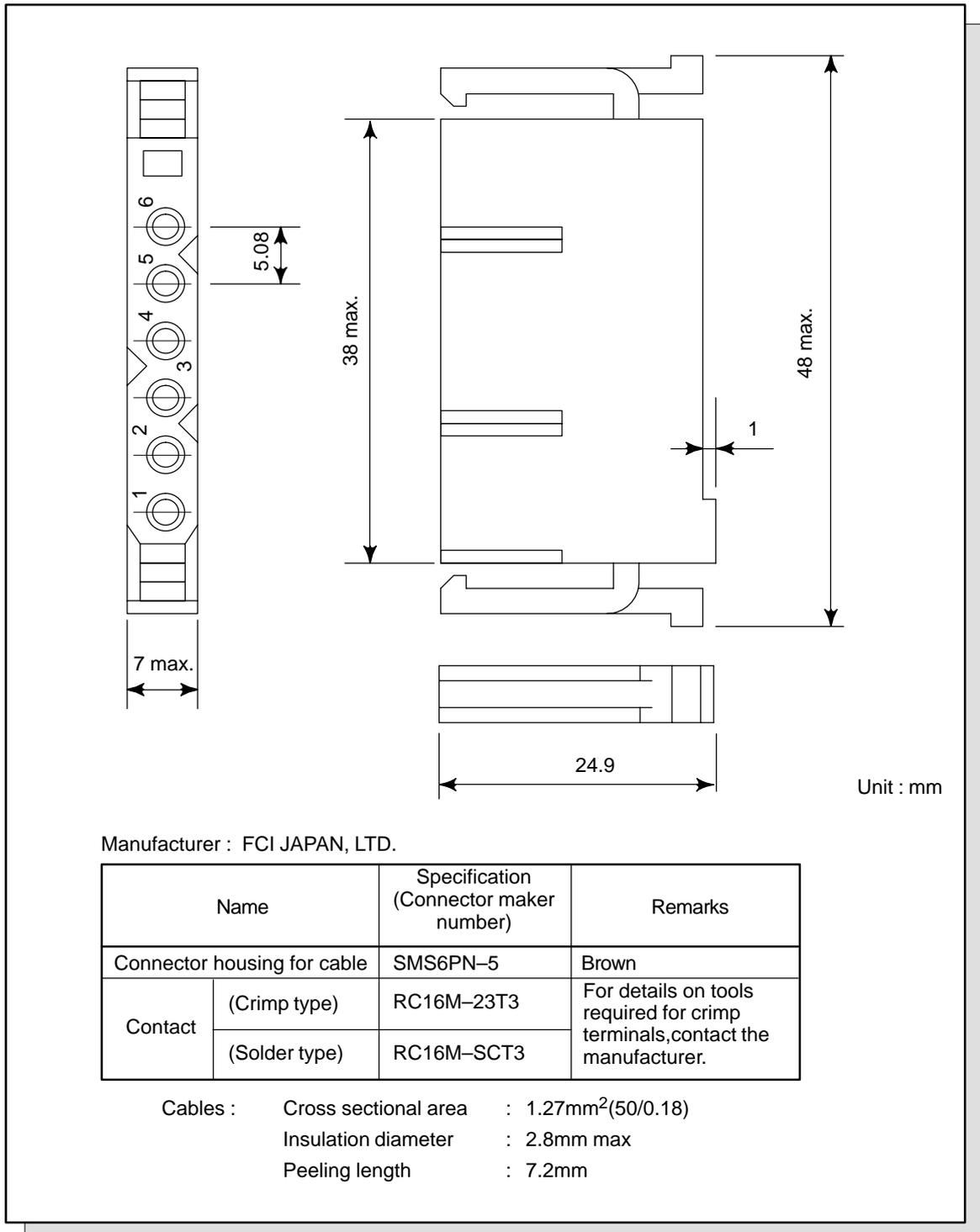
**Fig. 17** Punch panel connector for RS-232-C serial port
