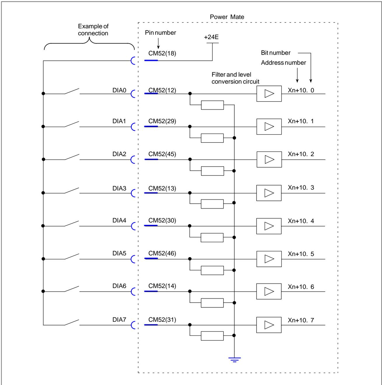
Fig. 6.6.3 (k) I/O card machine interface (11)
