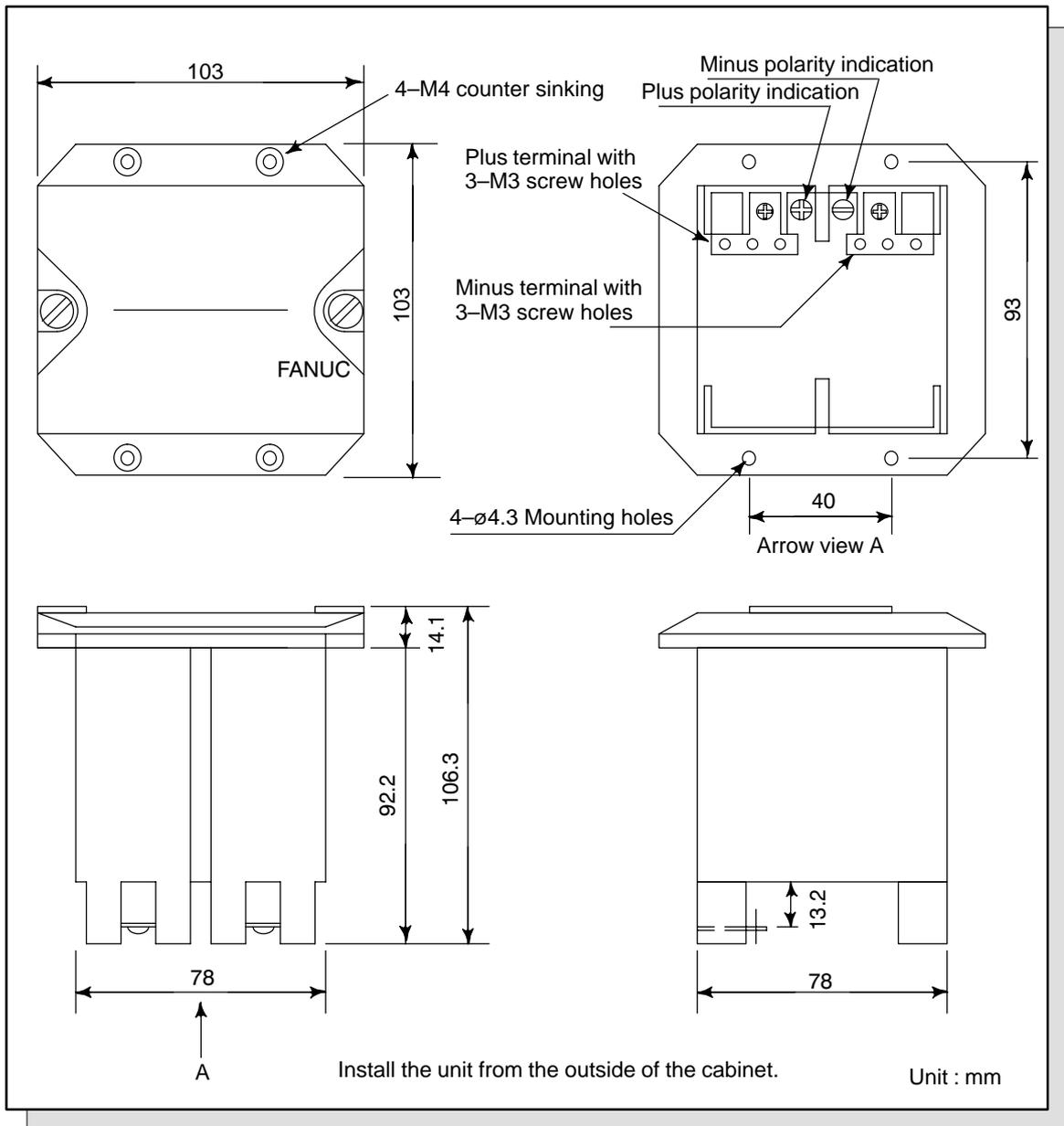
**Fig. 17** Battery case for external control unit
