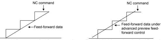
Fig. 4.6.2 (a) Conventional feed-forward control
