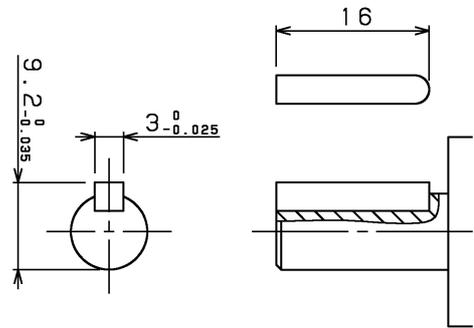
**Fig.2.4(e) Models  $\beta$ M0.4,  $\beta$ M0.5, and  $\beta$ M1 : Outline drawing (with a brake)**
