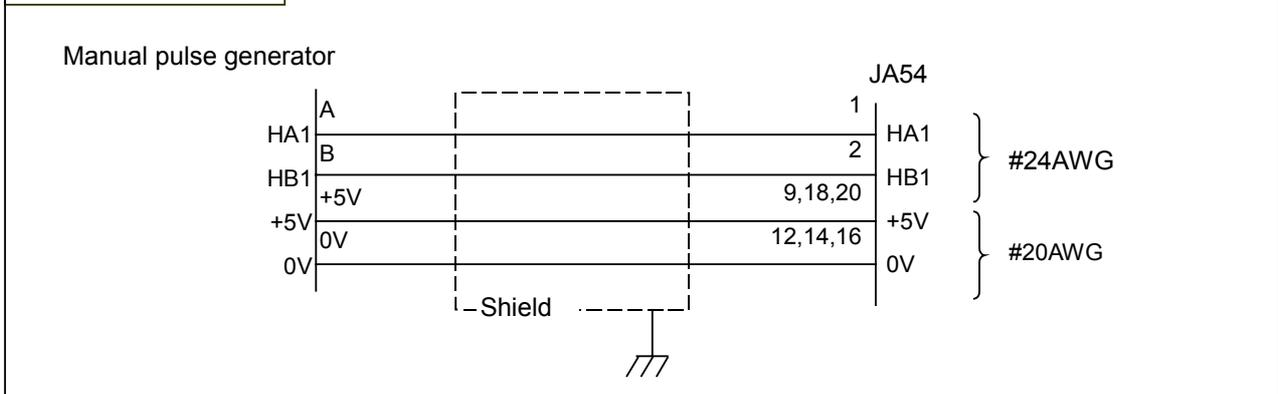
Recommended wire : A66L-0001-0286 (#20AWG × 6 + #24AWG × 3 pairs)
