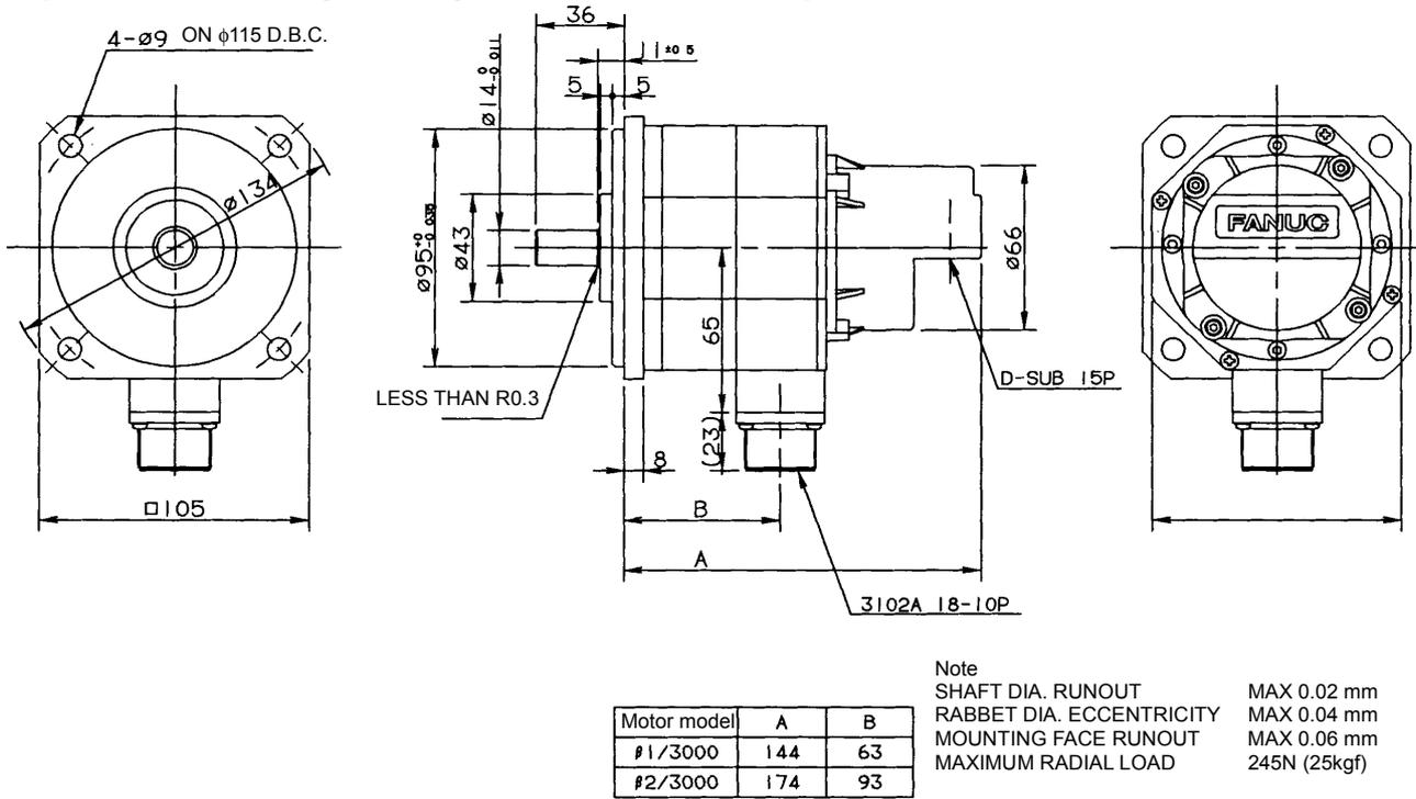
Fig.2.4(b) Models  $\beta 1$  and  $\beta 2$  : Outline drawing (with a brake)
