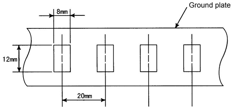
Fig.7.3.4(d) Ground plate holes
