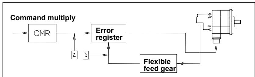
In the above figure, each ratio is set so that the units of the two inputs (a and b) of the error register are the same. The β pulse coder uses a flexible feed gear as standard. So, CMR is normally set to 1. When other than 1 is to be set for CMR, contact FANUC for details.
