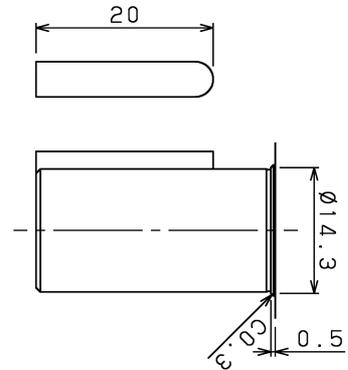
Fig.2.4(h) Models  $\beta$ M0.4,  $\beta$ M0.5, and  $\beta$ M1 : Connector mating diagram (elbow)
