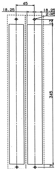
When two units of natural air cooling type are installed in parallel
