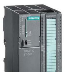
SIMATIC S7-300, CPU 313C-2 DP Compact CPU with MPI, 16 DI/16 DO, 3 high-speed counters (30 kHz), integrated DP interface, Integr. power supply 24 V DC, work memory 128 KB, Front connector (1x 40-pole) and Micro Memory Card required
