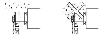
• Prevent the cutting fluid from being led to the motor through the cable. When the motor connector is used in the up position, put a drip loop in the cable.
