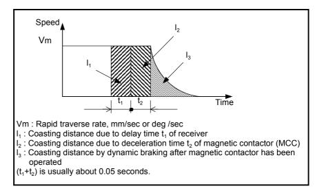
Coasting distance due =  $Vm \times (t_2 + t_2) + (Jm + J_L) \times (A \times No + B \times No^3) \times L$ [mm] or [deg]
