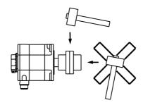
Suppress the rotary unbalance of the connected power transmission element to the level as low as possible. It is usually believed that there is no problem in the symmetrical form. Be careful when rotating continuously the asymmetrical different form power transmission element. Even if the vibration caused by the unbalance is as small as 0.5G, it may damage the motor bearing or the sensor.
