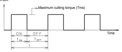
t<sub>ON</sub> : Time maximum cutting torque (Tmc) is applied
