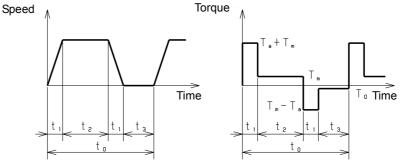
From the time-torque graph, obtain the root-mean-square value of torques applied to the motor during the single operation cycle. Check whether the value is smaller than or equal to the torque at stall (condition 3).
