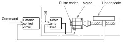
This method is shown in the figure above by block diagram. The response of this control system is determined by the adjustment value (position loop gain) of the position control circuit. In other words, the position loop gain is determined by the specified response time of the control system. In the diagram above, the section enclosed by the broken line is called the velocity loop.
