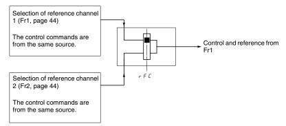
Use parameter rFC (page 45) to select reference channel Fr1 or Fr2, or to configure a logic input or a control word bit for remote switching between the two channels. Refer to the diagram on page 42.
