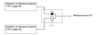
Use parameter rFC (page 45) to select reference channel Fr1 or Fr2, or to configure a logic input or a control word bit for remote switching between the two channels.
