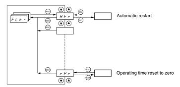
Fault Menu parameters can only be modified when the drive is stopped and no run command is present.
