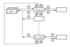
The Communication menu parameters can only be modified when the drive controller is stopped and no run command is present. Modifications to parameters Add, tbr, tFO, AdCO, and bdCO take effect only after a restart.
