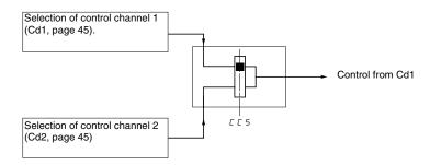
Use parameter CCS (page 46) to select control channel Cd1 or Cd2, or to configure a logic input or a control word bit for remote switching between the two channels.
