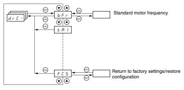
With the exception of tUn, drive control parameters can only be modified when the drive controller is stopped and no run command is present. This menu can be accessed with the access locking switch on the remote keypad display in the  $\Box$  position. Drive controller performance can be optimized by:
