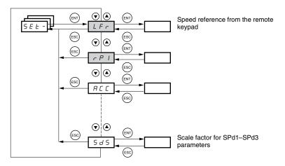
The parameters in the SEt- menu can be modified with the drive controller running or stopped. However, we recommend making modifications to the settings with the drive controller stopped.
