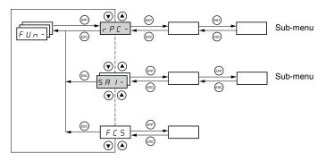
Application function parameters can only be modified when the drive controller is stopped and with no run command present. On the remote keypad display, this menu can be accessed with the access locking switch in the  $\ \cap$  position.
