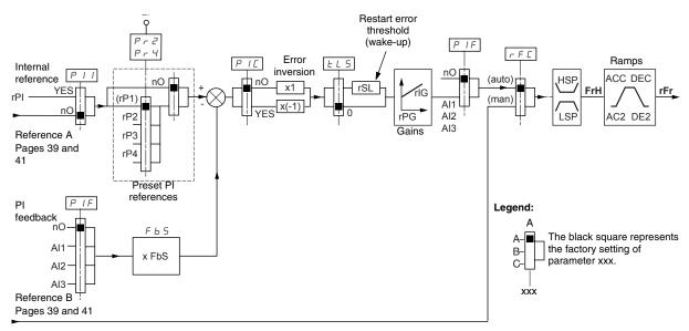
The **PI regulator feedback** parameter (PIF, see page 66) must be assigned to one of the analog inputs (AI1, AI2, or AI3).
