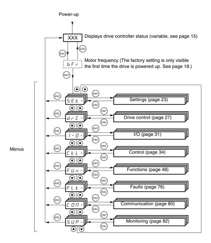
For added convenience, some parameters can be accessed in more than one menu. For example, return to factory settings (FCS) and saving the configuration (SCS) are available in multiple menus.
