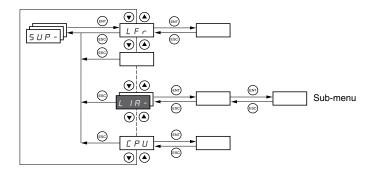
The display menu parameters can be accessed with the drive controller running or stopped. This menu can be accessed with the access locking switch on the remote keypad display in any position.
