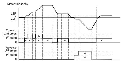
Use of double action buttons is incompatible with 3-wire control.
