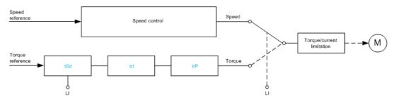
The function can be used to switch between operation in speed regulation mode and operation in torque control mode.
