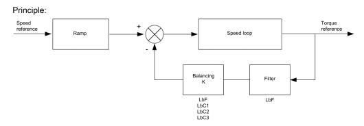
The load sharing factor K is determined by the torque and speed, with two factors K1 and K2 ( $K = K1 \times K2$ ).
