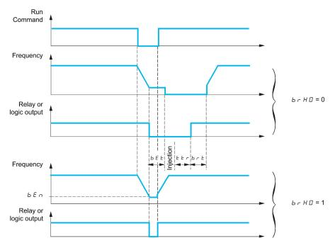
**NOTE:** if a run command is requested during the **[Time to restart]** *E E r* phase, the complete brake control sequence is initialized.
