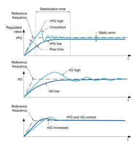
The oscillation frequency depends on the system kinematics:
