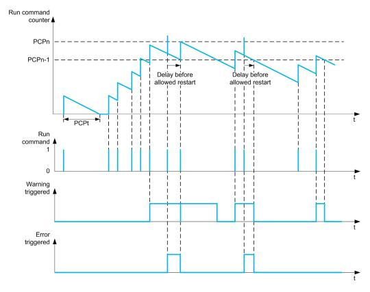
If [PumpCycle Monitoring]  $P \ \Box P \ \Pi$  is set to [Mode 1]  $n \ \Box r \ \Pi$ , the function is activated without power Off time management.
