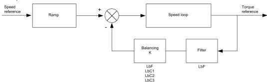
The load sharing factor K is determined by the torque and speed, with two factors K1 and K2 (K = K1 x K2).
