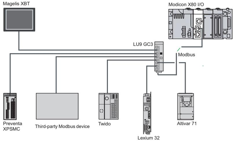
The Modbus serial link is used for master/slave architectures (it is necessary, however, to check that the Modbus services used by the application have been implemented on all relevant devices).
