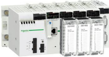
Ethernet Modbus/TCP DIO drop with PRA module
