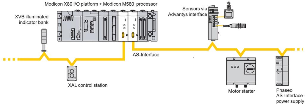
The AS-Interface cabling system consists of a master station (Modicon X80 I/O platform) and slave stations. The master supporting the AS-Interface profile interrogates the devices connected on the AS-Interface line one-by-one and stores the information (actuator/sensor status, device operating status) in the PLC memory. Communication on the AS-Interface line is managed totally transparently in relation to the application PLC program.
