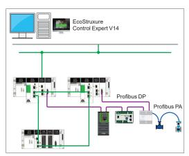
Redundant (HSBY) topology to connect the Profibus DP master X80 module to M580/X80 platforms with PMEPXM0100
