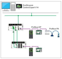
Standalone topology to connect Profibus DP master X80 module to M580/X80 platforms with PMEPXM0100
