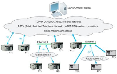
Example of an RTU system architecture
