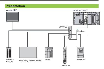
The Modbus serial link is used for master/slave architectures (it is necessary, however, to check that the Modbus services used by the application have been implemented on all relevant devices).
