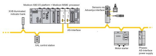
The AS-Interface cabling system consists of a master station (Modicon X80 I/O platform) and slave stations. The master supporting the AS-Interface profile interrogates the devices connected on the AS-Interface line one-by-one and stores the information (actuator/sensor status, device operating status) in the PLC memory. Communication on the AS-Interface line is managed totally transparently in relation to the application PLC program.
