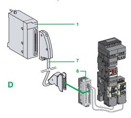
Example of connection to the TeSys Quickfit installation system
