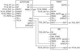
Example: PID controller with MS manual control
