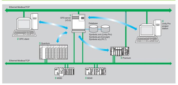
The OFS server 1 is at the center of the data exchanges. It makes variables exchanged between the OPC client 2 and the PAC 3 consistent in one of three ways, using a symbol (or variables) database:
