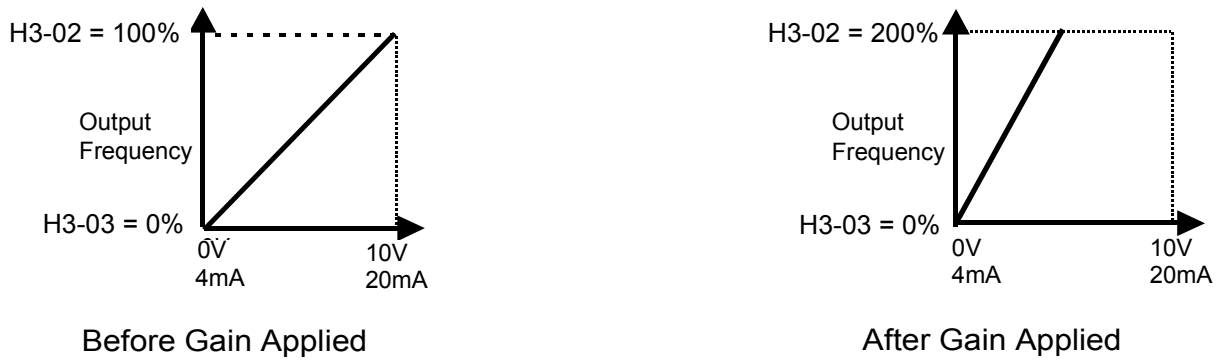
Fig 5.14 Terminal A1 and A2 Analog Inputs Gain Adjustment Example
