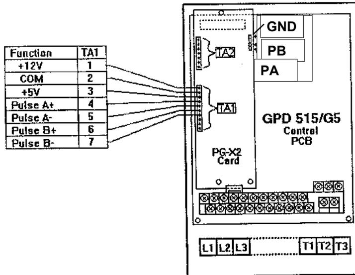
Using channel 1 of the oscilloscope, connect the probe between the test pins labeled "PA" and "Gnd" located on the PG-X2 option card. Connect the test probe attached to channel 2 to test pins "PB" and "Gnd" also on the PG-X2 card.
