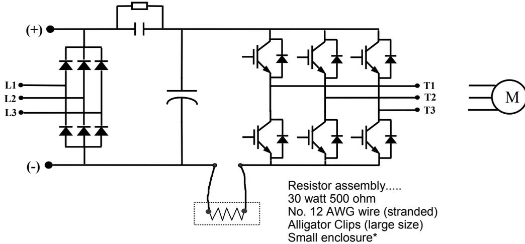
\* In case of a short, the enclosure will contain the resistor if it fragments.
