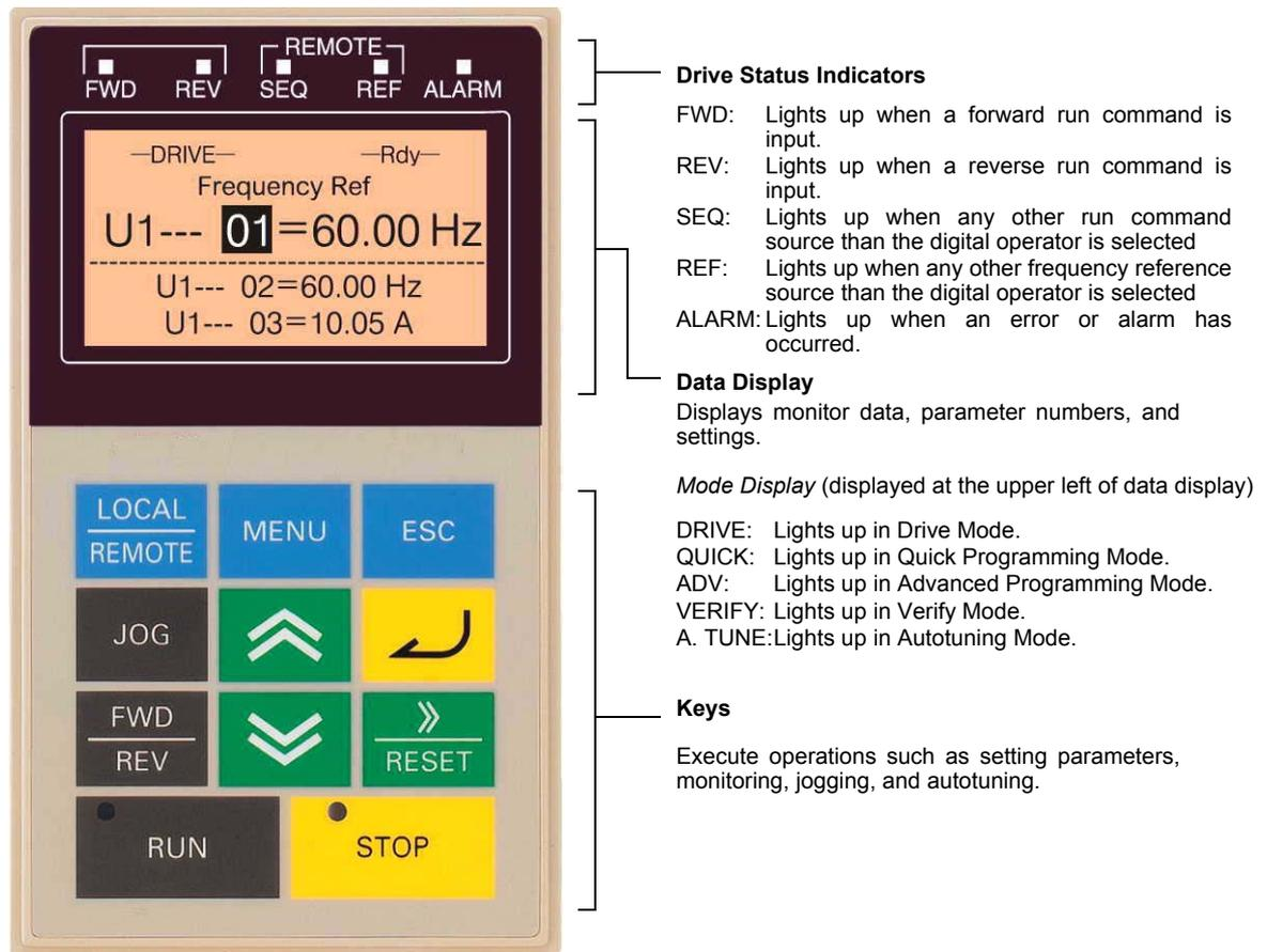
Fig 3.22 Digital Operator Component Names and Functions
