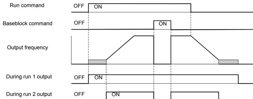
Fig 5.50 Timing Chart for "During RUN" Output
