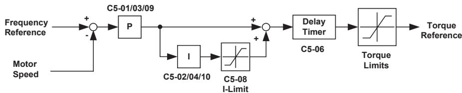
Fig 5.1 ASR Structure Block Diagram
