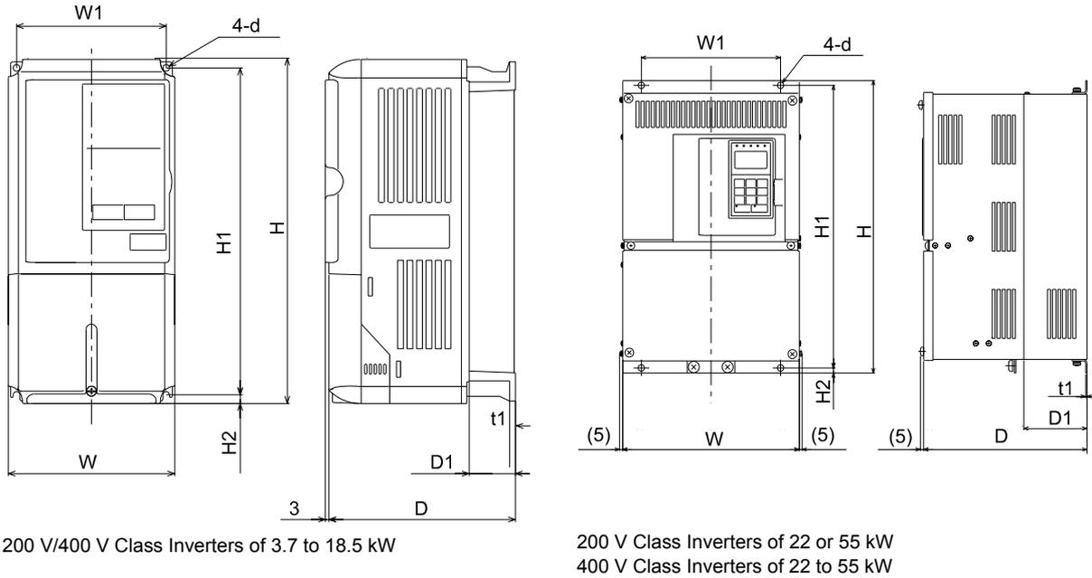
Fig 1.8 Exterior Diagrams of Open Chassis Inverters
