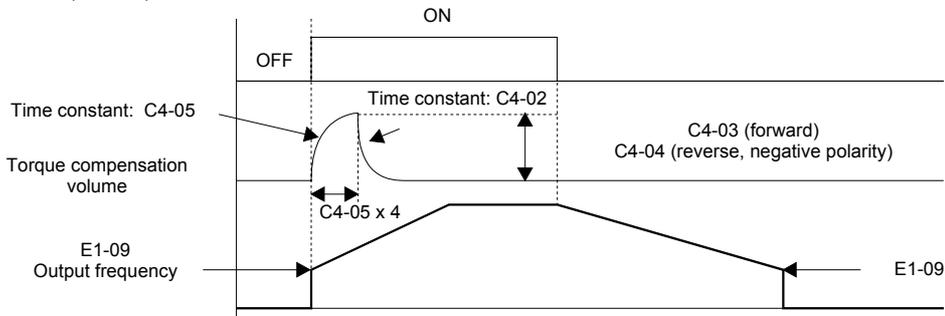
Fig 5.40 Time Chart for Starting Torque Frequency
