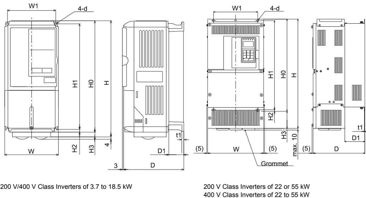
Fig 1.9 Exterior Diagrams of Enclosed Wall-mounted Inverters
