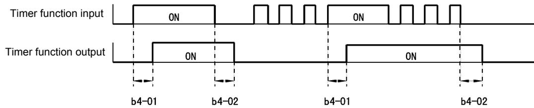
Fig 5.49 Timer Function Operation Example
