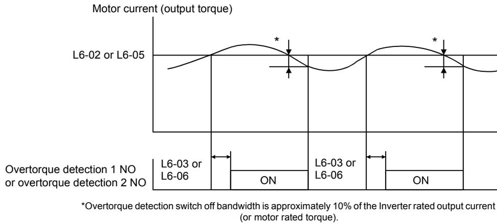
Fig 5.43 Overtorque Detection
