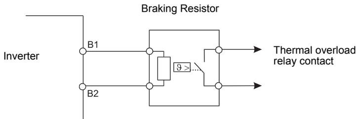
200 V and 400 V Class Inverters with 22 kW or higher Output Capacity
