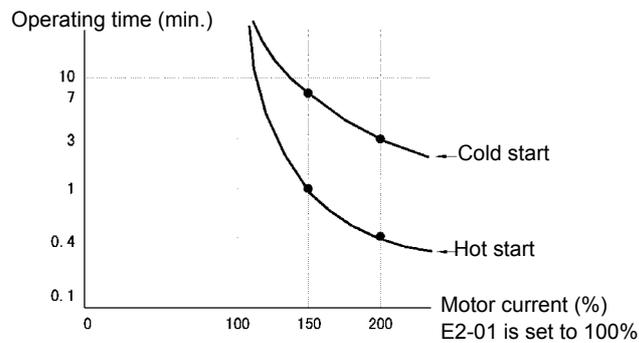
Fig 5.47 Motor Protection Operation Time
