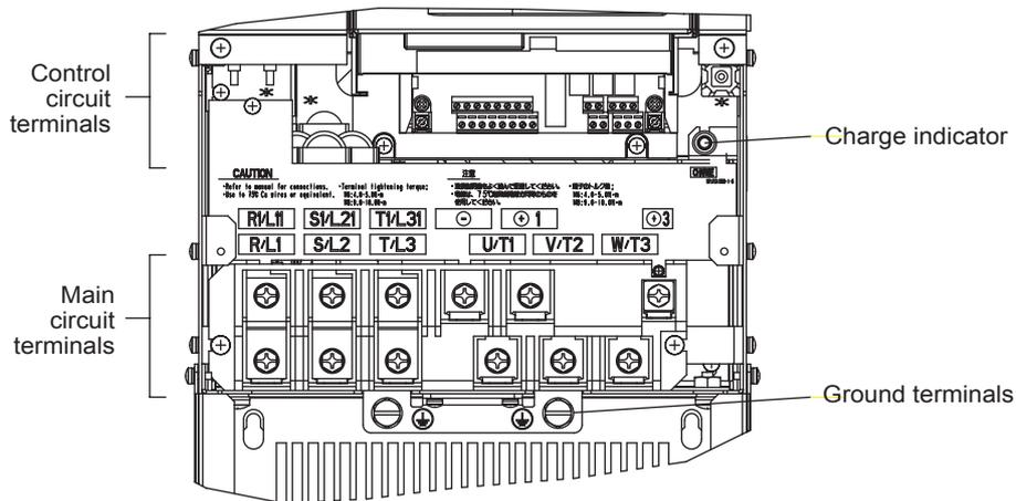
Fig 1.7 Terminal Arrangement (22 kW or More)
