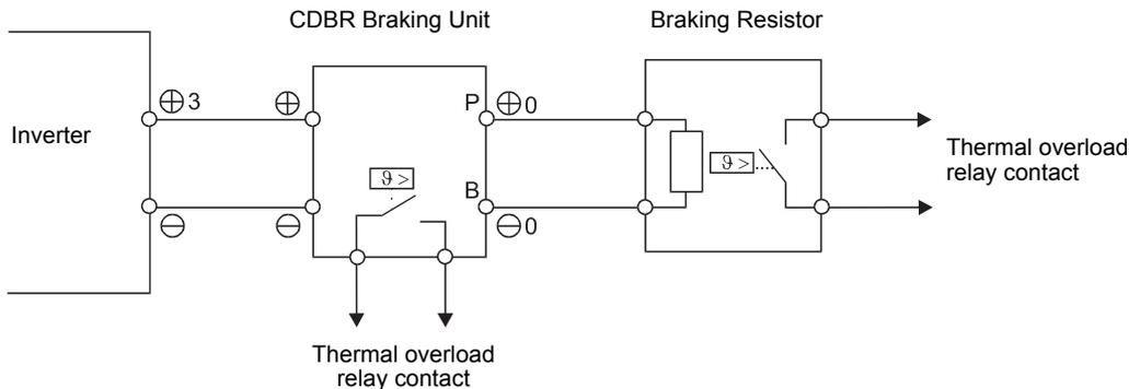
Fig 2.9 Connecting the Braking Resistor and Braking Unit
