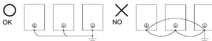
Fig 2.8 Ground Wiring
