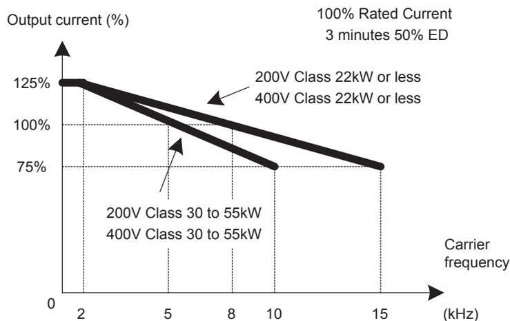
Fig 5.30 Current Derating depending on the carrier frequency
