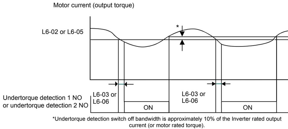
Fig 5.44 Undertorque Detection
