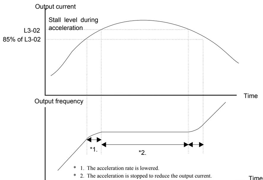
Fig 5.38 Time Chart for Stall Prevention During Acceleration
