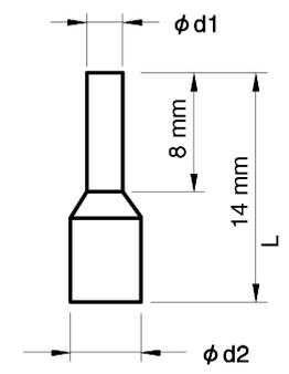
Fig 2.12 Straight Solderless Terminal Sizes
