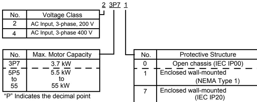
Fig 1.3 Inverter Specifications
