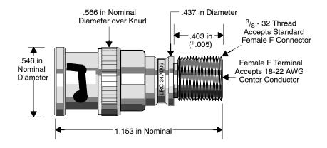
The 52-0614-000 Adapter permits the F connector on an RG-11 trunk cable to be attached to the BNC connector on an RIO processor at the network head-end or the F connector on an RG-11 drop cable to be connected to a J810/J812 or J890/J892 drop adapter at the drop.
