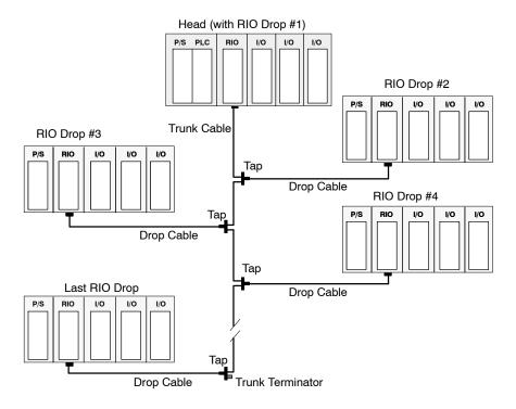
**Note** Because this example uses local I/O at the head, the first remote drop in the network will be I/O mapped as drop #2. If the PLC you are using does not support local I/O e.g., the 984A/B PLCs then the first drop in the I/O network will be I/O mapped as drop #1.
