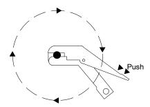
Step 3 If the cable is not fully stripped, squeeze the jaws of the tool together with your thumb and forefinger. Using light pressure, make one or two revolutions of the tool around the cable until the tool cuts through the cable jacket.
