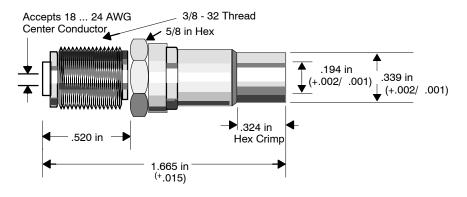
Both of these self-terminating F adapters have a return loss of 22 dB, a frequency range from 100 kHz  $\dots$  30 MHz, and an insertion loss of 0.03 dB.
