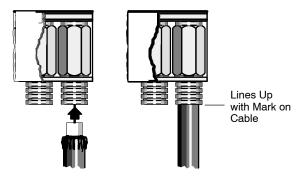
Step 3 Remove the F connector by sliding it out the side of the cassette.
