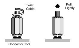
Step 7 Disconnect the F connector from the installation tool.
