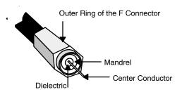
Step 4 Tighten the F connector nut onto the 60-0528-000 RG-6 Installation Tool connector with a <sup>7</sup>/<sub>16</sub> in torque wrench to 47 ... 57 in/lb of torque. Then pull on the cable to test the integrity of the connection. If the cable pulls out of the connector, begin the procedure again.
