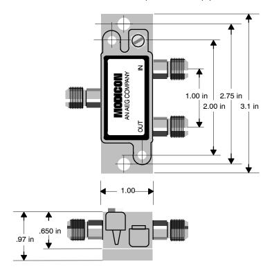
**Note** Although the trunk ports are labeled IN and OUT, these labels can be ignored i.e., the tap is not directional.
