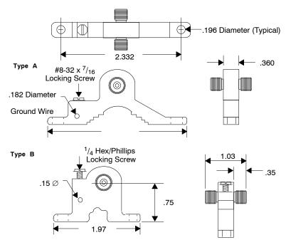
A special ground block with a gas-filled surge suppressor is available for outside installations or any other installations where the cable is exposed to lightning. Surge suppressors have a very low insertion loss, and they usually are not figured into the attenuation calculations unless five or more are used in that case, calculate an extra .2 dB into the trunk attenuation. A surge suppressor has a 75  $\Omega$  impedance, a return loss of >40 dB, and has a wide application frequency range.
