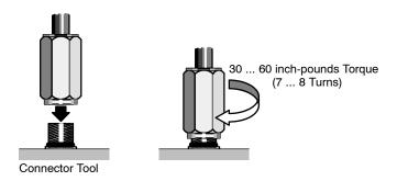
Step 5 Twist the cable directly behind the F connector. If the cable turns, apply more torque until no movement is observed. If the F connector has been completely torqued and/or bottomed out and the cable still twists, start the procedure over using another F connector in the 52-0401-000 cassette.
