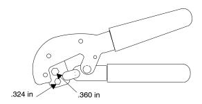
The Modicon 043509432 Crimp Tool is used to install BNC connectors onto RG-6 cable. The tool makes two sizes of hex crimp: 0.276 and 0.325 in.
