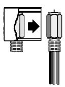
Step 4 Align the 60-0544-000 Crimp Tool on the F connector, and apply a .360 in crimp.
