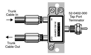
Step 3 Connect the F connector on the drop cable to the drop-cable tap port.
