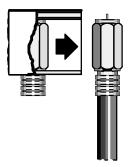
Step 3 Visually inspect the cable insertion depth by looking into the end of the F connector the white dielectric should be flush with the end of the mandrel.
