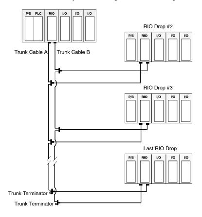
The two cables are treated as two separate networks, and each cable is an independent system running from the same RIO processor node to the same remote I/O drops. If a break occurs in cable A or cable B, an LED goes ON at the RIO head processor. The condition is also logged in words 179 ... 277 of the status table; these status words can be accessed via the STAT instruction (see *Modicon Ladder Logic Block Library User Guide*, 840 USE 101 00).
