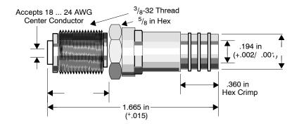
□ A Modicon 52-0399-000 model for non-quad shield cable
