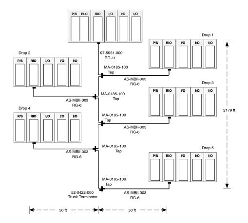
This system uses (Modicon 97-5951-000) RG-11 cable for the trunk; its specified attenuation is 0.24 dB/100 ft at 1.544 MHz. Running to the adapter at drop 5 is a Modicon AS-MBII-003 RG-6 drop cable, a 50 ft cable with an attenuation of 0.3 dB. To calculate end-to-end attenuation on the trunk cable (TCA), multiply 0.24 dB (the trunk attenuation per 100 ft) by 21.79:
