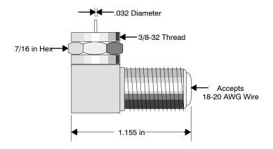
Modicon has also approved the FF90FM right-angle F adapter manufactured by LRC Electronics and the GFMF/90 right-angle F adapter manufactured by Gilbert Engineering.
