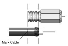
Step 2 Using a twisting motion, push the cable firmly into the end of the F connector in the MA-0329-001 Cassette until the cable mark lines up with the end of the crimp ring.
