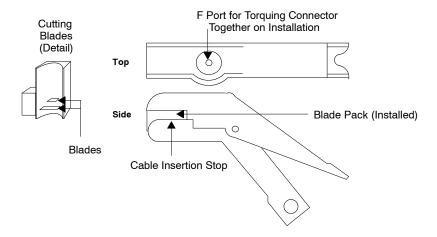
Make adjustments in the number of rotations so that the second blade cuts as little of the braid as possible. Usually the first blade has cut through the shields when the crackling noise stops. Apply some pressure to the tool while rotating it once more after the crackling stops to cut through the remaining dielectric, then pull off the cut cable. This method usually saves as much braid as possible.
