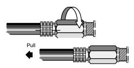
Step 5 If the connection holds, disconnect the F connector from the tool and install it onto the cable port of the RIO drop adapter, tap, or other cable hardware device using a  $^{7}/_{16}$  in open-end wrench.
