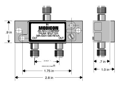
MA-0186-100 splitters have a minimum return loss of 18 dB on each port. Any unused port must be terminated. The splitter is installed between two PLCs in the main trunk cable and has three connectors (ports) on it. Each port is attenuated 6 dB from the other ports. All ports are split equally.
