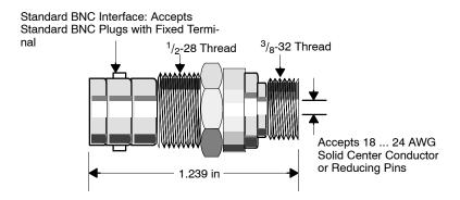
The 52-0370-000 Self-terminating BNC Adapter has a return loss of 40 dB, a frequency range from 100 kHz  $\dots$  30 MHz, and an insertion loss of 0.03 dB.
