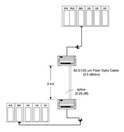
The specified power loss budget for a link using this optical cable is 11 dB. We know that the cable s attenuation over 3 km is  $3.5 \, dB/km \times 3 = 10.5 \, dB$ , and we are given an attenuation of  $0.25 \, dB$  for the cable splice. Thus, we have a total optical power loss of  $10.75 \, dB$  on the link, which is under budget and therefore legal.
