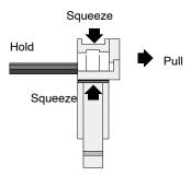
Step 4 Open the jaws and remove the cable. The dielectric plug and <sup>1</sup>/<sub>8</sub> in of the outer cable jacket should be cut from the cable. Remove any long braid strands remaining around the prepared cable end. (Long braid strands may indicate that a new blade pack is needed.) Remove any dielectric on the exposed center conductor.
