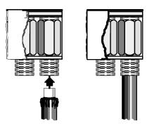
Step 2 Remove the F connector by sliding it out the side of the cassette.
