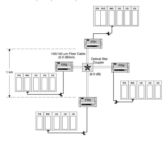
The specified power loss budget for a link using this optical cable is 16.5 dB. The cable attenuation over 1 km is 5 dB, and an attenuation of 8 dB is specified for the star coupler device itself. Two ST connectors for the Tx and Rx lines through the star coupler incur 1 dB loss each. Thus, we have a total optical power loss of:
