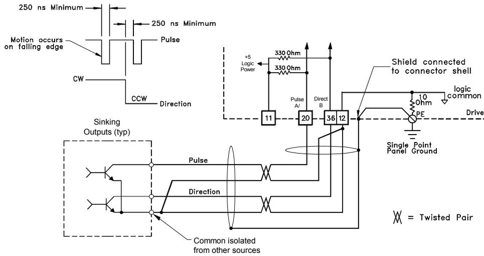
Figure 51: Pulse Mode, Single Ended Output to Single Ended Input (twisted pair cable)
