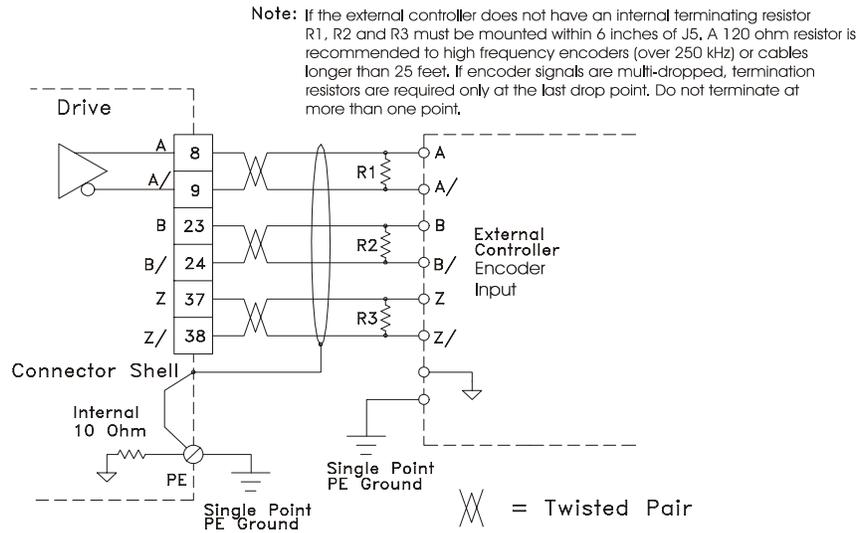
Figure 47: Command Connector (J5) Encoder Output Wiring
