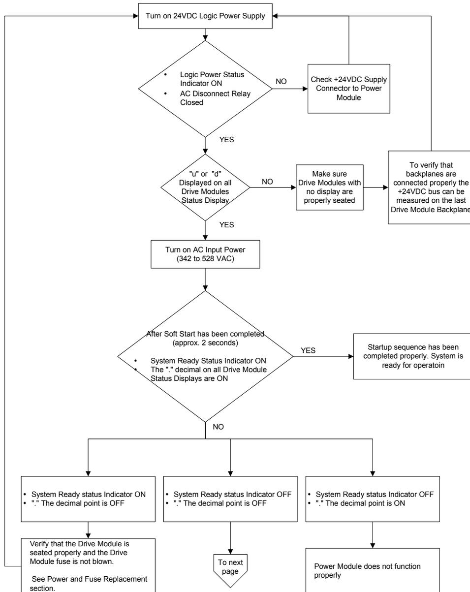
Figure 59: Power Up Sequence Flow Chart - Part 1
