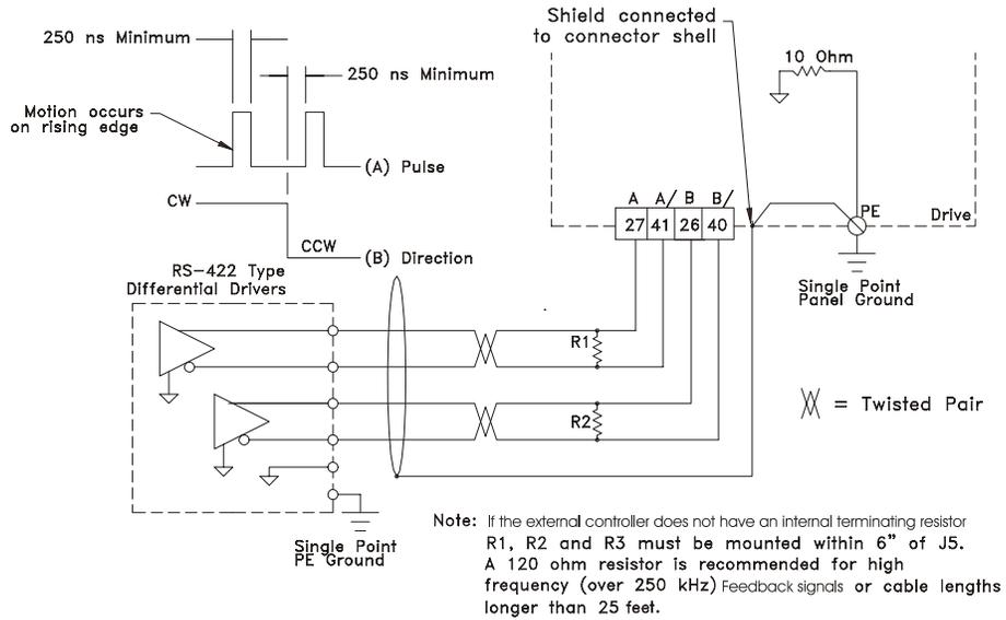
Figure 49: Pulse Mode, Differential Output to Differential Input
