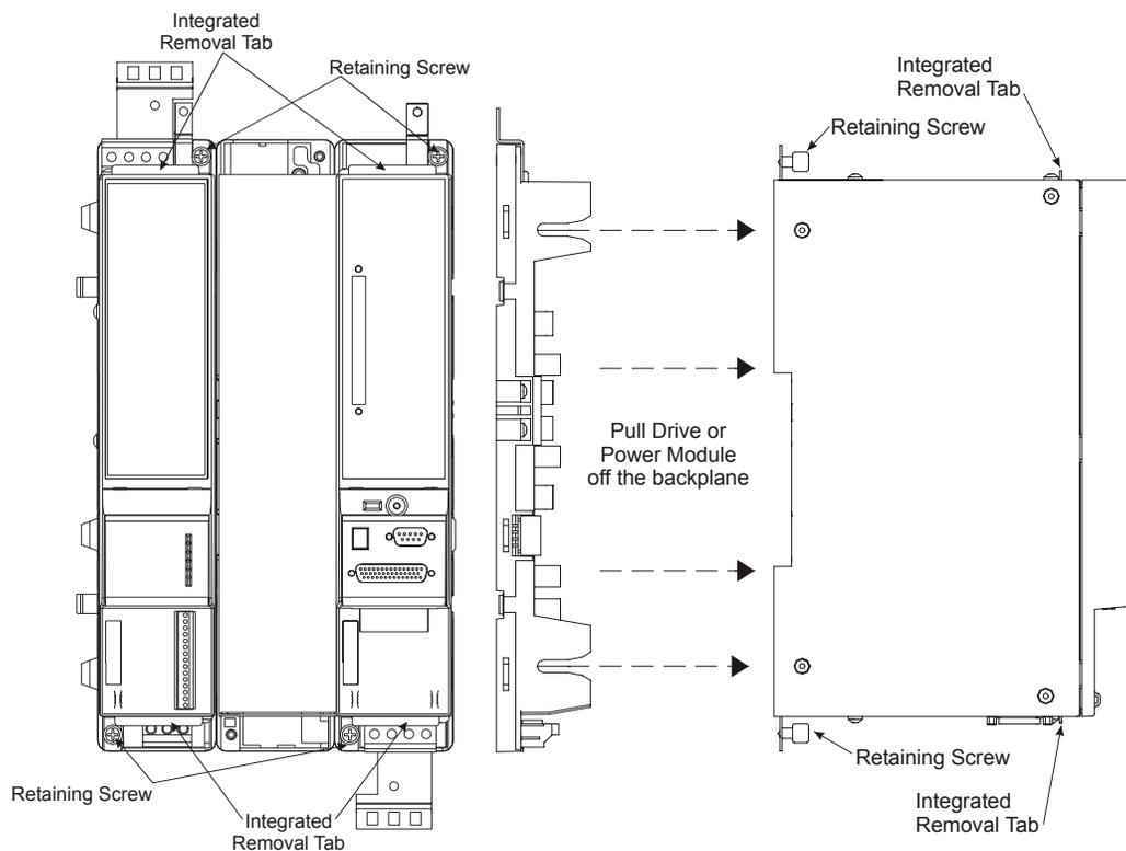
Figure 62: Power and Drive Module Removal Diagram
