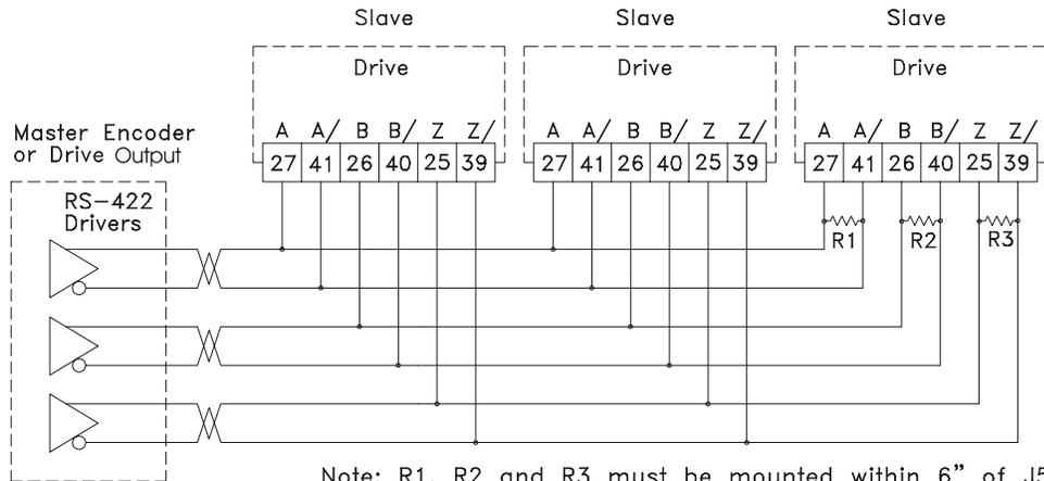
Note: R1, R2 and R3 must be mounted within 6" of J5. A 120 ohm resistor is recommended for high frequency (over 250 kHz) stepping or cable lengths longer than 25feet.
