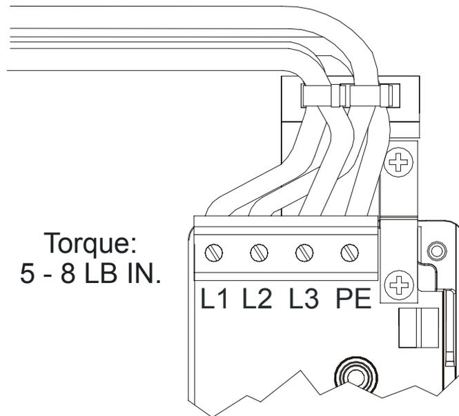
Figure 21: Power Module AC Power Wiring Diagram
