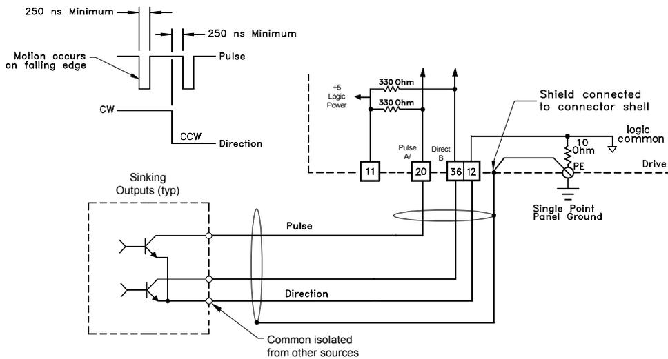
Figure 52: Pulse Mode, Single Ended Output to Single Ended Input (non-twisted pair cable)
