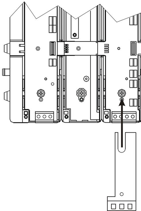
*Figure 14: Installing the Optional Cable Strain Relief Bracket*
