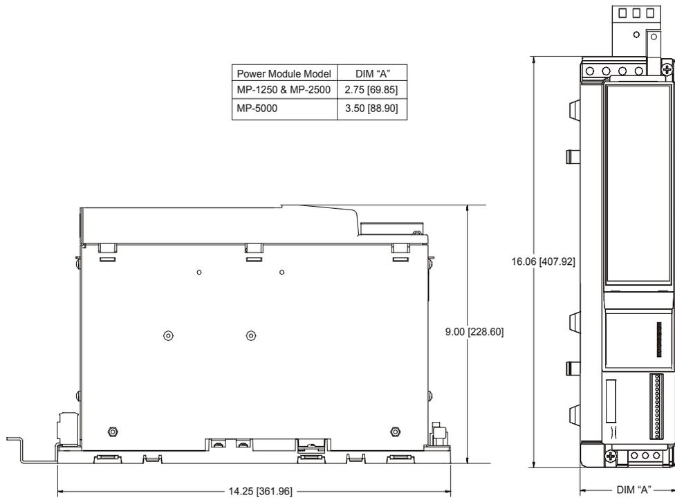
Figure 7: Power Module Dimensions - MP-5000 Shown
