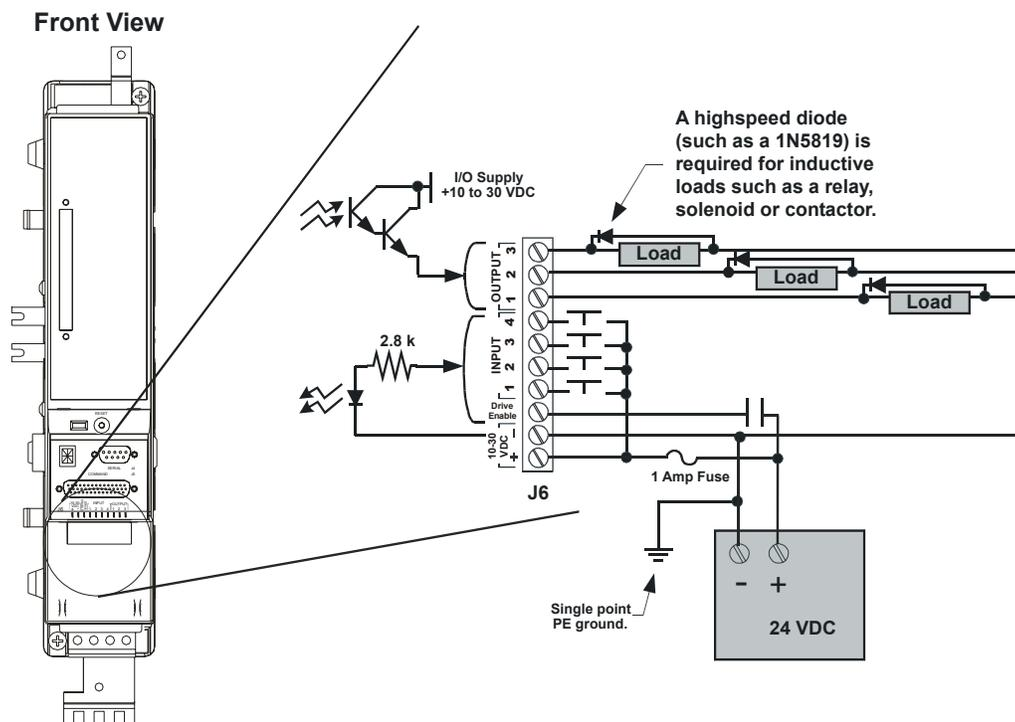
Figure 40: MDS Drive Module Input/Output Wiring Diagram
