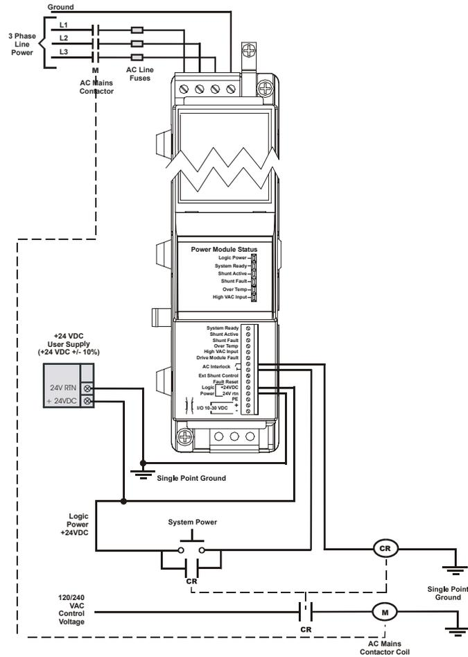
Figure 37: AC Interlock with 120/240VAC Mains Contactor
