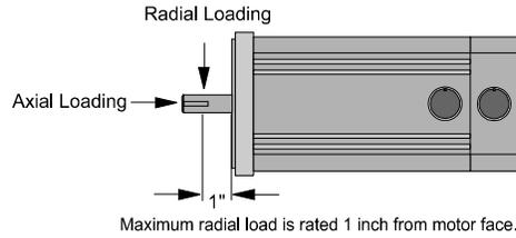
Figure 71: Axial/Radial Loading
