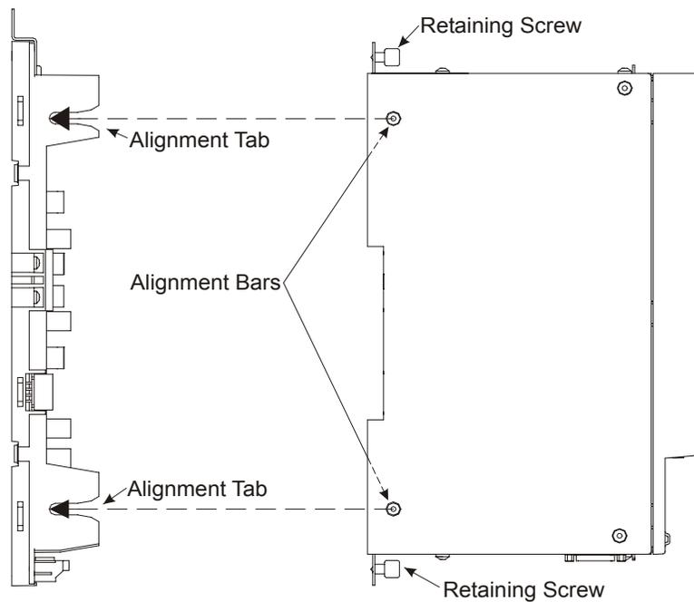
Figure 28: Drive Module Assembly Diagram
