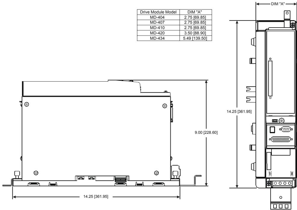
Figure 10: Drive Module Dimensions - MD-420 Shown
