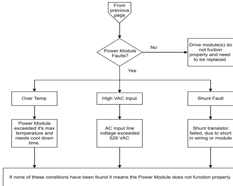
Figure 60: Power Up Sequence Flow Chart - Part 2
