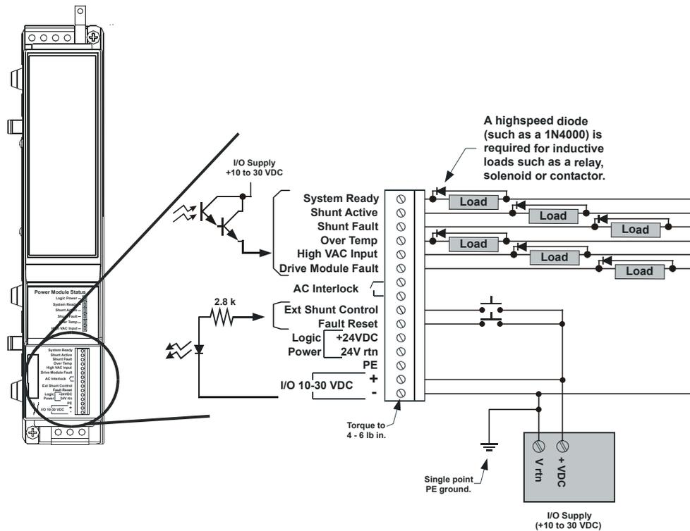
Figure 35: Power Module I/O Wiring Diagram
