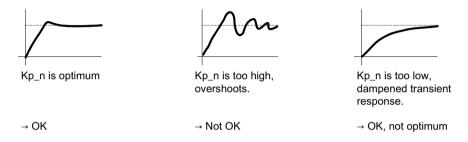
Figure 5-16 Setting the proportional gain K<sub>p</sub>
