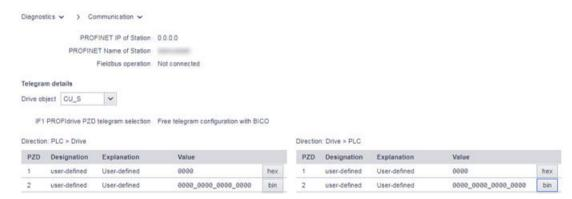
Figure 13-14 Example: Communication display area
