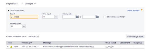
Figure 13-12 Example: Filtering messages
