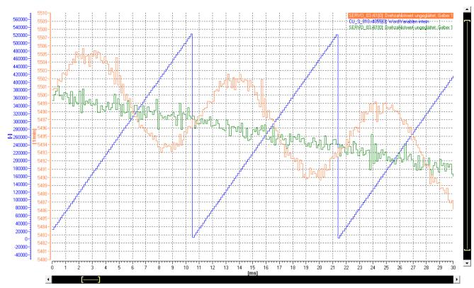
Figure 9-57 Example: Speed before and after compensation
