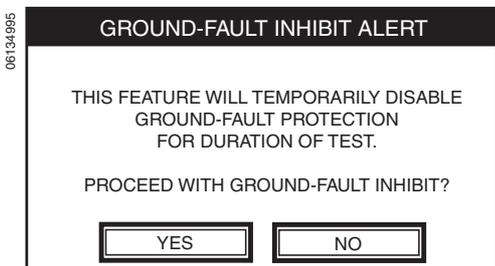
**Figure 48: Ground-fault Inhibit Initializing Screen**
