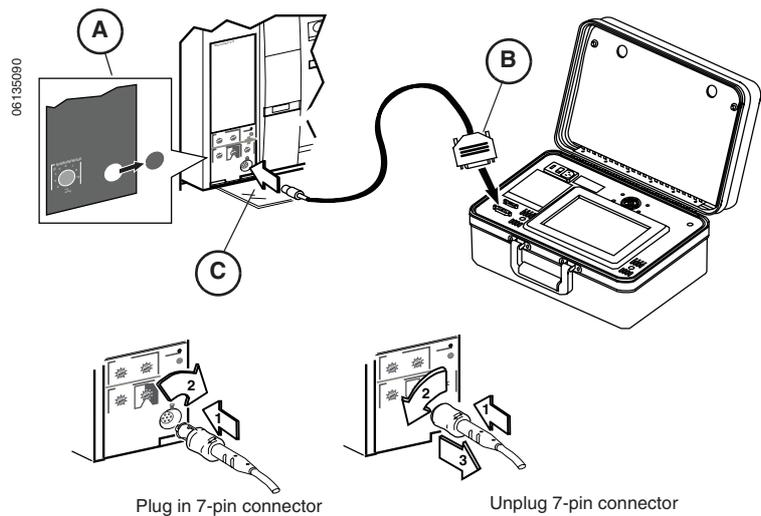
**NOTE: Older ET1.0 trip units have the test port covered. Cut the label (A) as shown to access the trip unit port.**
